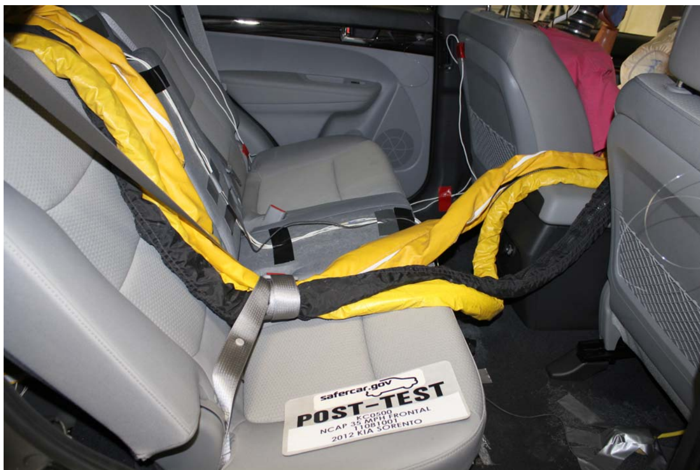
Post-Test Dummy Cable Routing
