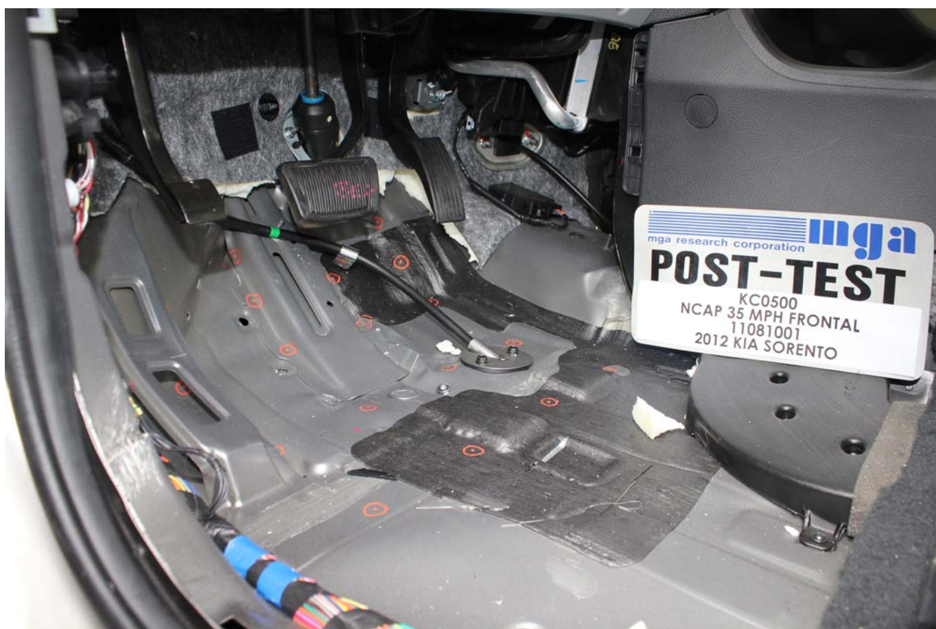
Post-Test Driver's Side Floorpan
