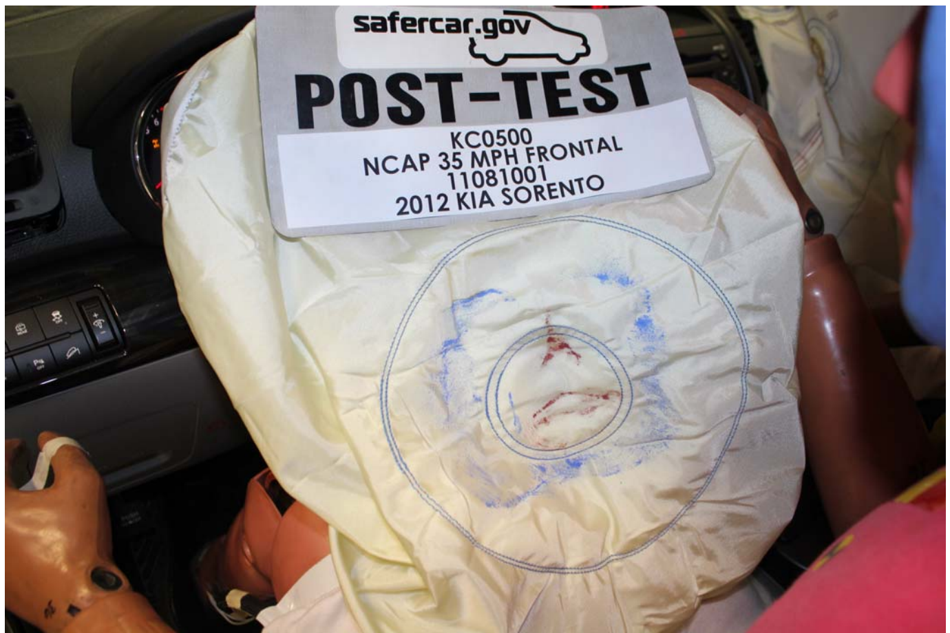
Post-Test Driver Dummy Contact with Airbag
