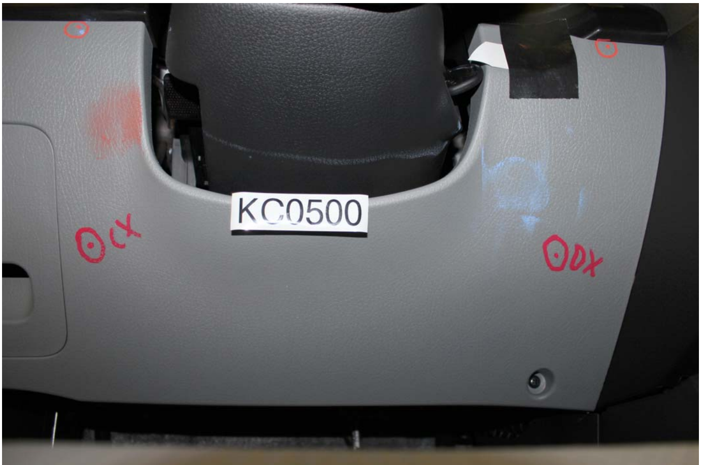
Post-Test Driver Dummy Contact with Knee Bolster
