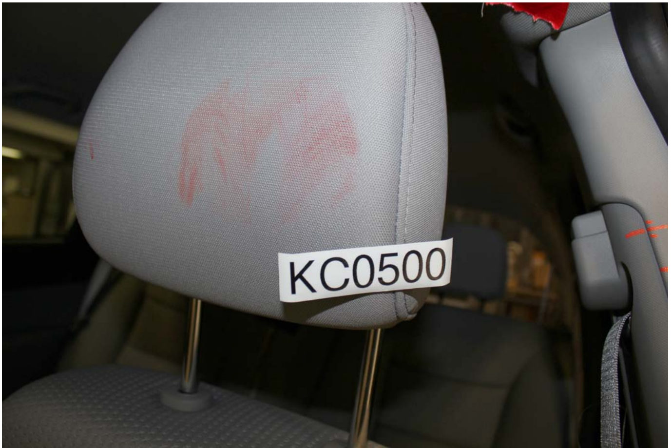
Post-Test Driver Dummy Contact with Headrest
