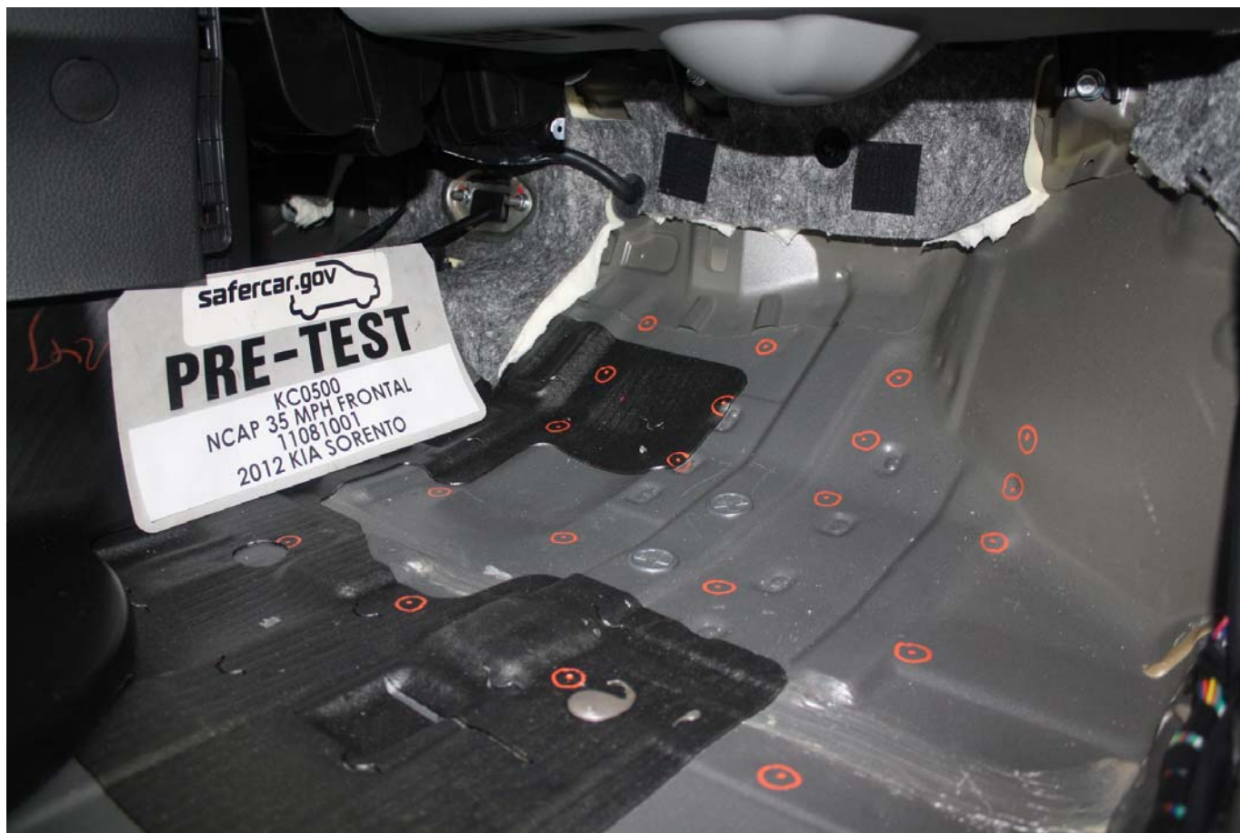
Pre-Test Passenger's Side Floorpan
