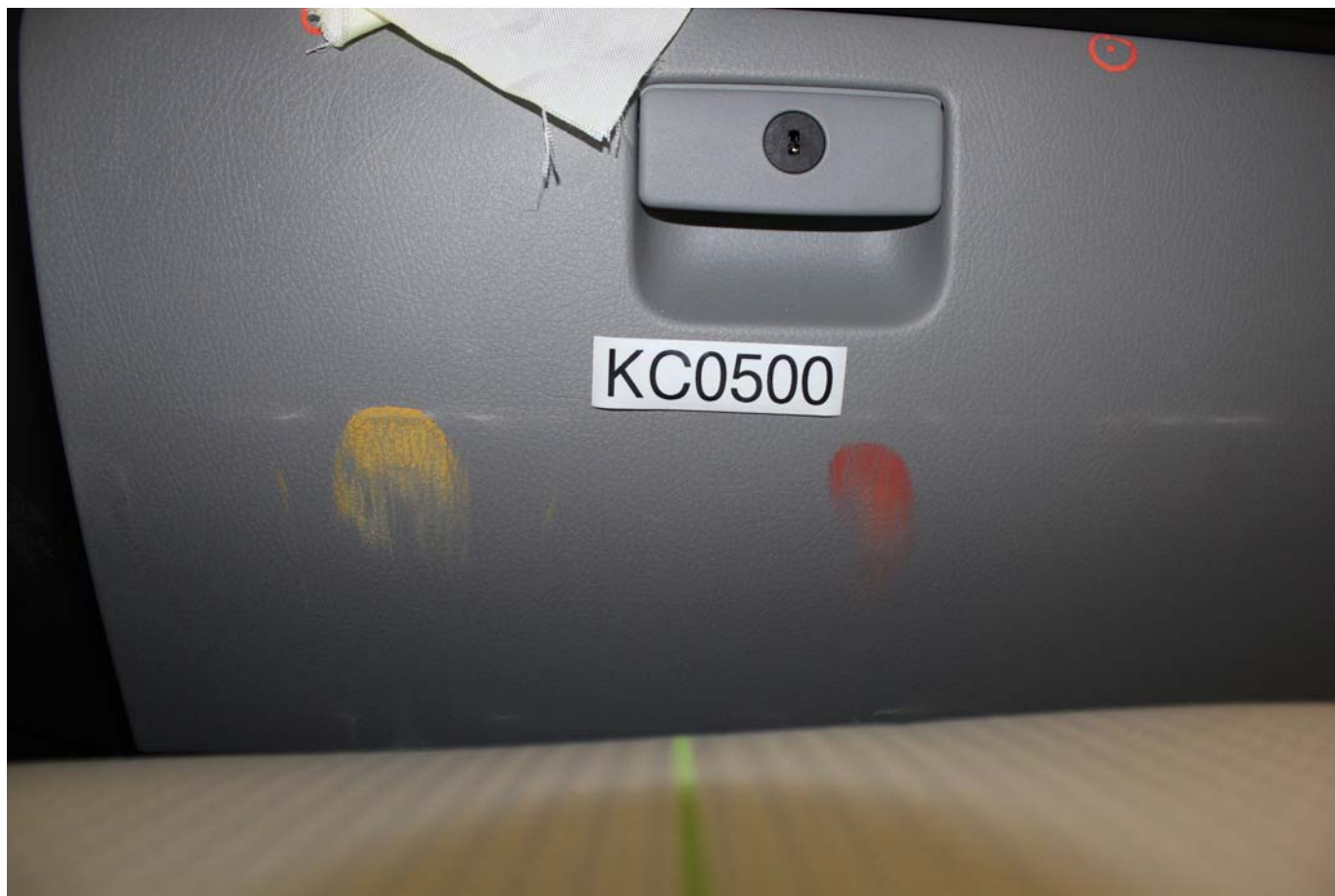
Post-Test Passenger Dummy Contact with Glovebox
