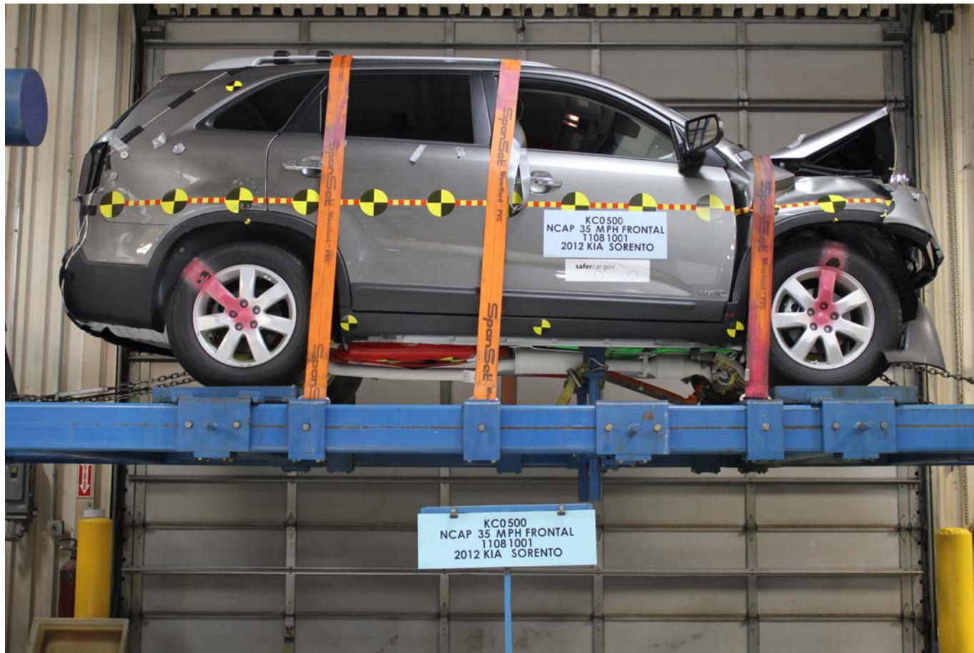
Vehicle at 360 Degrees on Static Rollover Device
