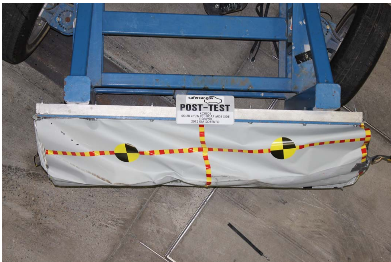
Post-Test Top View of MDB Impactor Face
