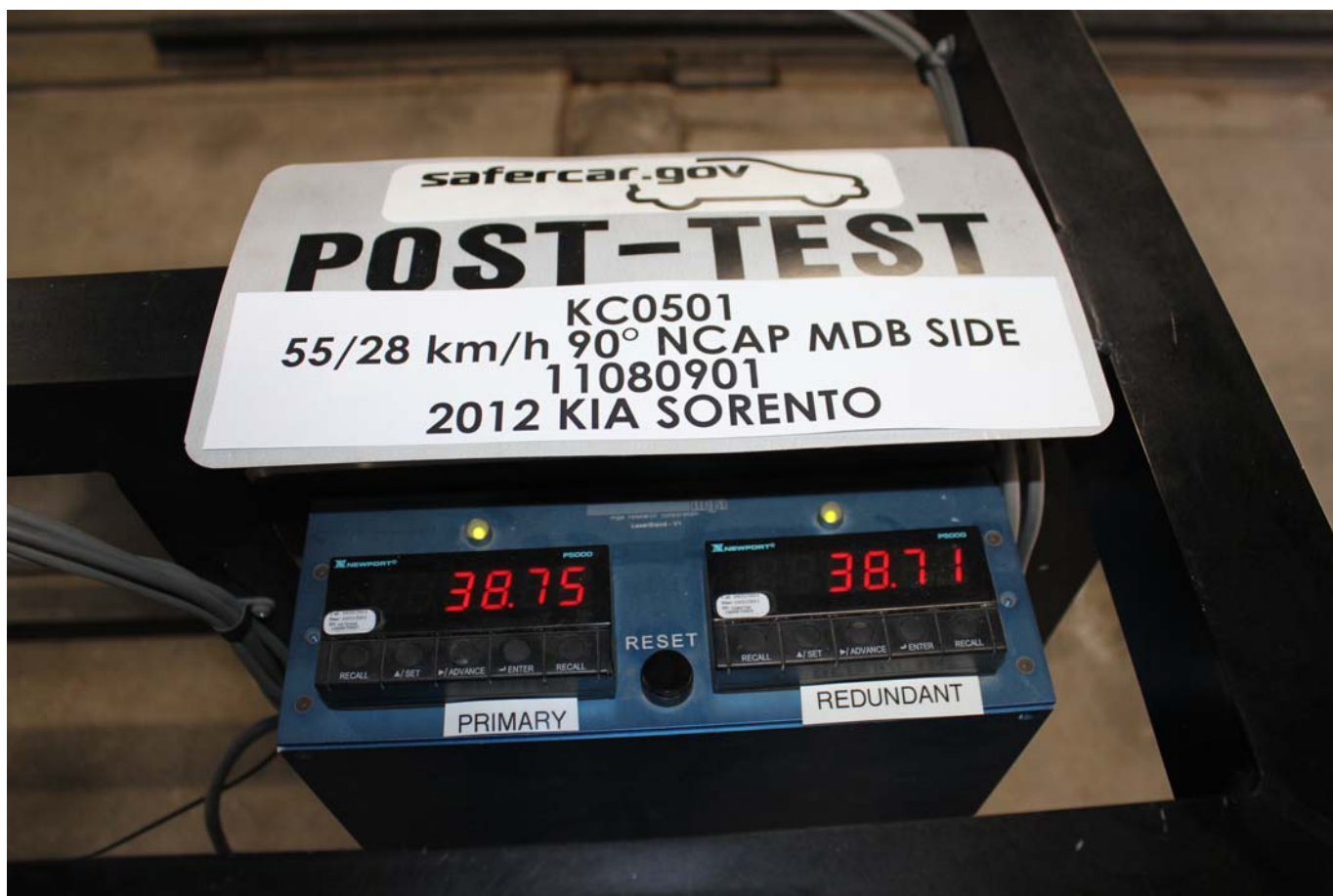
Post-Test Primary and Redundant Speed Trap Read-Out
