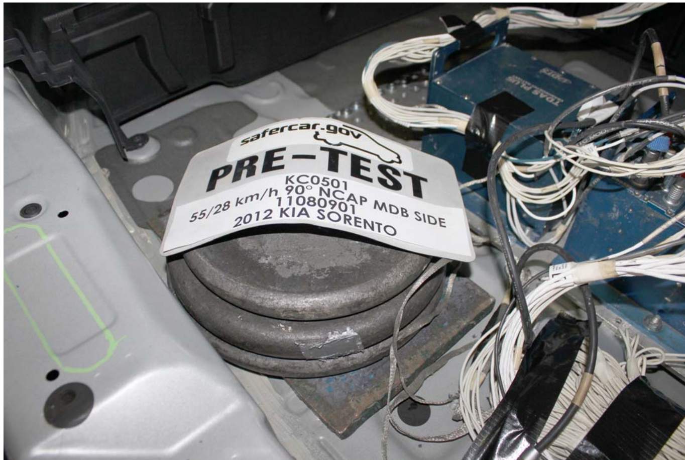
Pre-Test Ballast View
