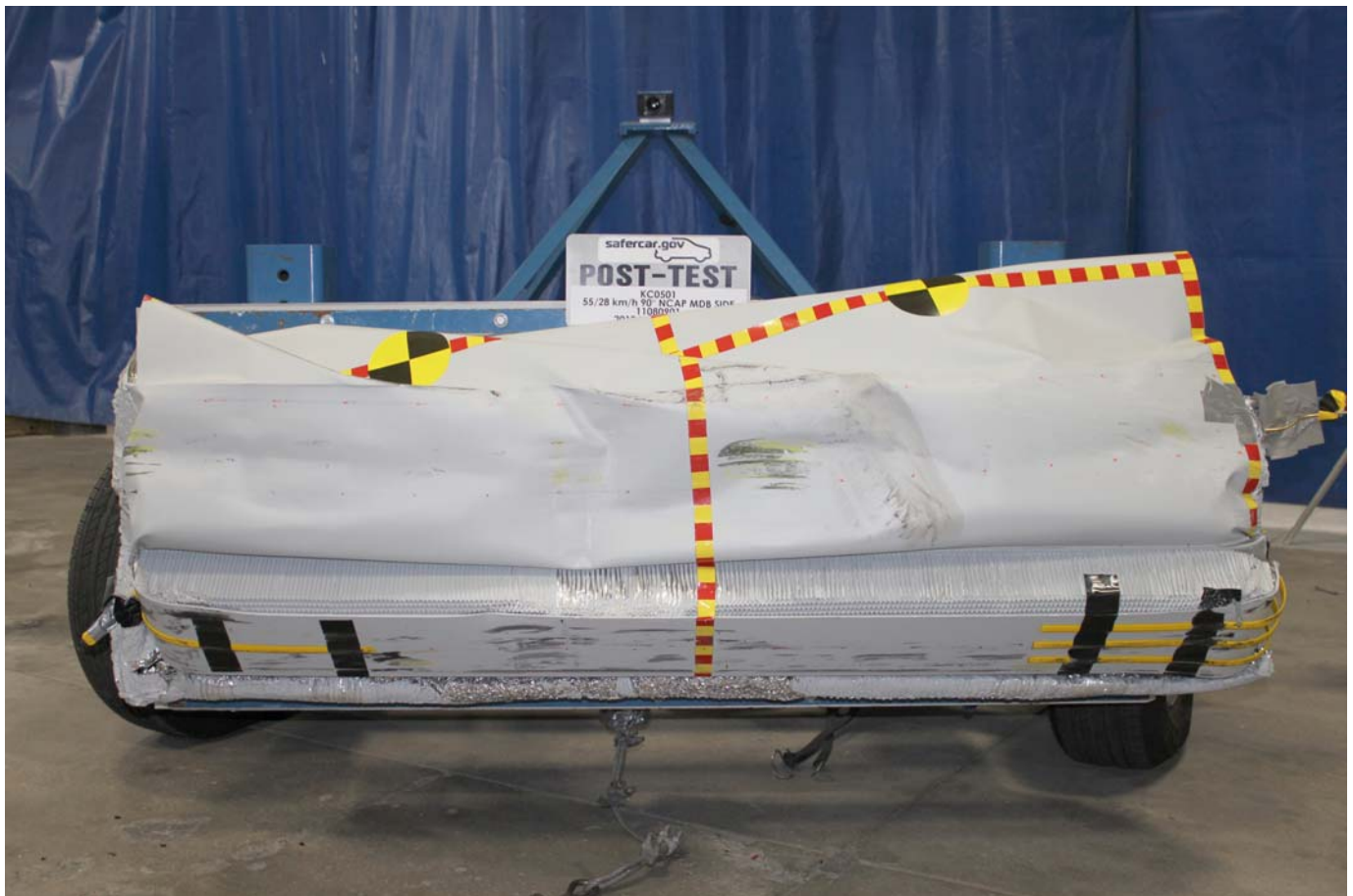
Post-Test Front View of MDB Impactor Face
