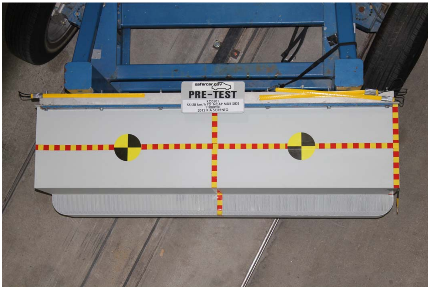
Pre-Test Top View of MDB Impactor Face
