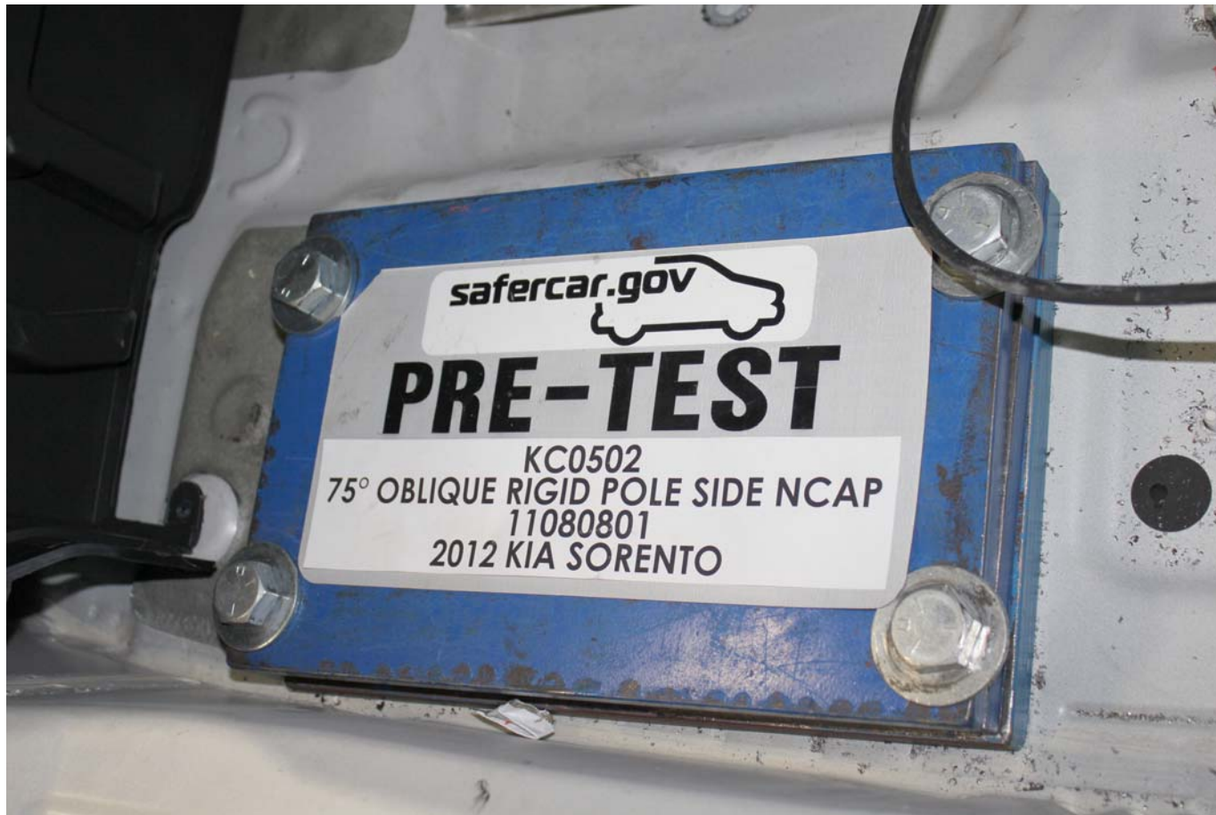
Pre-Test Ballast View
