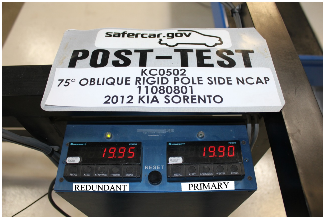
Post-Test Primary and Redundant Speed Trap Read-Out
