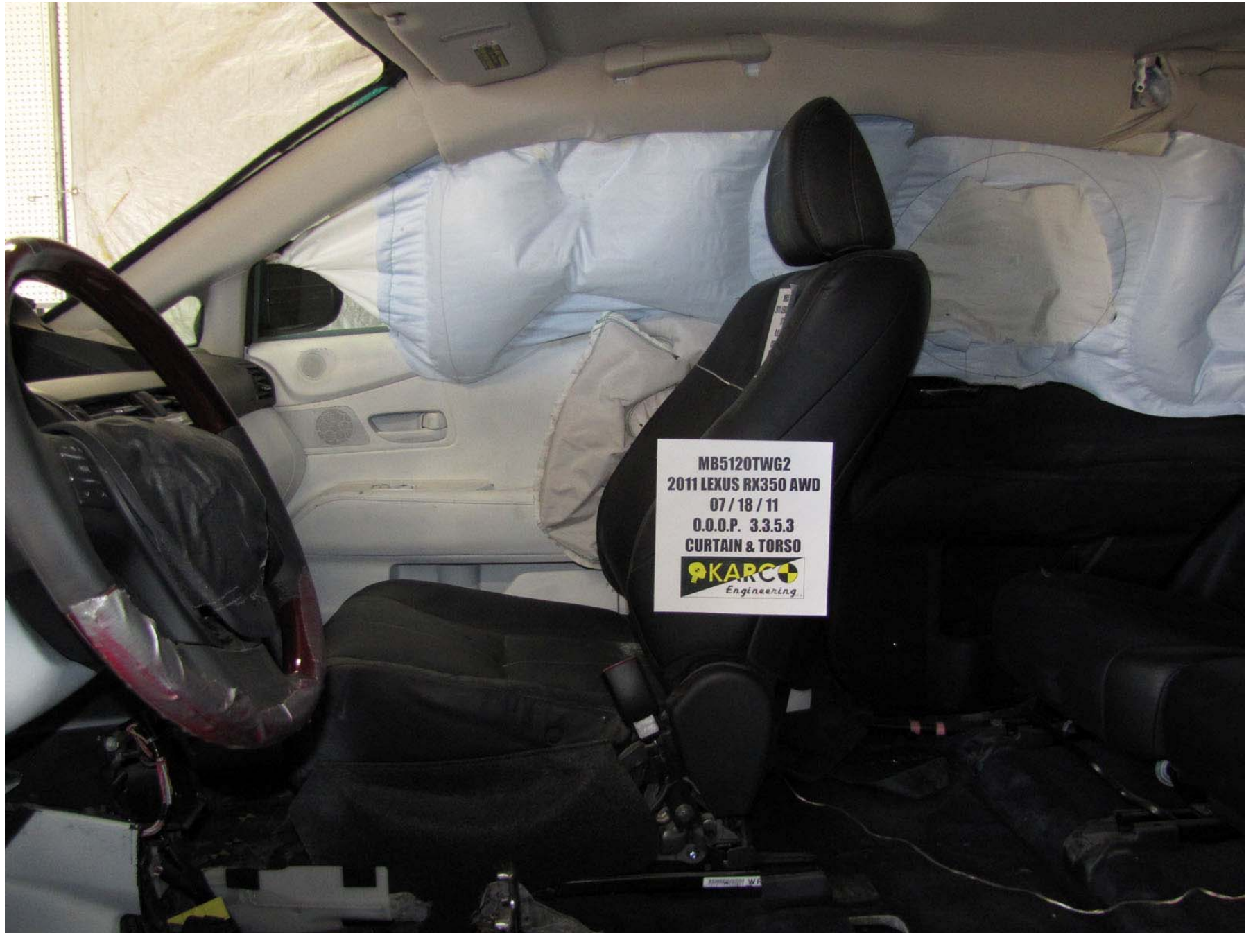
Figure A-9: Post-Test Airbags, Left Side View
