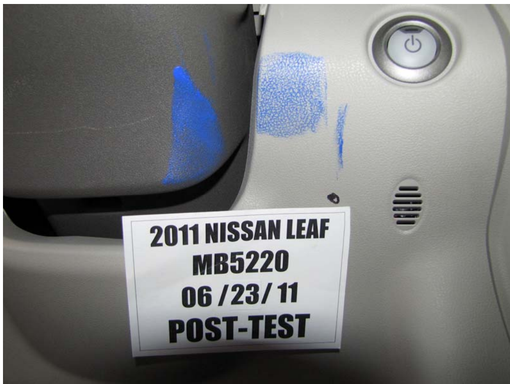
FIGURE 43c. Post-Test Driver Dummy Contact With Steering Column
