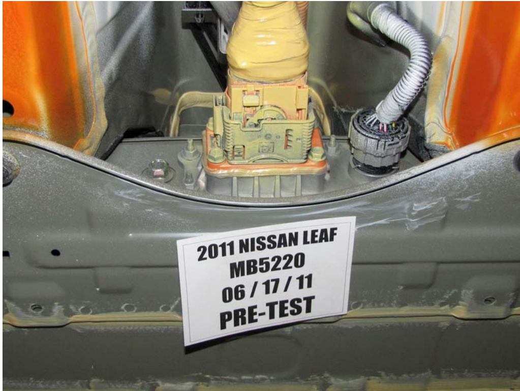
FIGURE 102. Pre-Test High Voltage Connections
