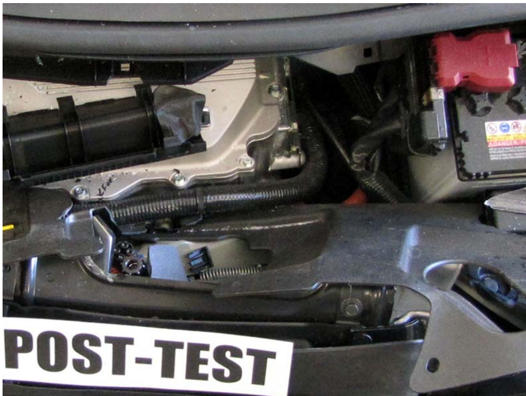
FIGURE 93. Post-Test High Voltage Connections
