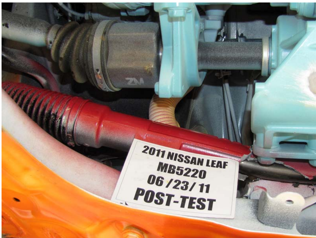
FIGURE 101. Post-Test High Voltage Connections
