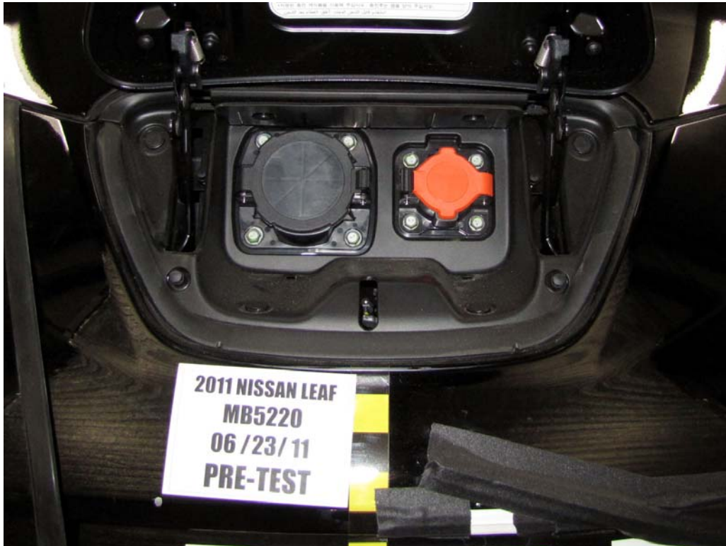
FIGURE 80. Pre-Test Battery Charging Port
