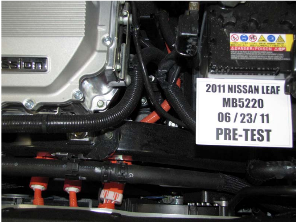
FIGURE 92. Pre-Test High Voltage Connections
