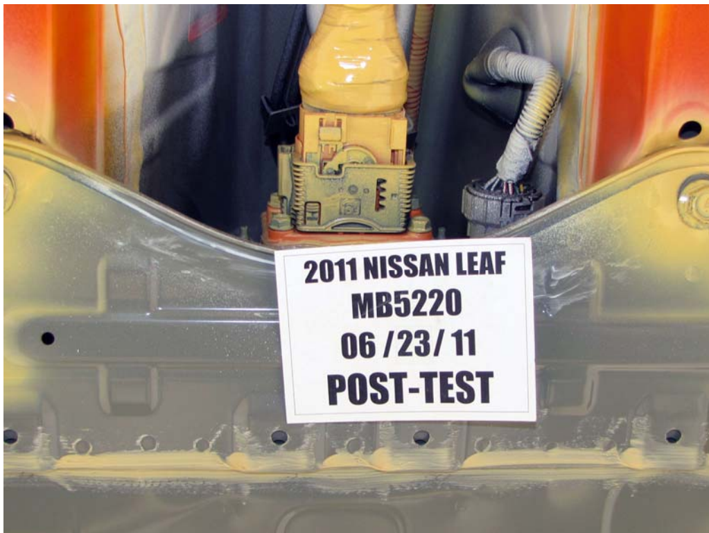
FIGURE 103. Post-Test High Voltage Connections
