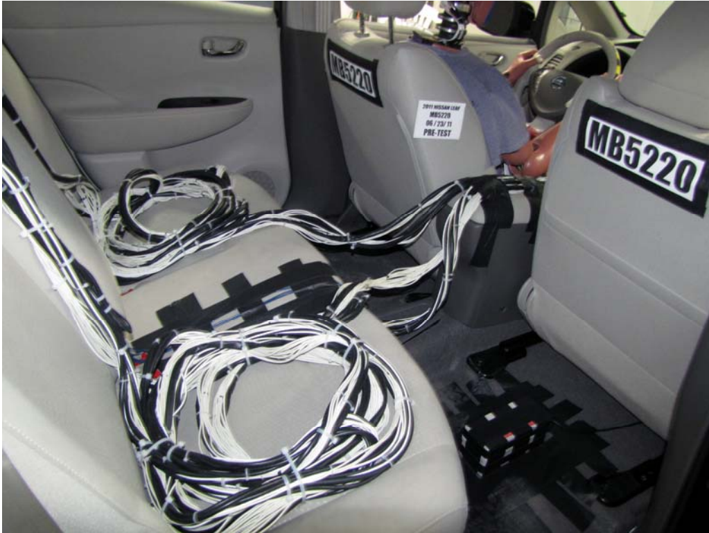
FIGURE 27. Pre-Test Dummy Cable Routing
