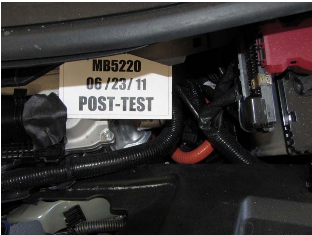
FIGURE 95. Post-Test High Voltage Connections
