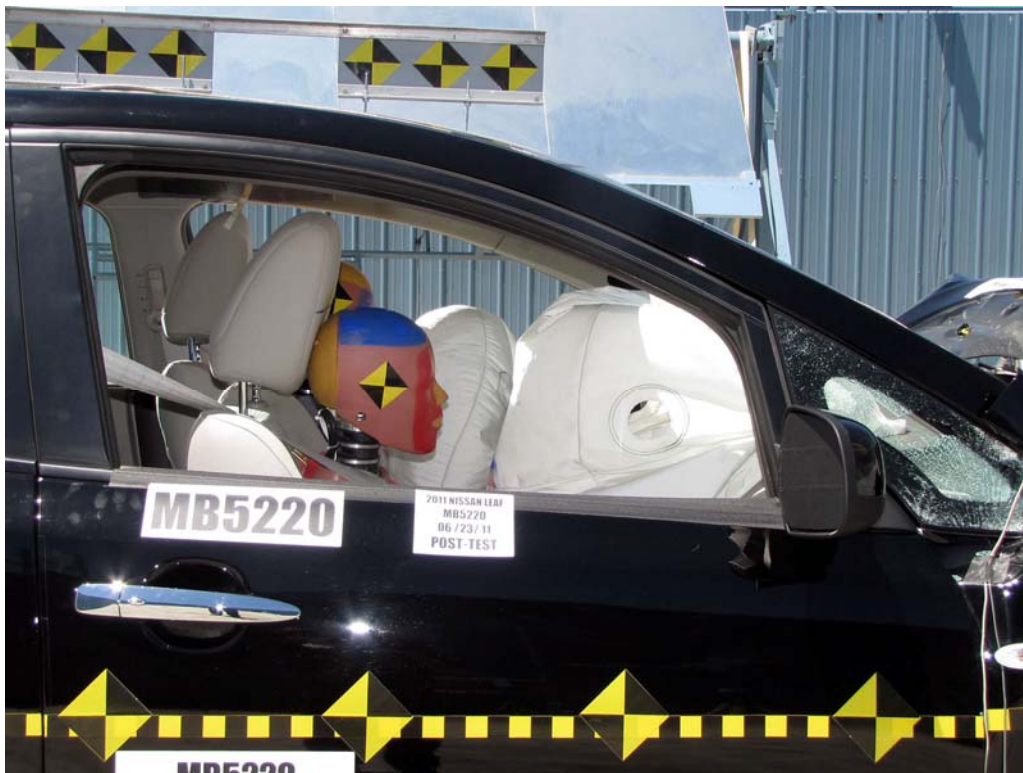
FIGURE 49. Post-Test Passenger Dummy Window View
