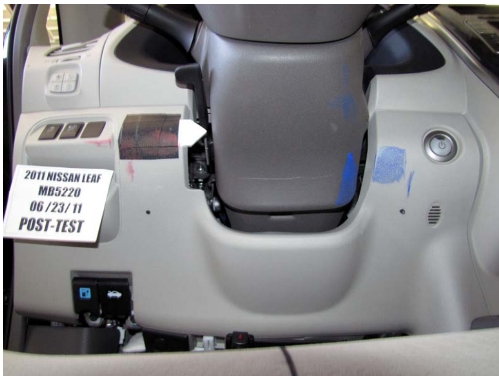
FIGURE 45. Post-Test View of Steering Column Shear Capsule
