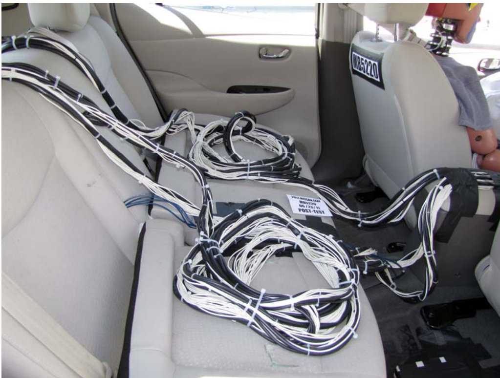
FIGURE 28. Post-Test Dummy Cable Routing
