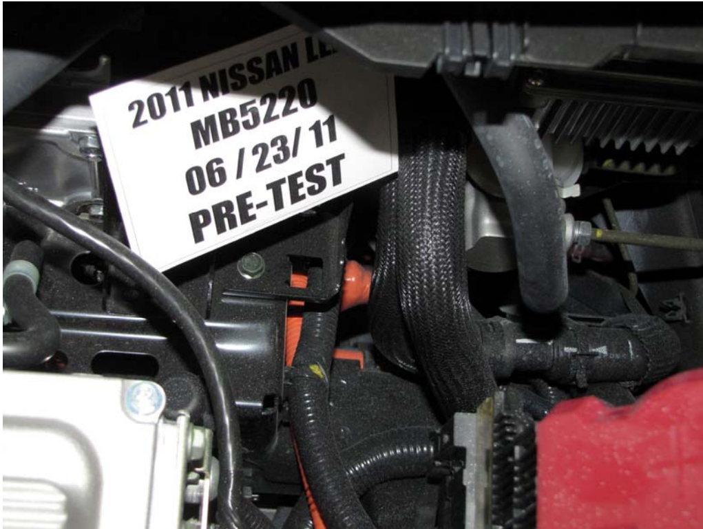
FIGURE 94. Pre-Test High Voltage Connections
