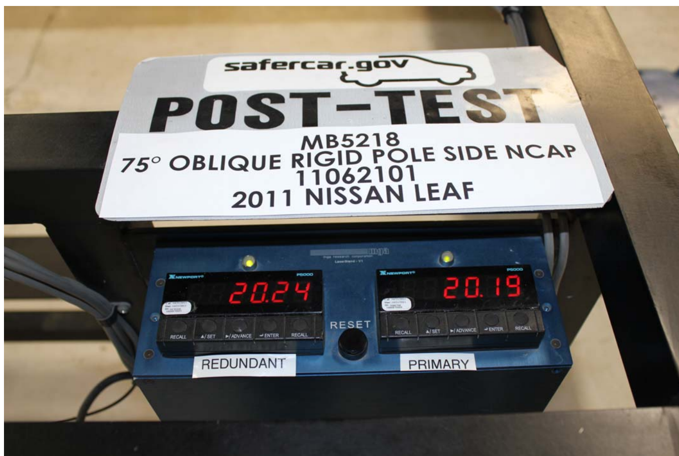
Post-Test Primary and Redundant Speed Trap Read-Out
