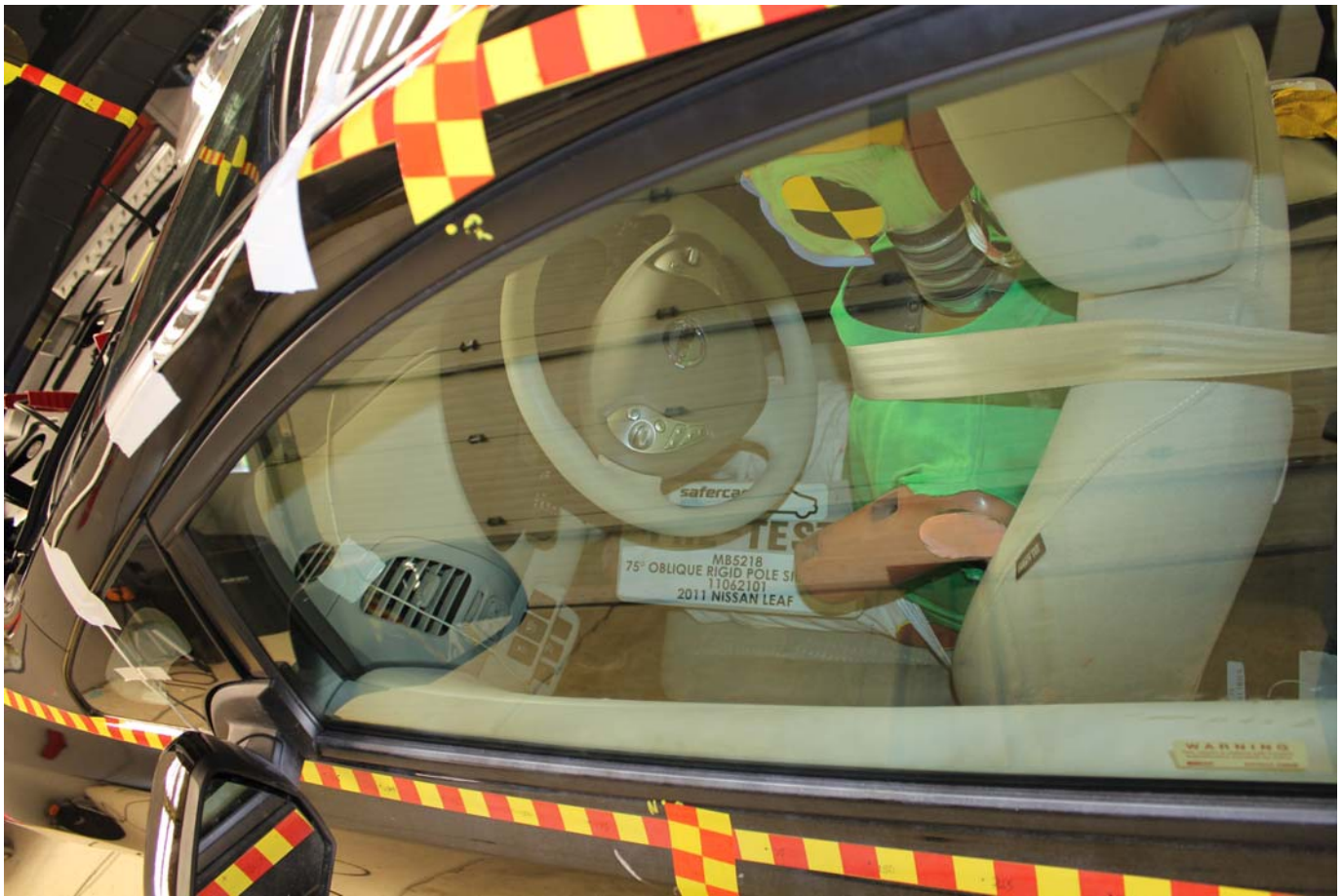
Pre-Test Dummy and Door Clearance View
