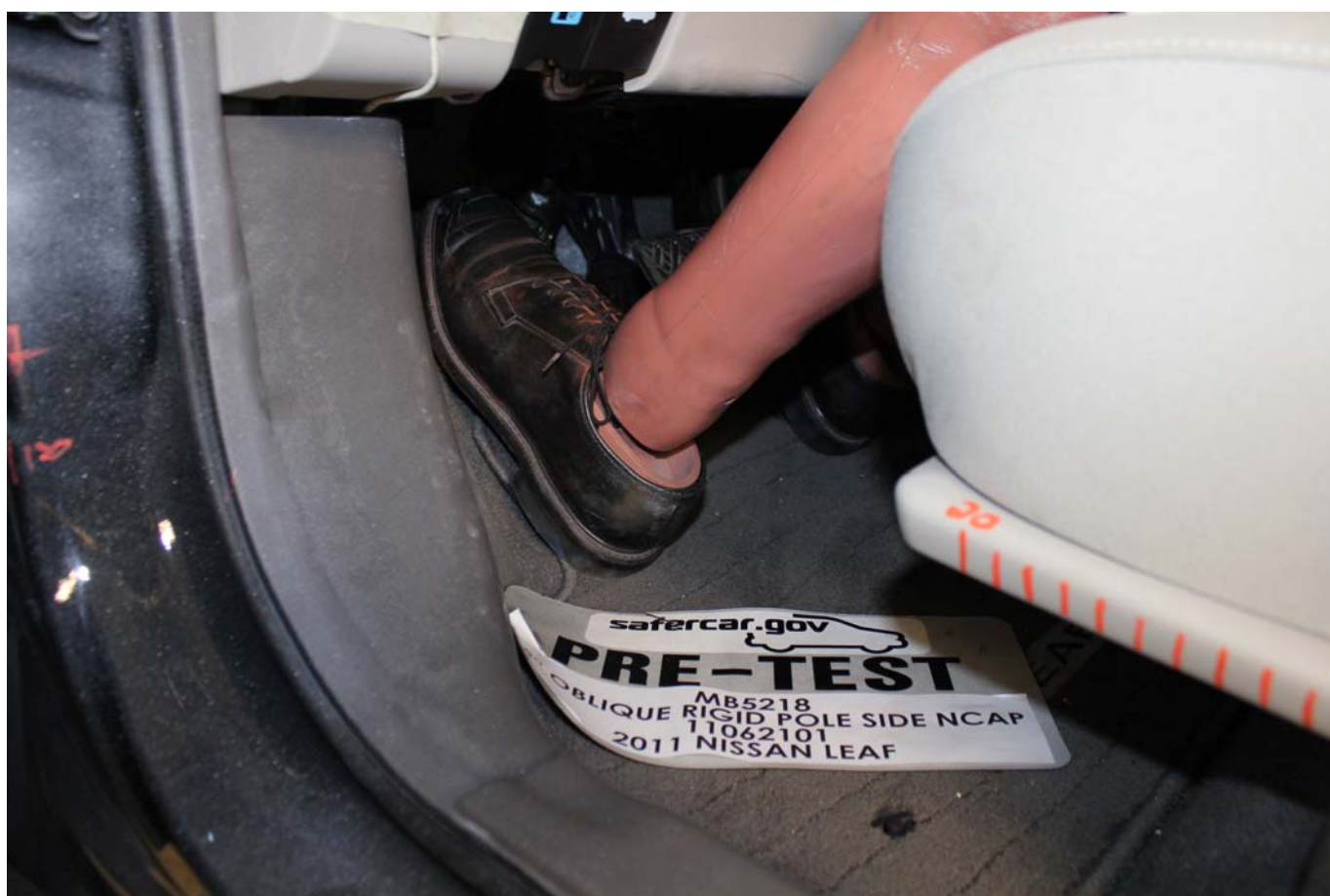
Pre-Test Placement of Dummy's Feet
