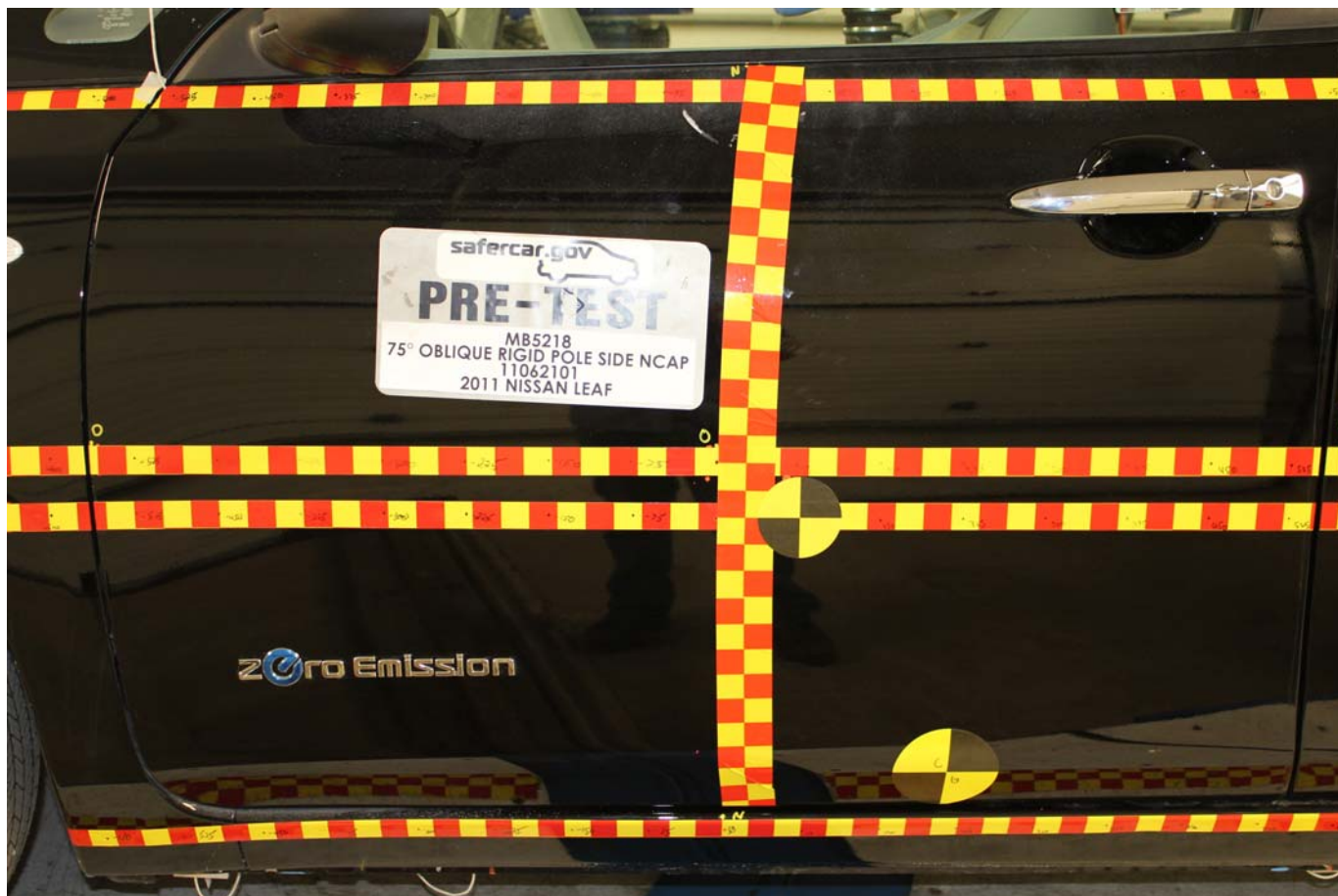
Pre-Test Close-Up View of Impact Point Target
