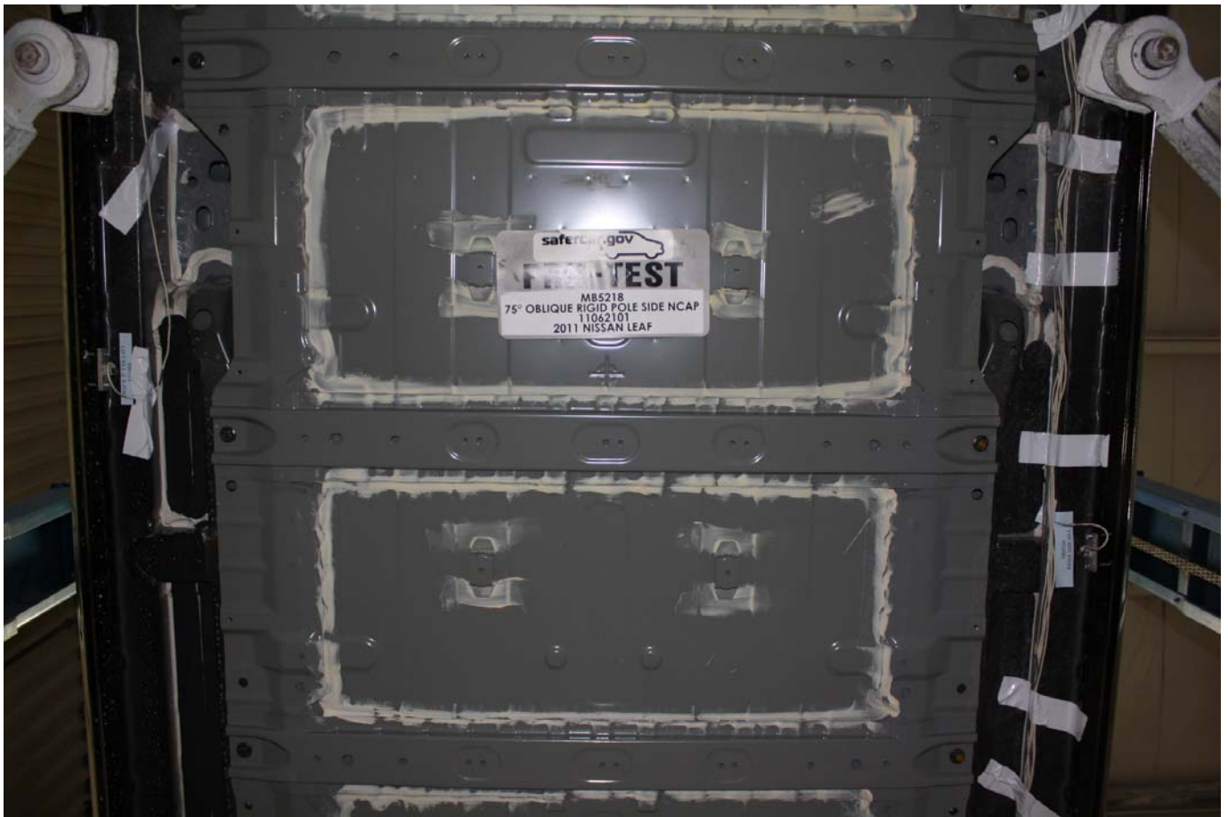
Pre-Test View of Propulsion Battery
