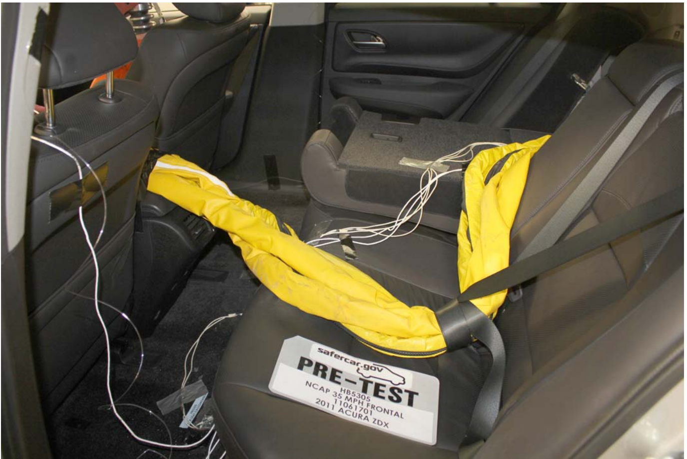
Pre-Test Dummy Cable Routing
