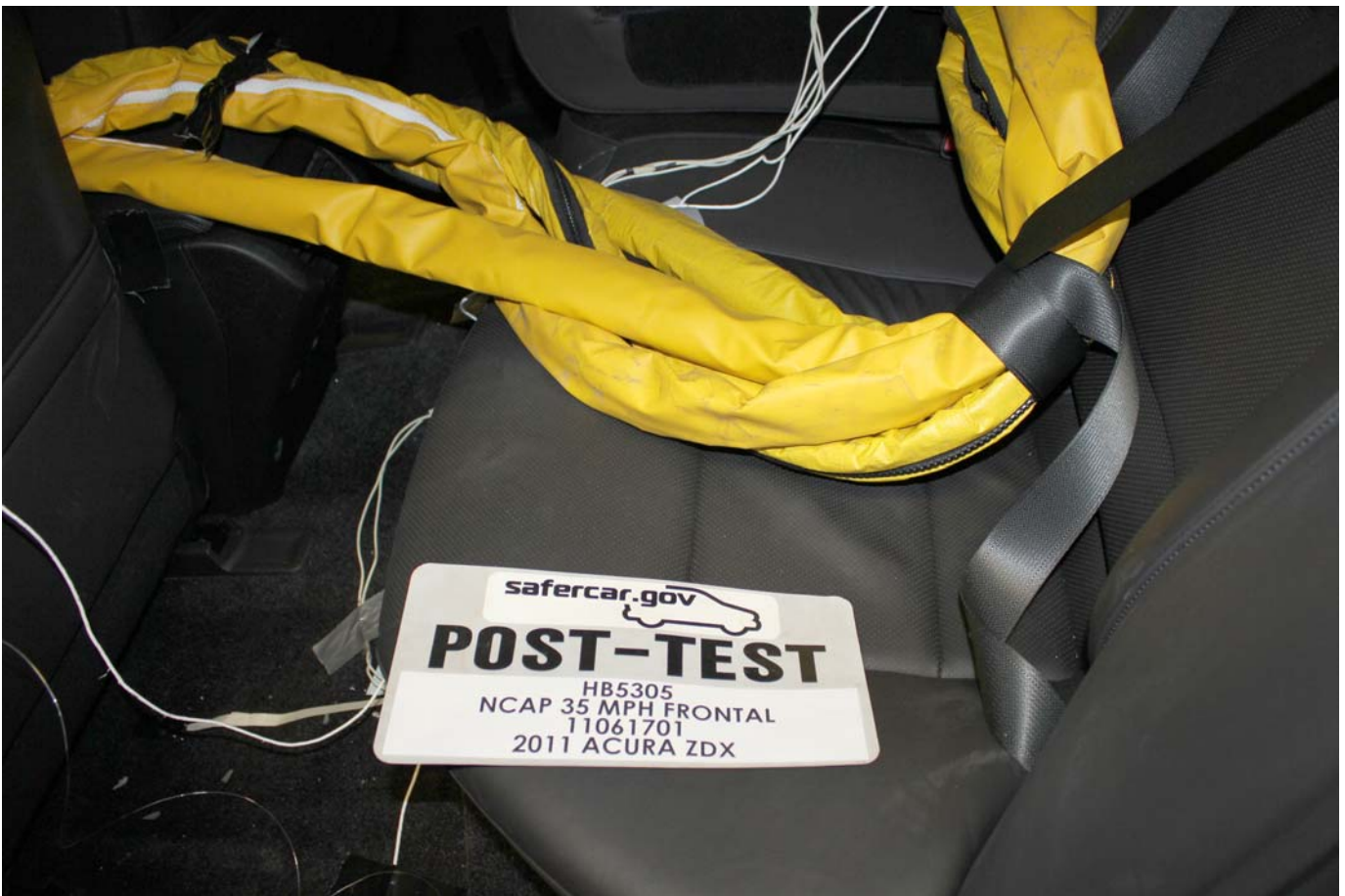
Post-Test Dummy Cable Routing
