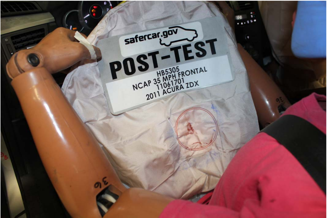
Post-Test Driver Dummy Contact with Airbag
