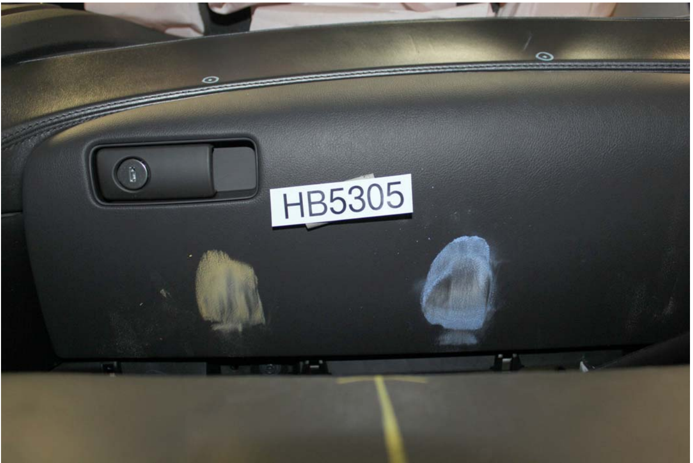
Post-Test Passenger Dummy Contact with Glovebox
