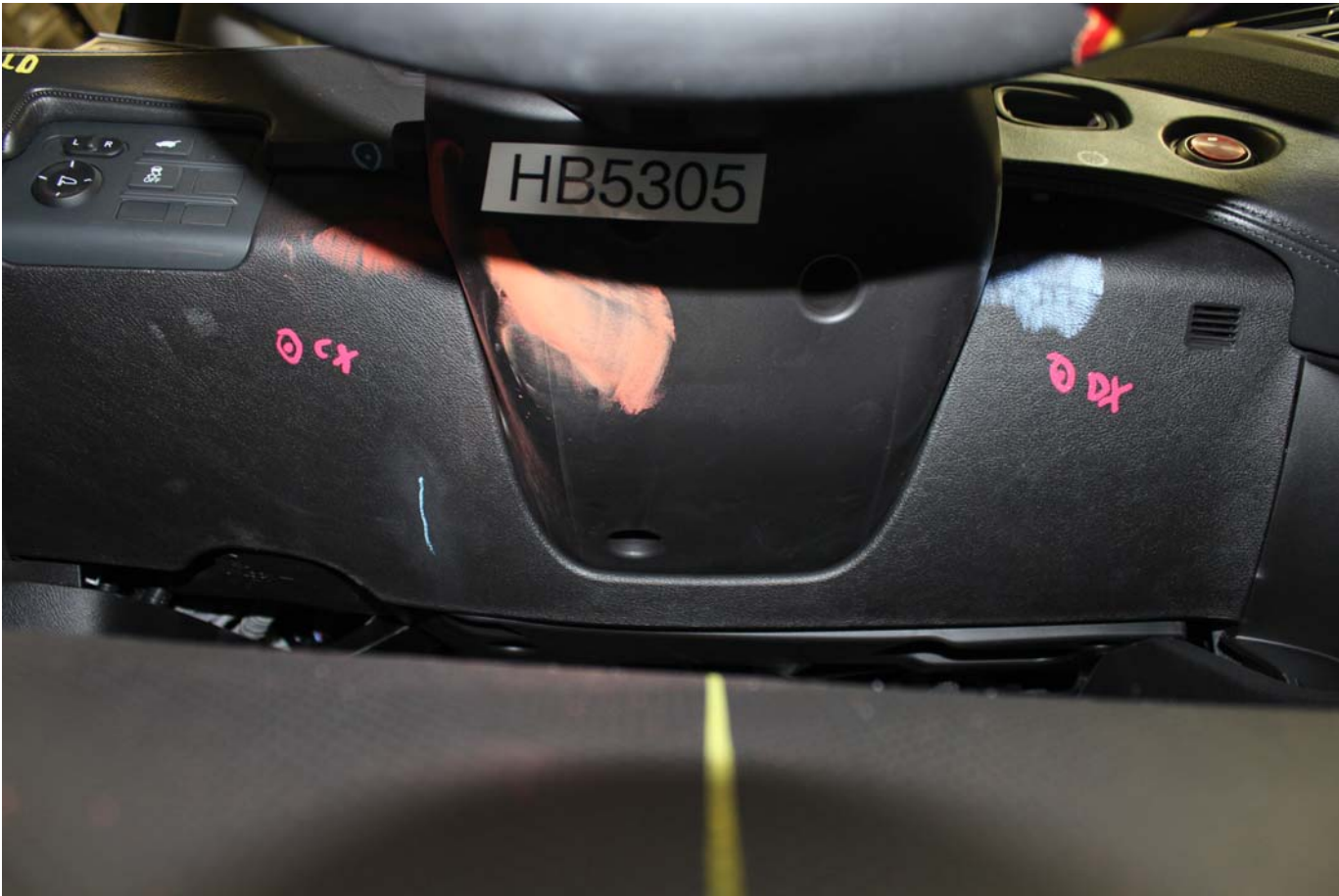
Post-Test Driver Dummy Contact with Knee Bolster
