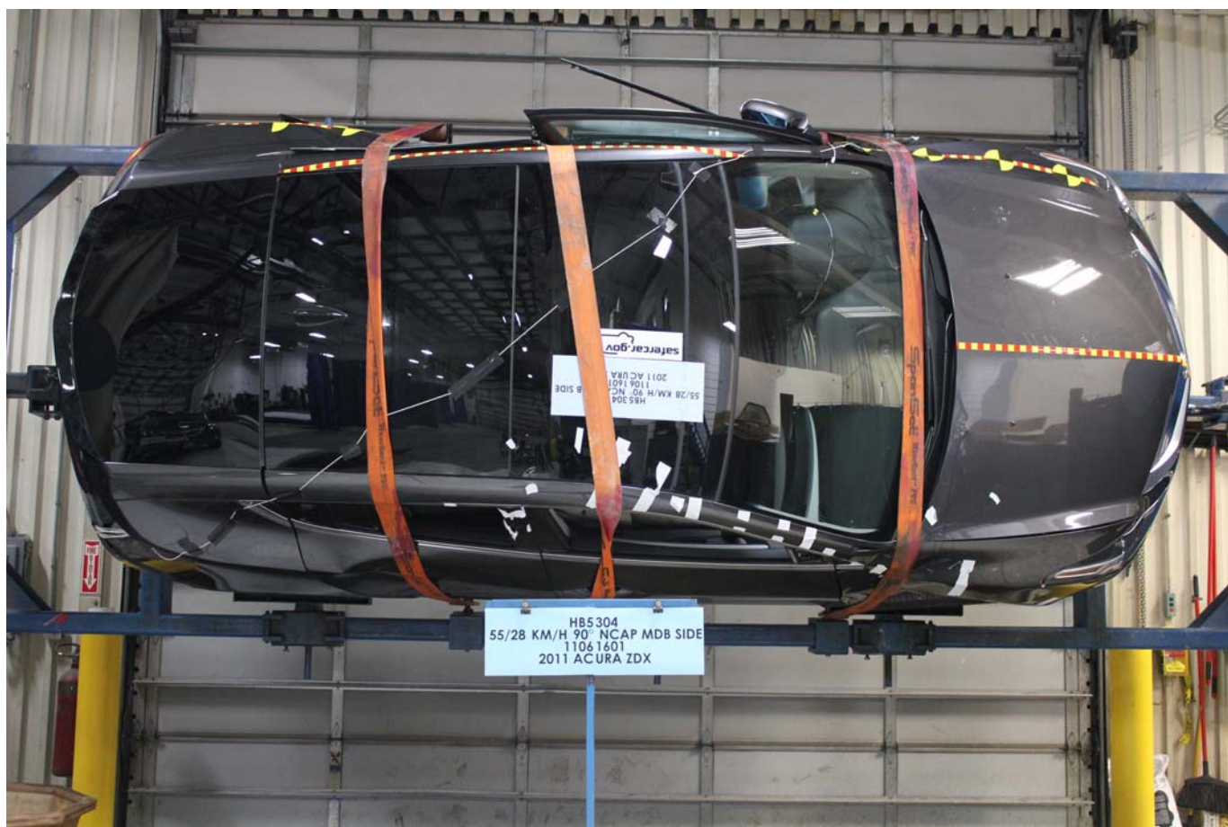
FMVSS No. 301/305 Rollover 270 Degrees
