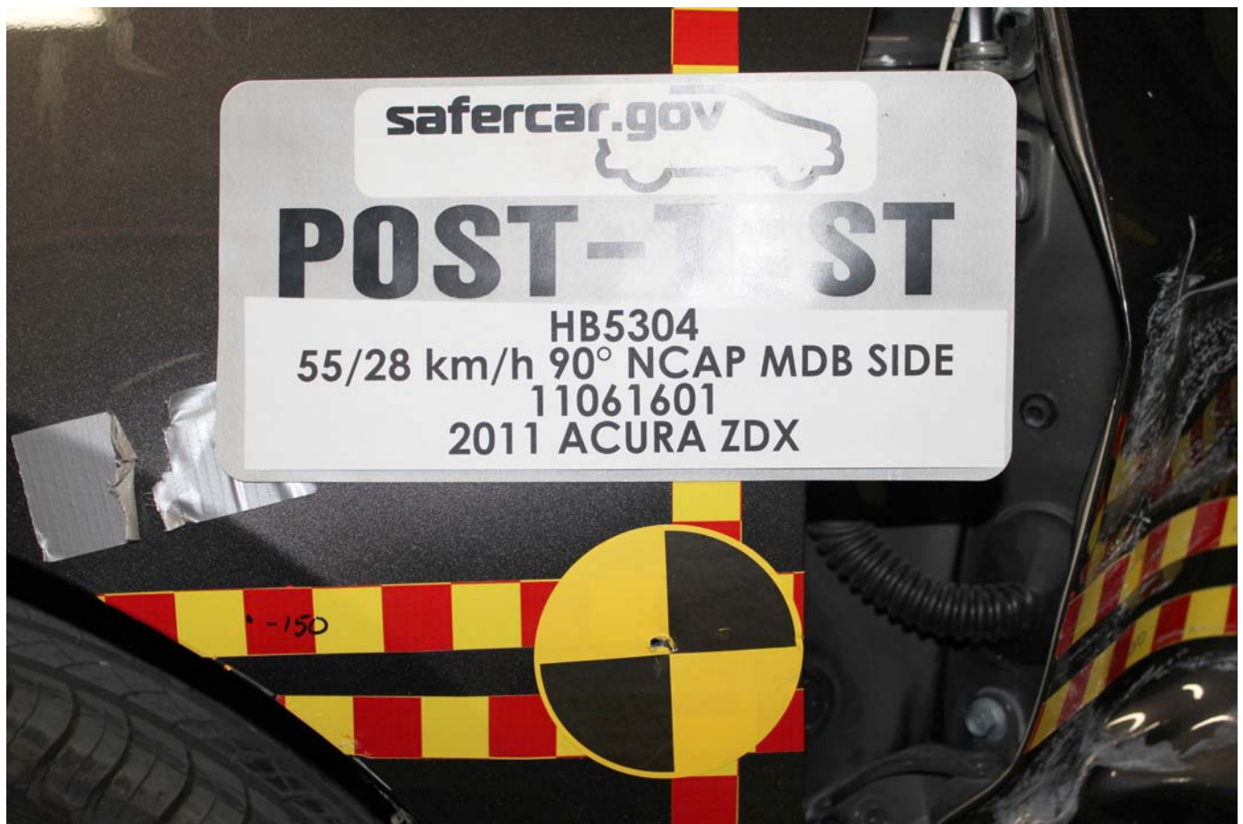
Post-Test Close-Up View of Impact Point Target
