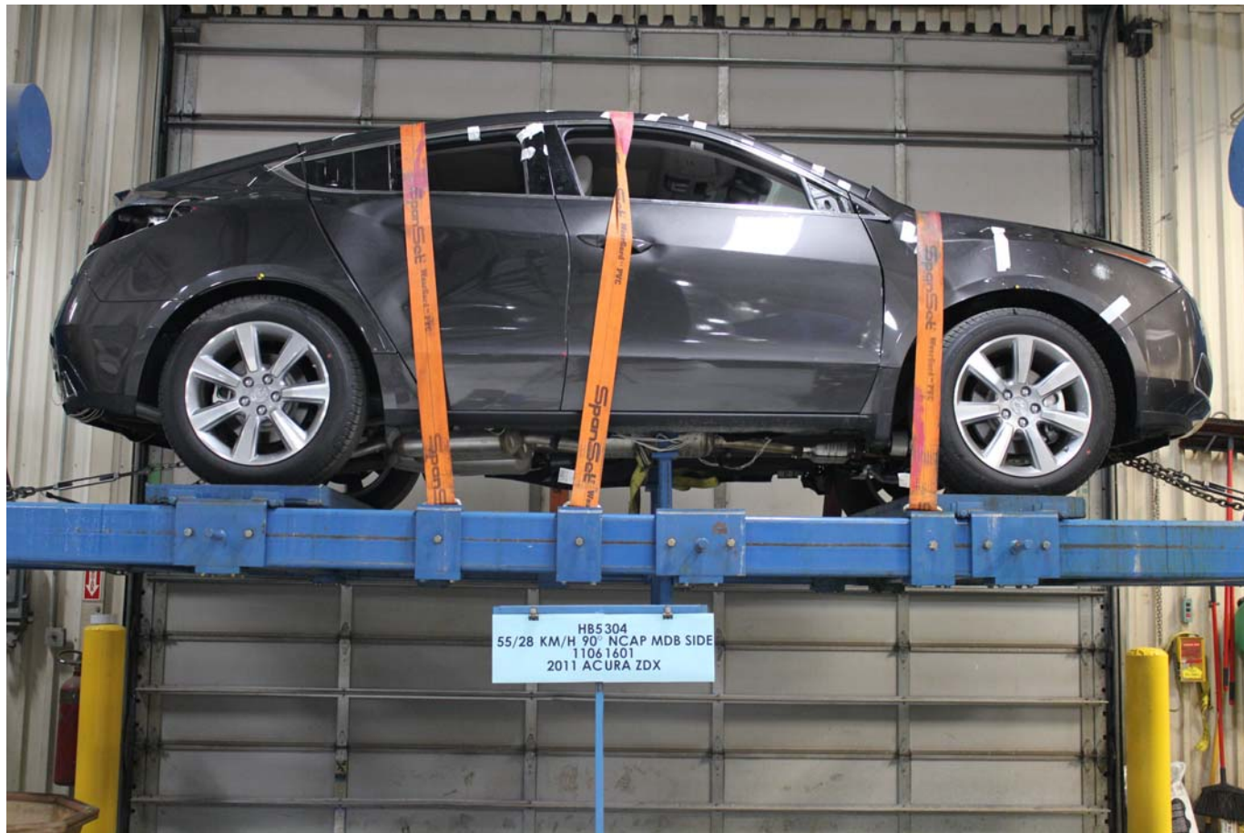
FMVSS No. 301/305 Rollover 360 Degrees
