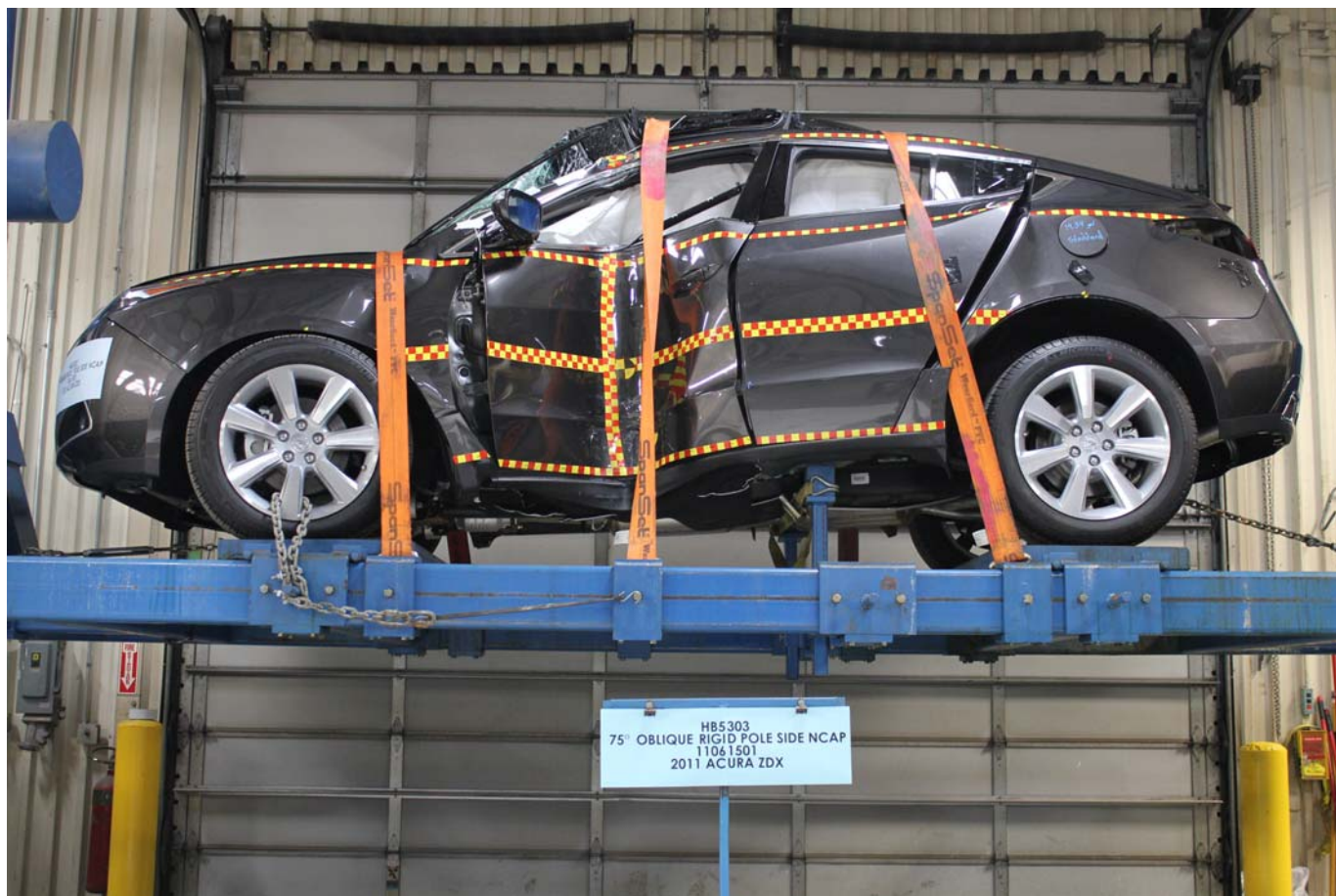
FMVSS No. 301/305 Rollover 360 Degrees
