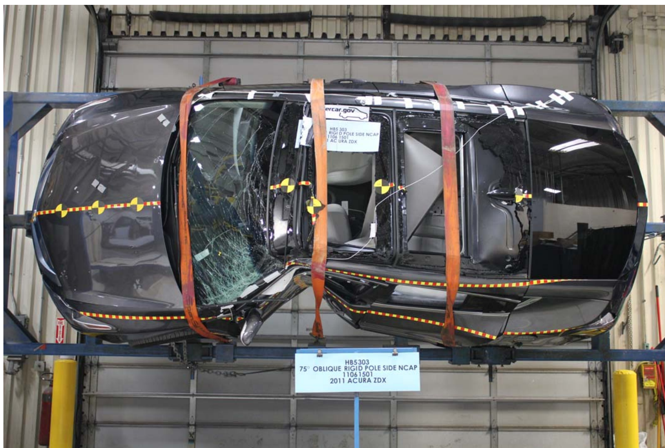
FMVSS No. 301/305 Rollover 90 Degrees
