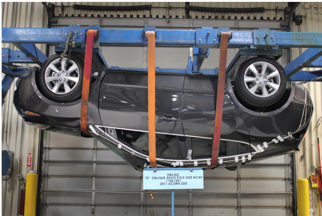
FMVSS No. 301/305 Rollover 180 Degrees
