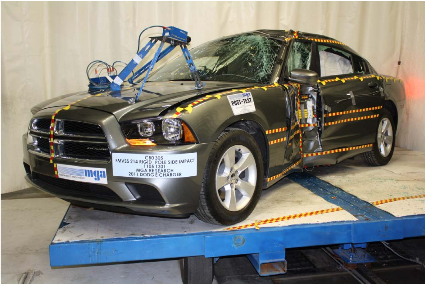
Post-Test \frac{3}{4} Front View of Impact Zone
