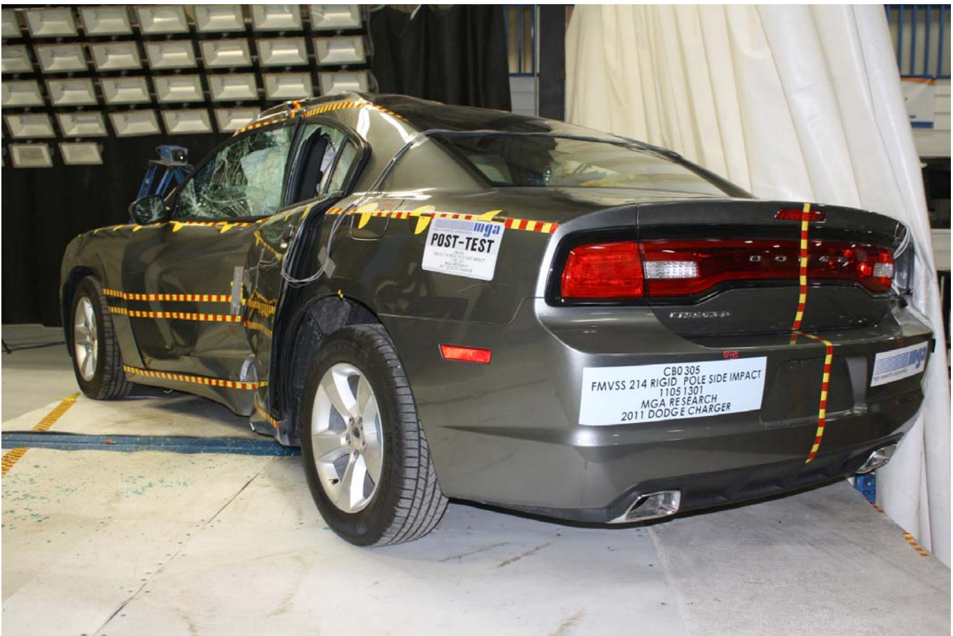
Post-Test \frac{3}{4} Rear View of Impact Zone
