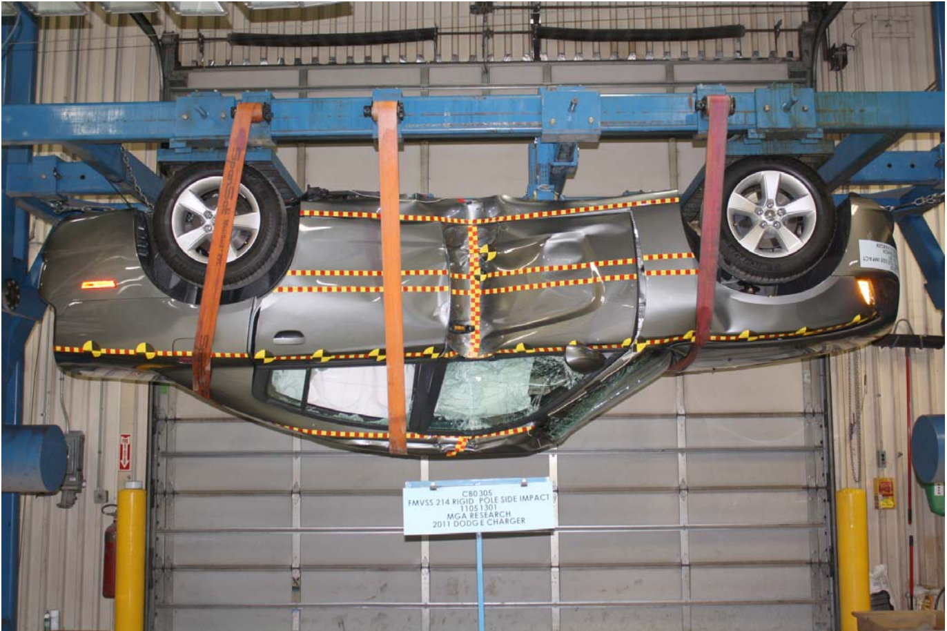
Post-Test Vehicle at 180 Degree Rollover
