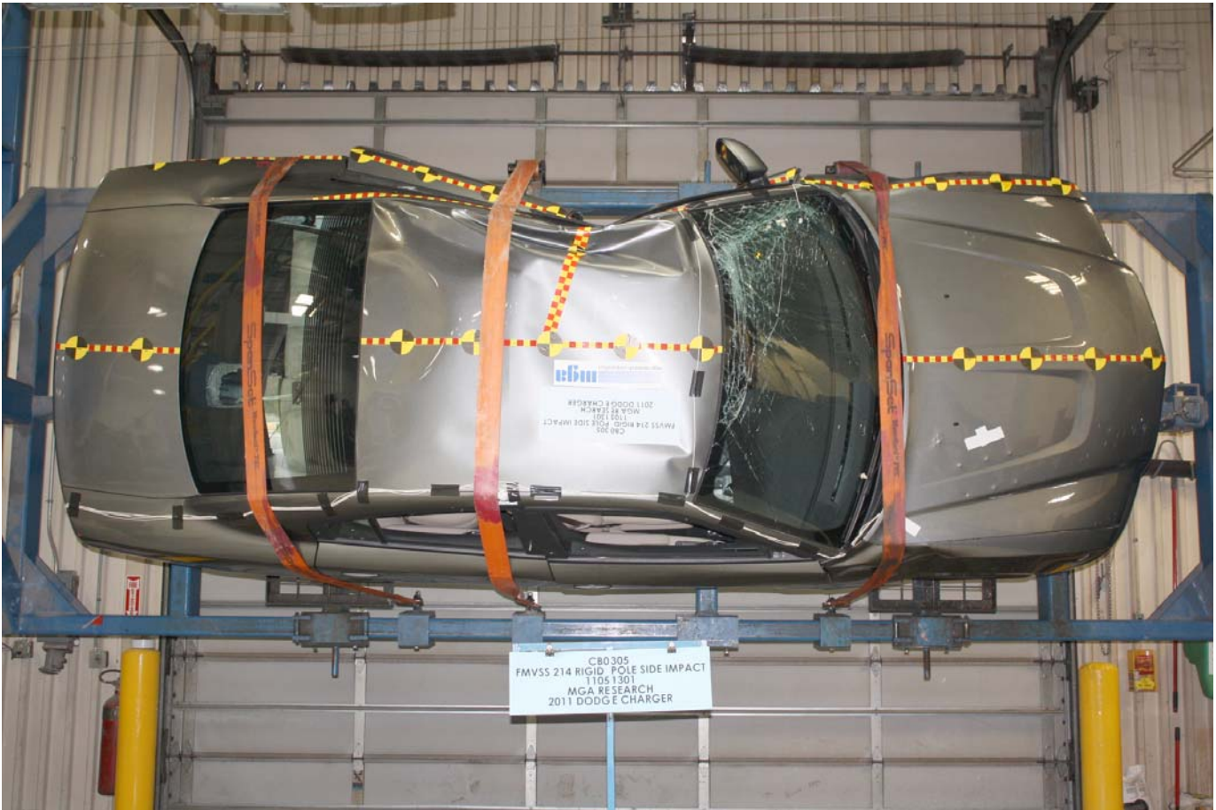
Post-Test Vehicle at 270 Degree Rollover
