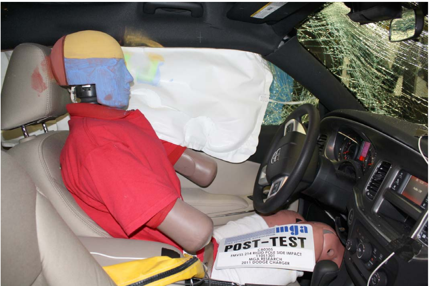
Post-Test Dummy Through Opposite Window
