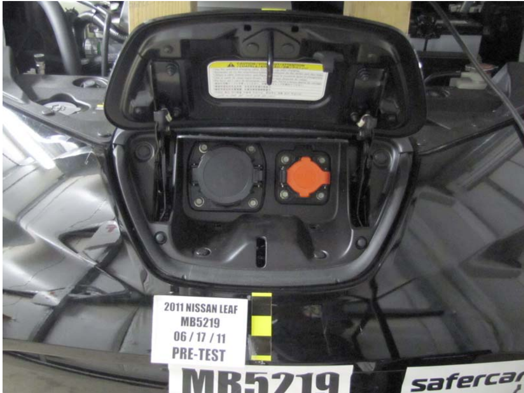
FIGURE 111. Pre-Test Battery Charging Port
