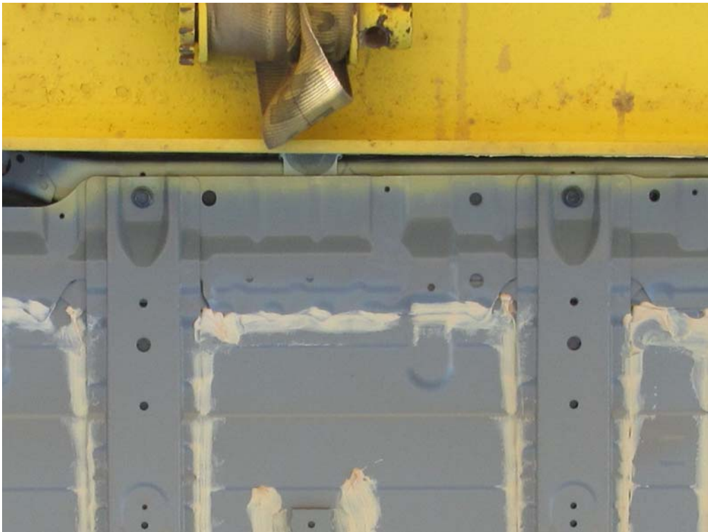
FIGURE 116. Post-Test Battery Mounting Hardware
