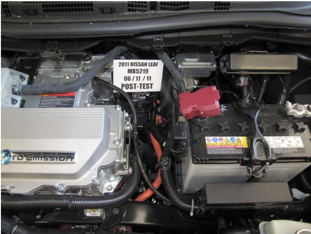
FIGURE 108. Post-Test Electric Drive Motor
