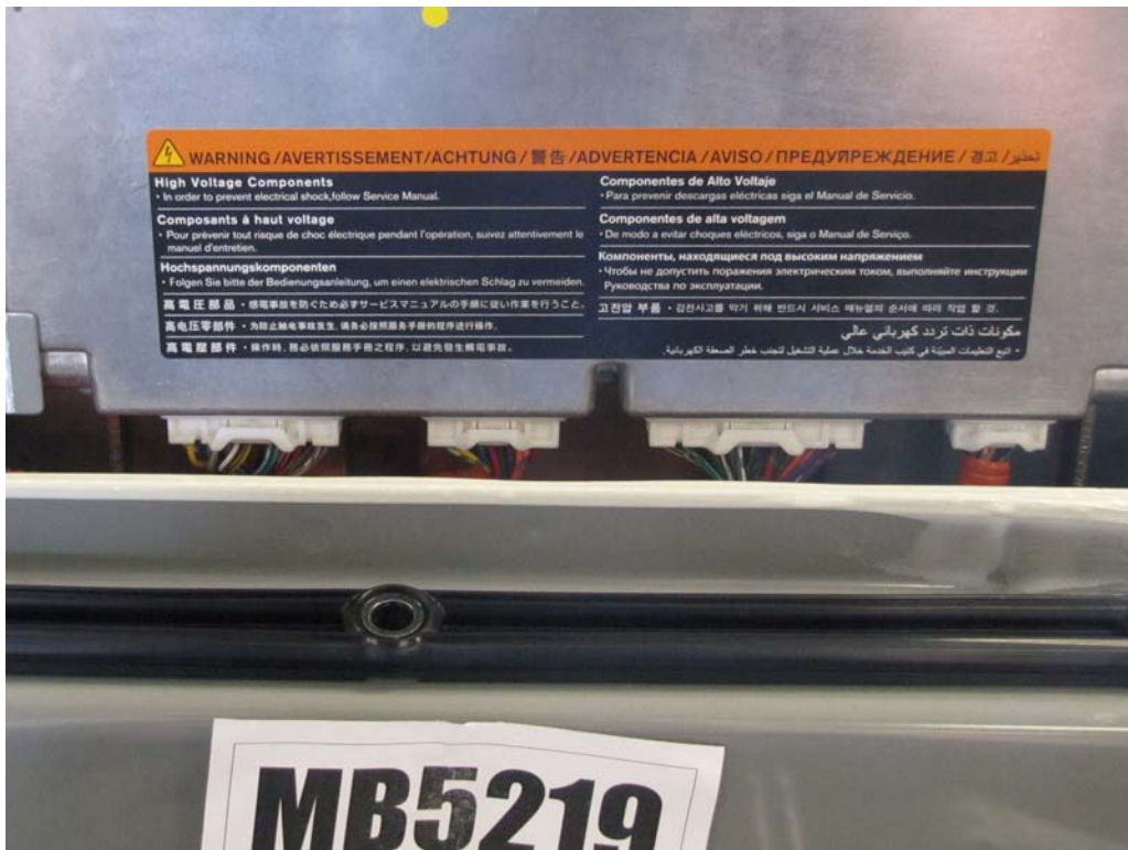
FIGURE 102. Electric System Label
