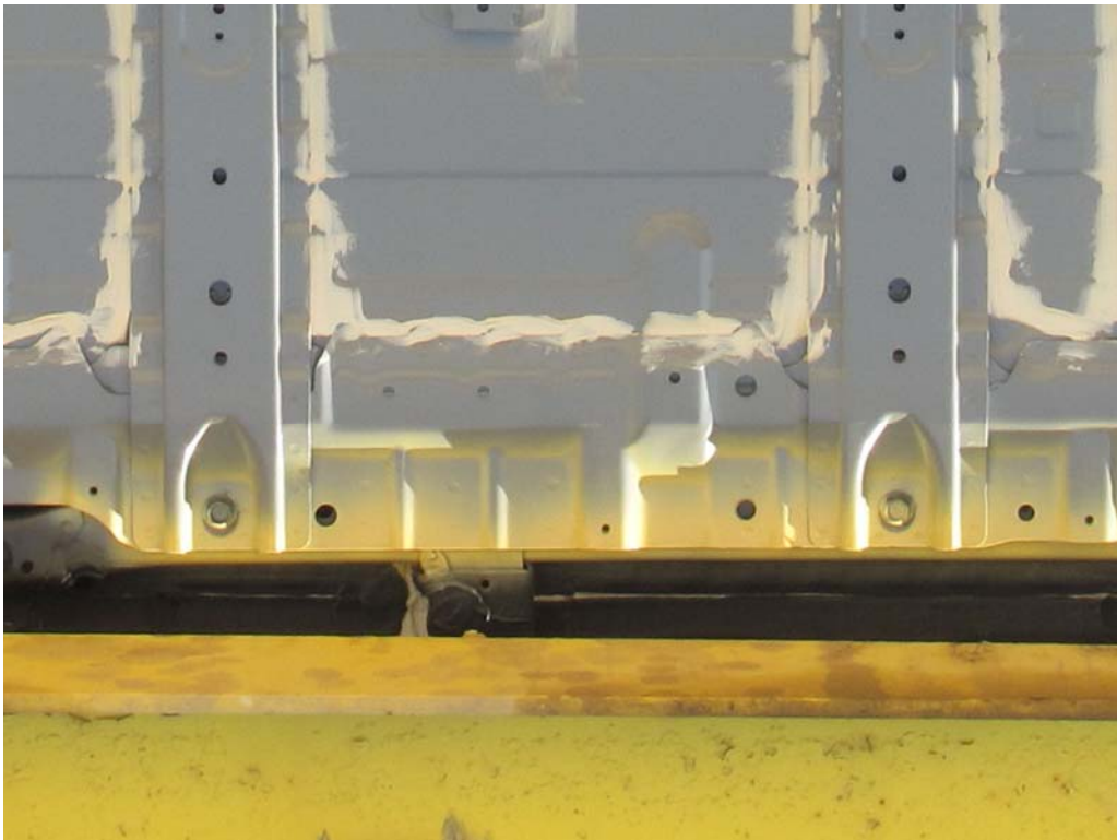
FIGURE 118. Post-Test Battery Mounting Hardware
