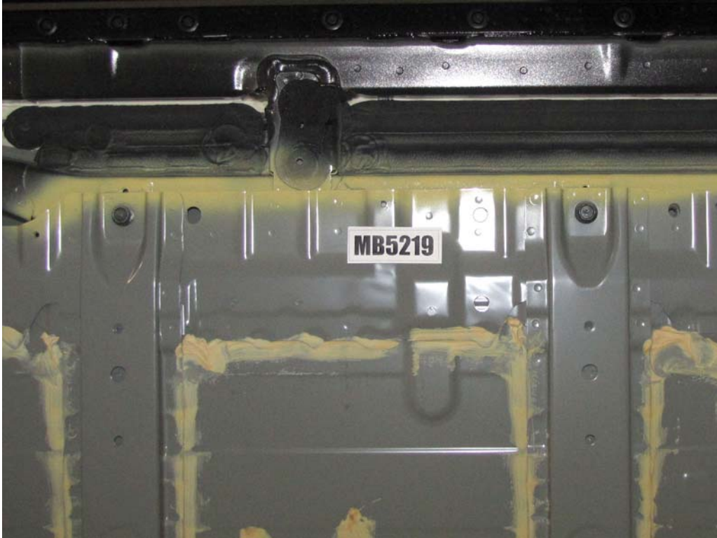
FIGURE 115. Pre-Test Battery Mounting Hardware
