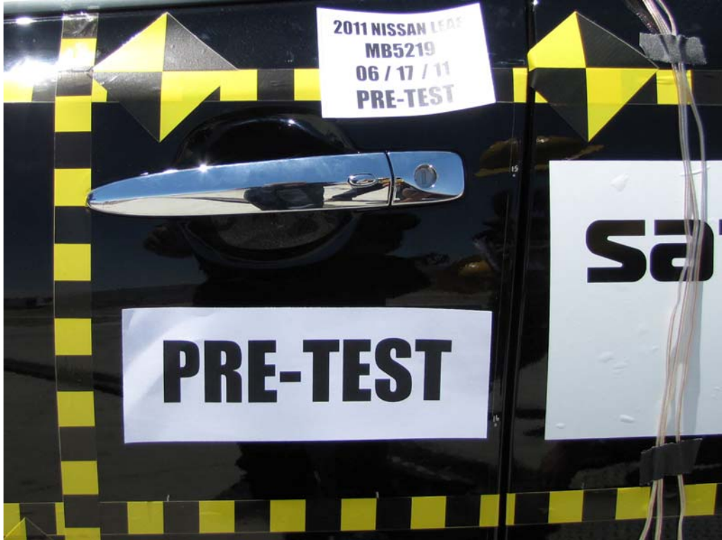
FIGURE 21. Pre-Test Left Front Door Latch Close-Up
