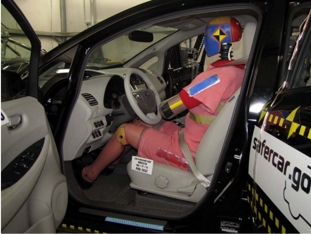
FIGURE 27. Pre-Test Left Side View of Driver Dummy Showing Belt, Chalking, and Contact Switches
