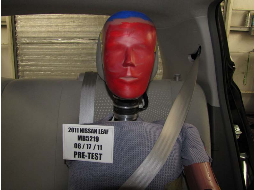
FIGURE 57. Pre-Test Frontal View of Rear Passenger Dummy Head and Shoulders in Relation to Head Restraint
