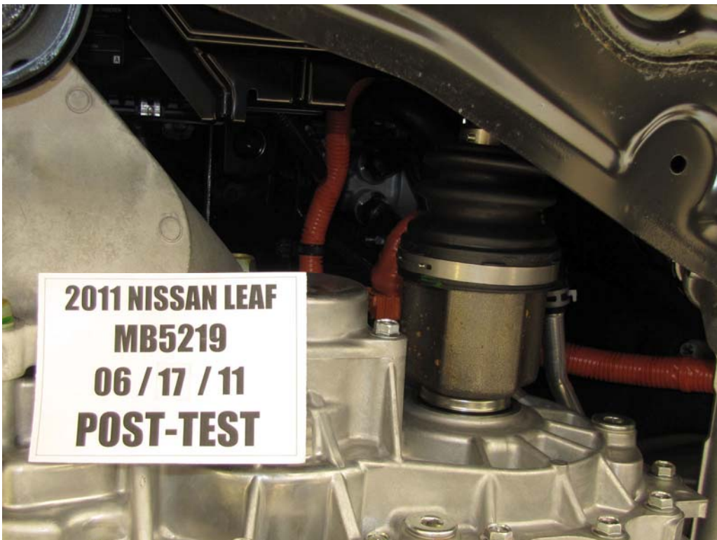
FIGURE 130. Post-Test High Voltage Connections
