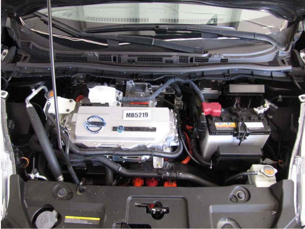
FIGURE 107. Pre-Test Electric Drive Motor
