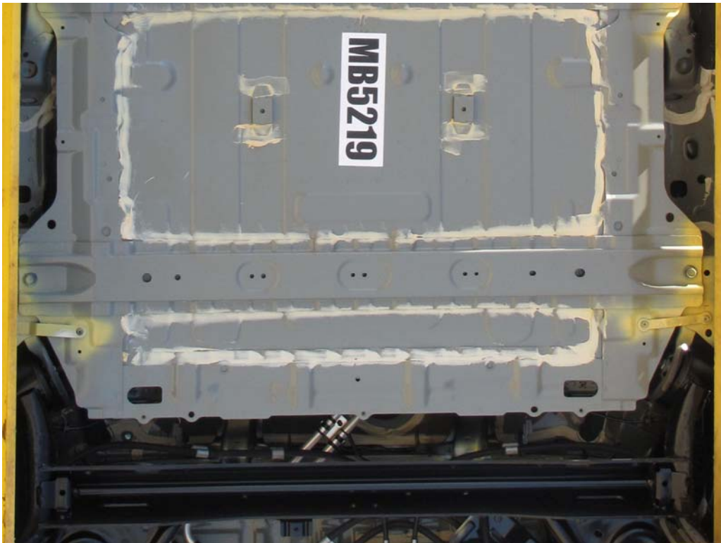
FIGURE 122. Post-Test Battery Mounting Hardware
