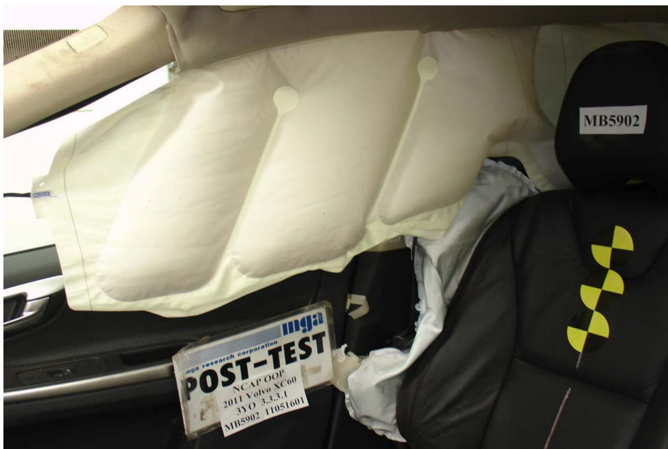
Post-Test Curtain Airbag Left ¾ Front View
