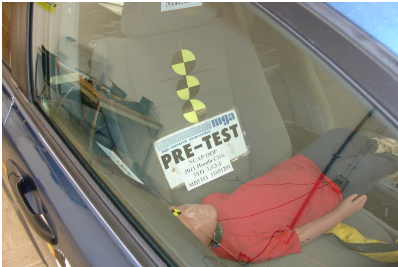
Pre-Test 3-Year-Old Child Dummy Right ¾ Front View
