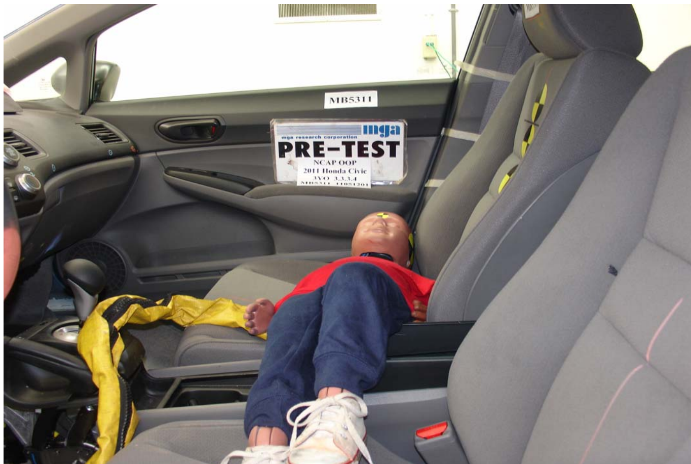
Pre-Test 3-Year-Old Child Dummy Left Side View
