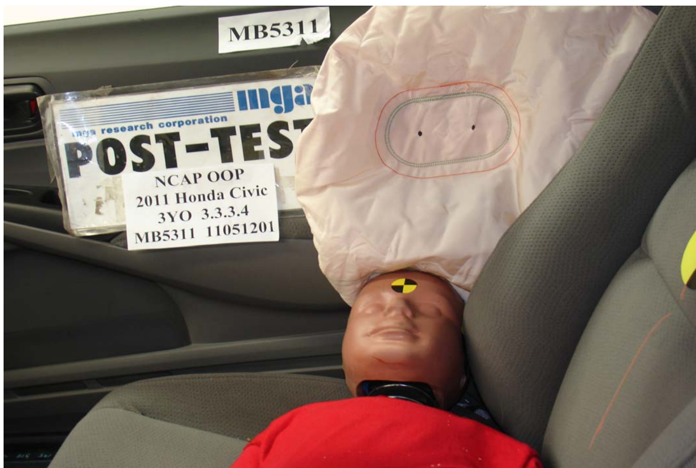
Post-Test 3-Year-Old Child Dummy Left Side Closeup View
