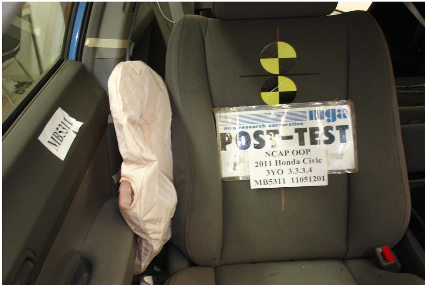
Post-Test Curtain and Torso Airbag Front View
