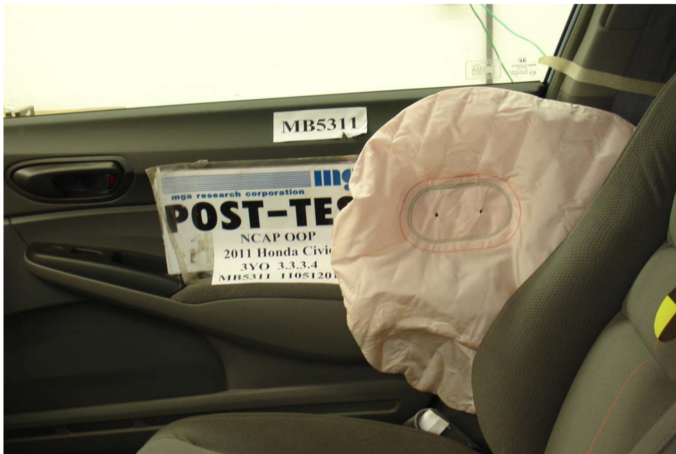
Post-Test Curtain and Torso Airbag Left Side View
