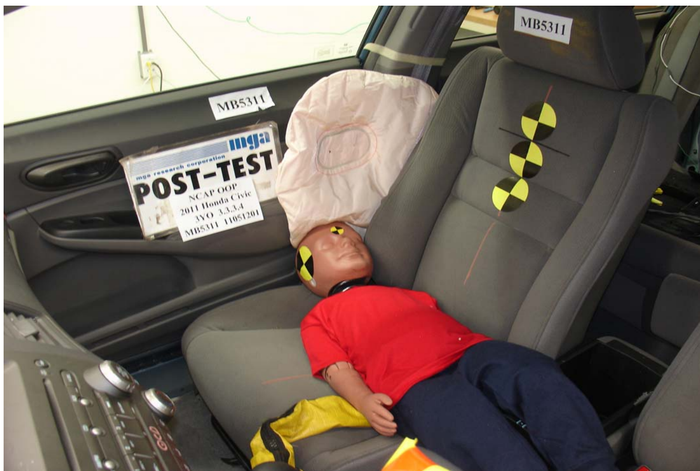
Post-Test 3-Year-Old Child Dummy Left 3/4 Front View
