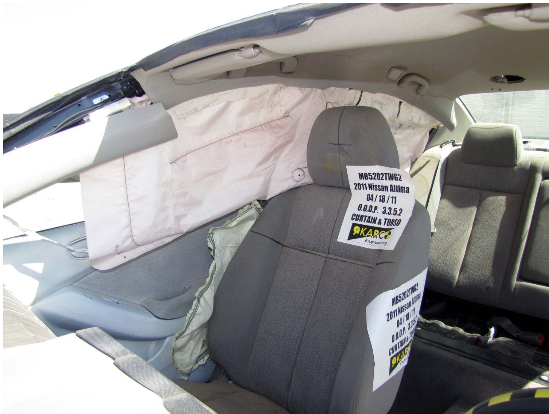
Figure A-10: Post-Test Airbags, Left Front \frac{3}{4} View
