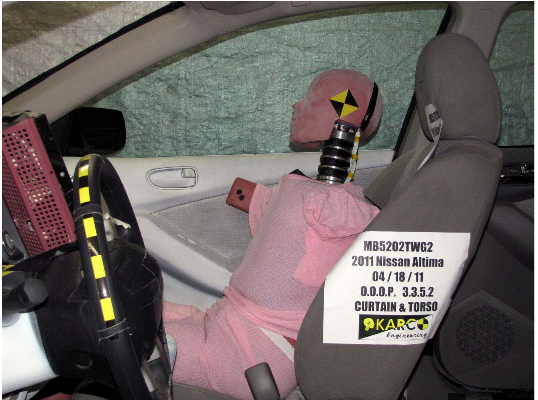
Figure A-5: Pre-Test Dummy Position, Left Side View
