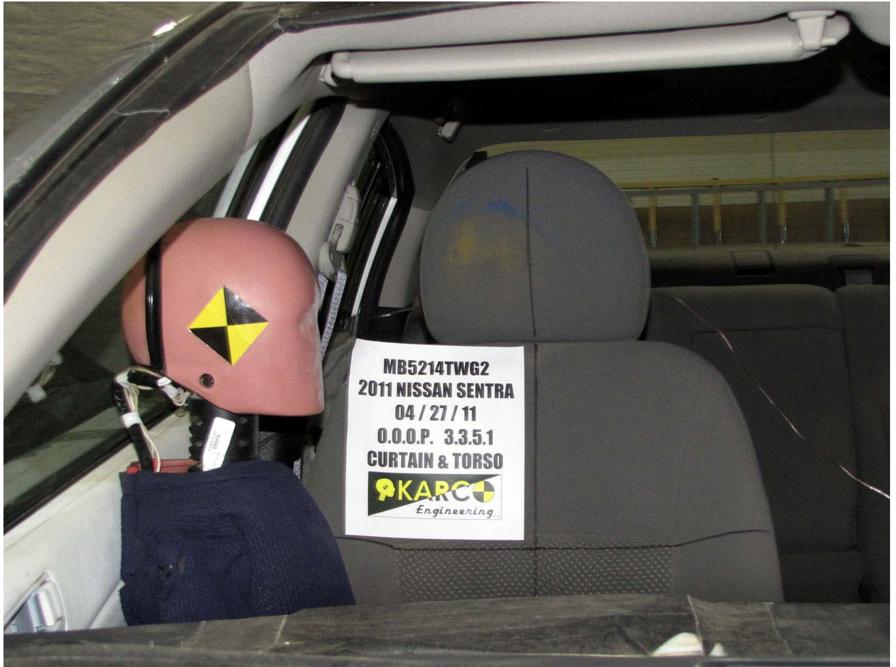
Figure A-7: Pre-Test Dummy Position, Front View
