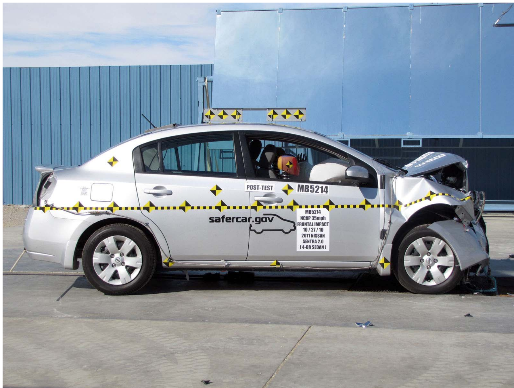
Figure A-4: Post-Test Right Side View of Frontal NCAP Test
