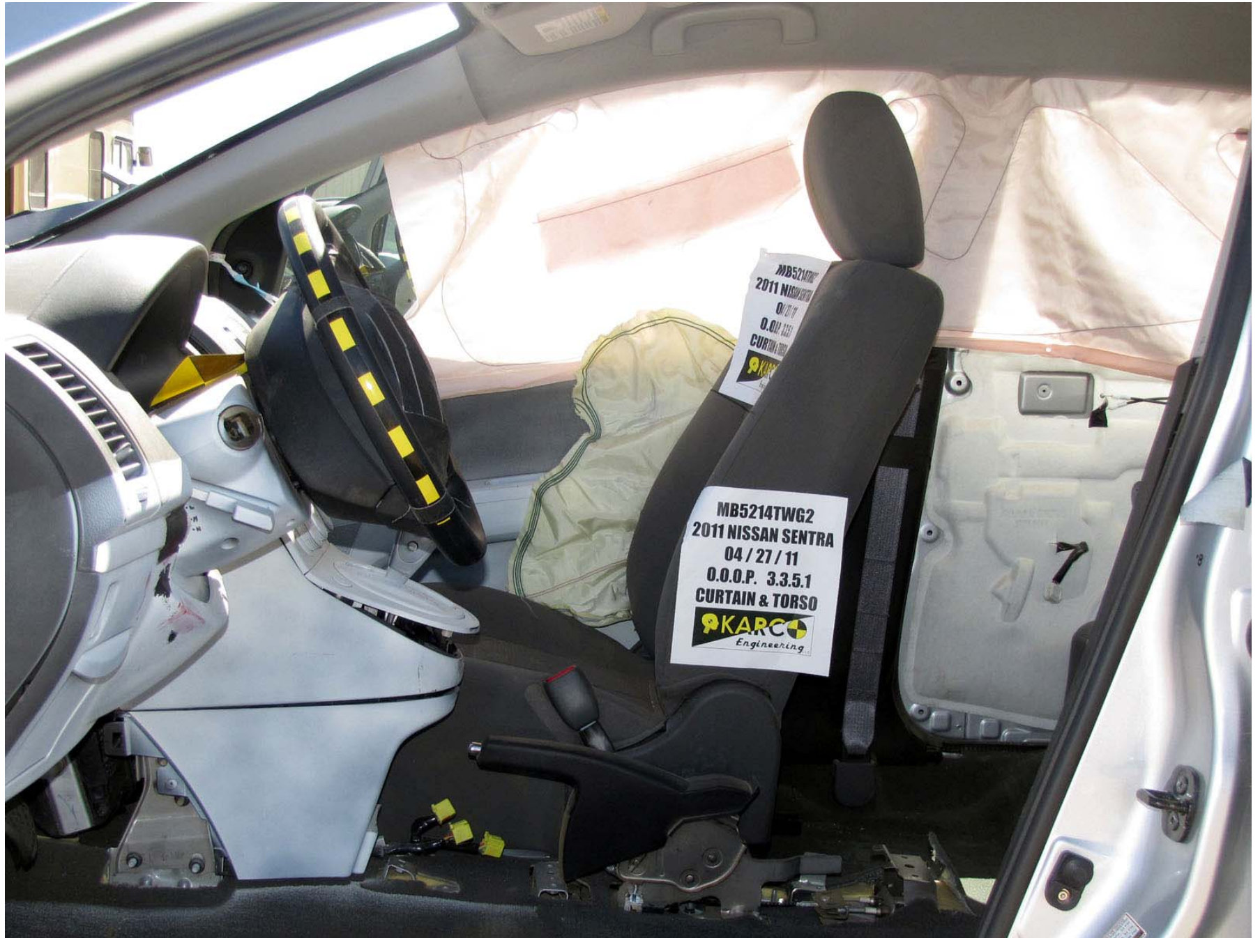
Figure A-9: Post-Test Airbags, Left Side View
