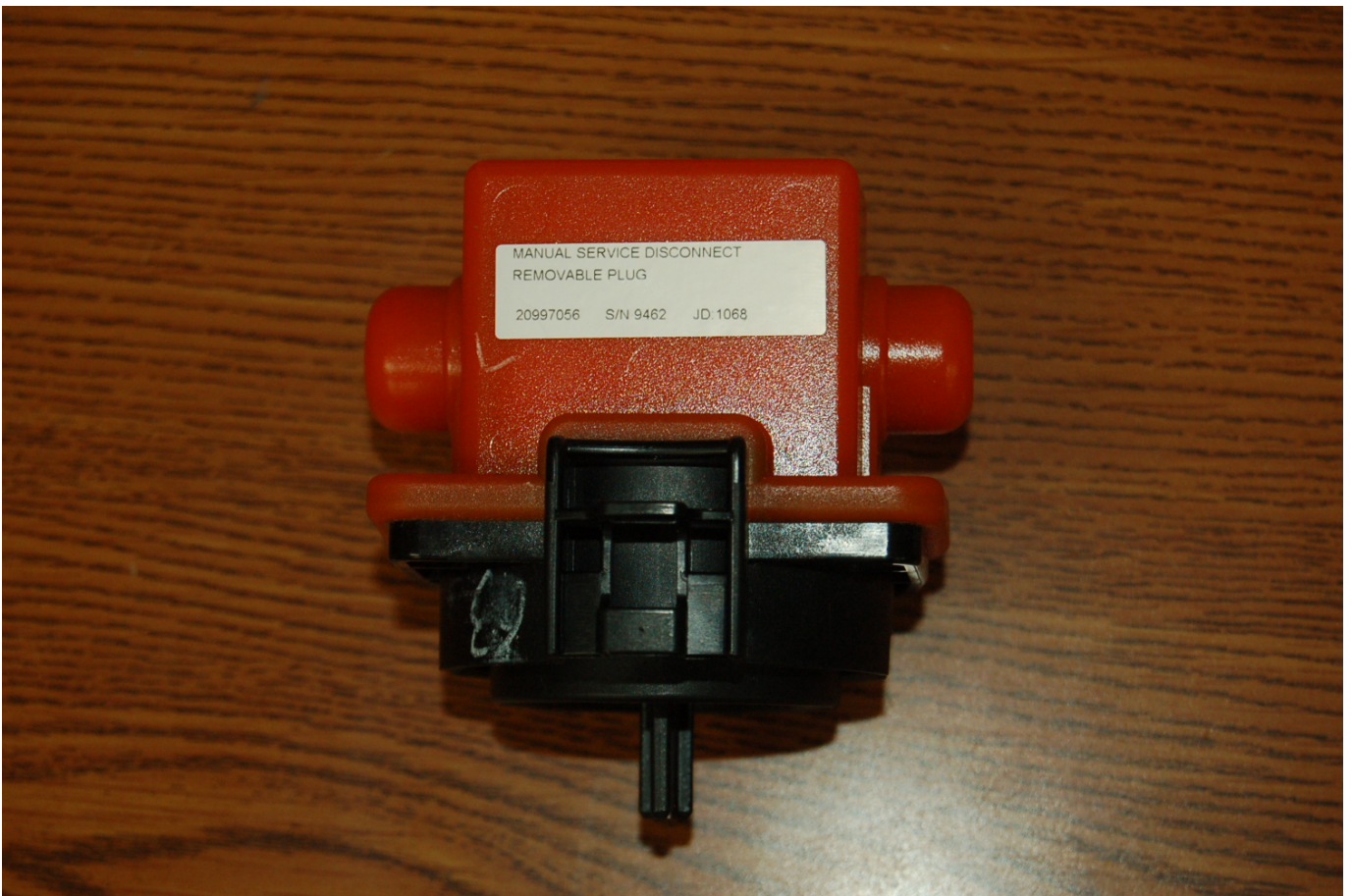
Manual High Voltage Service Disconnect
