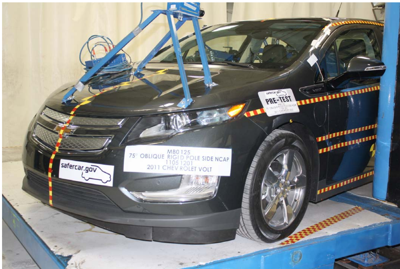
Pre-Test Left Side View of Pole Positioned Against Side of Vehicle at Ideal Impact Point
