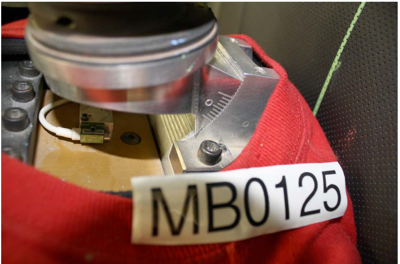
Pre-Test View of Dummy's Neck Showing Position of Adjustable Neck Bracket
