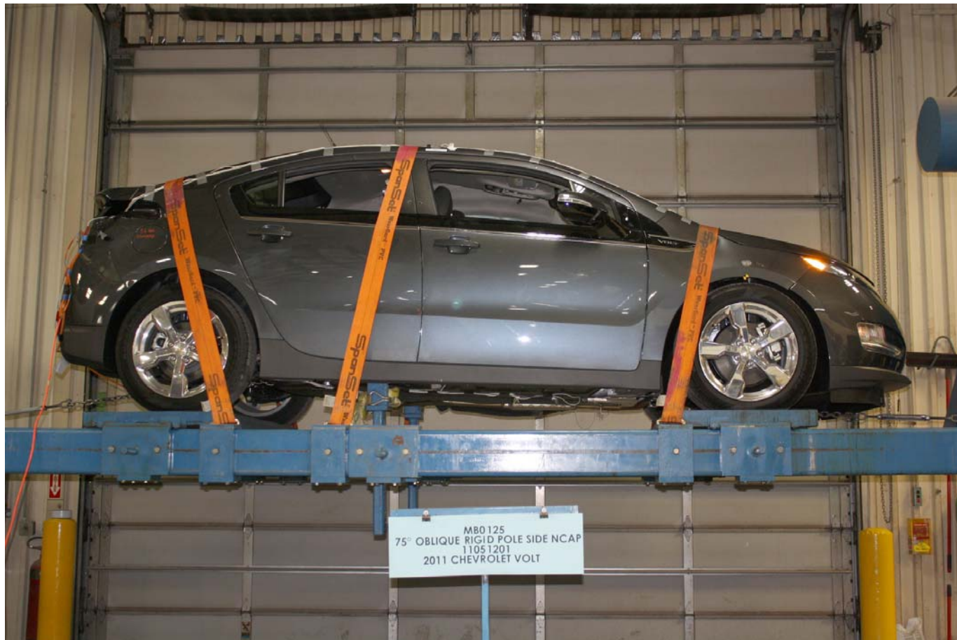
FMVSS No. 301/305 Rollover 0 Degrees
