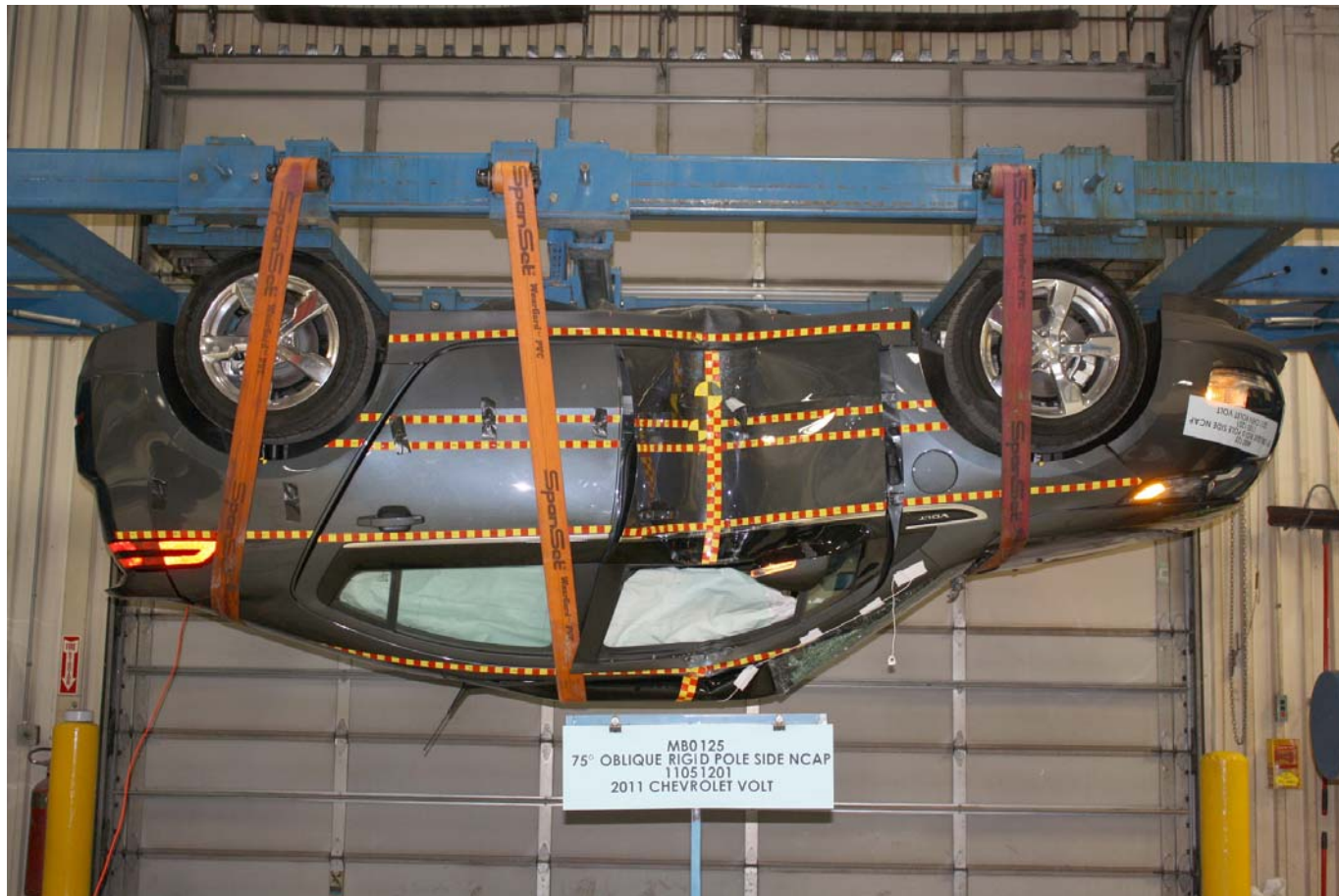
FMVSS No. 301/305 Rollover 180 Degrees
