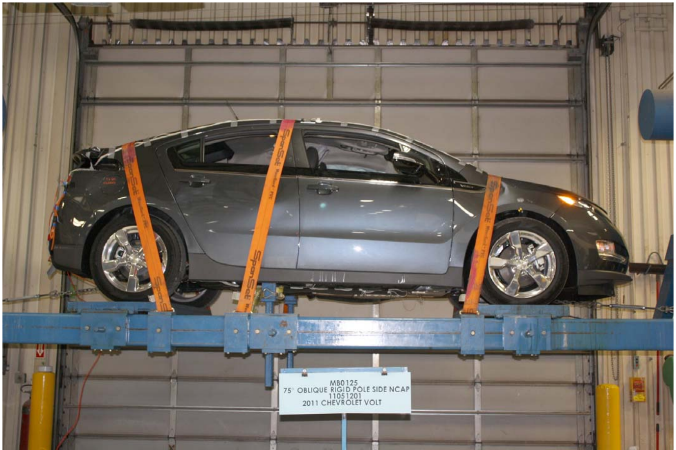
FMVSS No. 301/305 Rollover 360 Degrees
