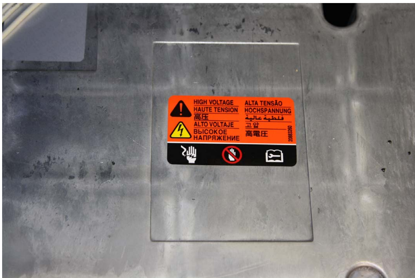
Power Inverter Warning Label
