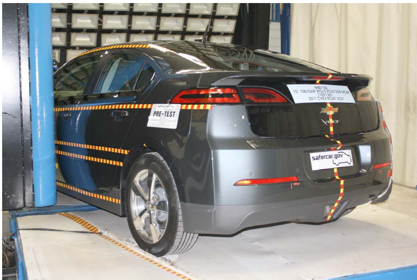
Pre-Test Right Side View of Pole Positioned Against Side of Vehicle at Ideal Impact Point
