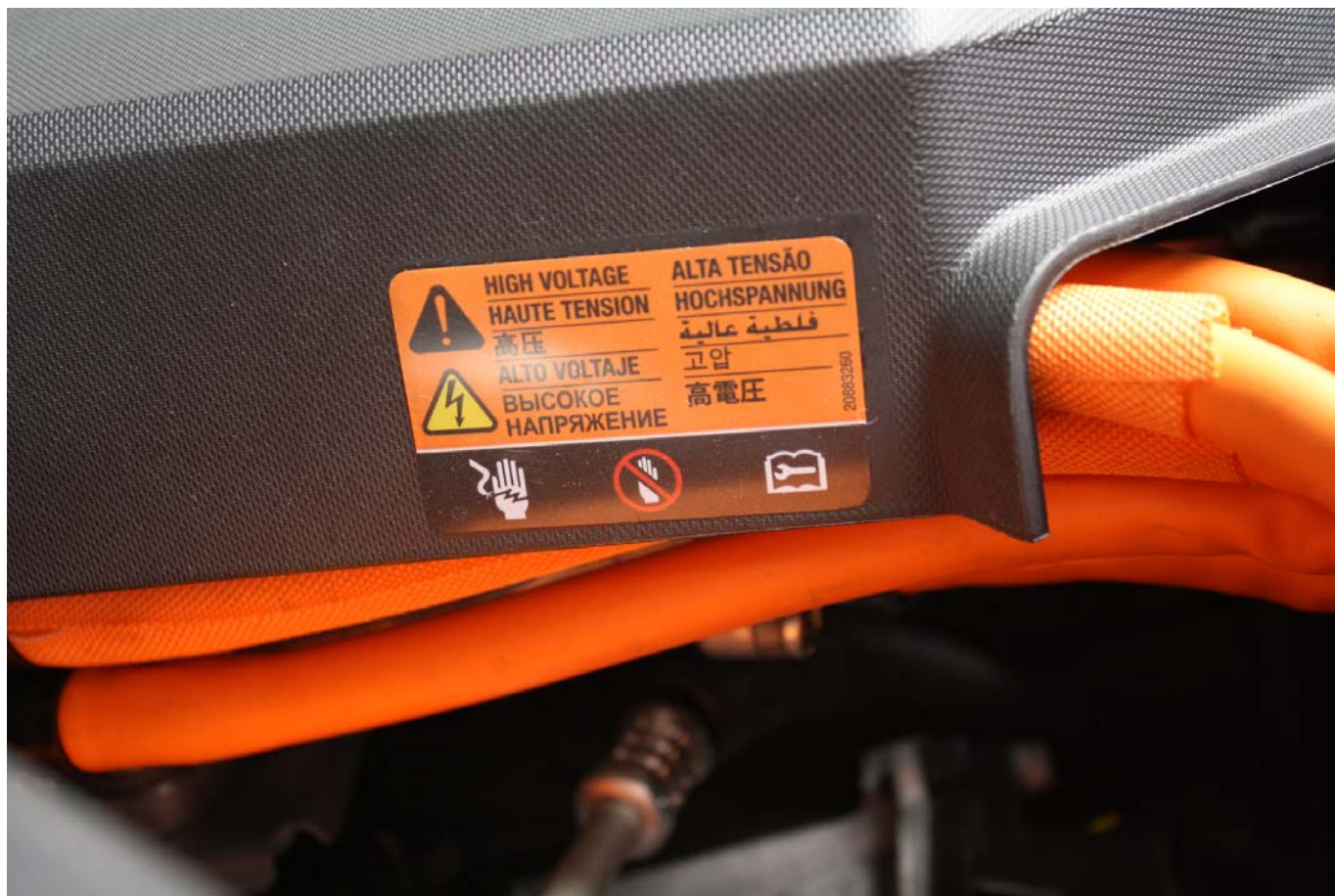
Auxiliary Power Module Warning Label
