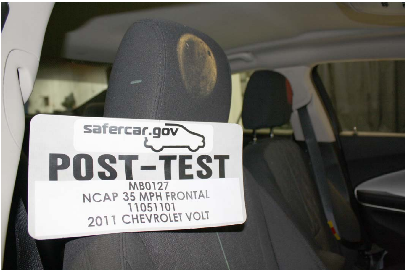
Post-Test Passenger Dummy Contact with Headrest
