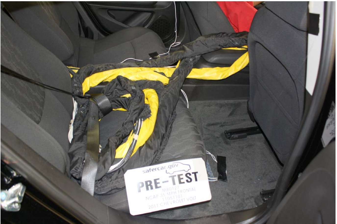
Pre-Test Dummy Cable Routing
