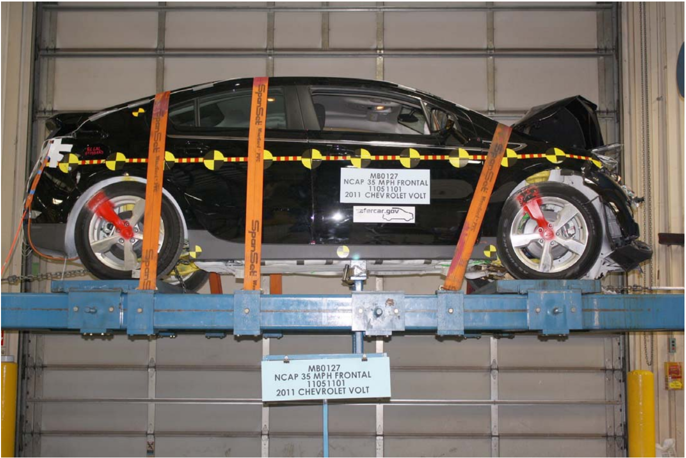
Vehicle at 0 Degrees on Static Rollover Device
