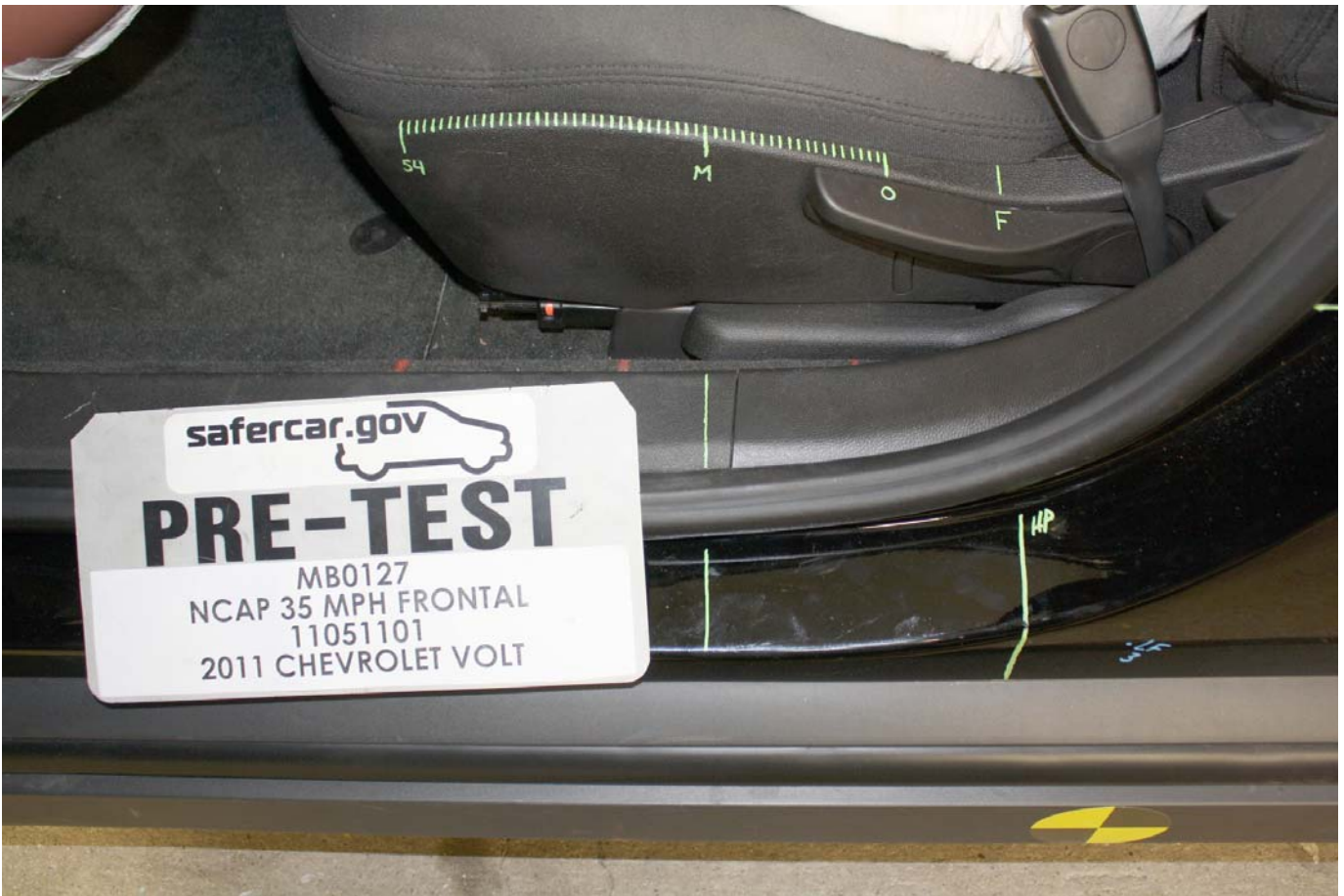
Pre-Test Driver's Seat Fore-Aft Markings
