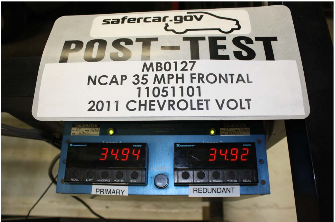
Post-Test Speed Trap Read-Out
