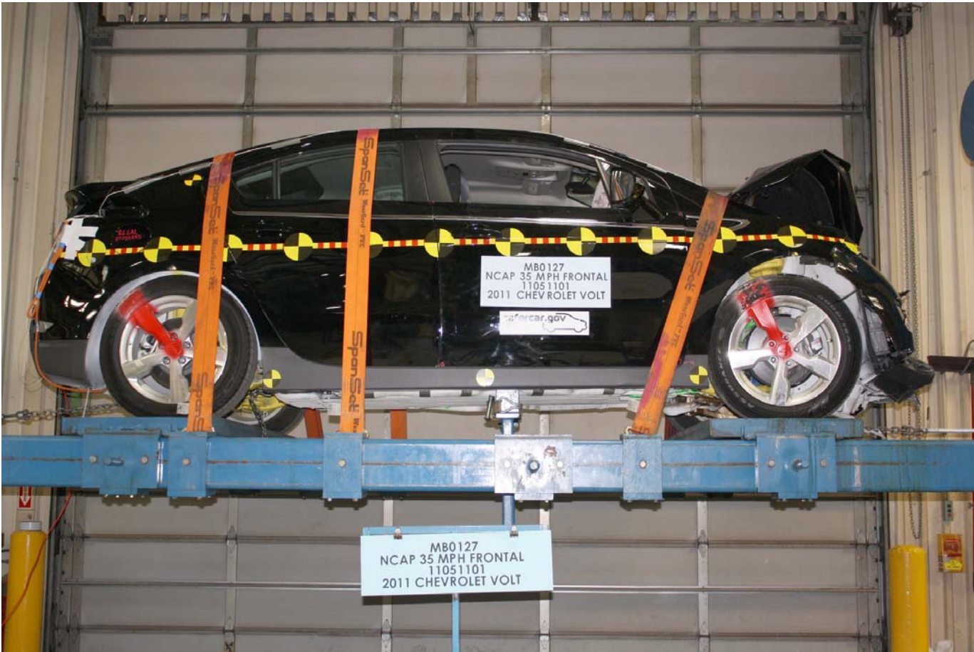
Vehicle at 360 Degrees on Static Rollover Device
