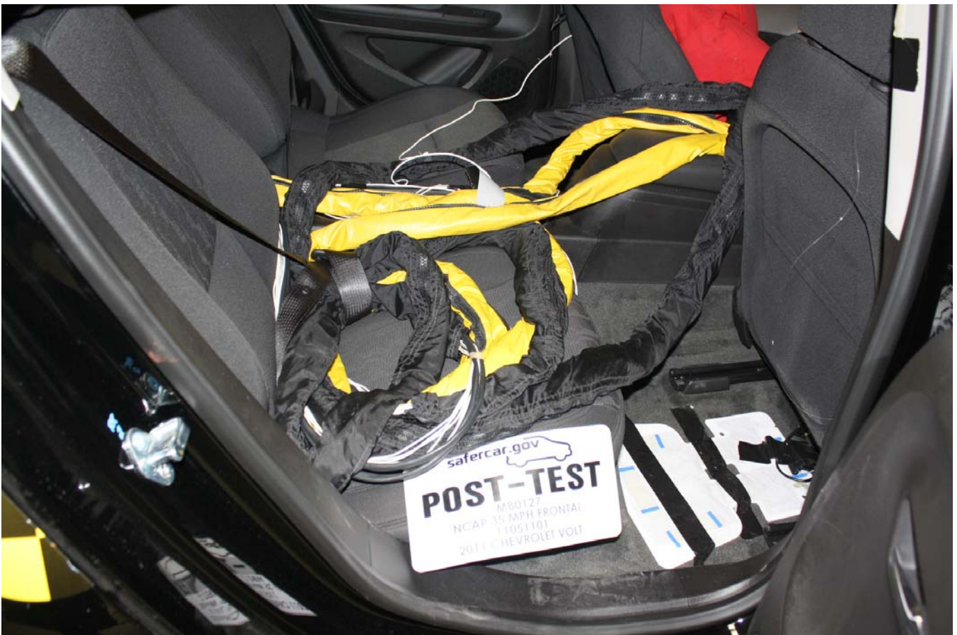
Post-Test Dummy Cable Routing
