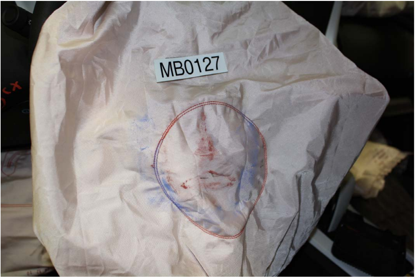
Post-Test Driver Dummy Contact with Airbag
