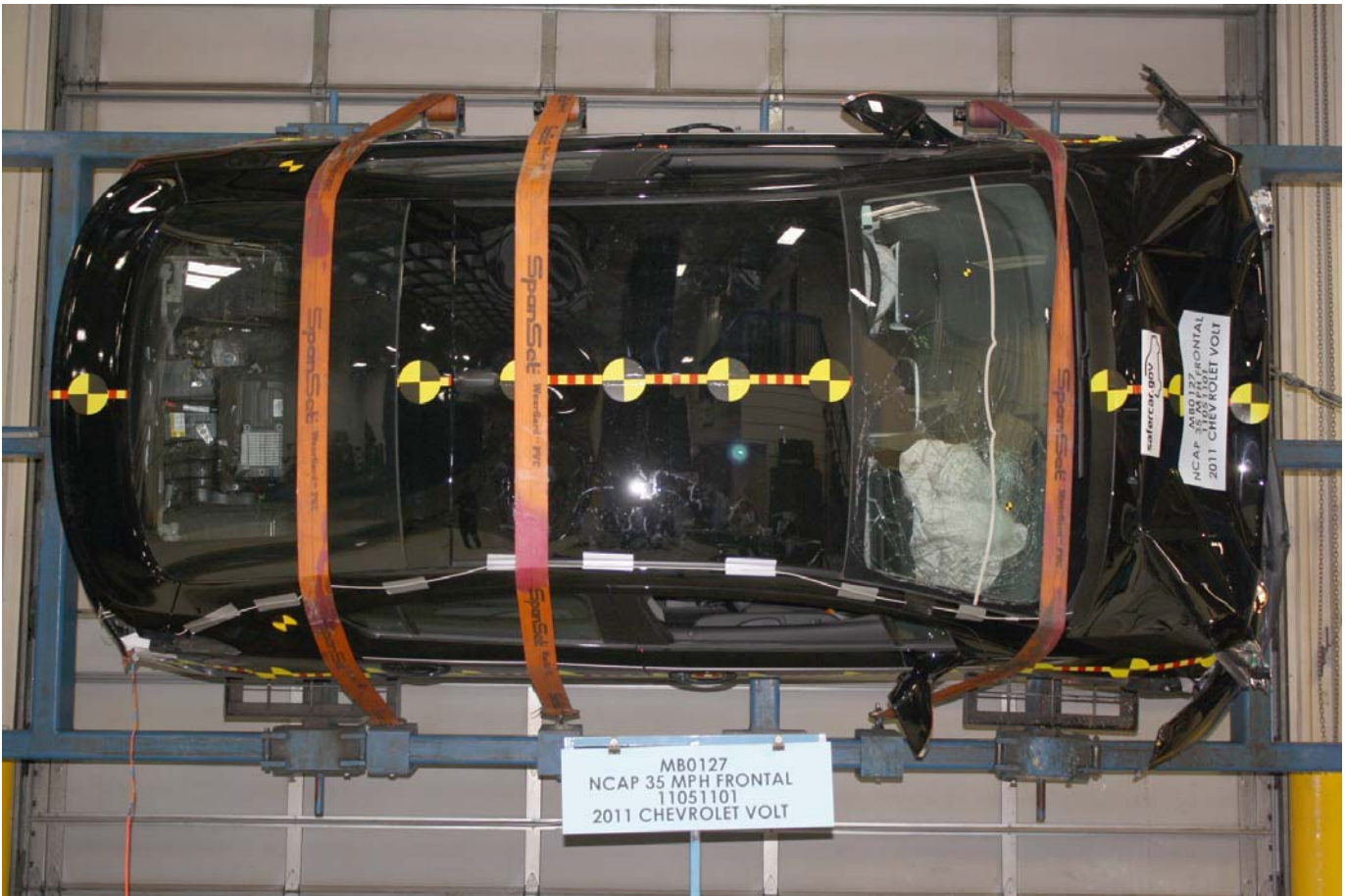
Vehicle at 90 Degrees on Static Rollover Device
