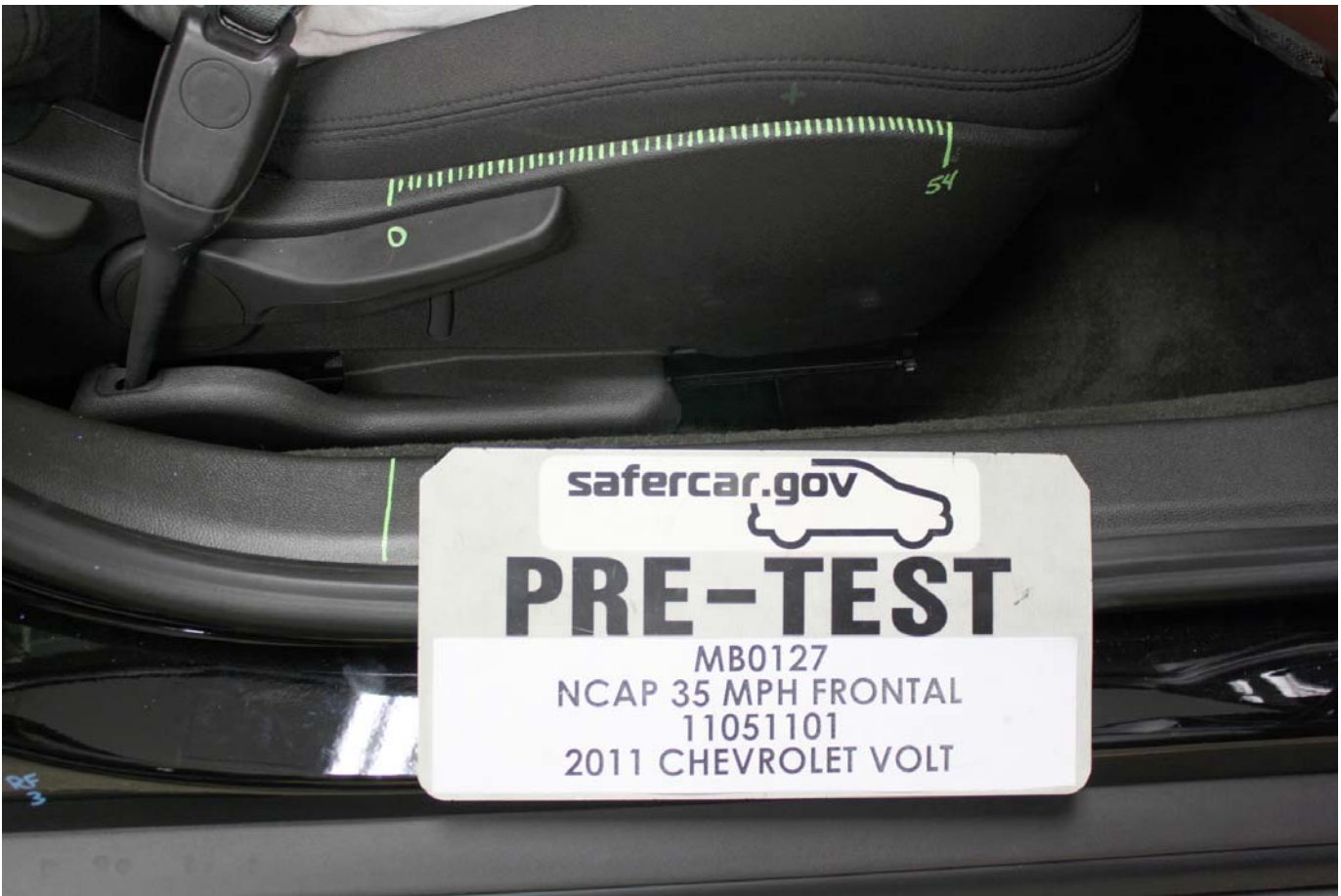
Pre-Test Passenger's Seat Fore-Aft Markings
