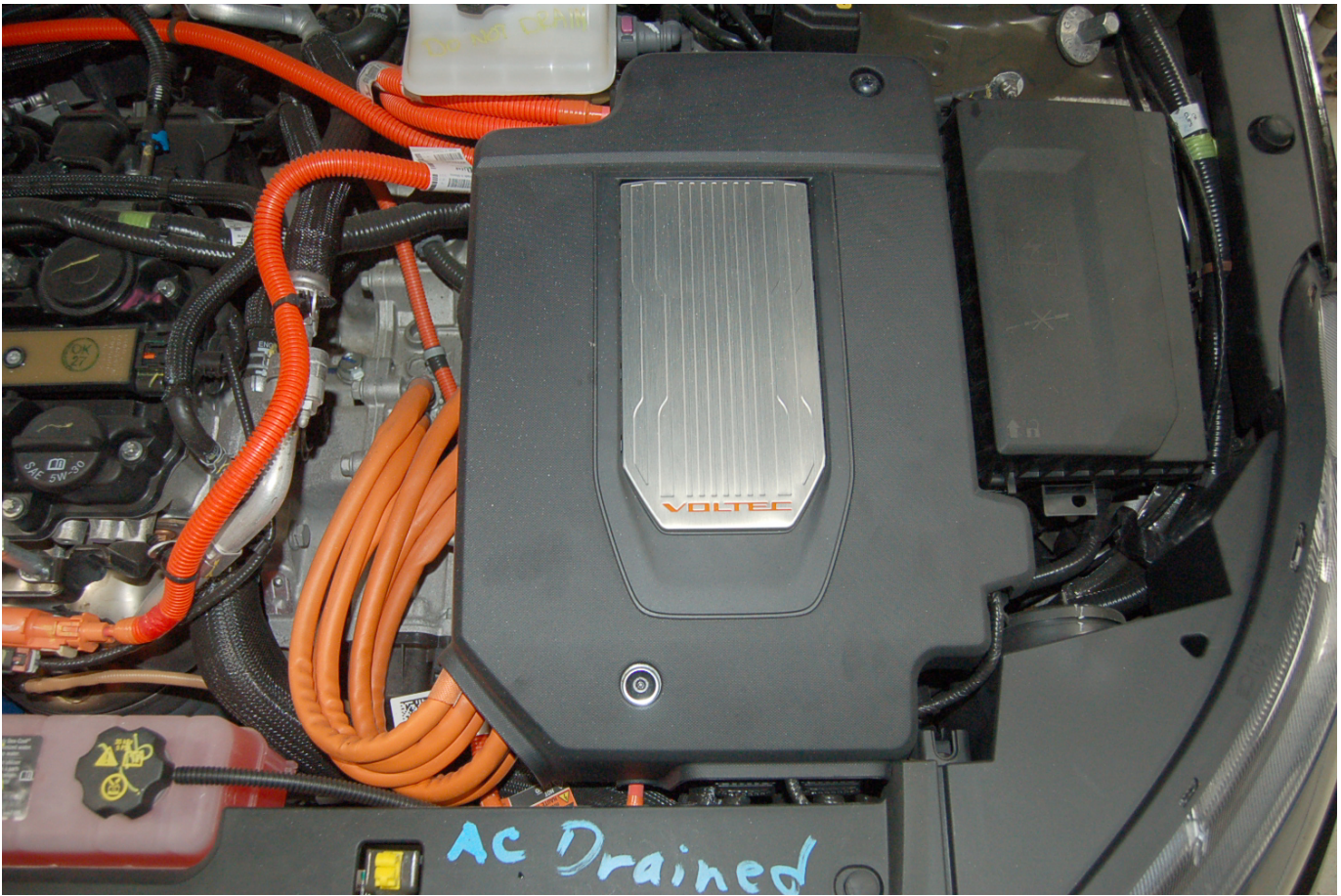
View of Electric Propulsion Drive
