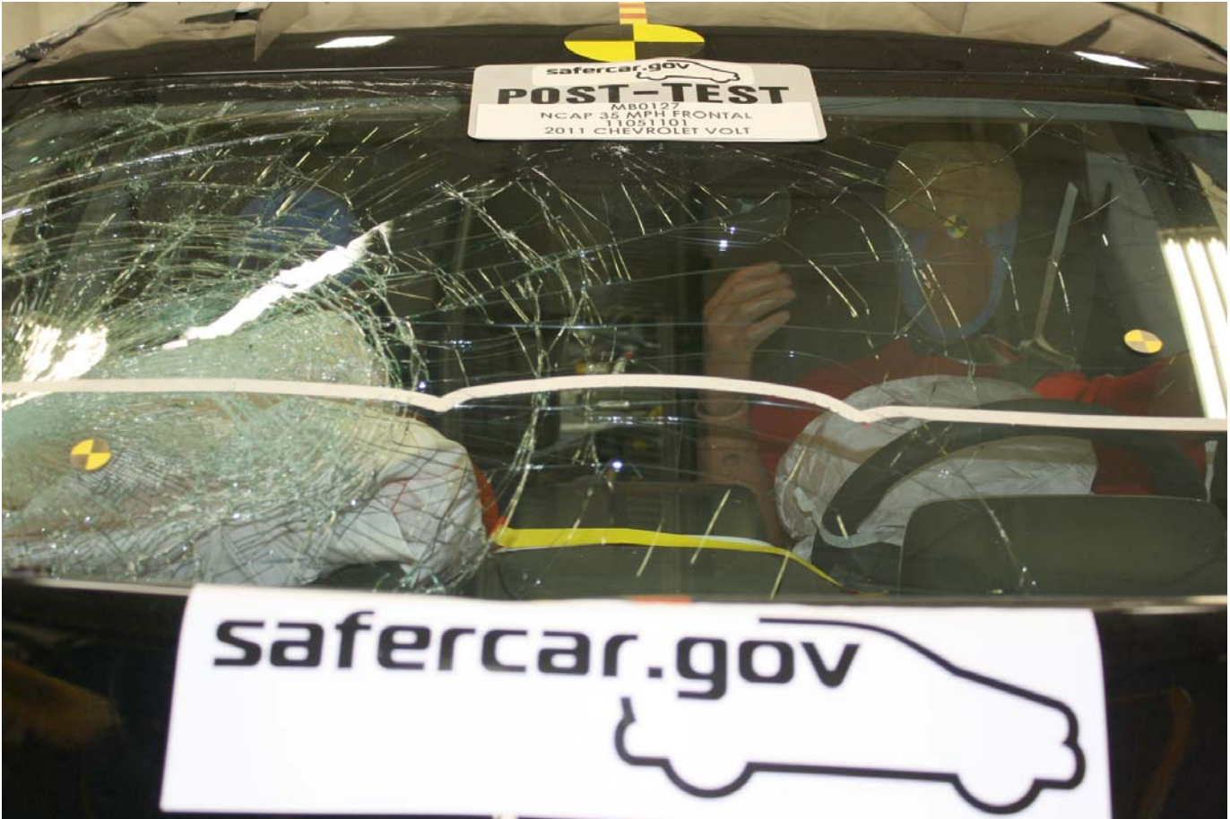
Post-Test Windshield View
