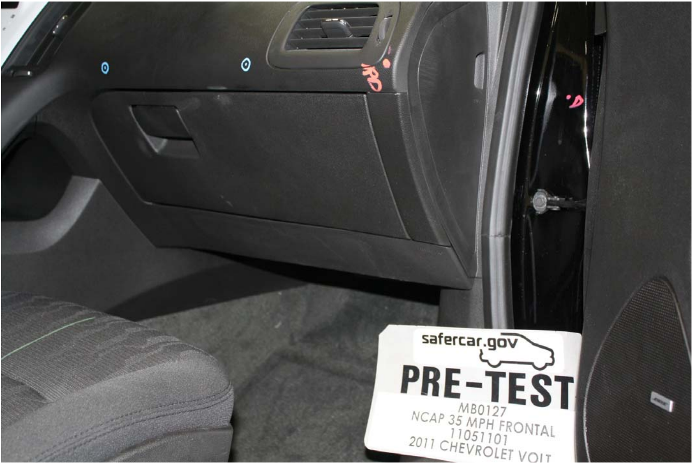
Pre-Test Passenger's Side Knee Bolster (without dummy)
