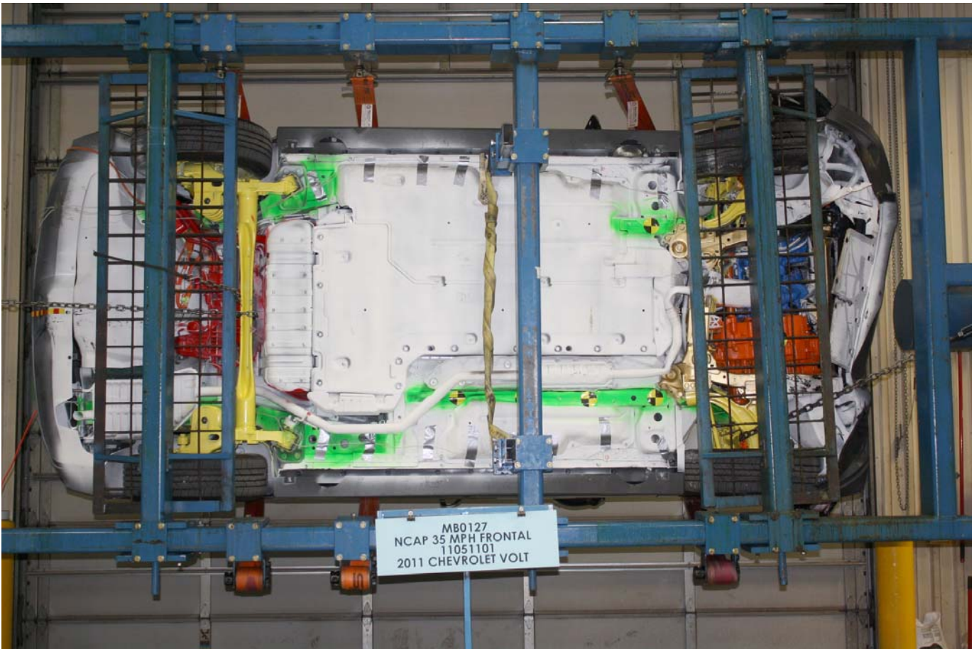
Vehicle at 270 Degrees on Static Rollover Device
