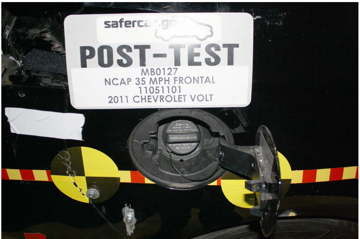
Post-Test Fuel Cap View
