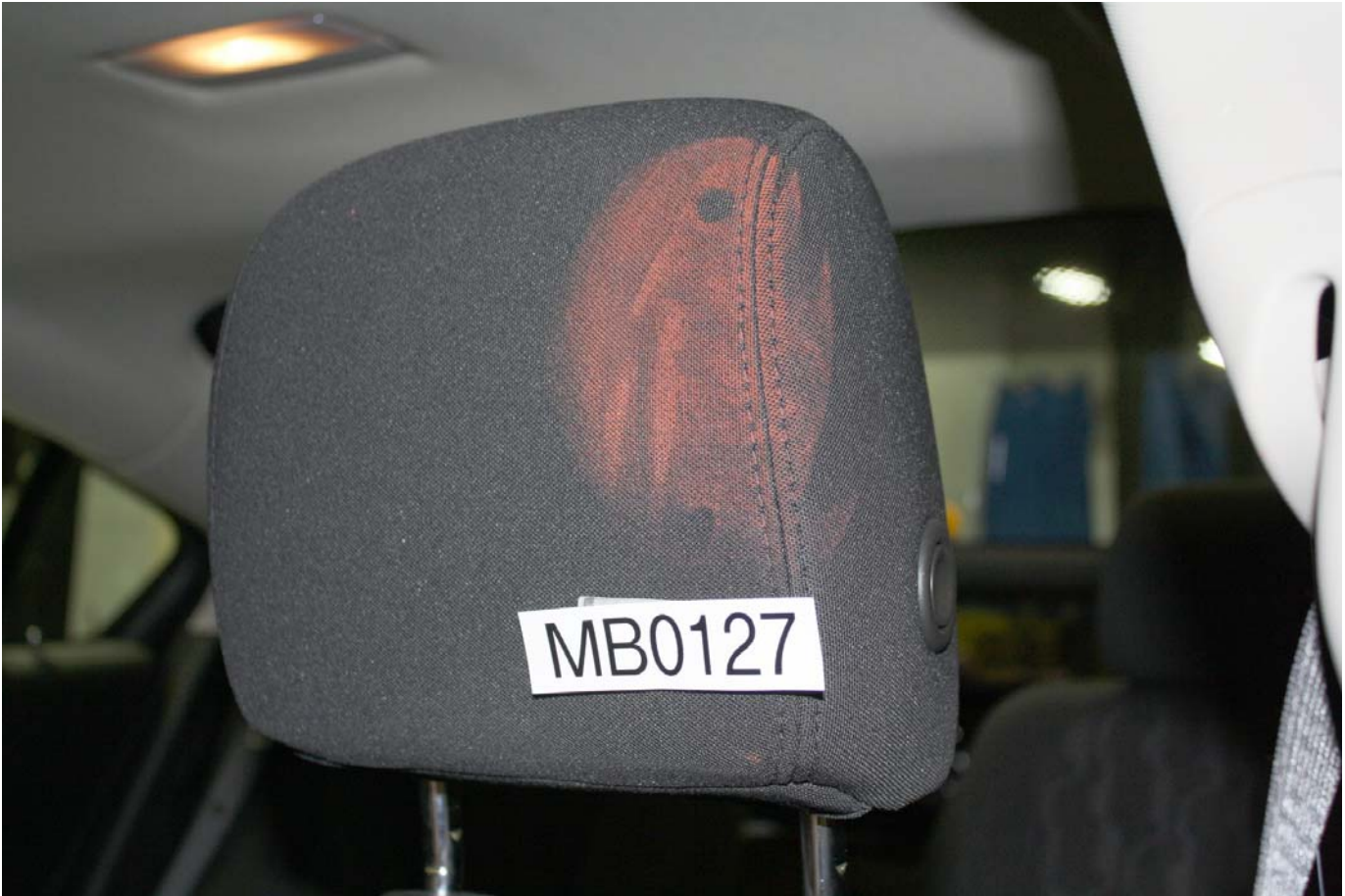
Post-Test Driver Dummy Contact with Headrest
