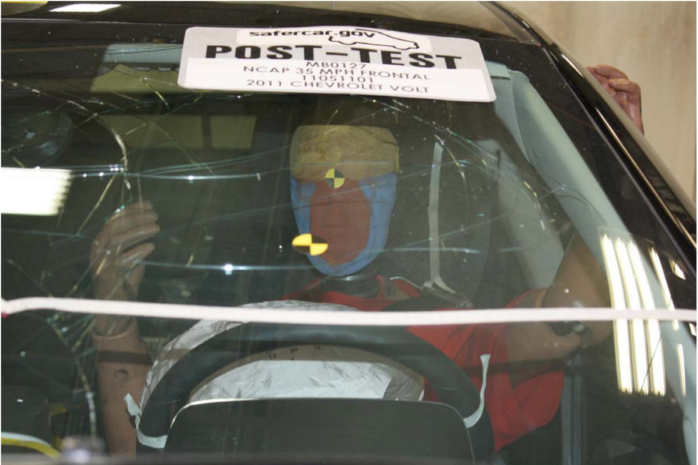
Post-Test Driver Dummy Front View
