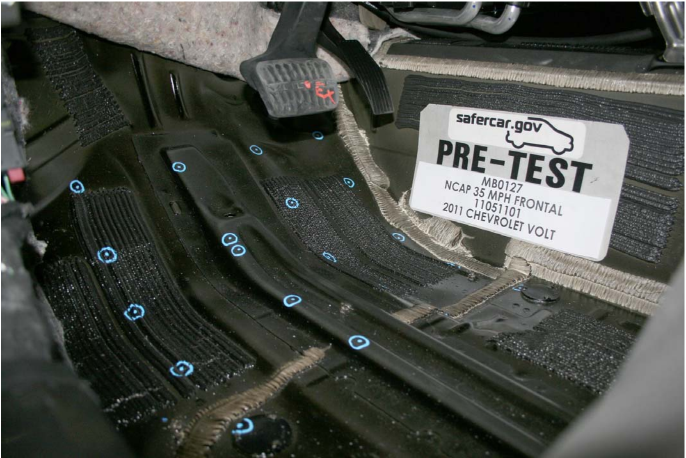
Pre-Test Driver's Side Floorpan
