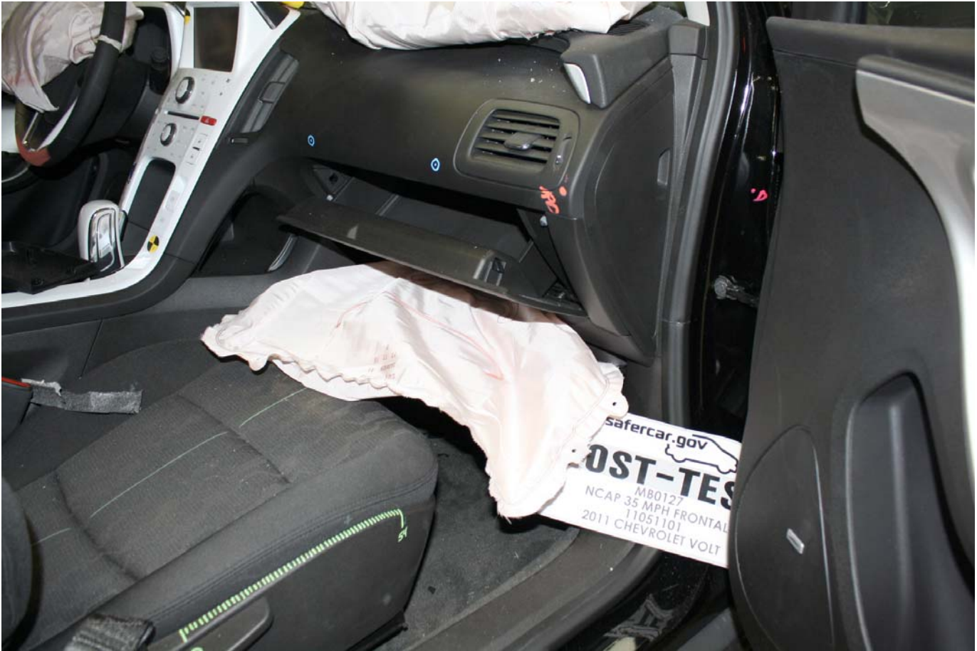
Post-Test Passenger's Side Knee Bolster (without dummy)
