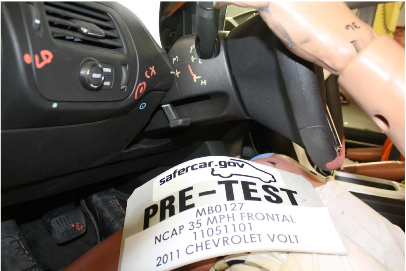
Pre-Test View of Steering Column Shear Capsule
