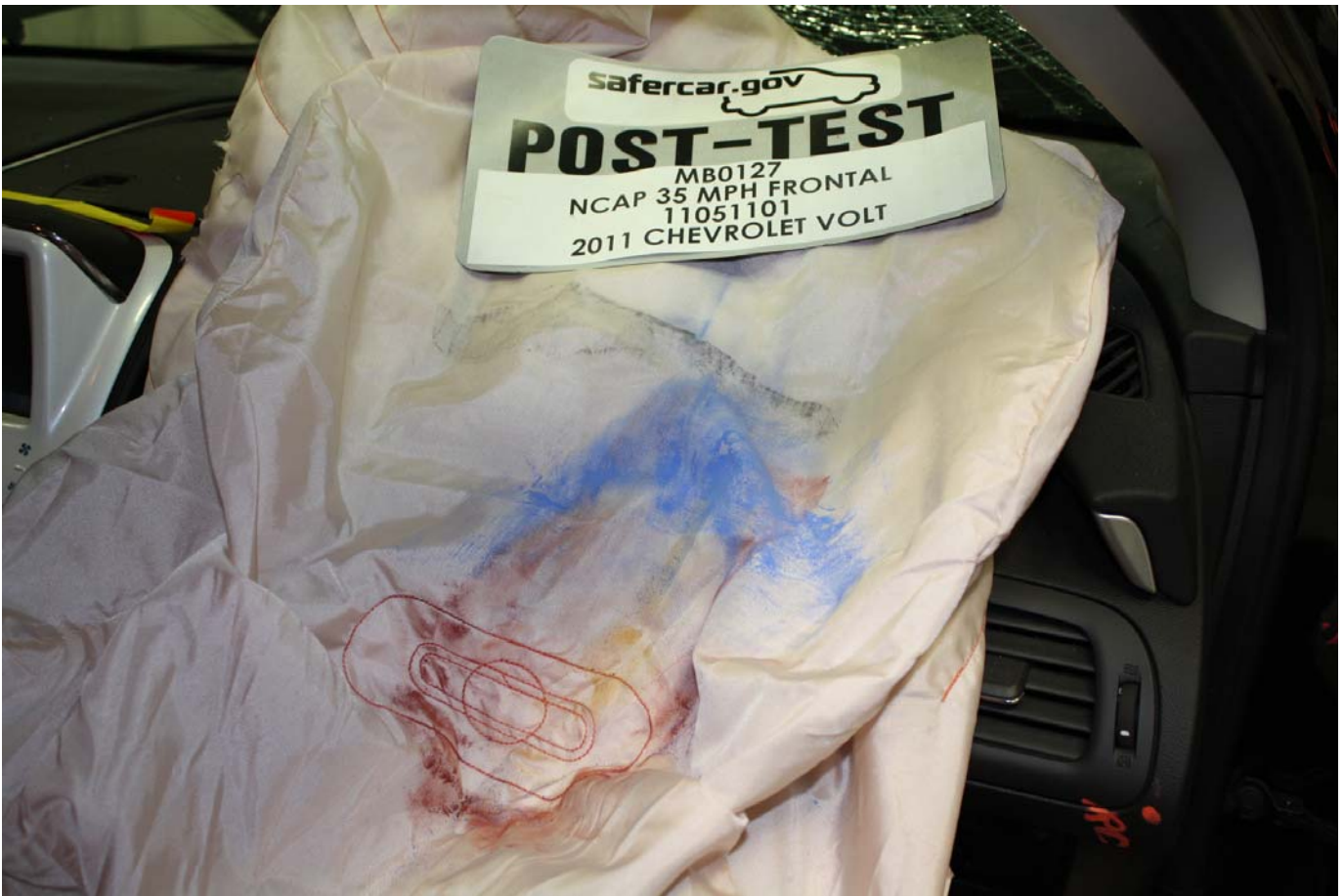
Post-Test Passenger Dummy Contact with Airbag
