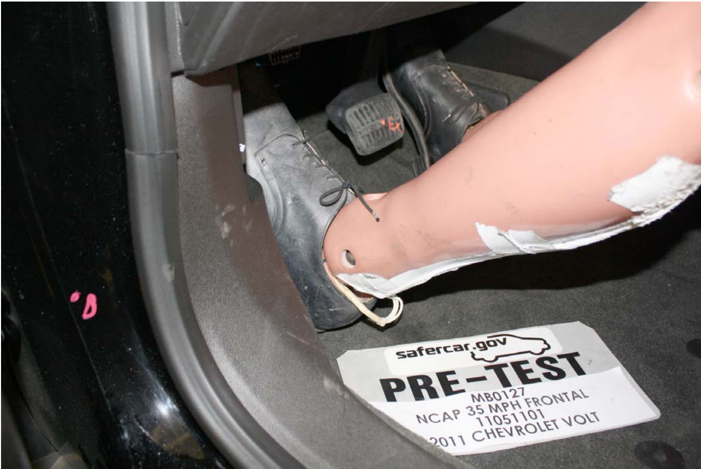
Pre-Test Driver Dummy Feet
