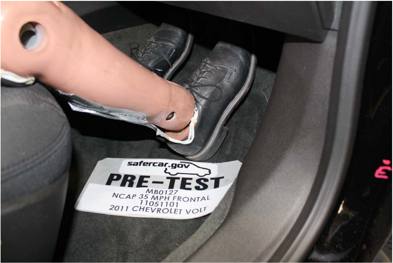
Pre-Test Passenger Dummy Feet
