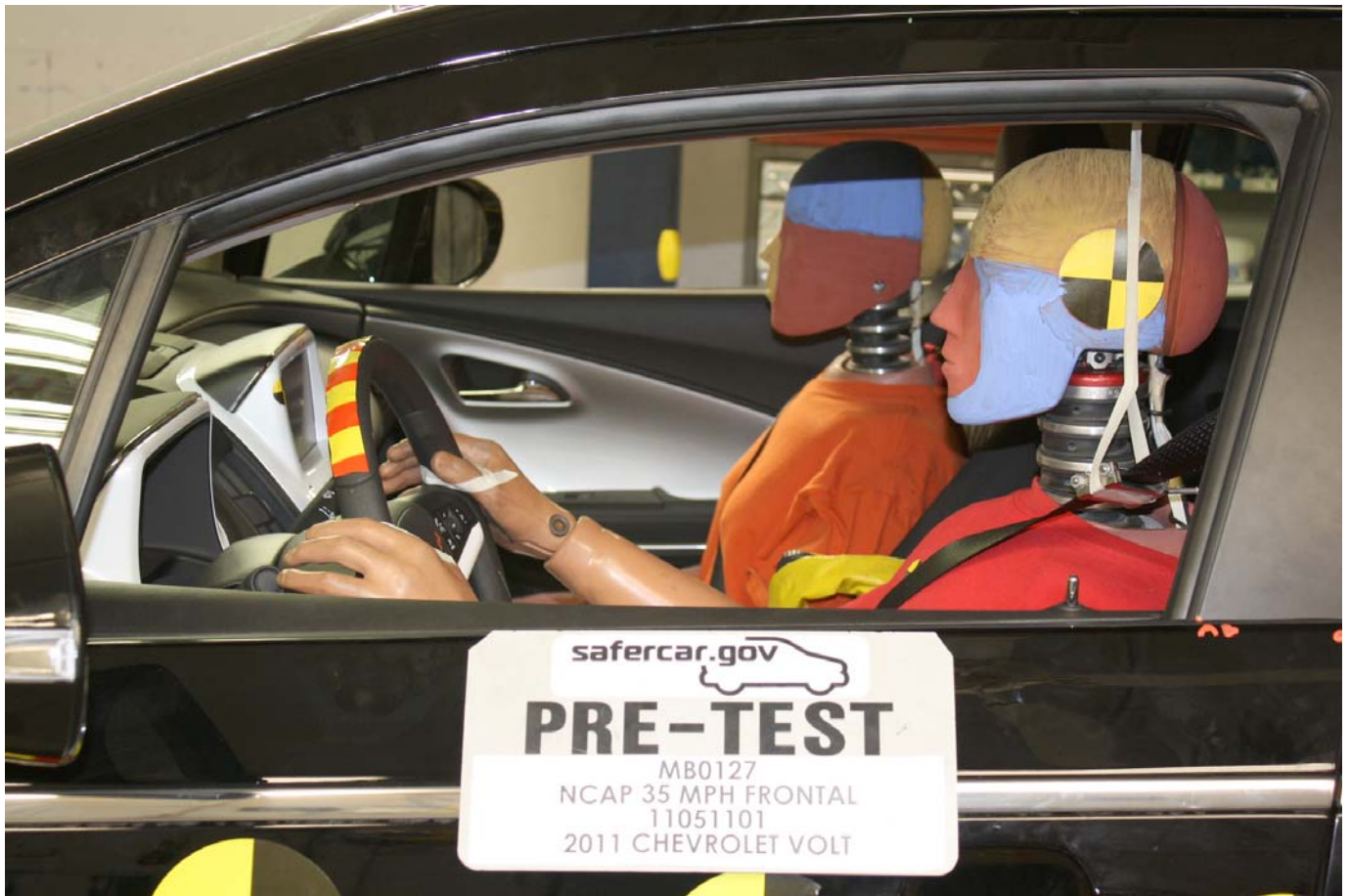
Pre-Test Driver Dummy Window View
