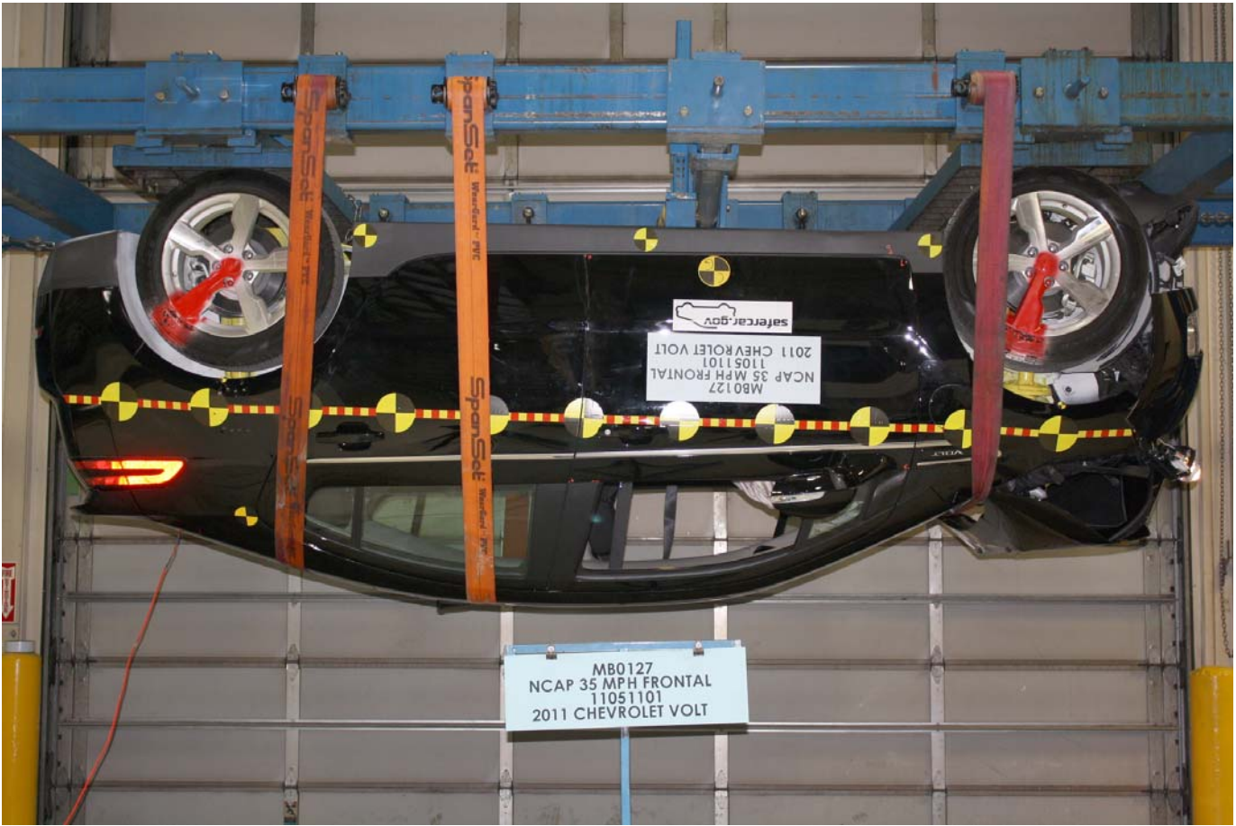
Vehicle at 180 Degrees on Static Rollover Device
