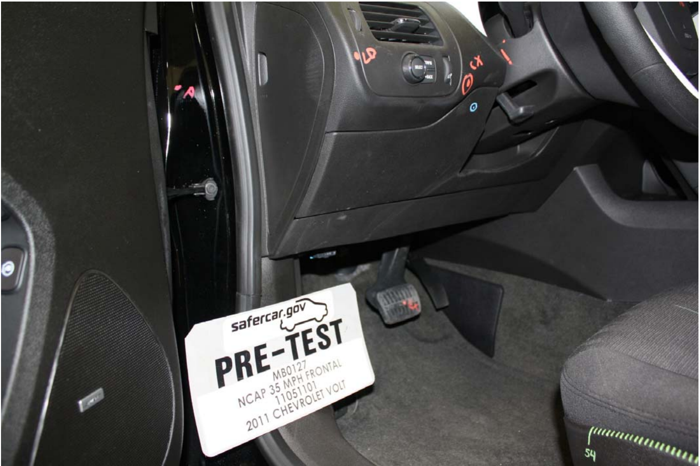
Pre-Test Driver's Side Knee Bolster (without dummy)
