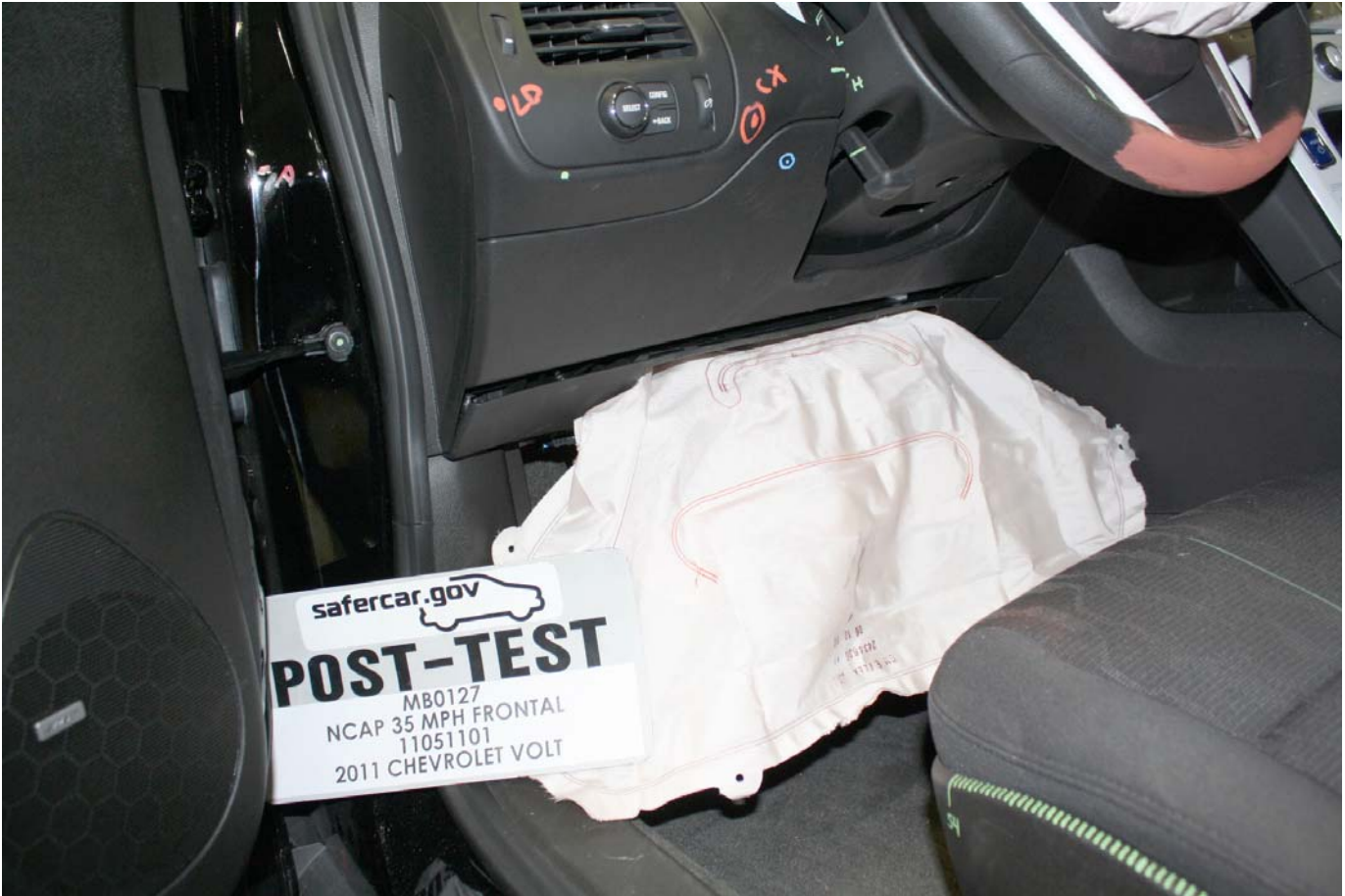
Post-Test Driver's Side Knee Bolster (without dummy)
