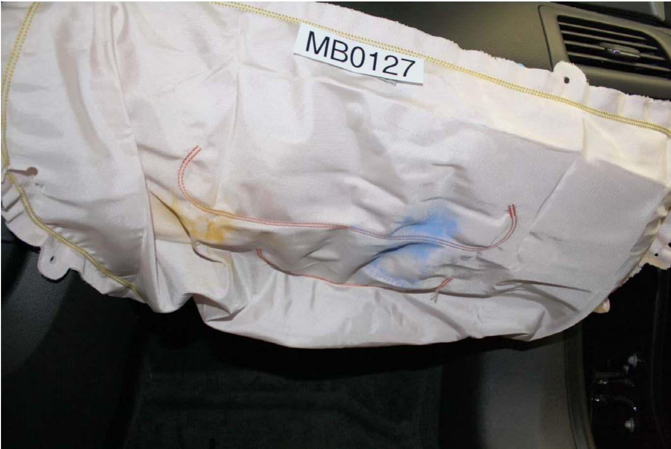
Post-Test Passenger Dummy Contact with Knee Airbag
