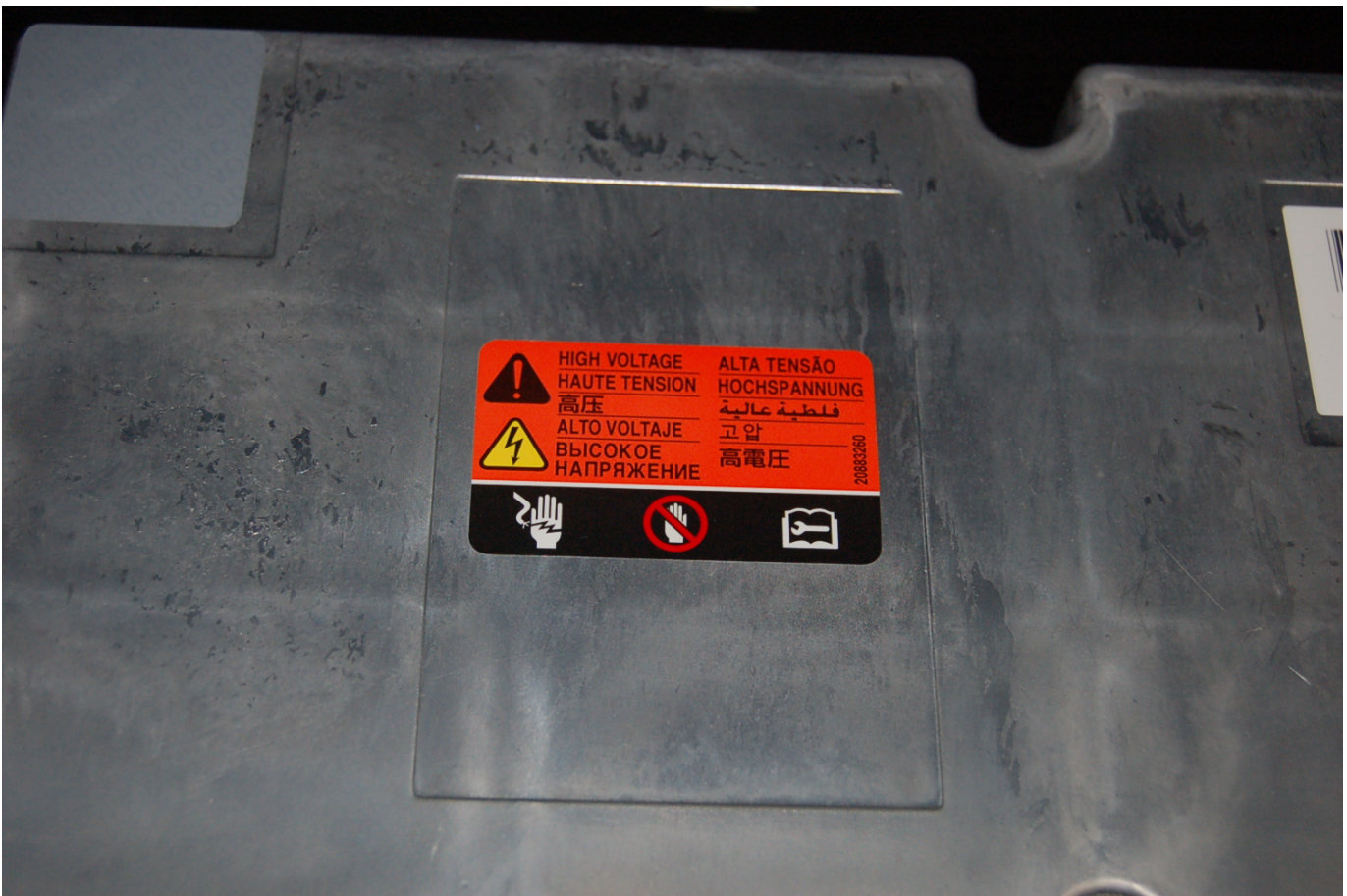
Auxiliary Power Module Warning Label
