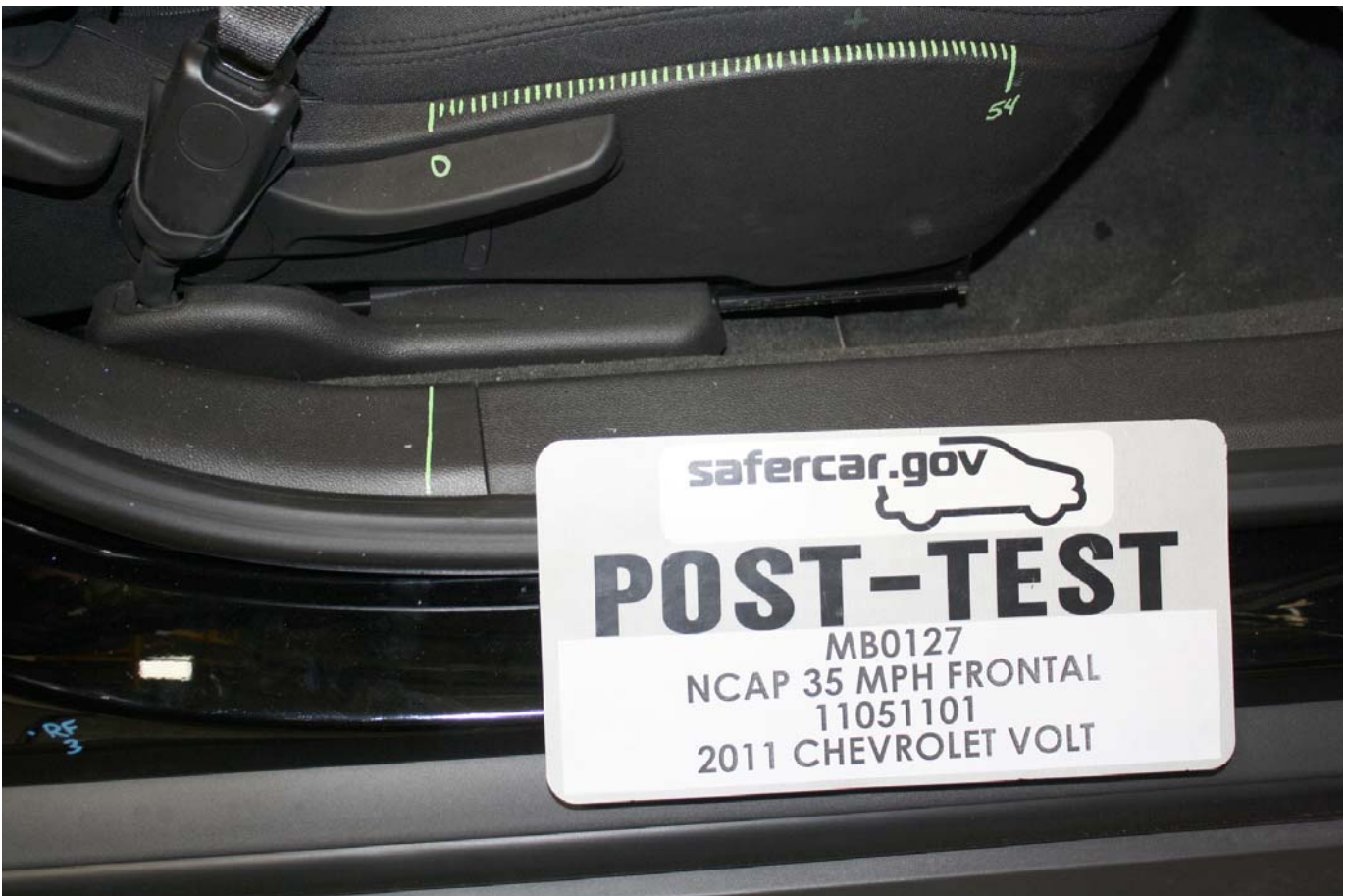
Post-Test Passenger's Seat Fore-Aft Markings
