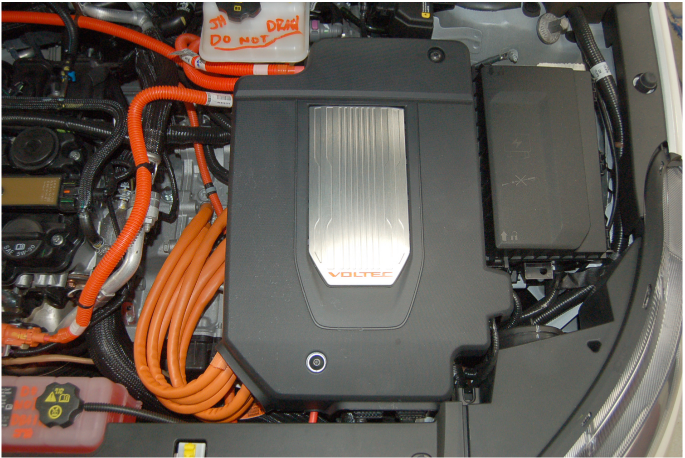
View of Electric Propulsion Drive
