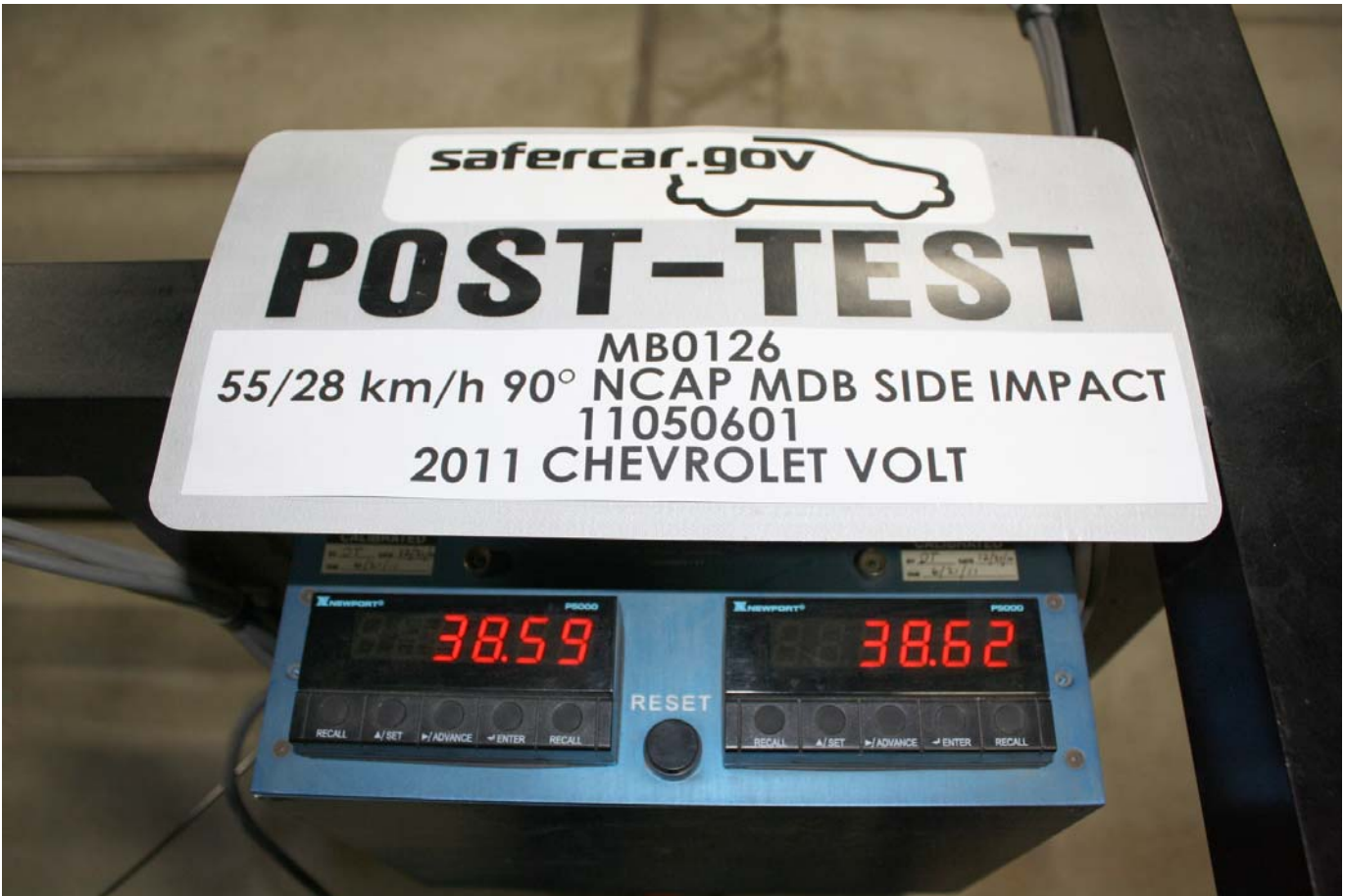
Post-Test Primary and Redundant Speed Trap Read-Out
