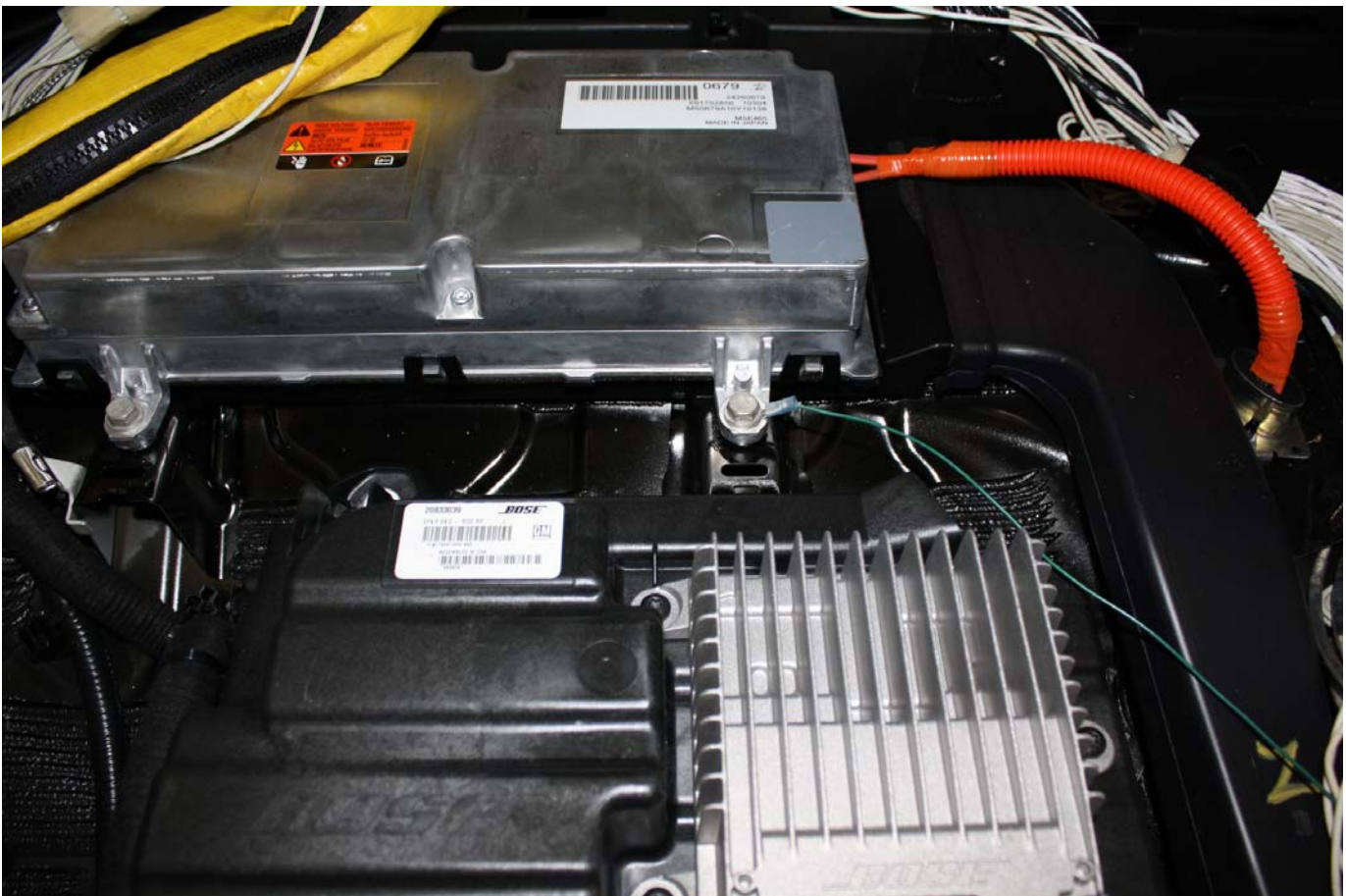
Close-Up of Ground Lead Attached
