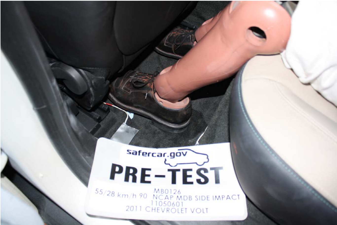
Pre-Test Placement of Rear Passenger Dummy's Feet
