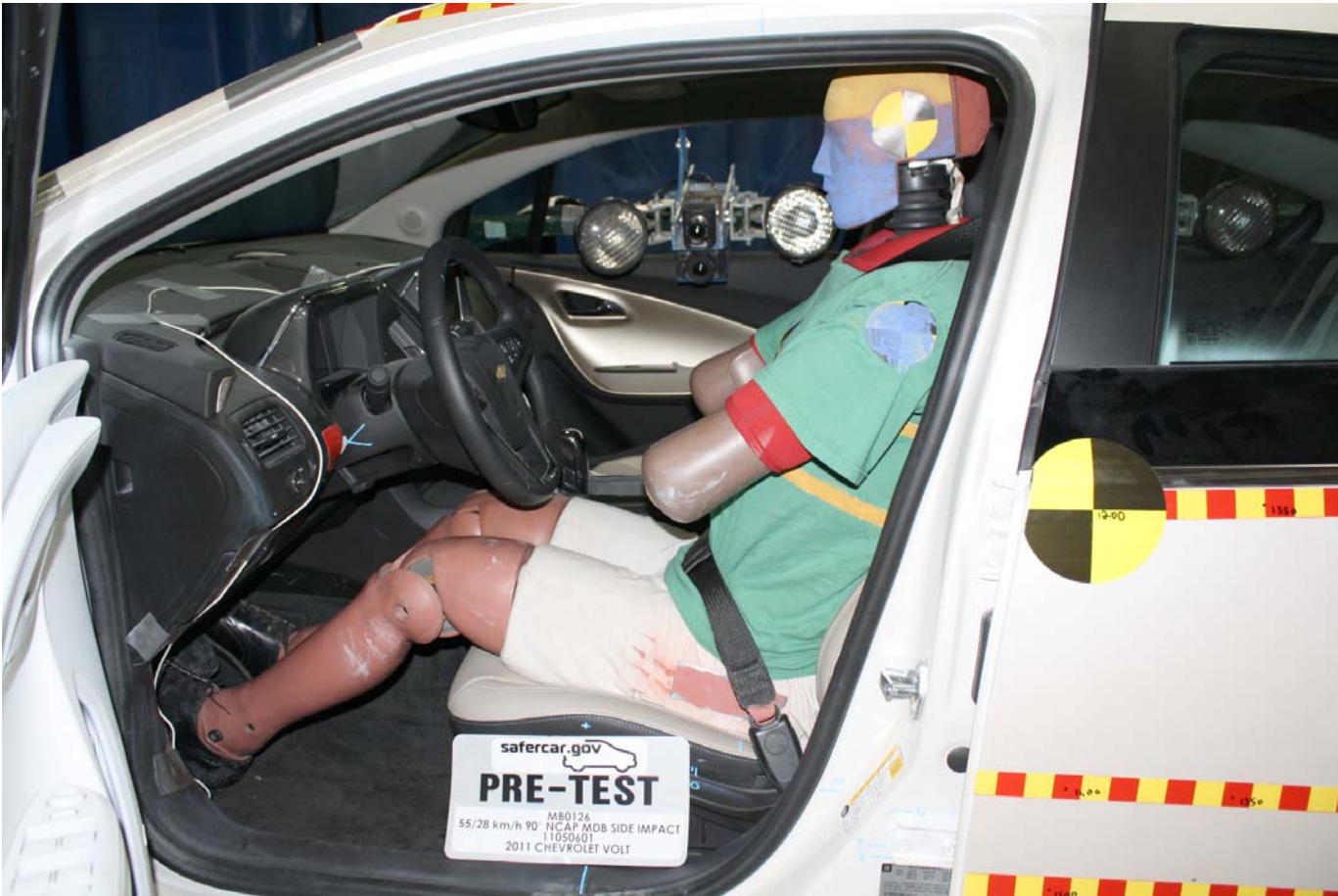
Pre-Test Left Side View of Driver Dummy Showing Belt, Chalking, and Contact Switches
