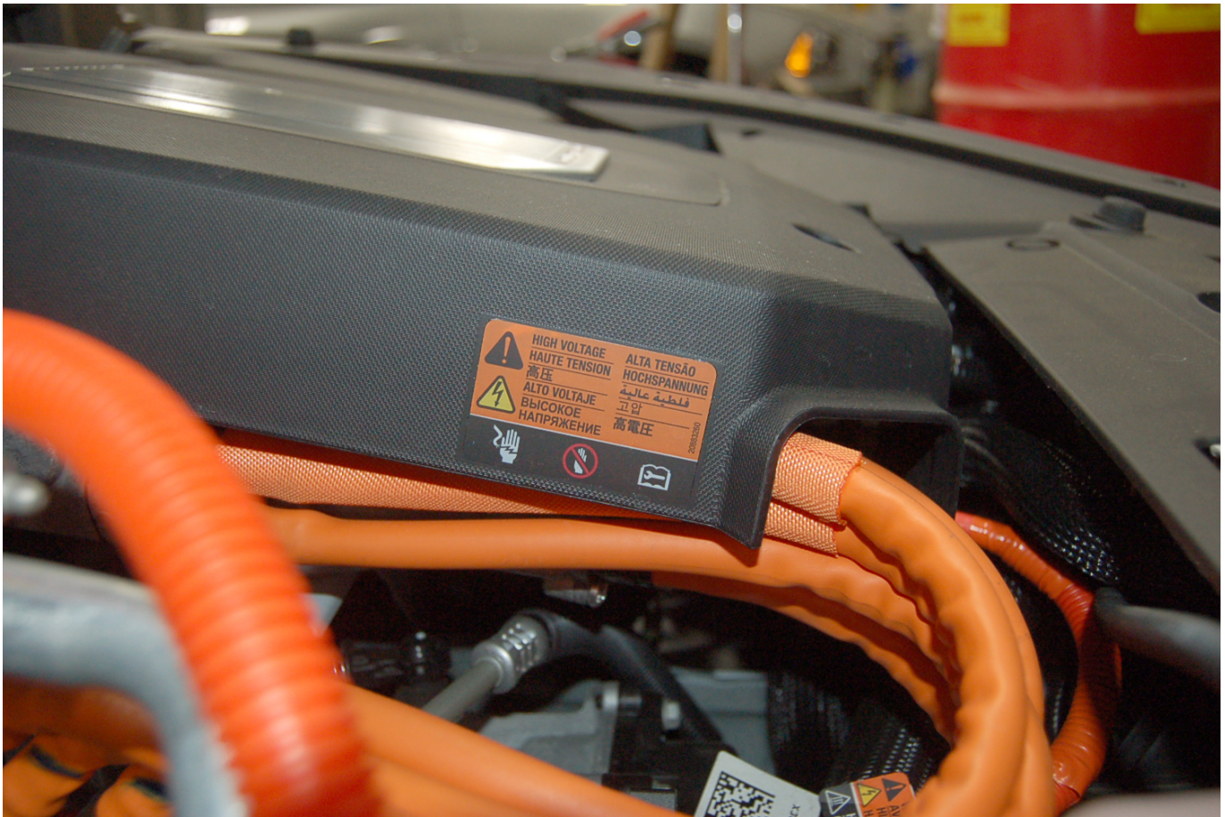
Power Inverter Warning Label
