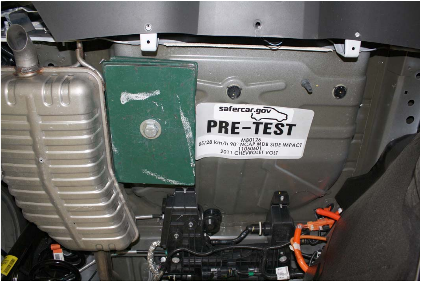
Pre-Test Ballast View
