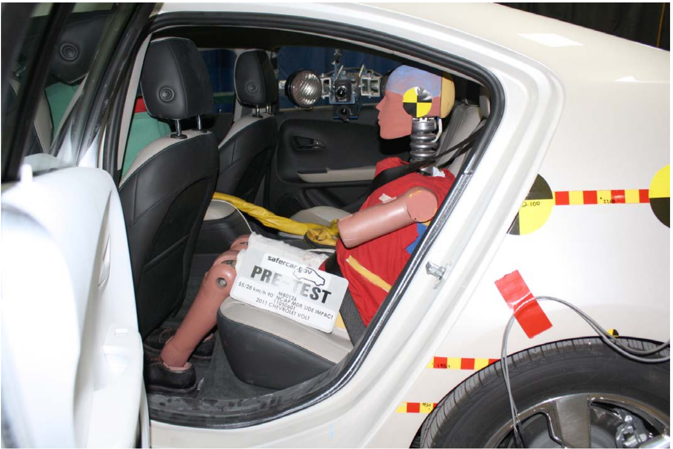
Pre-Test Left Side View of Passenger Dummy Showing Belt, Chalking, and Contact Switches
