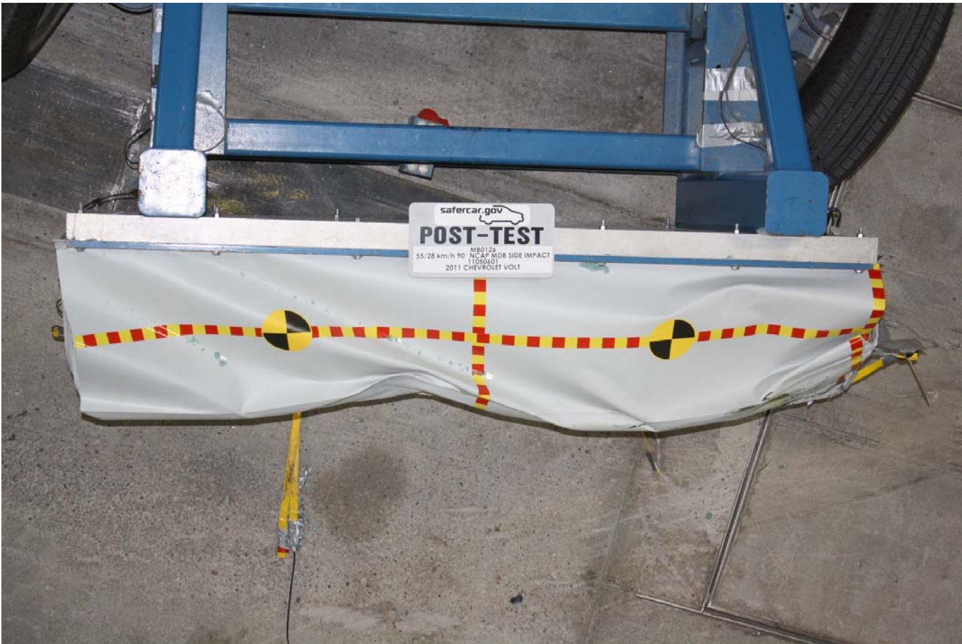
Post-Test Top View of MDB Impactor Face
