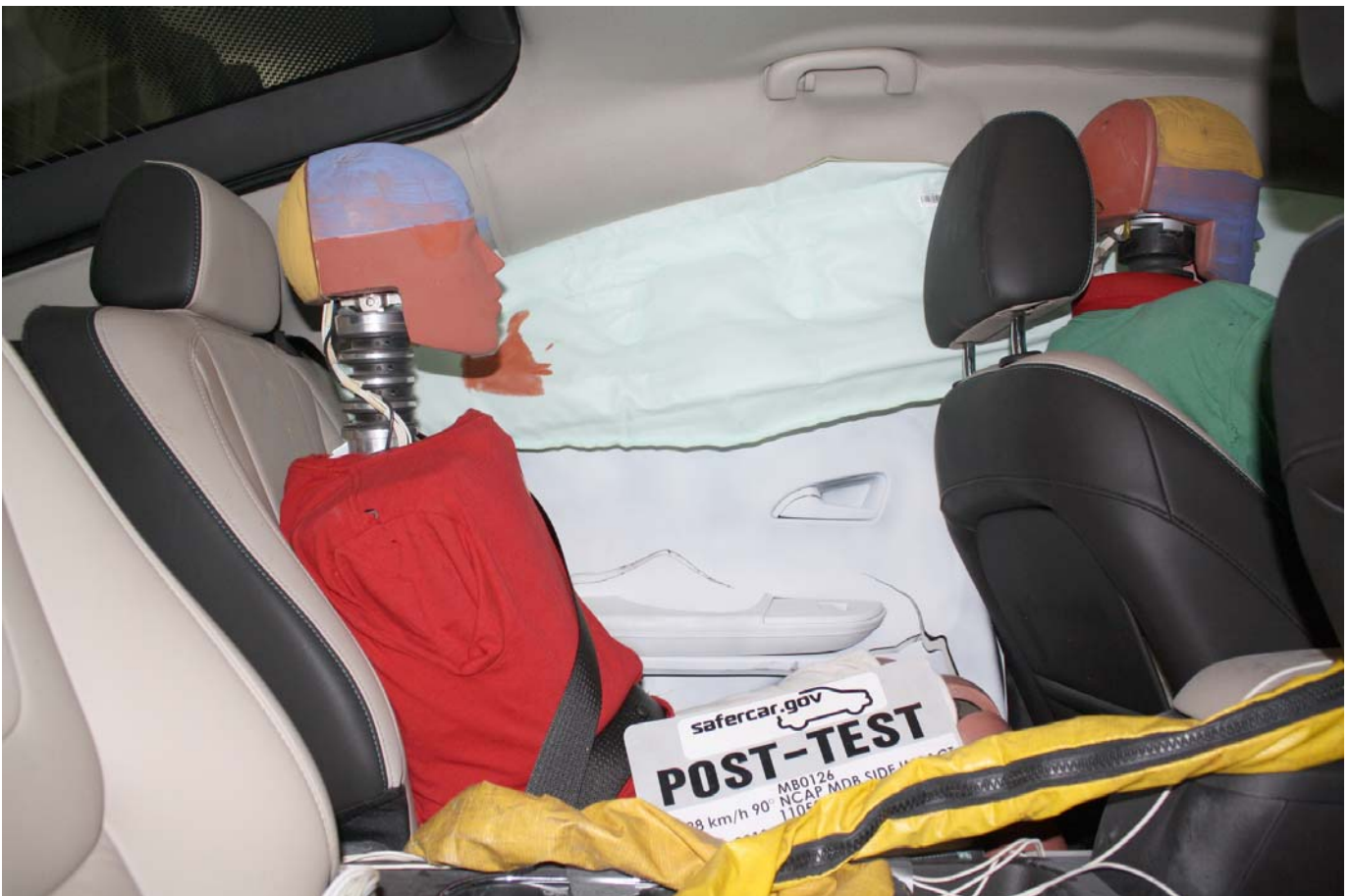
Post-Test Right Side View of Rear Passenger Dummy Seat and Rear Seat Occupant Compartment
