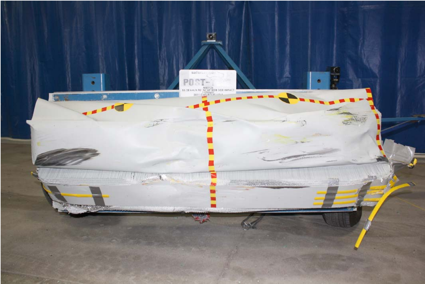
Post-Test Front View of MDB Impactor Face
