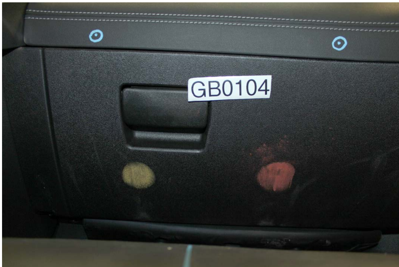
Post-Test Passenger Dummy Contact with Glovebox
