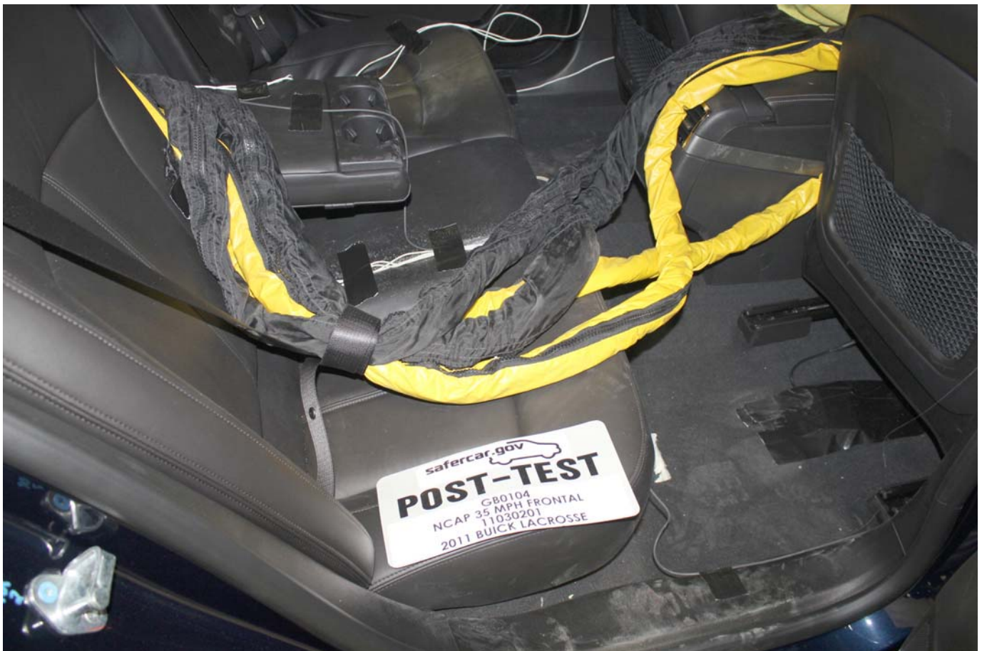
Post-Test Dummy Cable Routing
