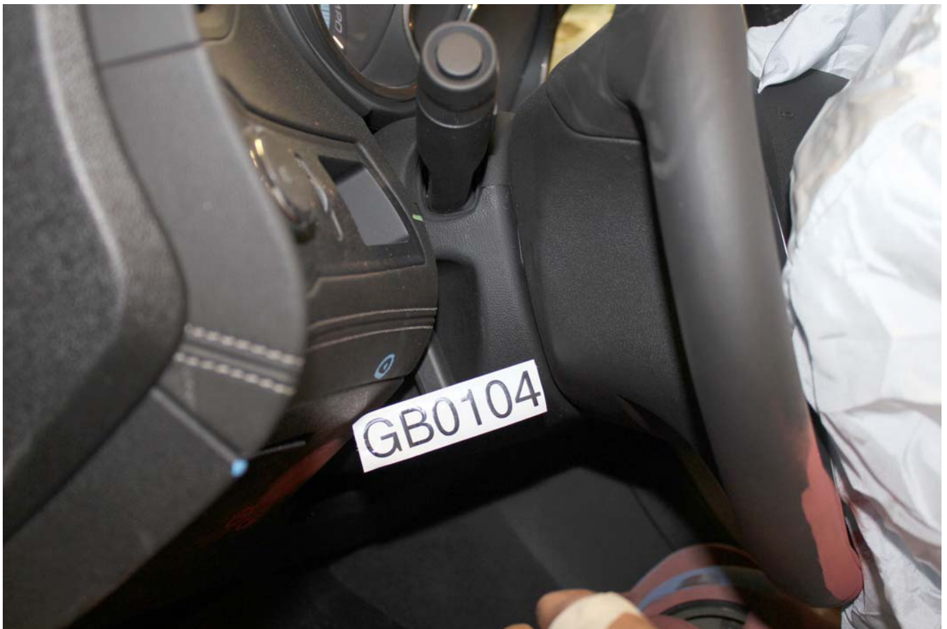
Post-Test View of Steering Column Shear Capsule
