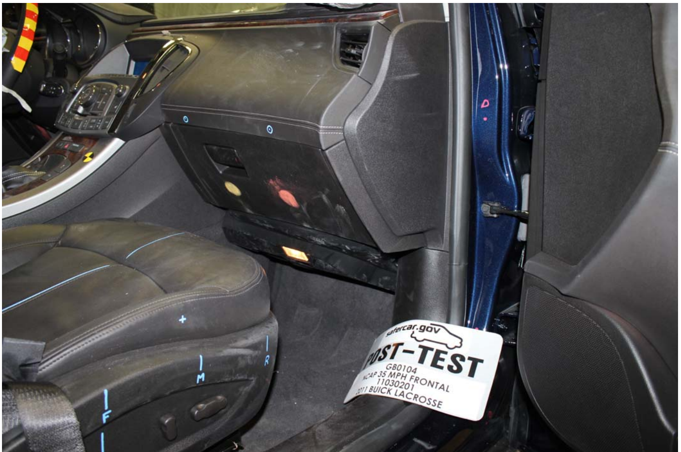
Post-Test Passenger's Side Knee Bolster (without dummy)
