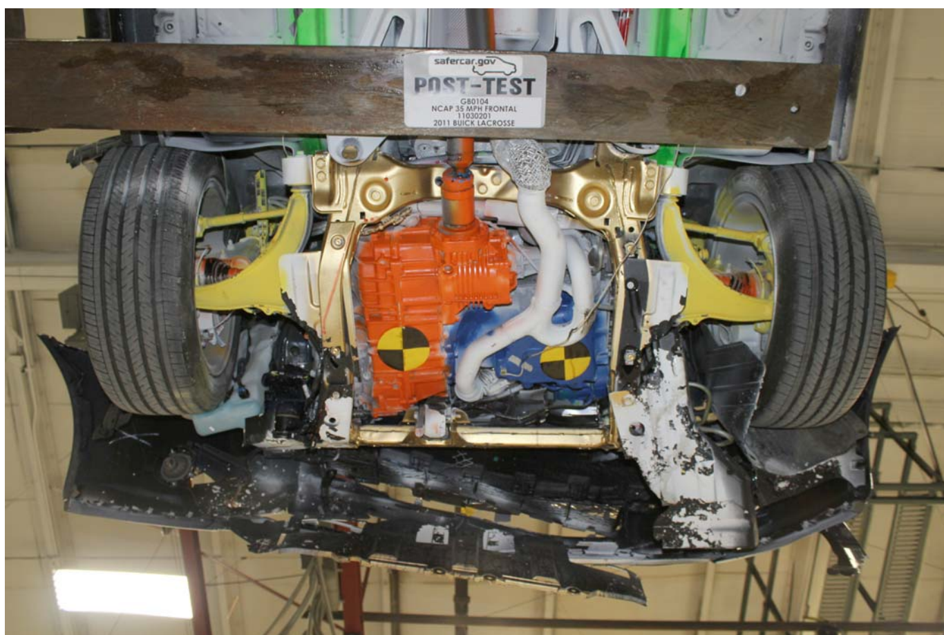
Post-Test Front Underbody View
