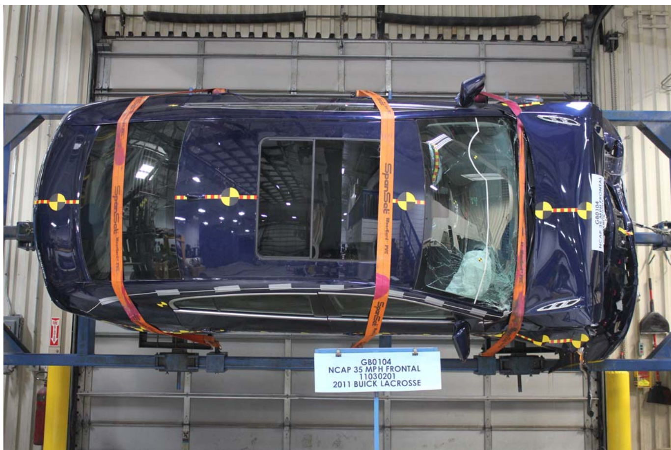
Vehicle at 90 Degrees on Static Rollover Device
