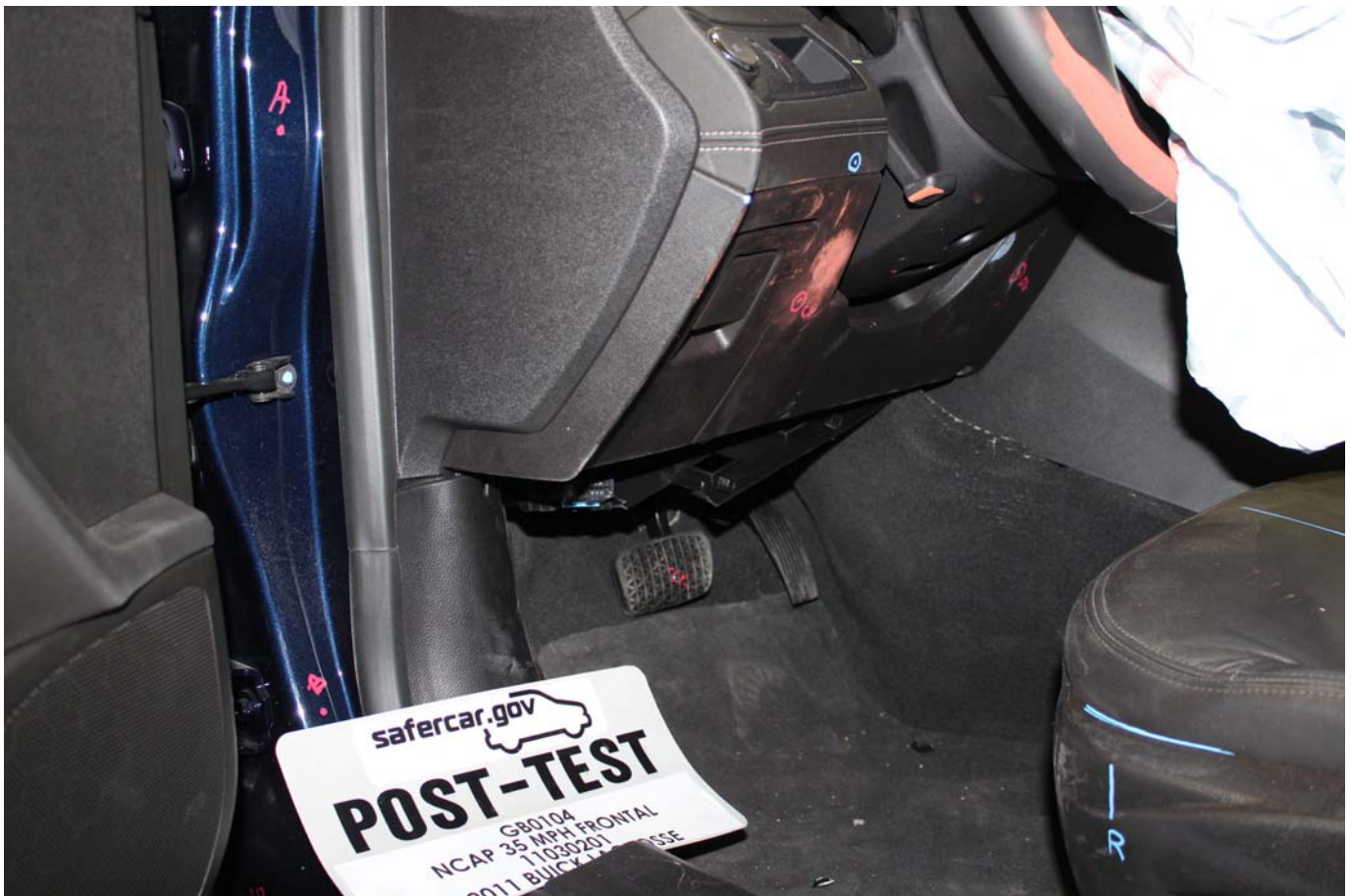
Post-Test Driver's Side Knee Bolster (without dummy)
