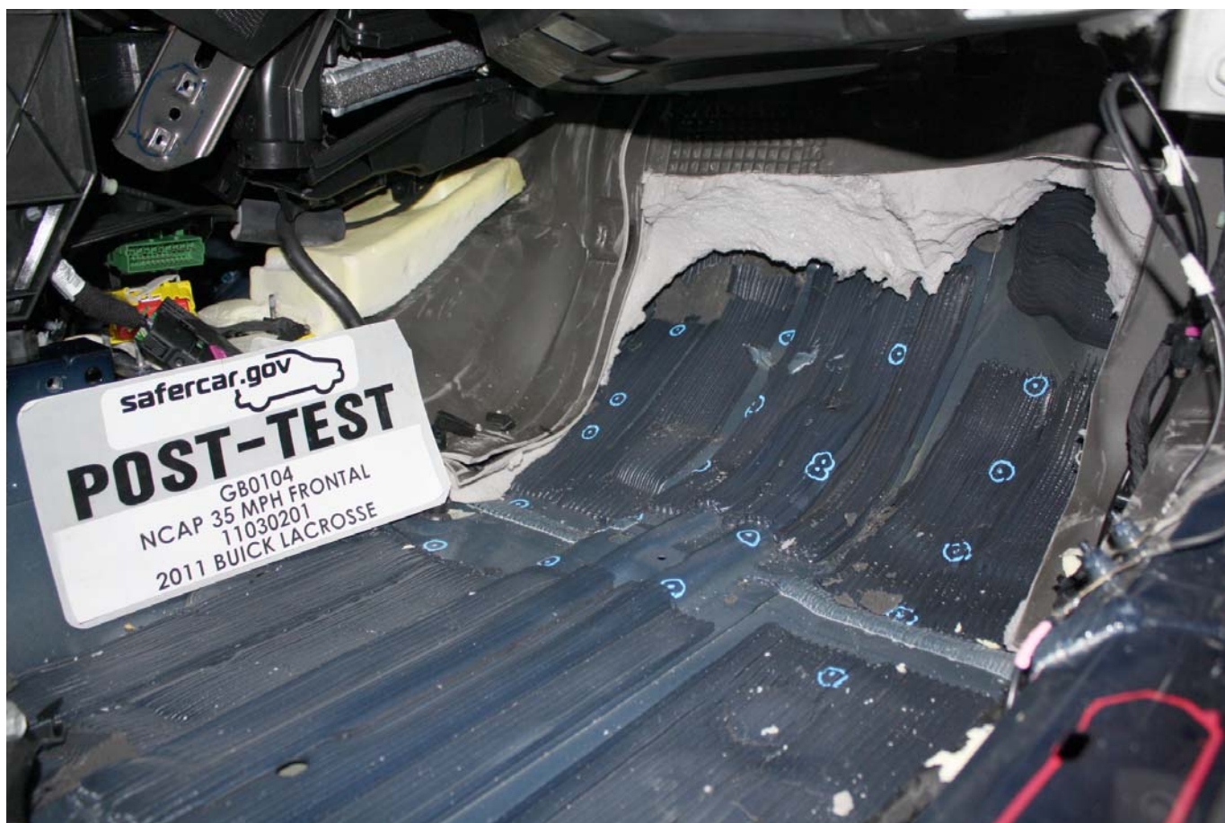
Post-Test Passenger's Side Floorpan
