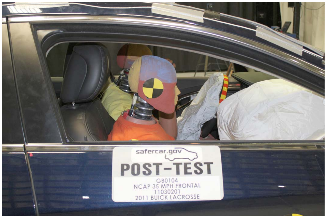
Post-Test Passenger Dummy Window View
