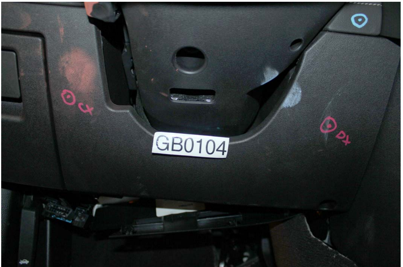
Post-Test Driver Dummy Contact with Knee Bolster
