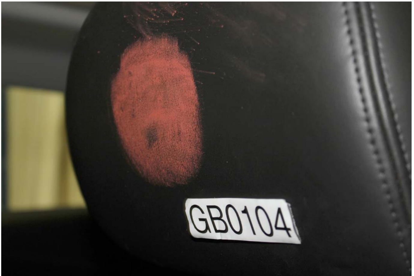
Post-Test Driver Dummy Contact with Headrest
