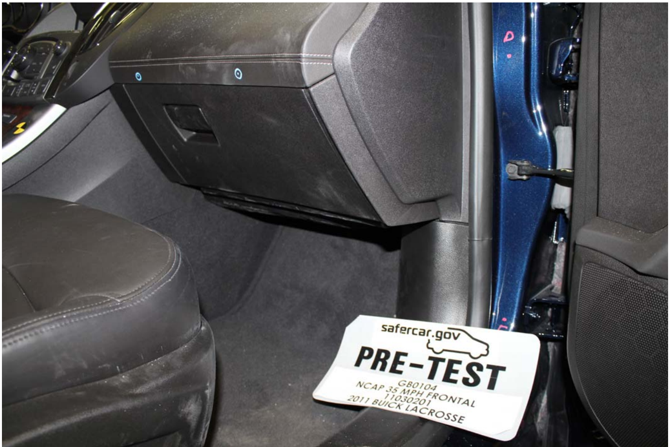
Pre-Test Passenger's Side Knee Bolster (without dummy)
