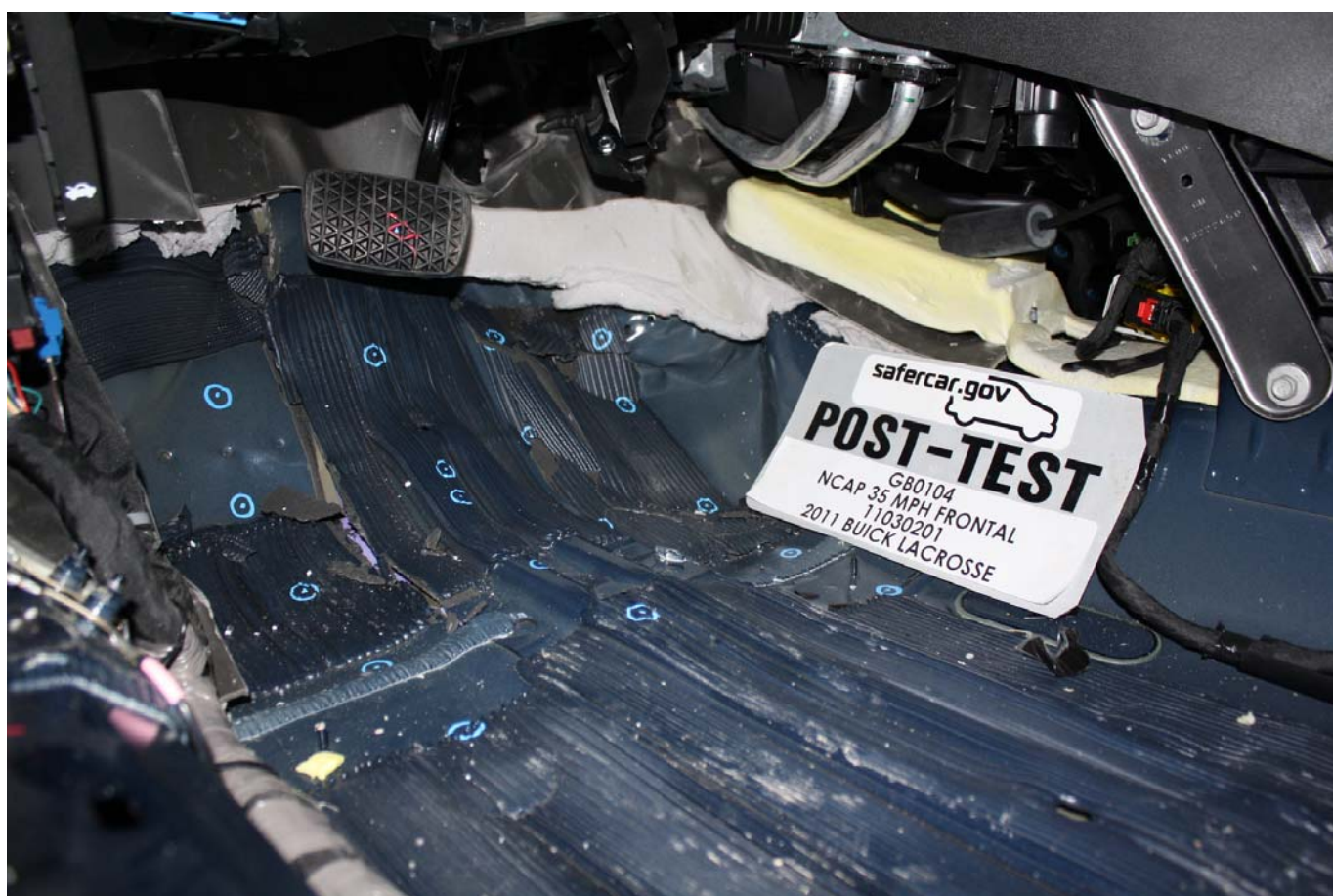
Post-Test Driver's Side Floorpan
