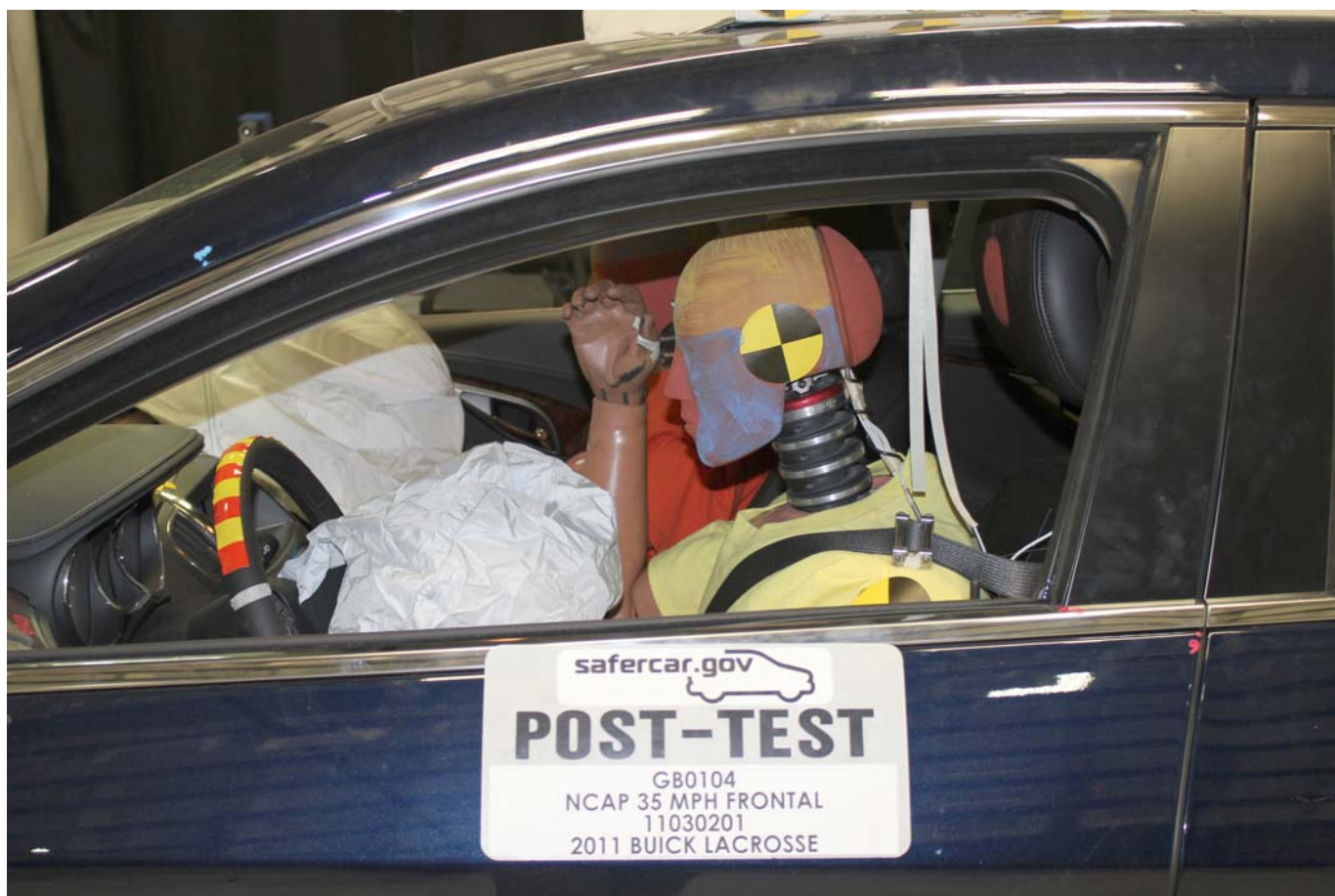
Post-Test Driver Dummy Window View
