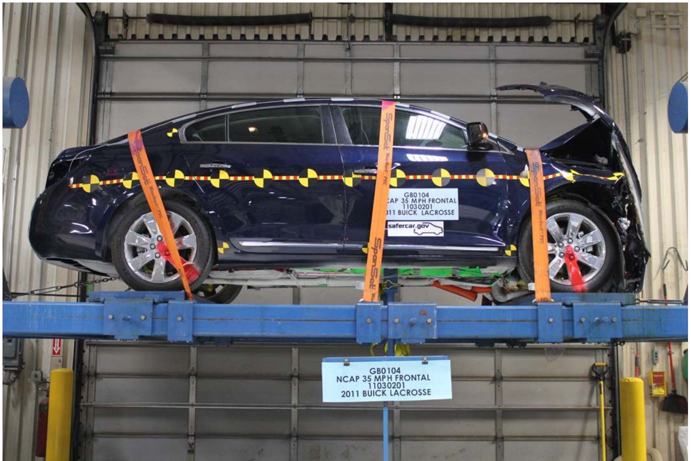
Vehicle at 360 Degrees on Static Rollover Device
