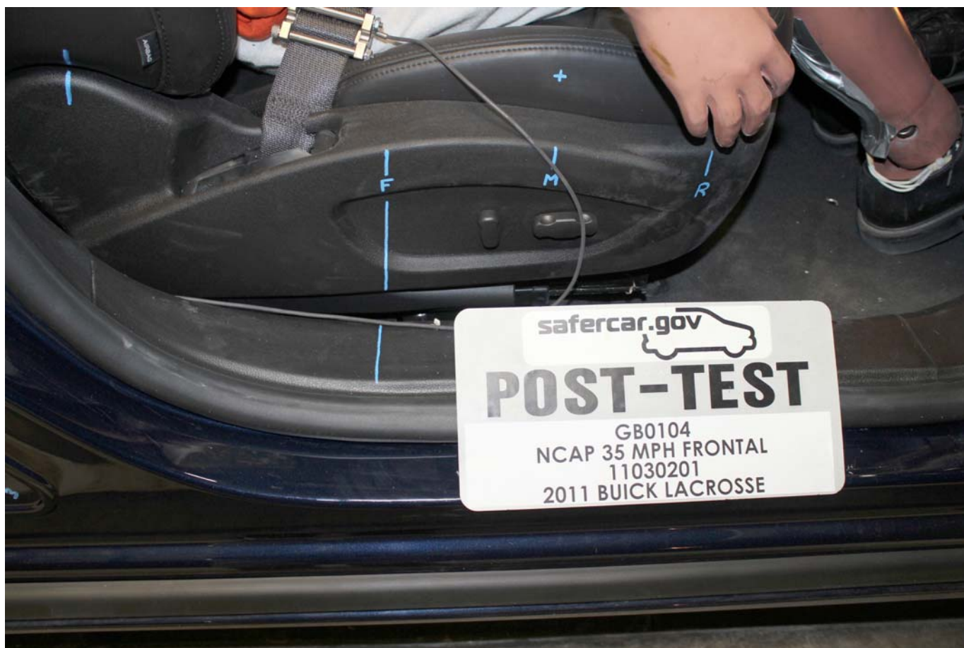
Post-Test Passenger's Seat Fore-Aft Markings
