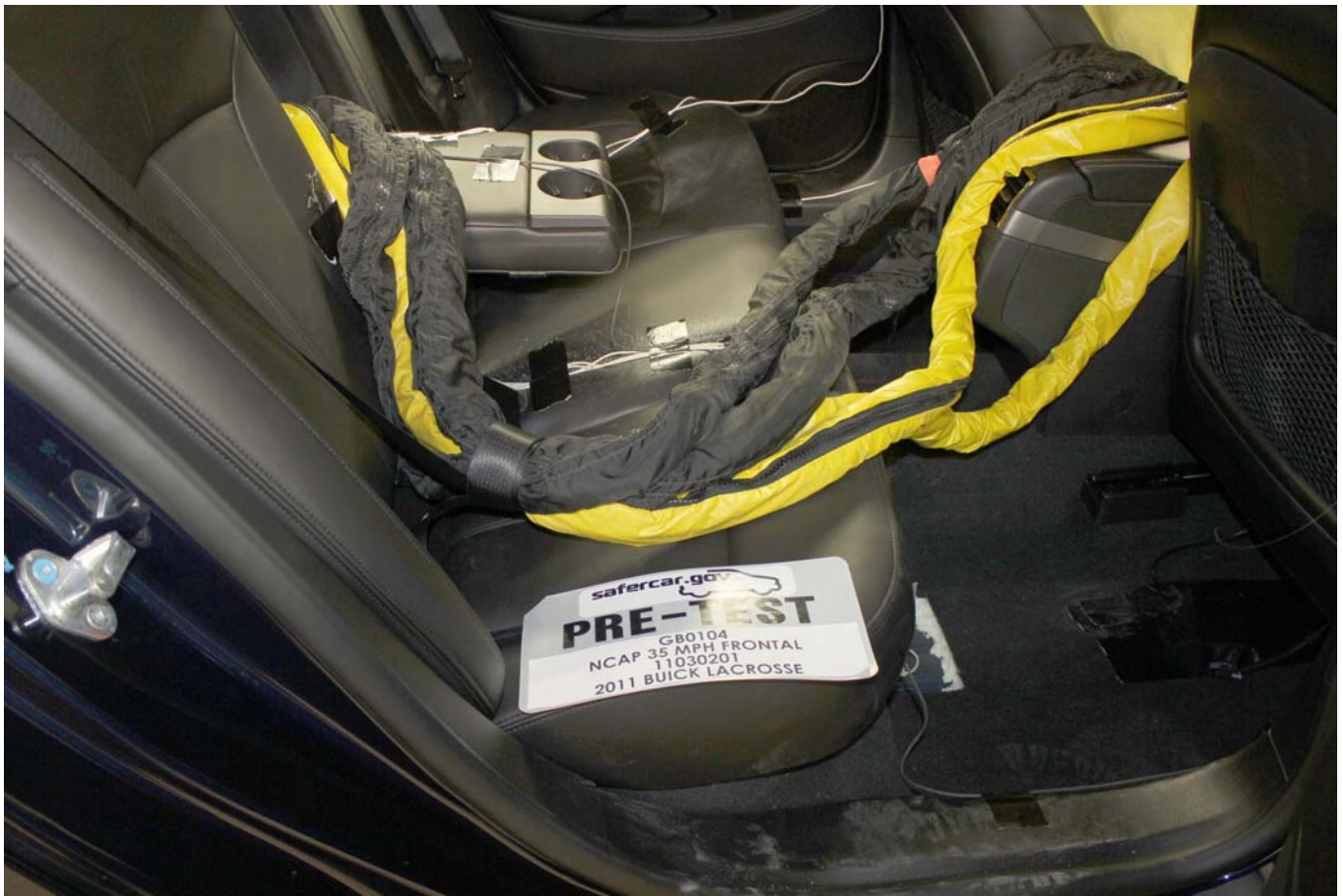
Pre-Test Dummy Cable Routing
