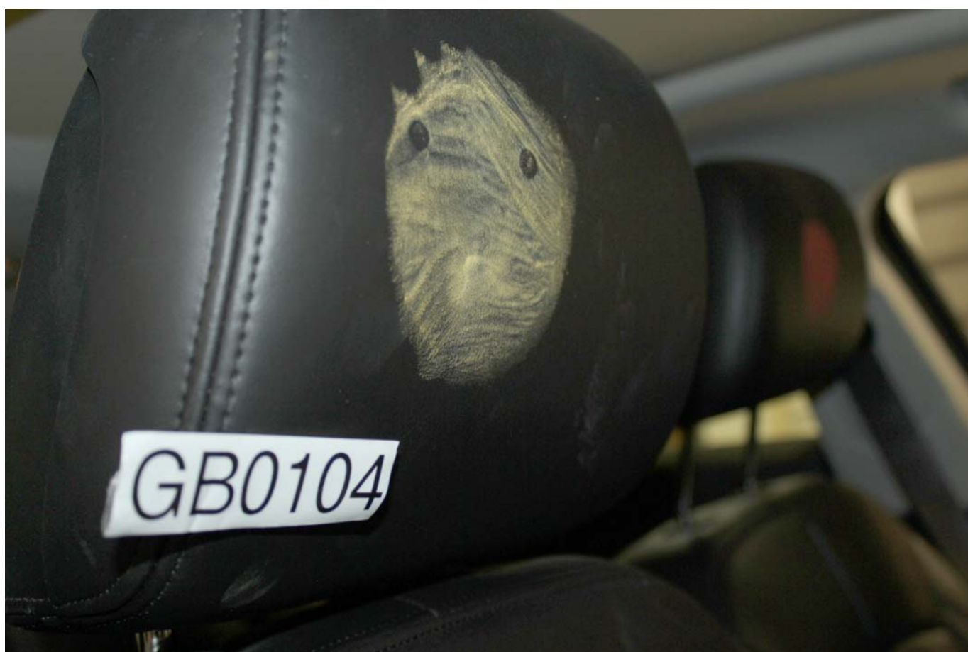
Post-Test Passenger Dummy Contact with Headrest
