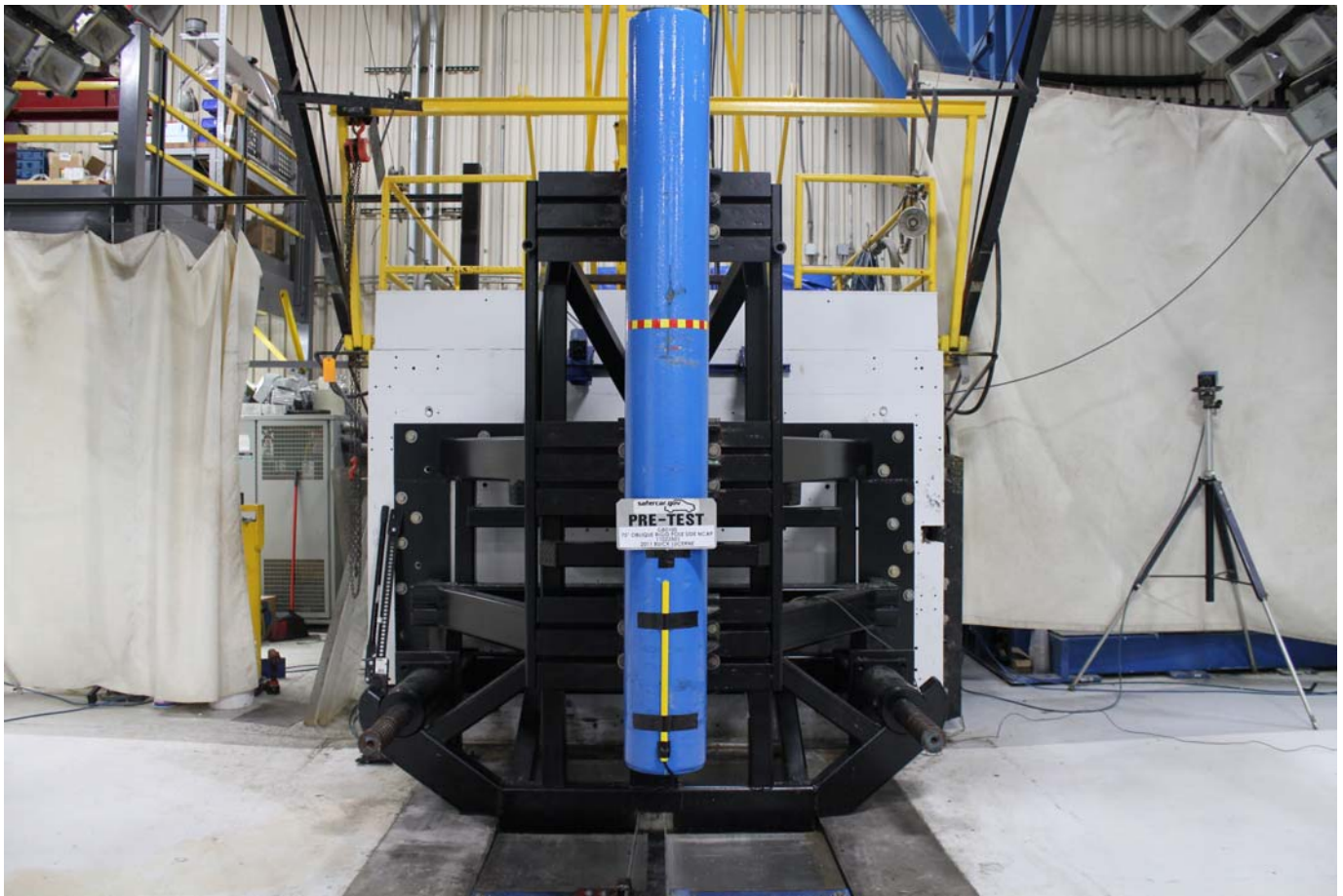
Pre-Test Pole Barrier Front View
