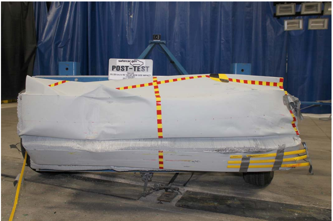
Post-Test Front View of MDB Impactor Face
