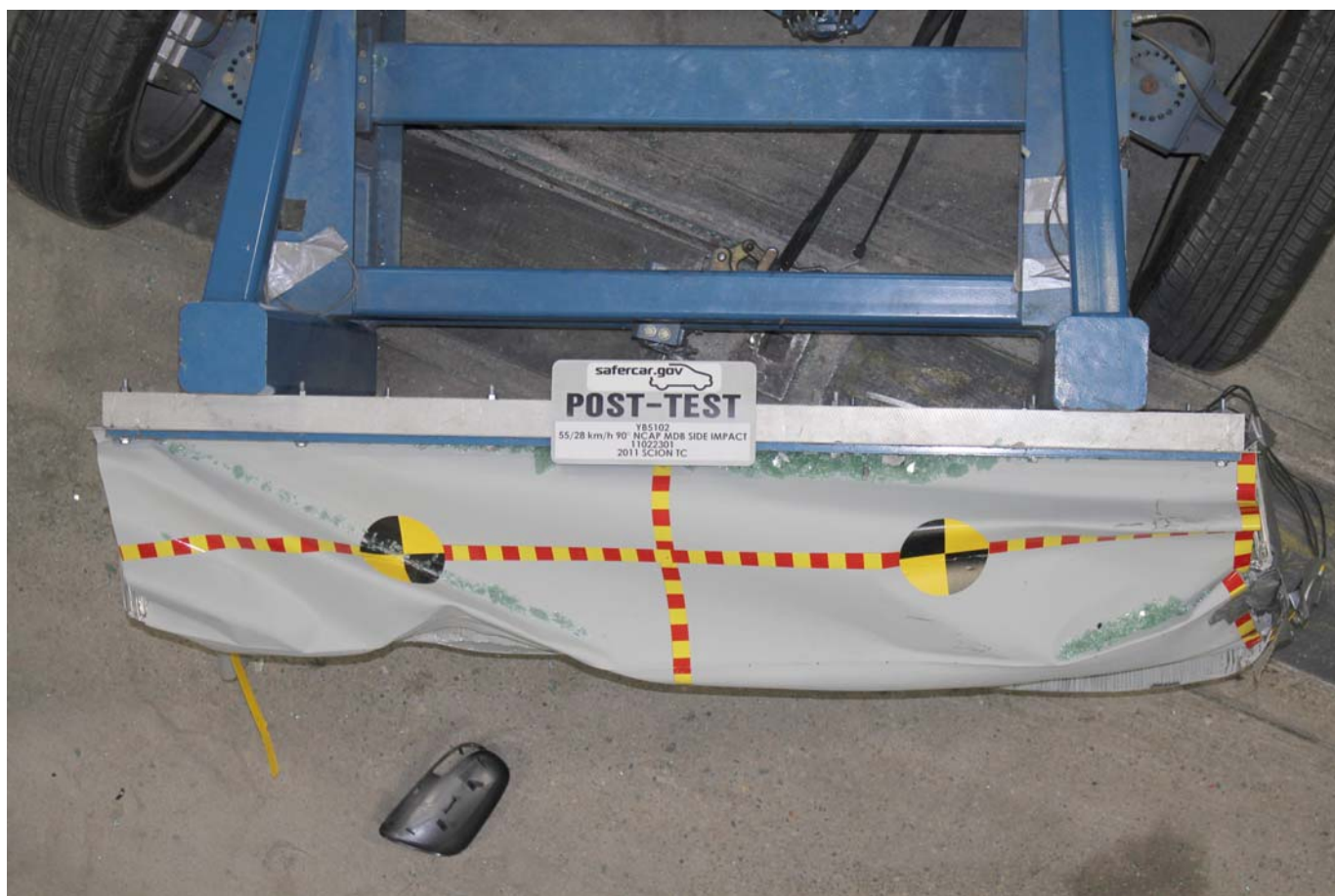
Post-Test Top View of MDB Impactor Face
