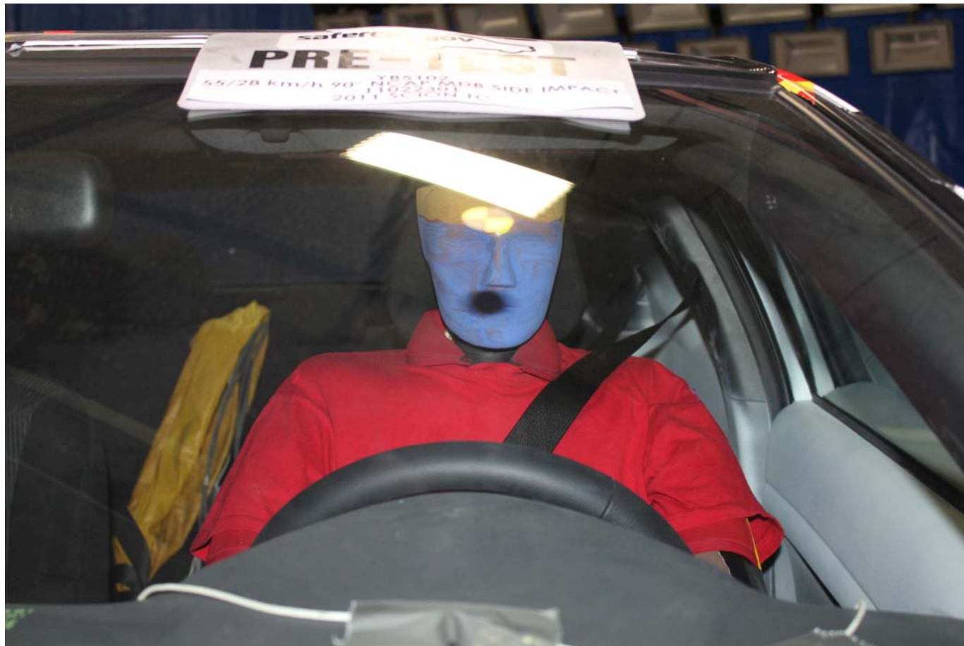
Pre-Test Front Close-Up View of Driver Dummy
