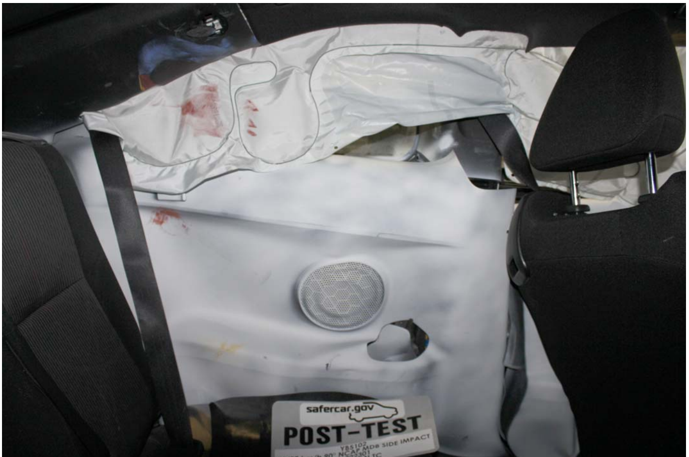
Post-Test Rear Passenger Inner Door Panel View Showing Dummy Contact Locations
