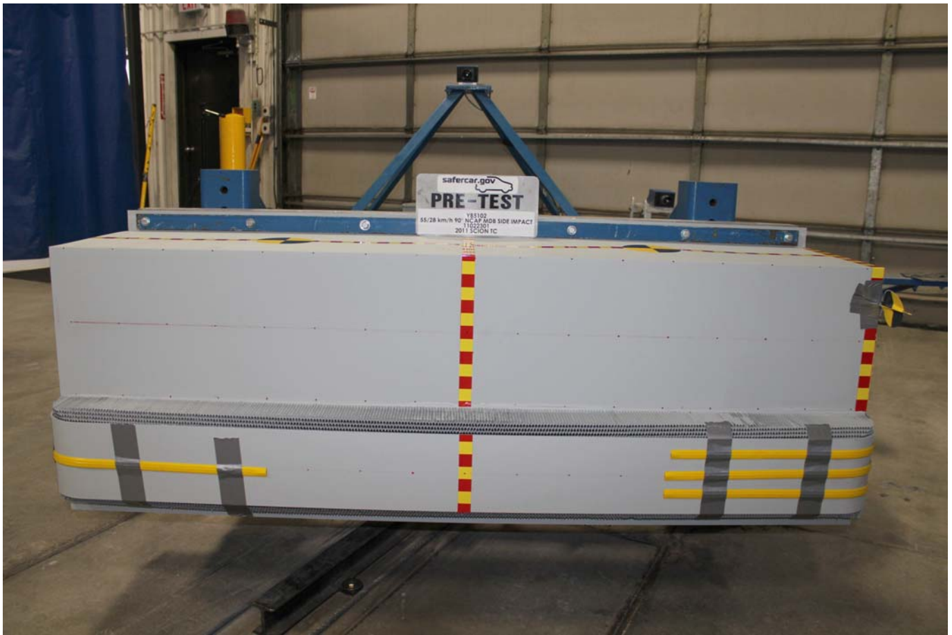
Pre-Test Front View of MDB Impactor Face
