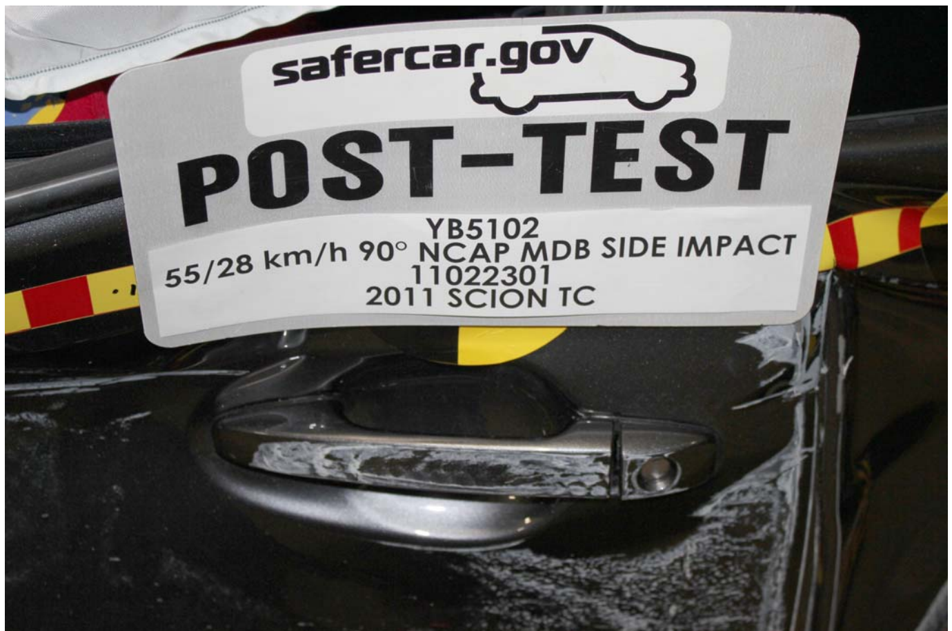
Post-Test Left Front Door Latch Close-Up
