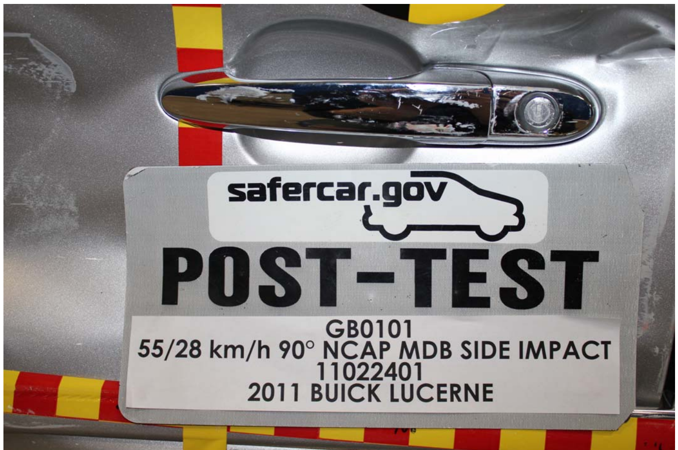
Post-Test Left Front Door Latch Close-Up
