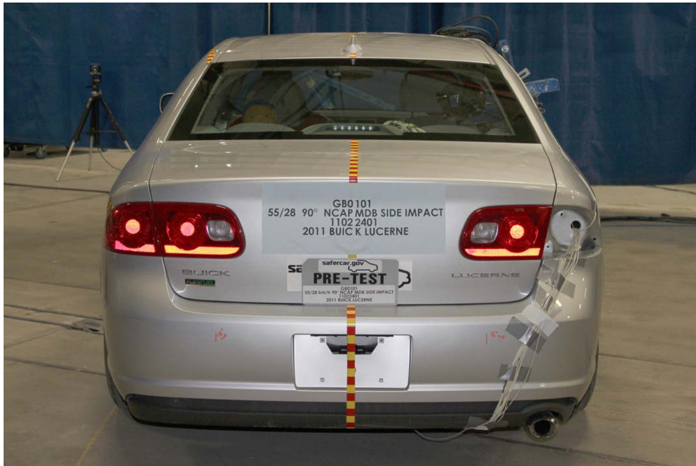
Pre-Test Rear View of Test Vehicle
