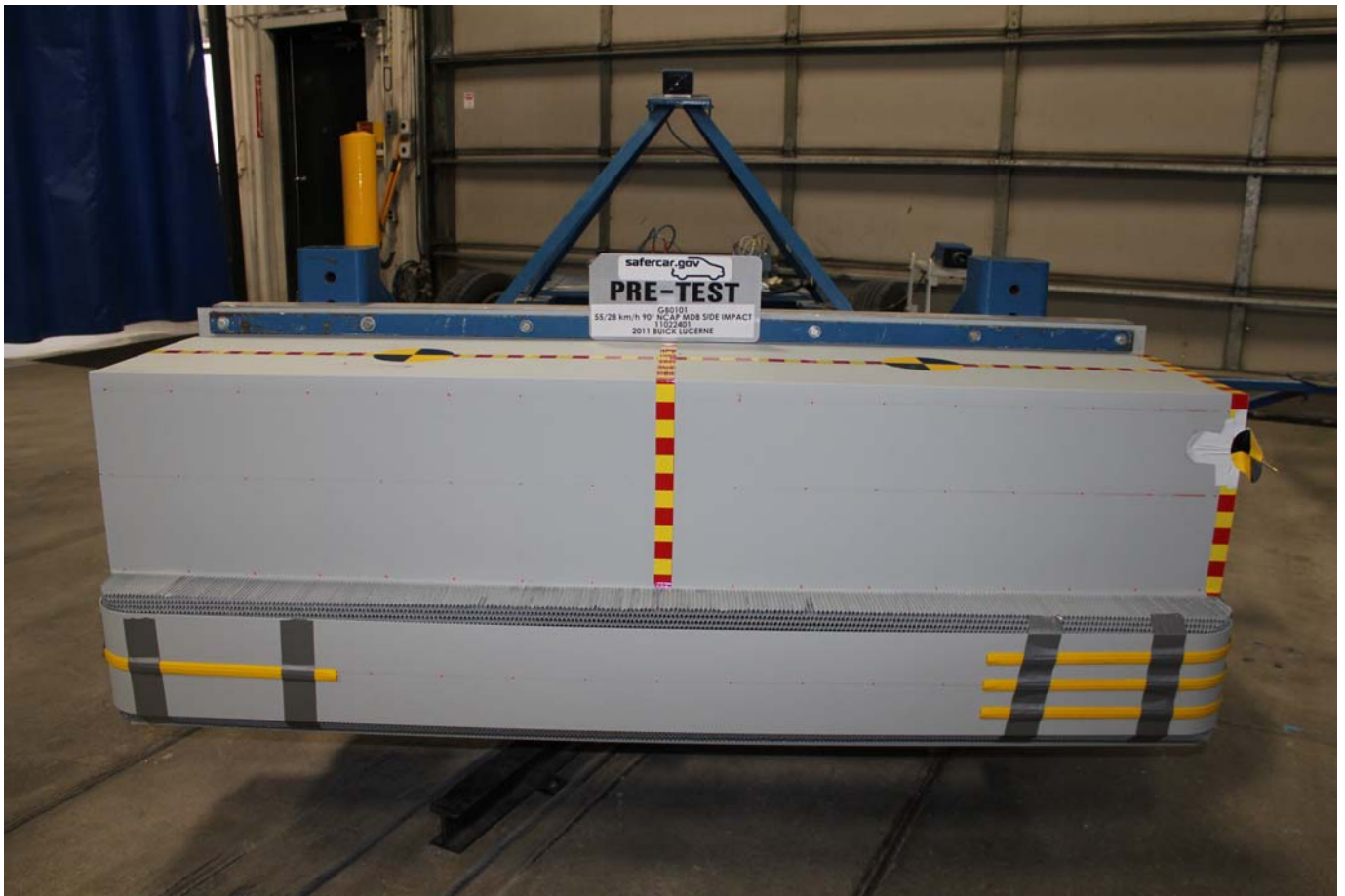
Pre-Test Front View of MDB Impactor Face
