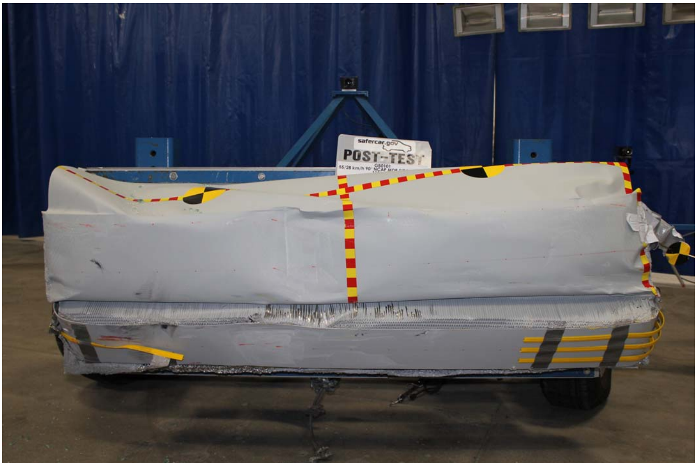
Post-Test Front View of MDB Impactor Face
