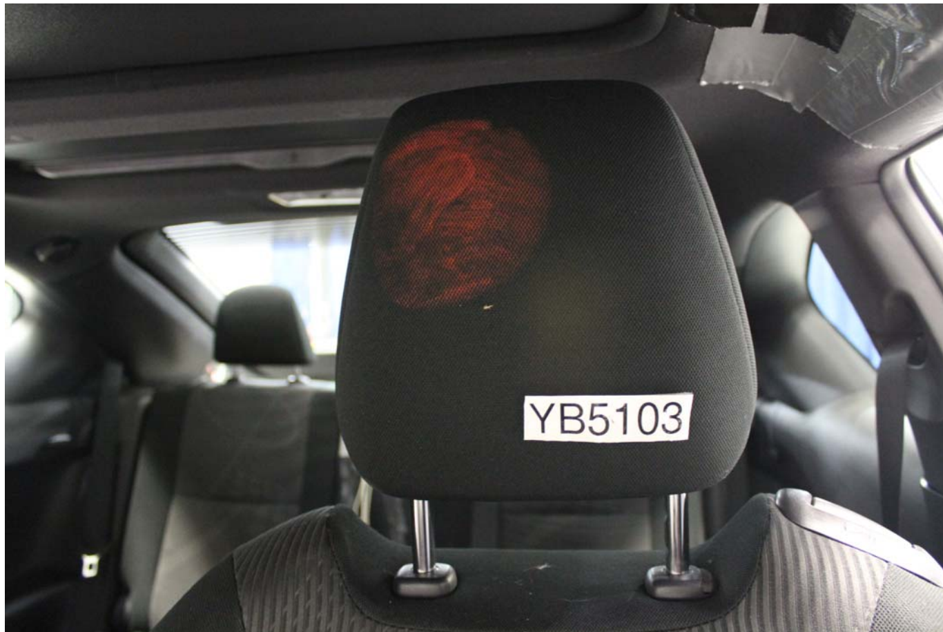
Post-Test Driver Dummy Contact with Headrest
