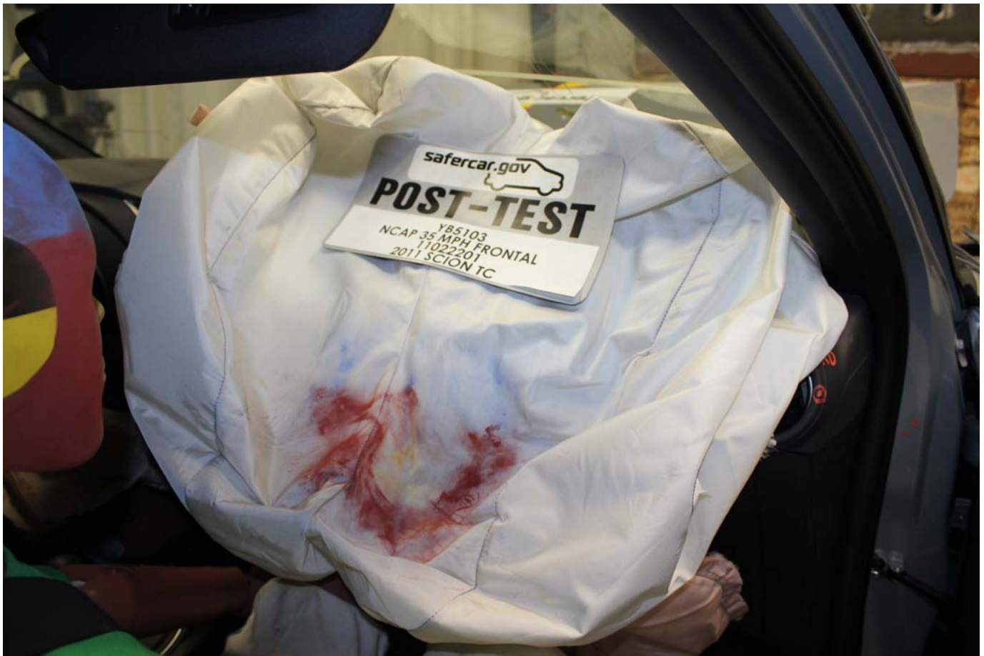
Post-Test Passenger Dummy Contact with Airbag
