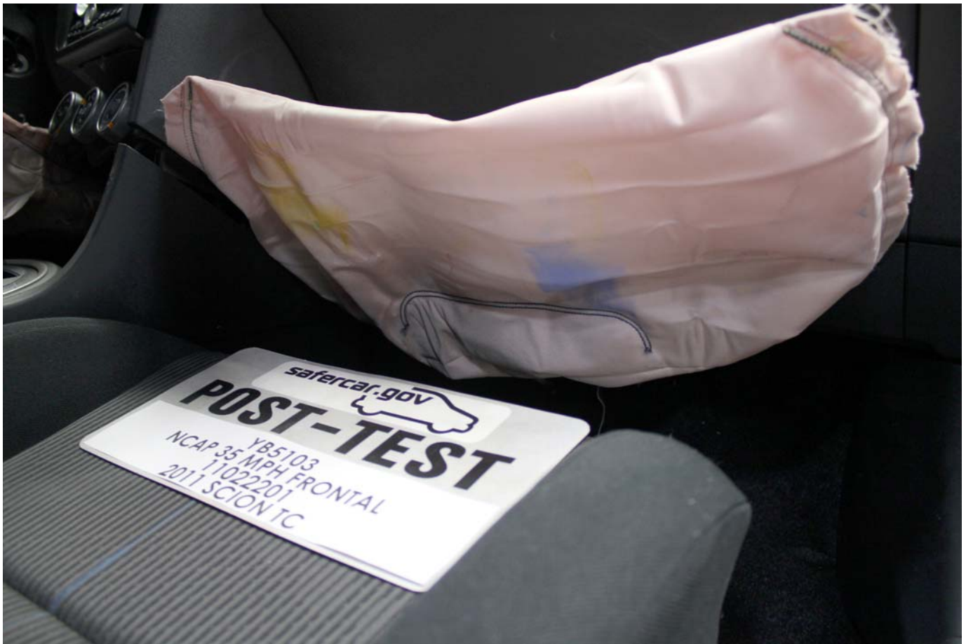
Post-Test Passenger Dummy Contact with Knee Airbag
