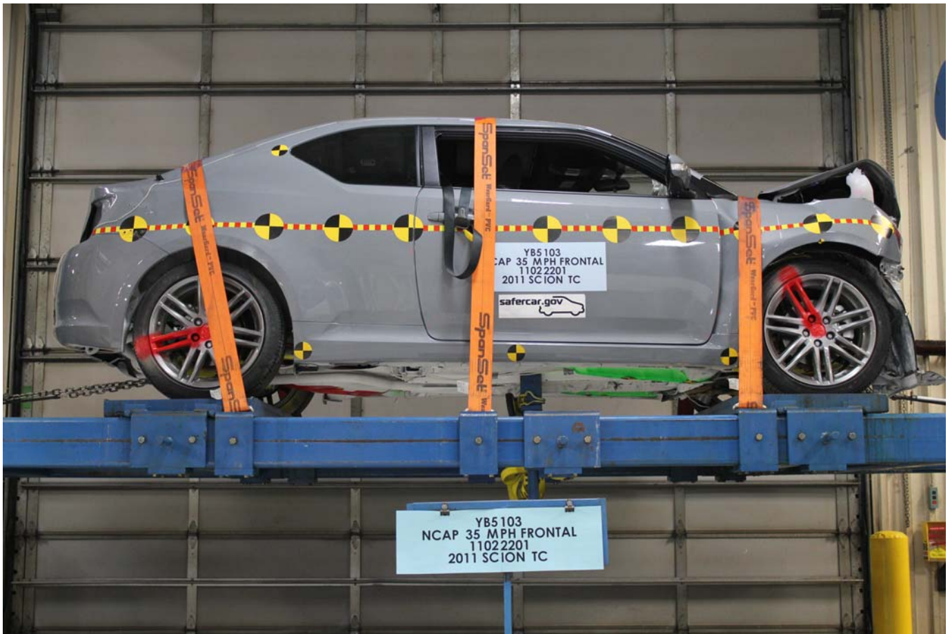
Vehicle at 360 Degrees on Static Rollover Device
