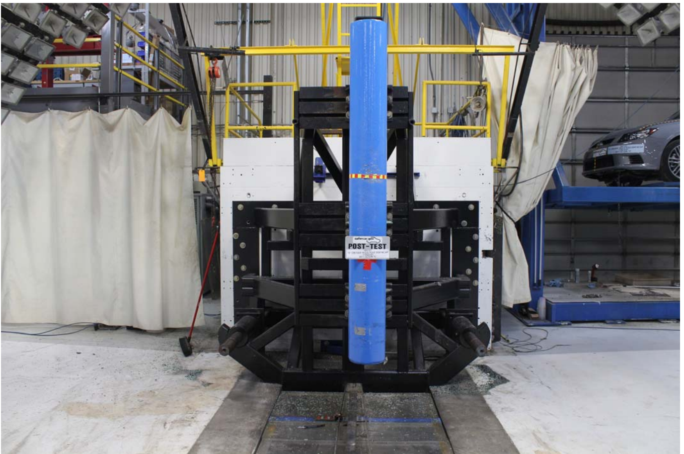
Post-Test Pole Barrier Front View
