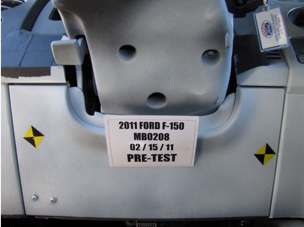
FIGURE 44. Pre-Test View of Steering Column Shear Capsule
