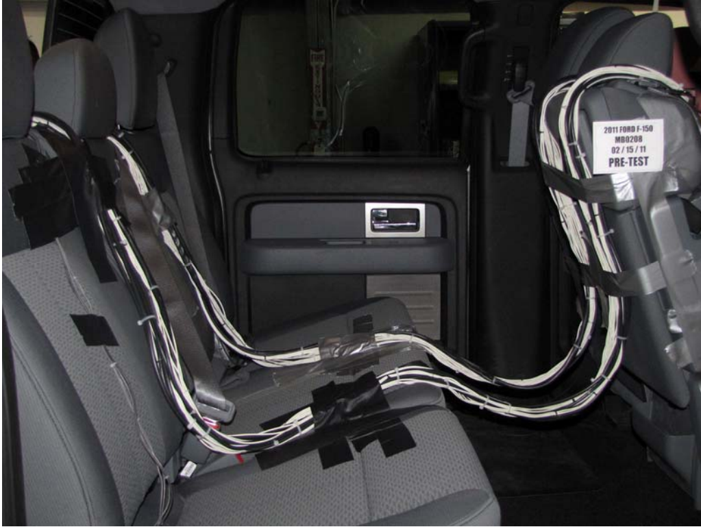
FIGURE 27. Pre-Test Dummy Cable Routing
