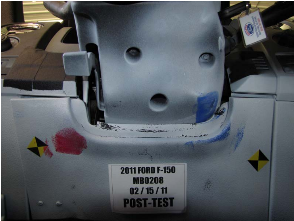
FIGURE 45. Post-Test View of Steering Column Shear Capsule
