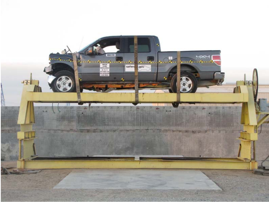
FIGURE 68. Vehicle at 360° on Static Rollover Device
