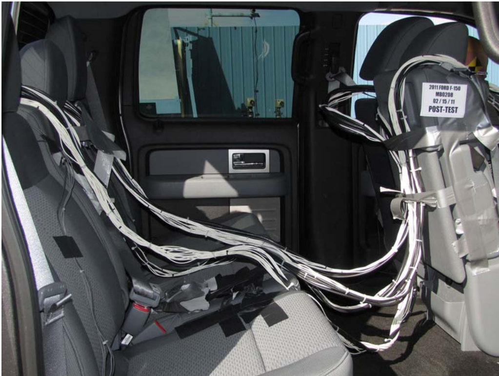
FIGURE 28. Post-Test Dummy Cable Routing
