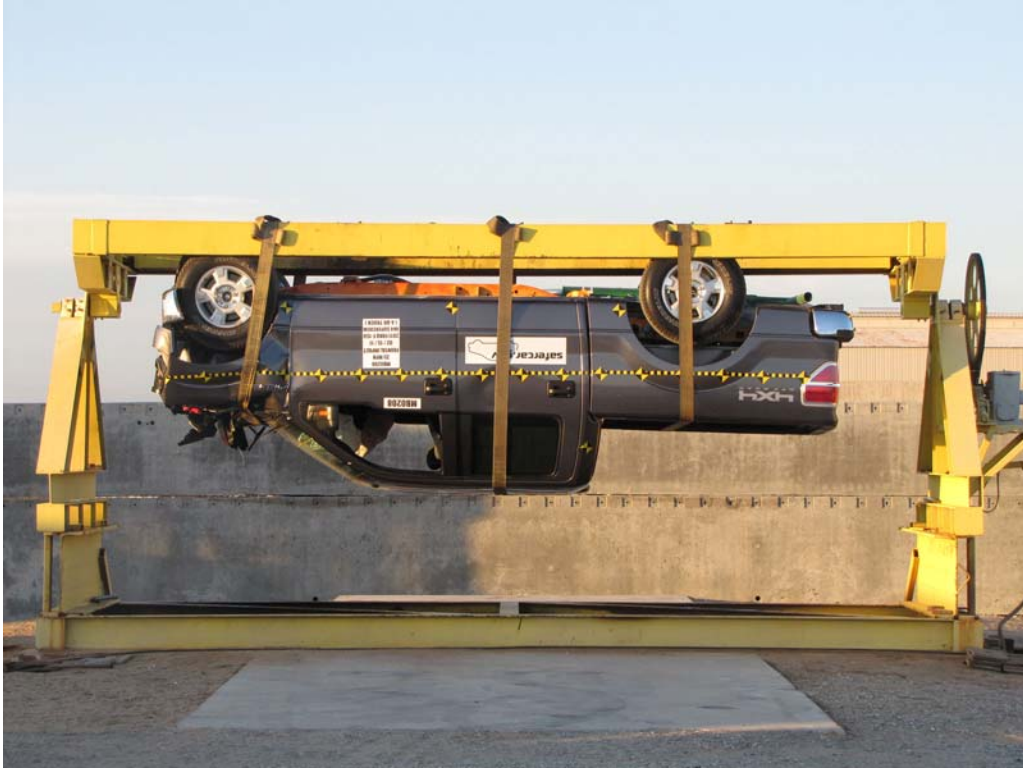
FIGURE 66. Vehicle at 180°on Static Rollover Device
