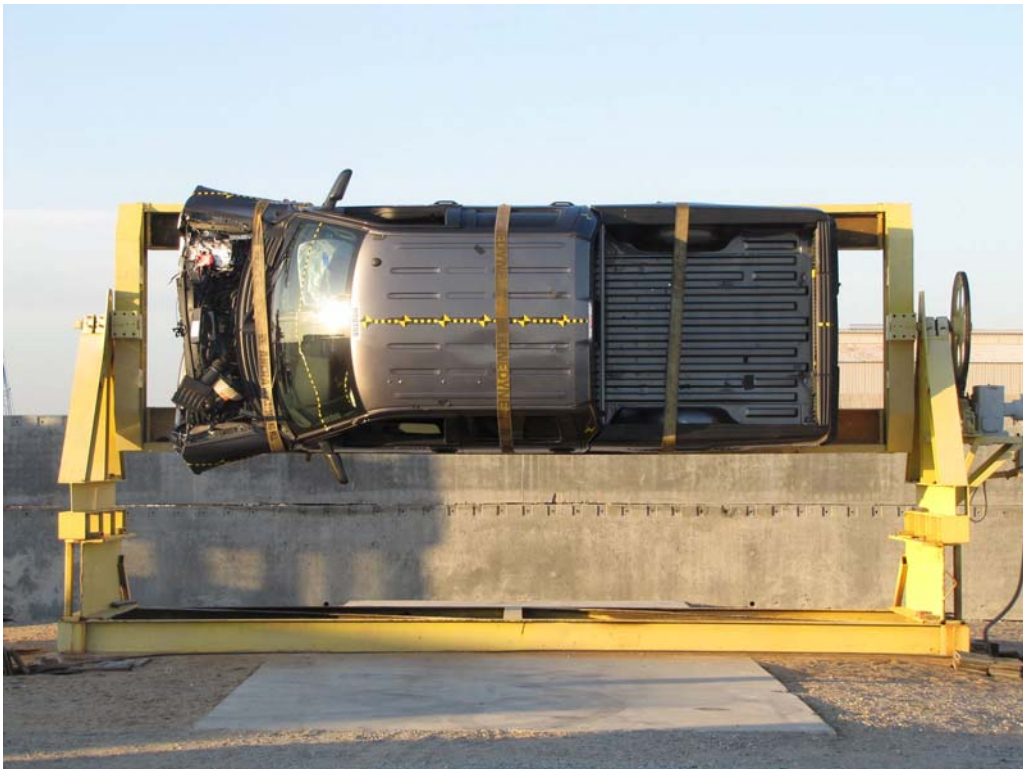
FIGURE 65. Vehicle at 90°on Static Rollover Device
