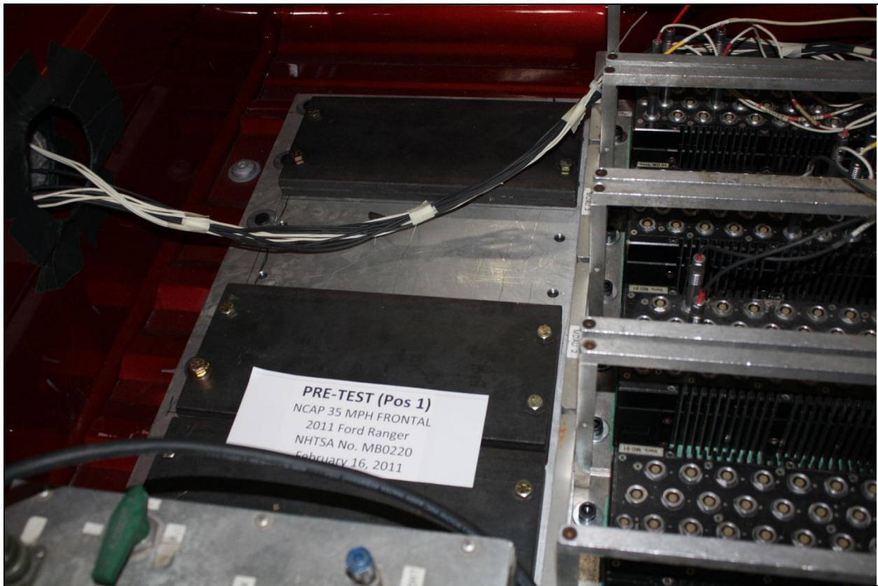
Figure A-61: Photograph of Ballast Installed Vehicle
