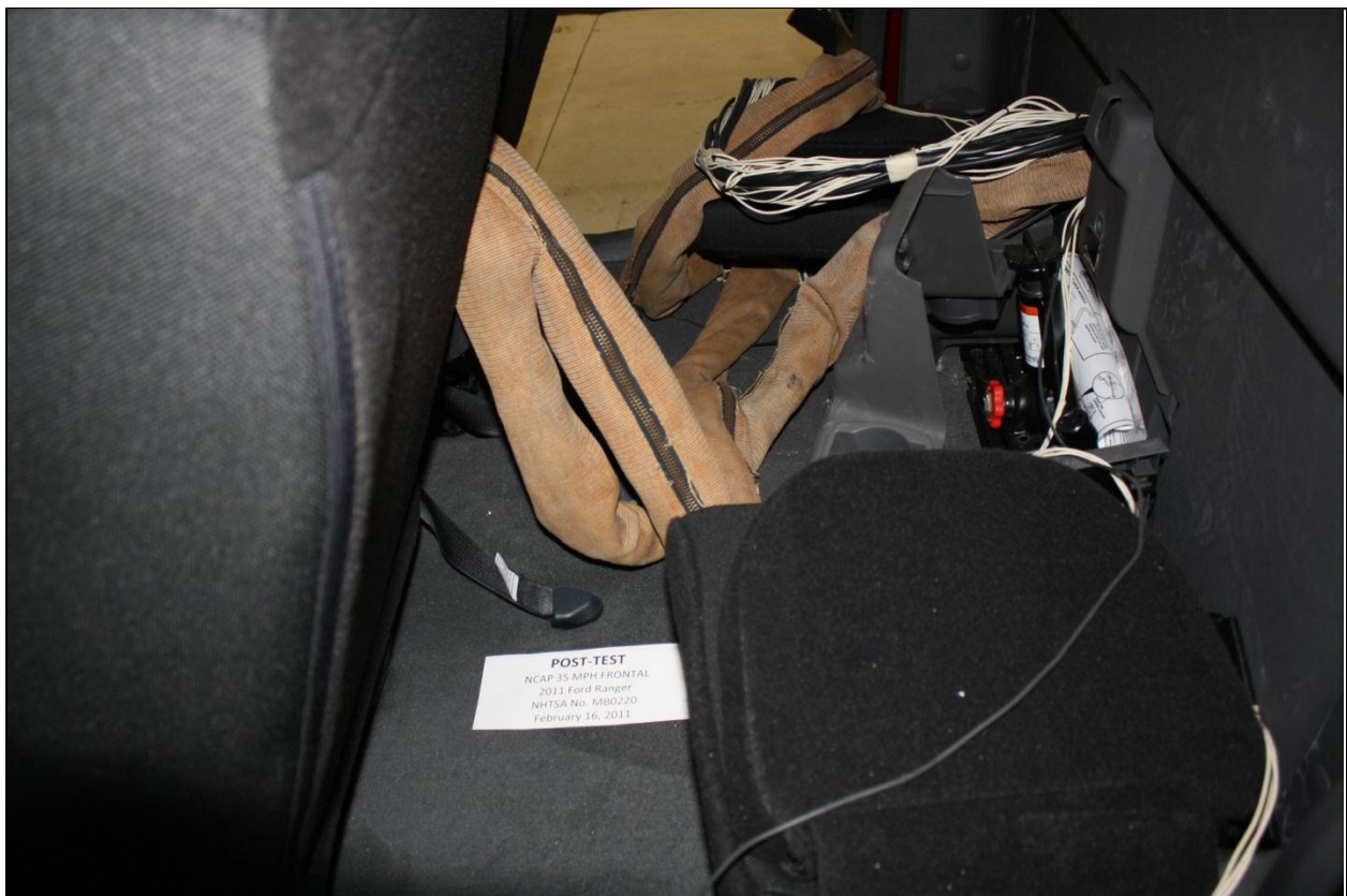
Figure A-28: Post-Test Dummy Cable Routing
