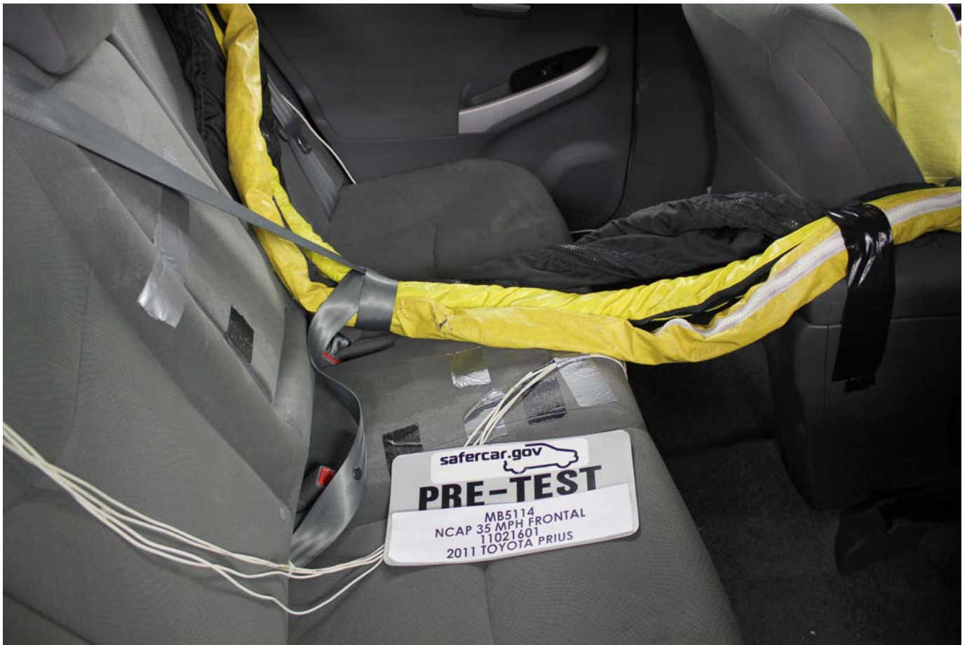
Pre-Test Dummy Cable Routing
