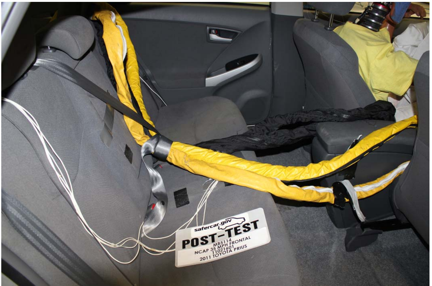
Post-Test Dummy Cable Routing
