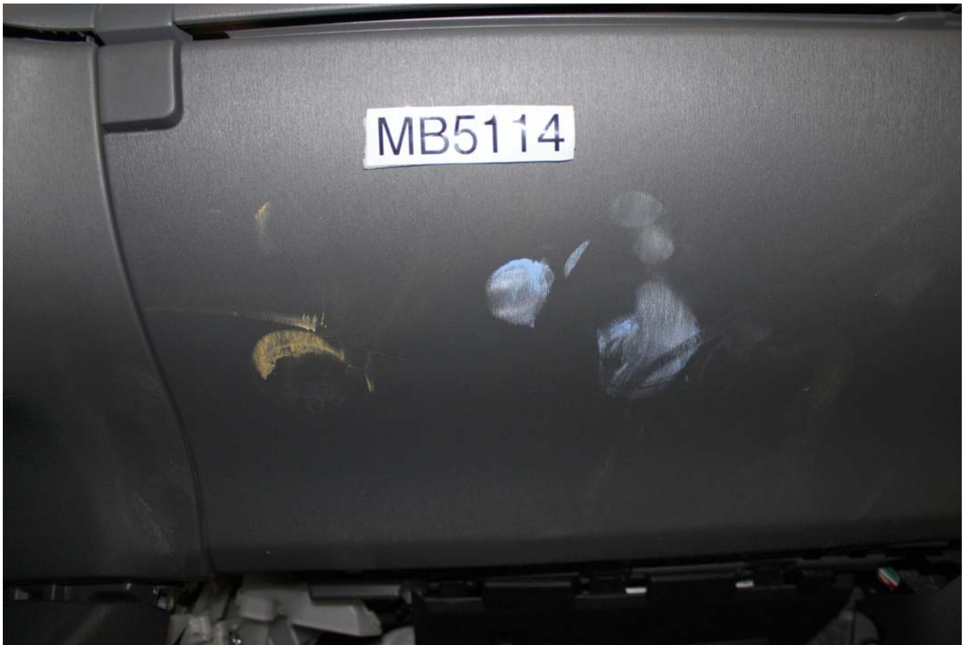
Post-Test Passenger Dummy Contact with Glovebox
