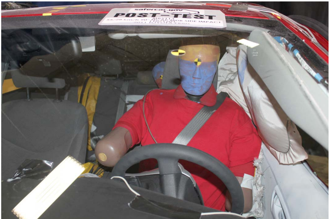
Post-Test Front Close-Up View of Driver Dummy
