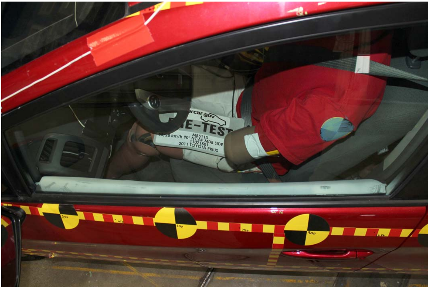
Pre-Test Driver Dummy and Door Clearance View
