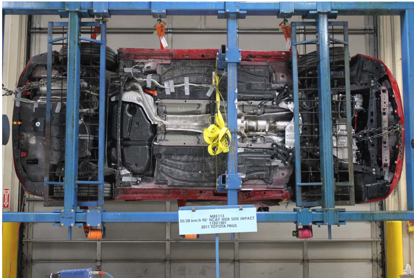
FMVSS No. 301/305 Rollover 90 Degrees
