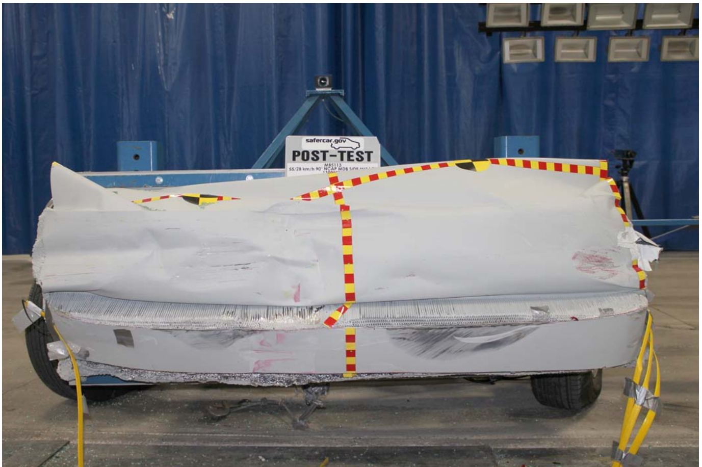
Post-Test Front View of MDB Impactor Face
