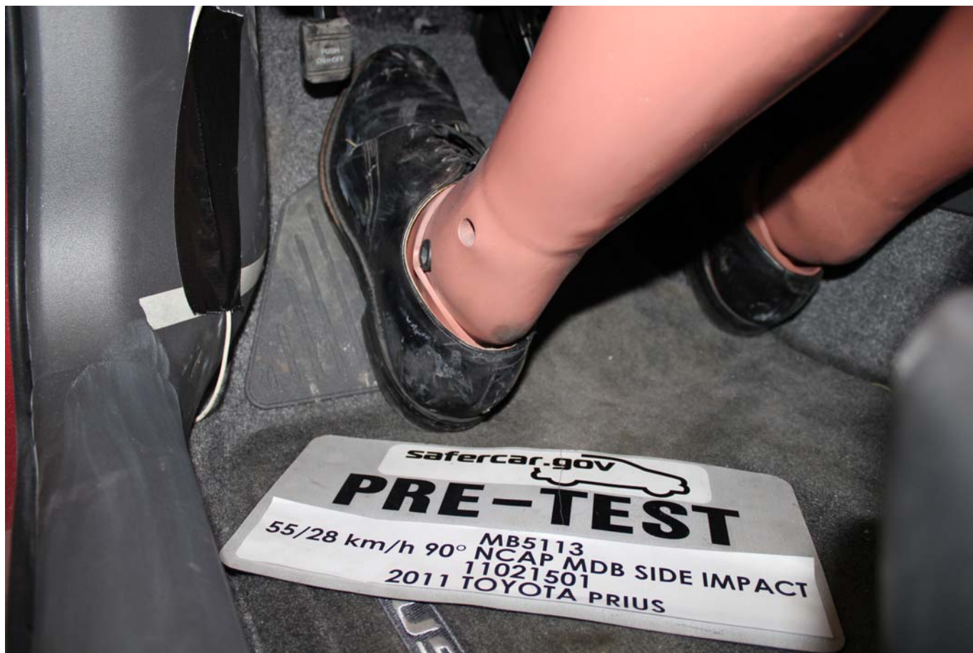
Pre-Test Placement of Driver Dummy's Feet
