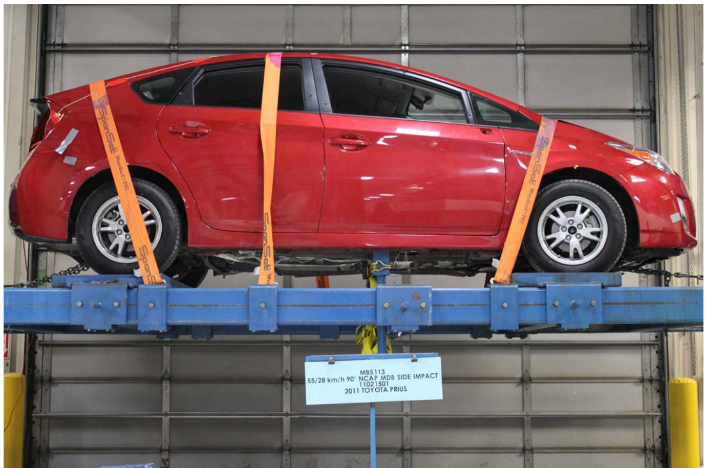
FMVSS No. 301/305 Rollover 0 Degrees
