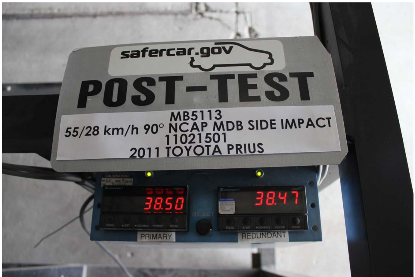
Post-Test Primary and Redundant Speed Trap Read-Out
