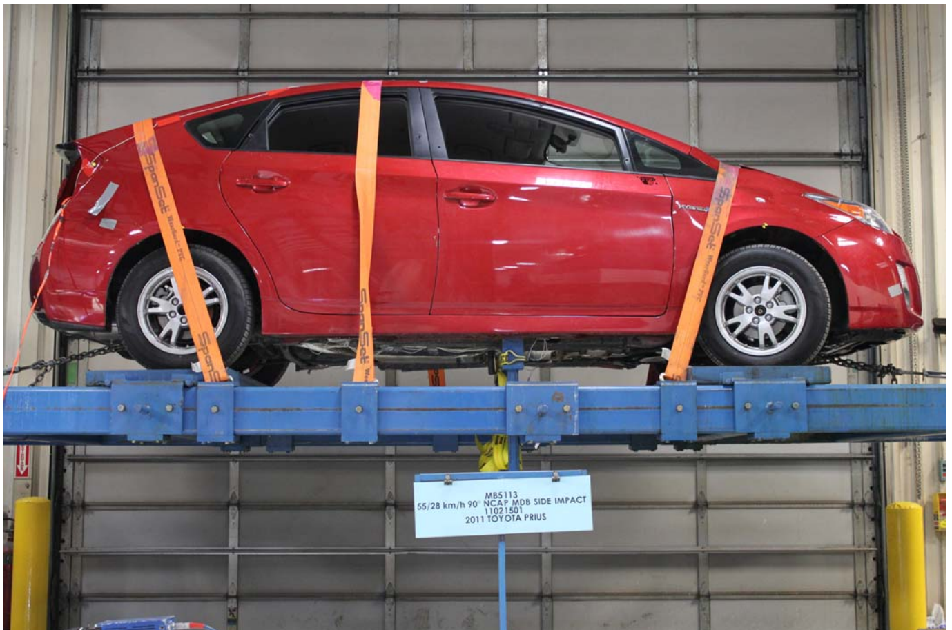
FMVSS No. 301/305 Rollover 360 Degrees
