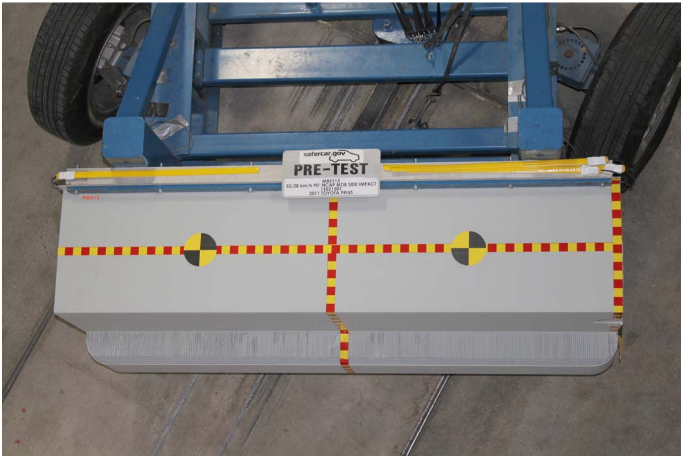
Pre-Test Top View of MDB Impactor Face
