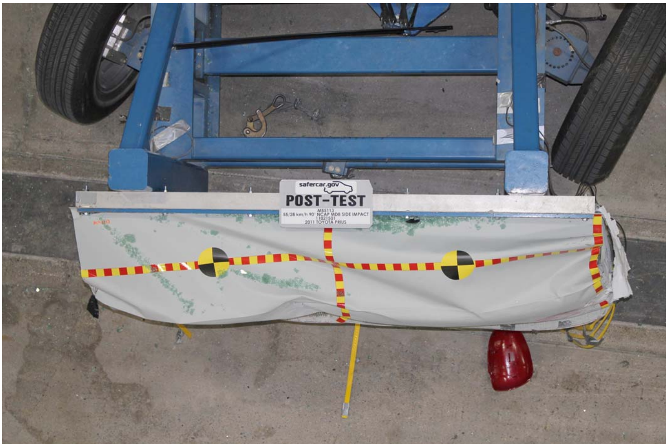
Post-Test Top View of MDB Impactor Face
