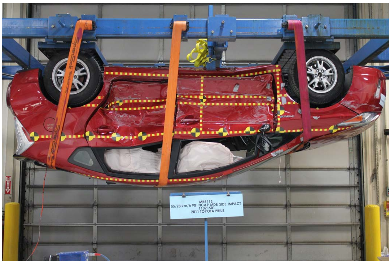
FMVSS No. 301/305 Rollover 180 Degrees
