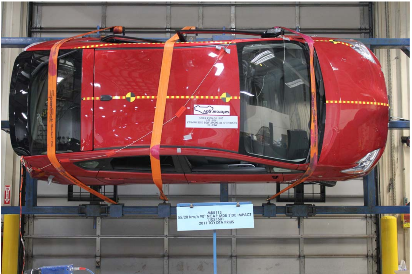
FMVSS No. 301/305 Rollover 270 Degrees
