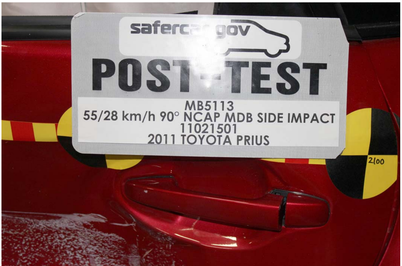
Post-Test Left Rear Door Latch Close-Up
