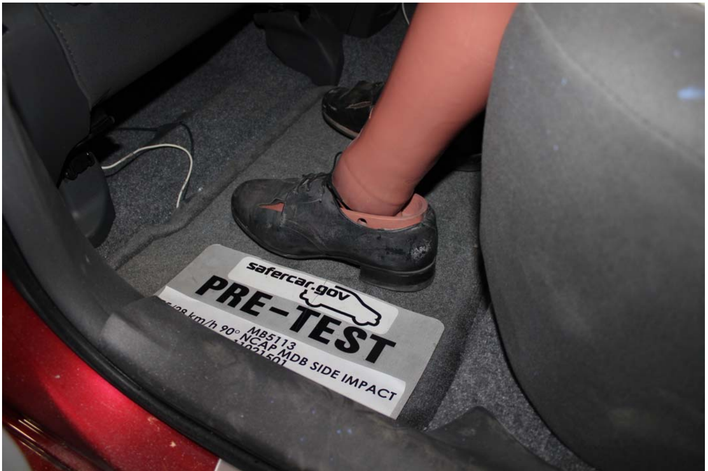
Pre-Test Placement of Rear Passenger Dummy's Feet
