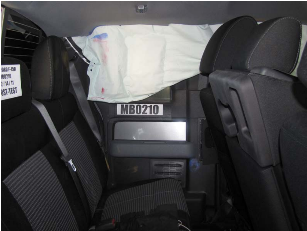
FIGURE 72. Post-Test Rear Passenger Inner Door Panel View Showing Rear Passenger Dummy Contact Locations
