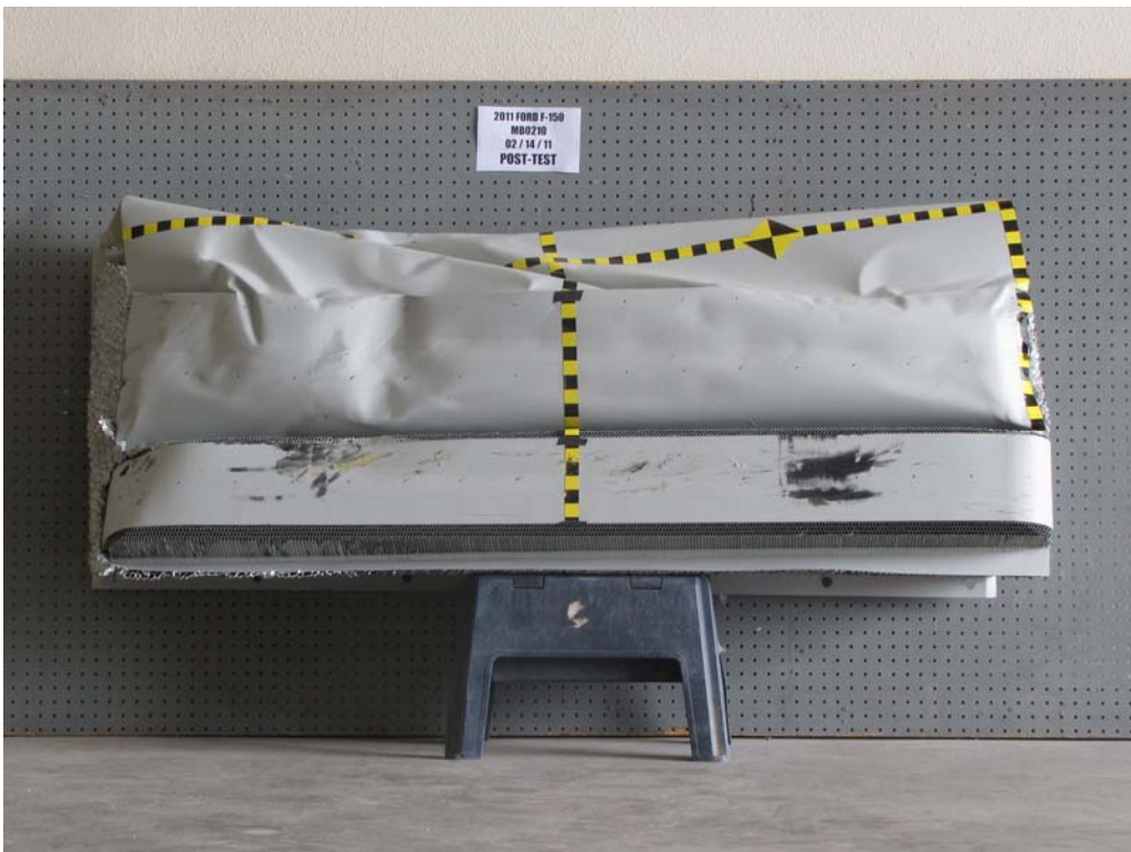
FIGURE 82. Post-Test Front View of MDB Impactor Face
