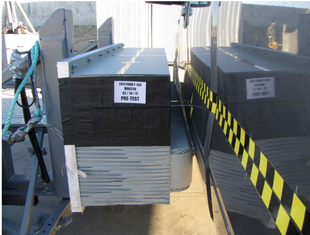
FIGURE 18. Pre-Test Right Side View of MDB Positioned Against Side of Test Vehicle at Ideal Impact Point
