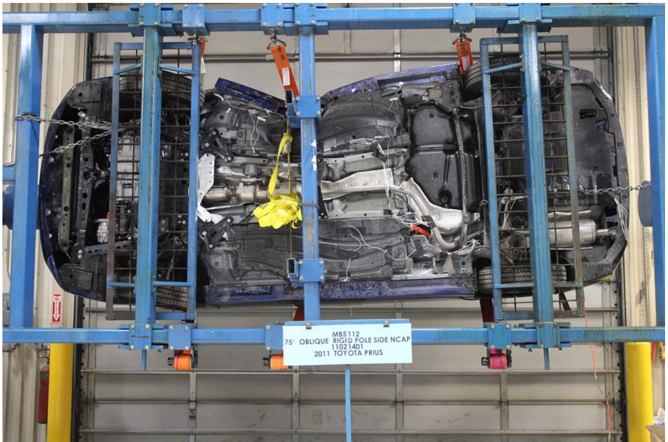
FMVSS No. 301/305 Rollover 270 Degrees
