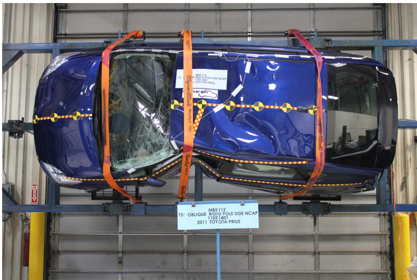
FMVSS No. 301/305 Rollover 90 Degrees
