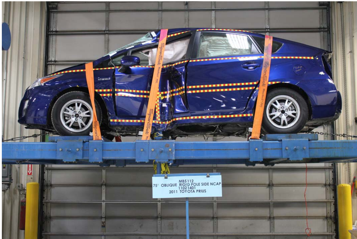
FMVSS No. 301/305 Rollover 0 Degrees
