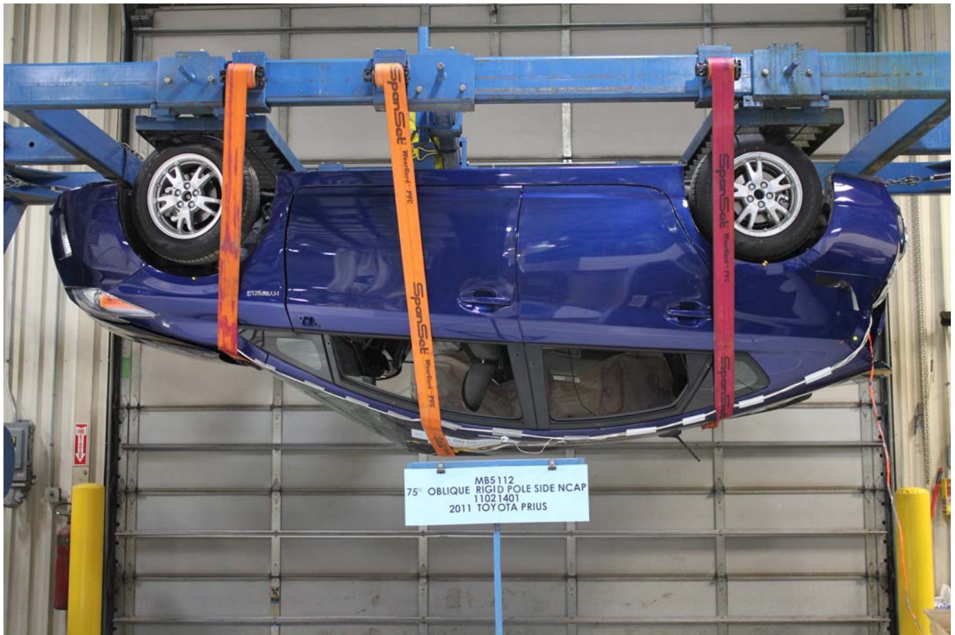
FMVSS No. 301/305 Rollover 180 Degrees
