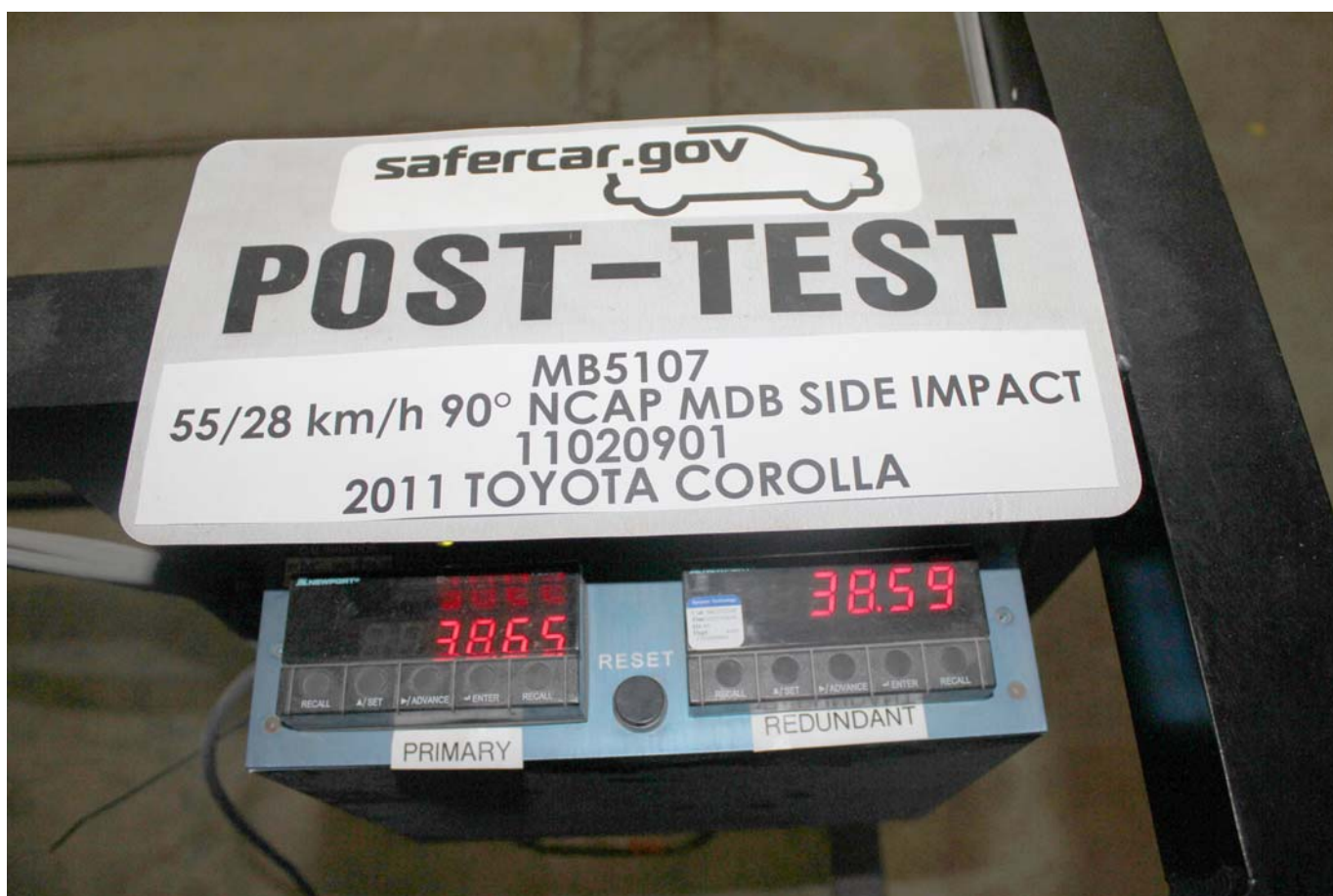
Post-Test Primary and Redundant Speed Trap Read-Out
