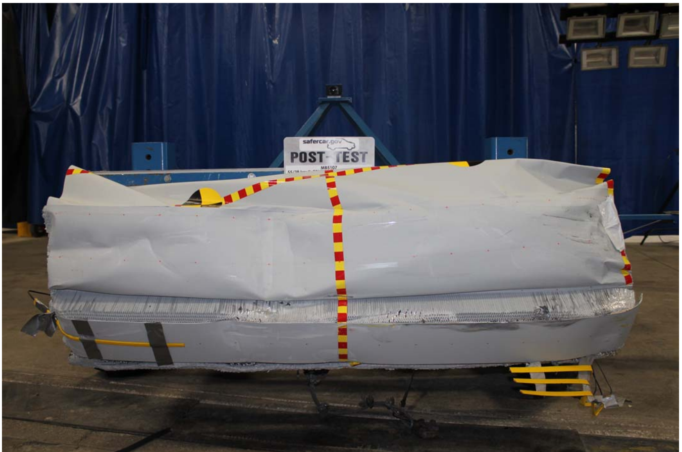
Post-Test Front View of MDB Impactor Face
