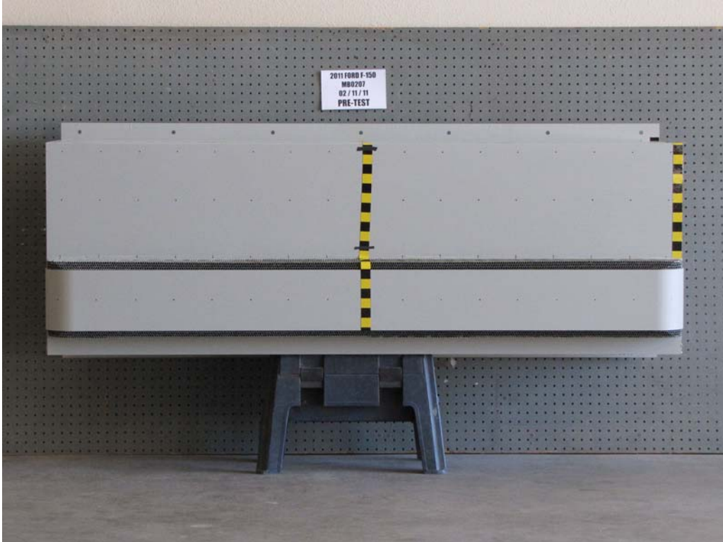
FIGURE 81. Pre-Test Front View of MDB Impactor Face
