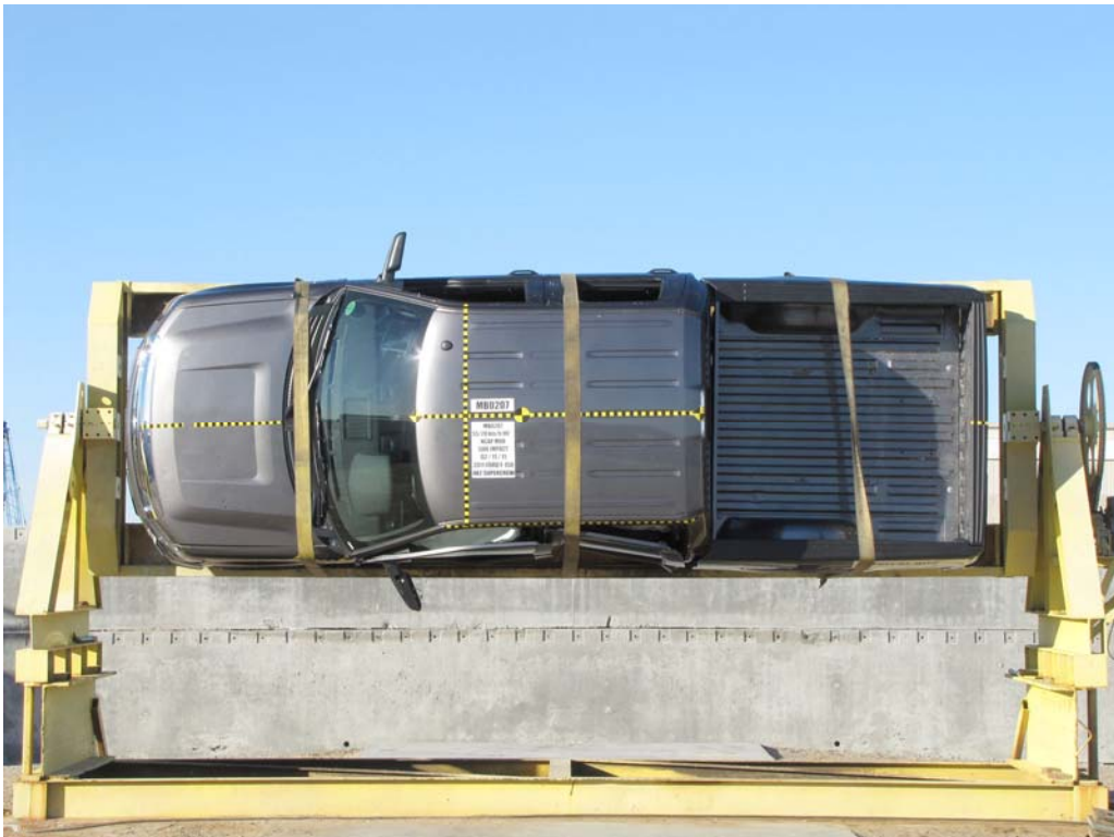
FIGURE 94. FMVSS No. 301/305 Rollover 90 Degrees
