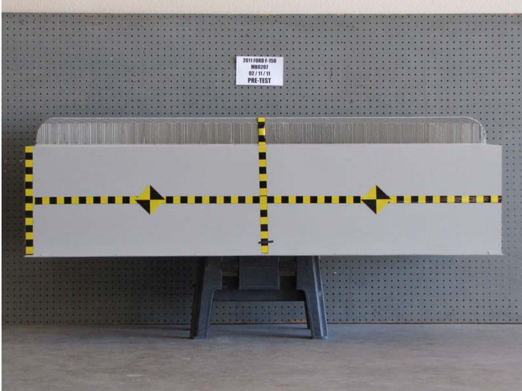
FIGURE 83. Pre-Test Top View of MDB Impactor Face
