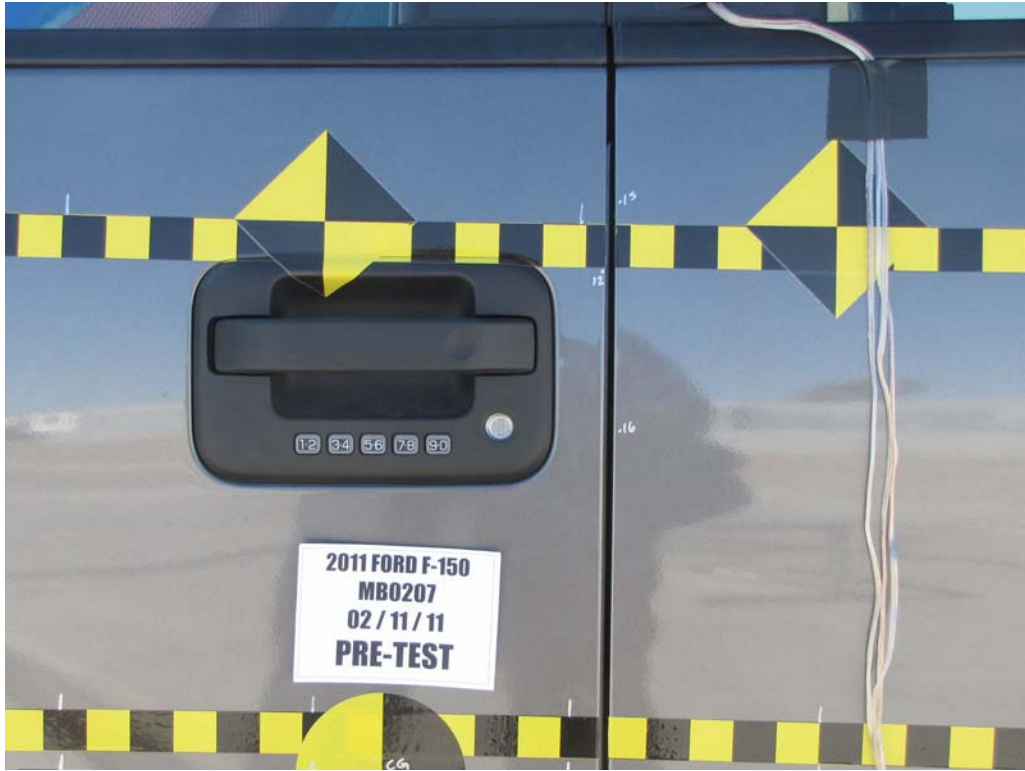
FIGURE 21. Pre-Test Left Front Door Latch Close-Up
