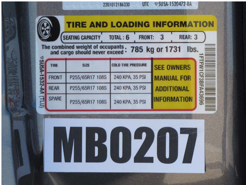
FIGURE 90. Close-Up View of Vehicle's Tire Information Placard
