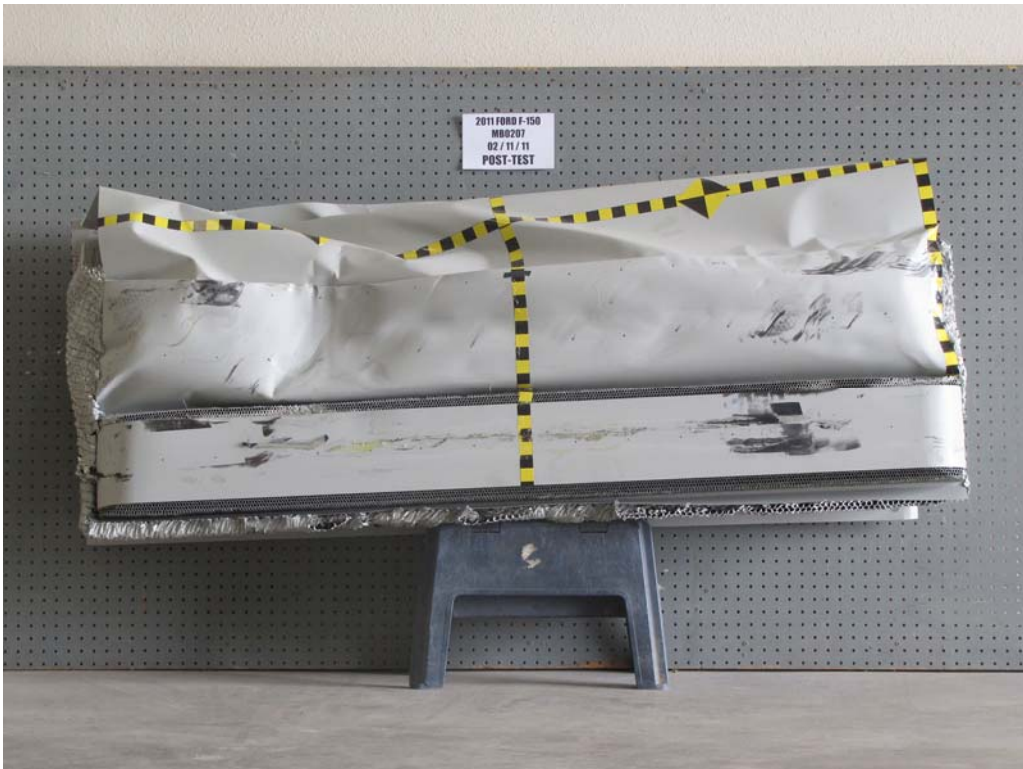
FIGURE 82. Post-Test Front View of MDB Impactor Face
