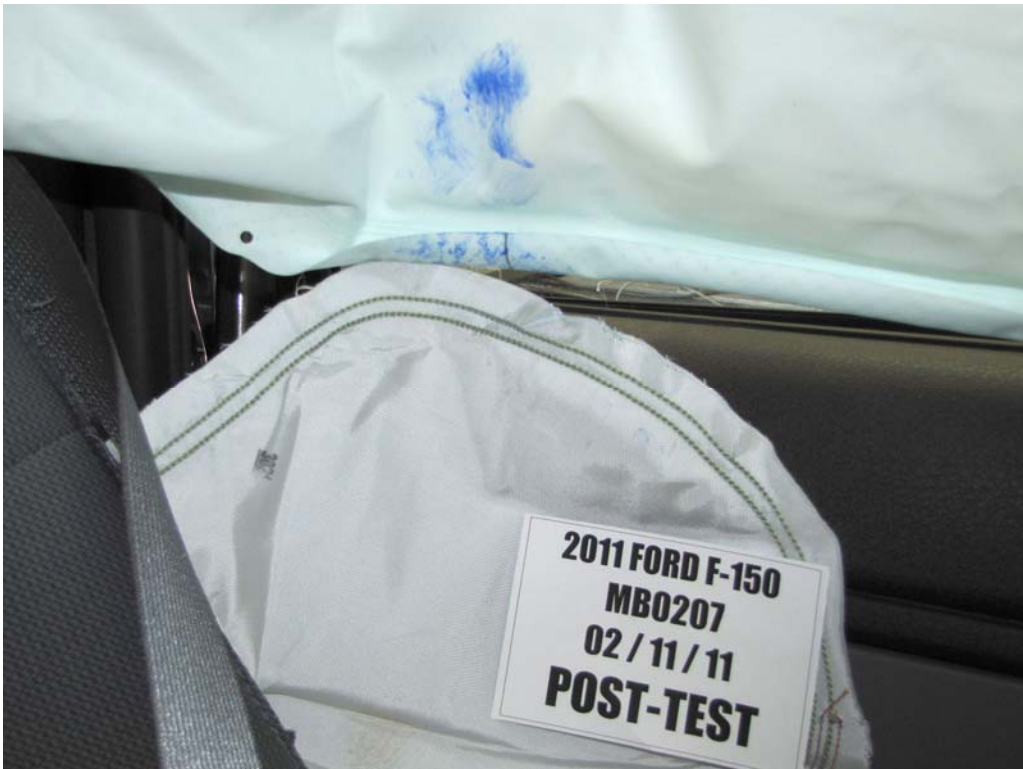
FIGURE 50. Post-Test Driver Dummy Close-Up Torso Contact with Side Airbag View
