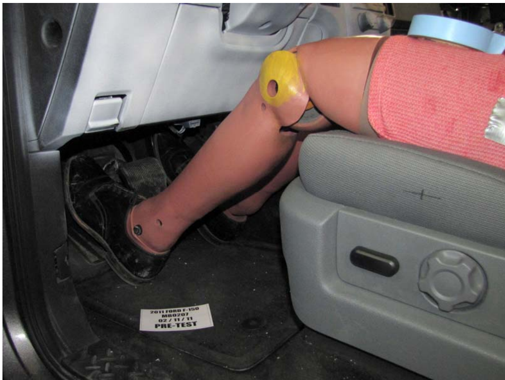
FIGURE 34. Pre-Test Placement of Driver Dummy's Feet
