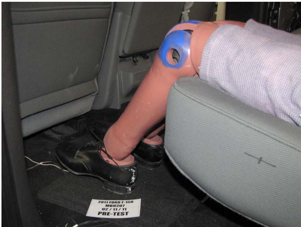
FIGURE 62. Pre-Test Placement of Rear Passenger Dummy's Feet
