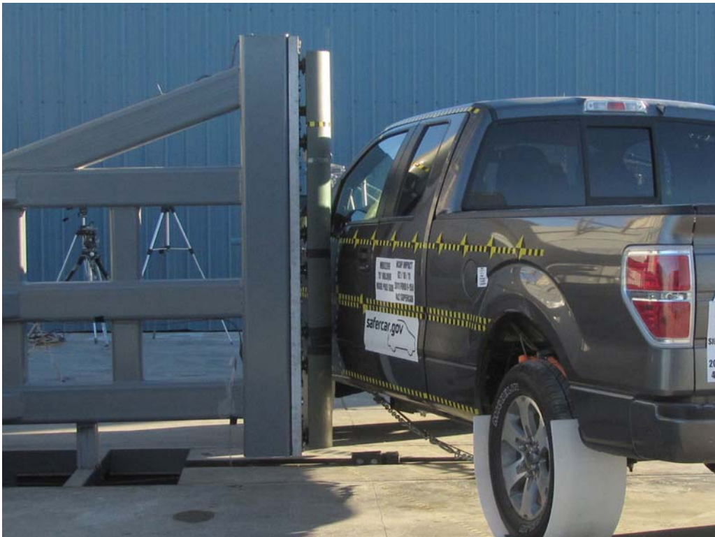
FIGURE 18. Pre-Test Right Side View of Pole Positioned Against Side of Vehicle at Ideal Impact Point
