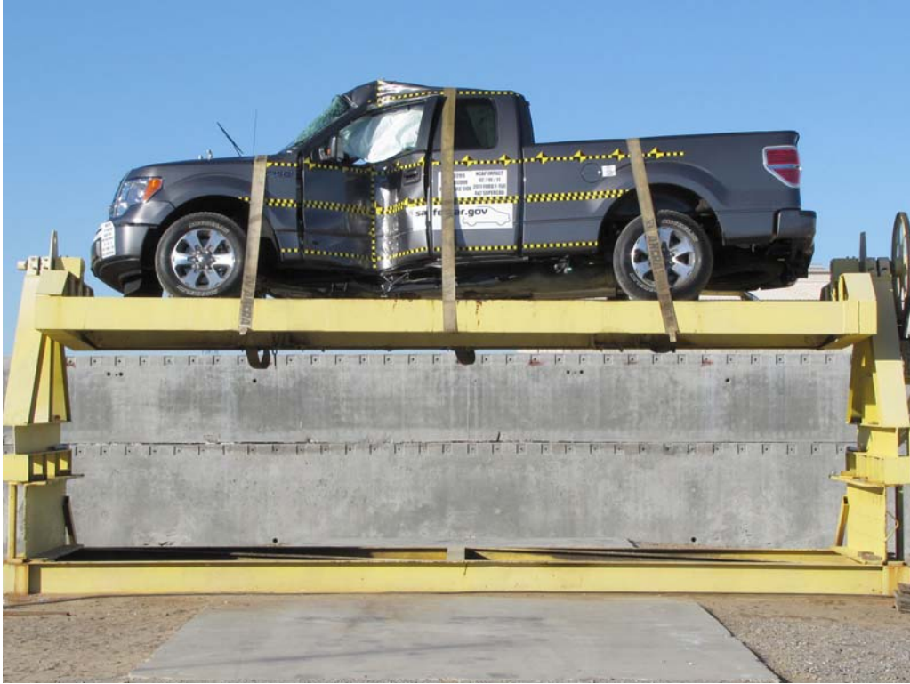
FIGURE 61. FMVSS No. 301-305 Rollover 0 Degrees
