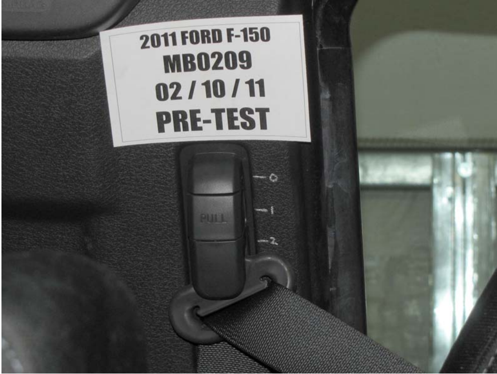
FIGURE 33. Pre-Test View of Belt Anchorage for Dummy
