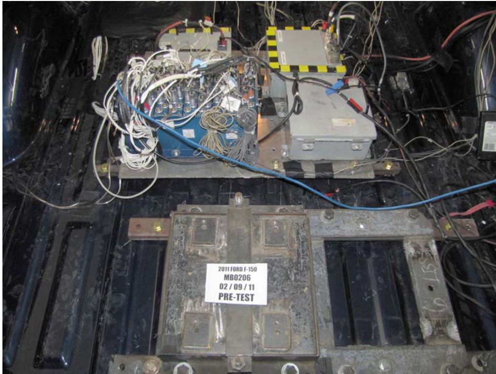
FIGURE 59. Pre-Test Ballast View
