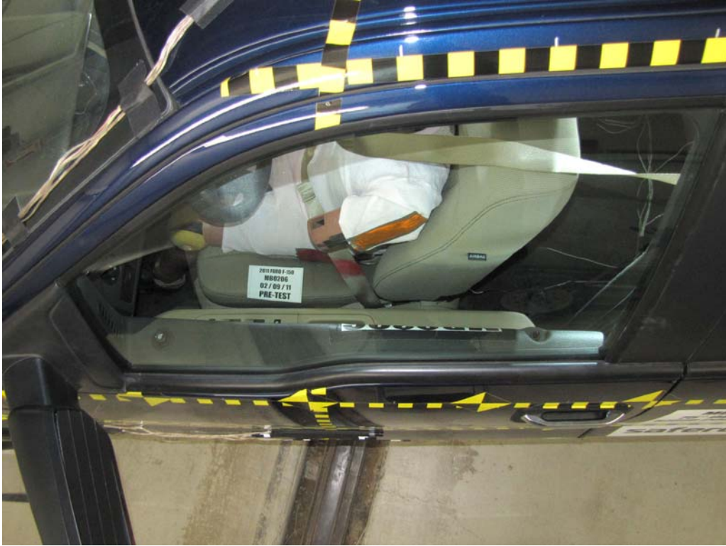
FIGURE 39. Pre-Test Driver Dummy and Door Clearance
