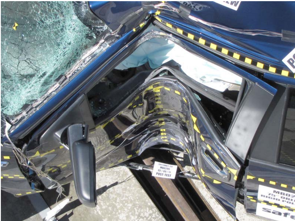
FIGURE 40. Post-Test Driver Dummy and Door Clearance
