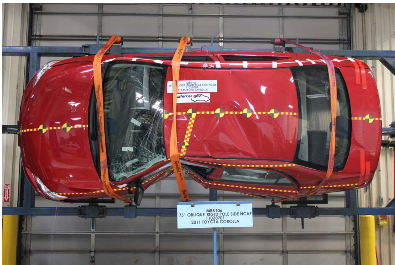
FMVSS No. 301/305 Rollover 90 Degrees
