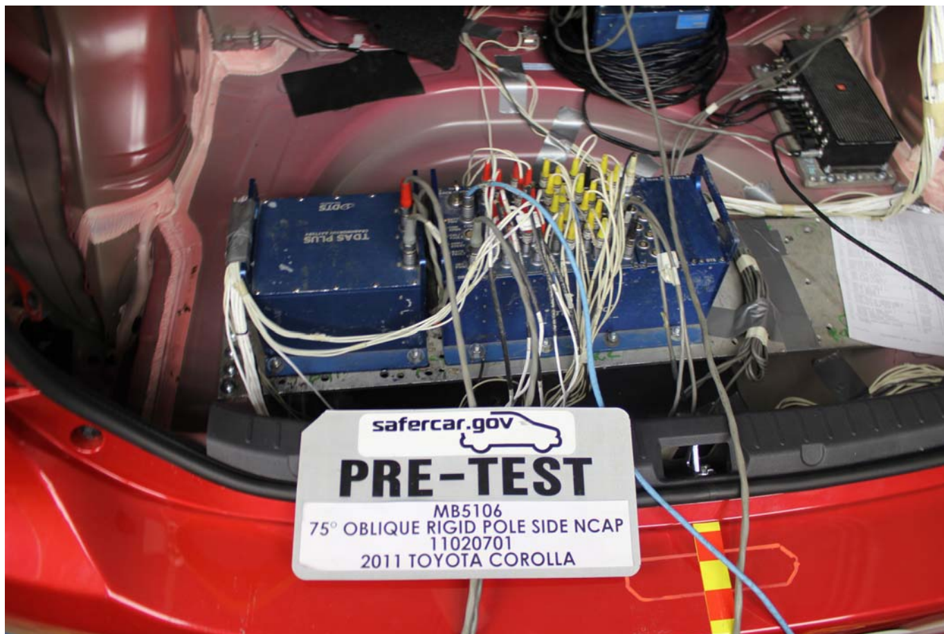
Pre-Test Ballast View
