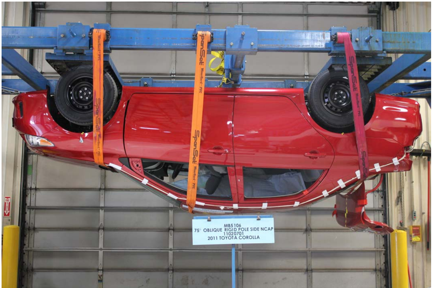
FMVSS No. 301/305 Rollover 180 Degrees
