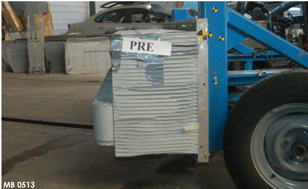
Figure A-85: Pre-Test Left Side View of MDB Impactor Face
