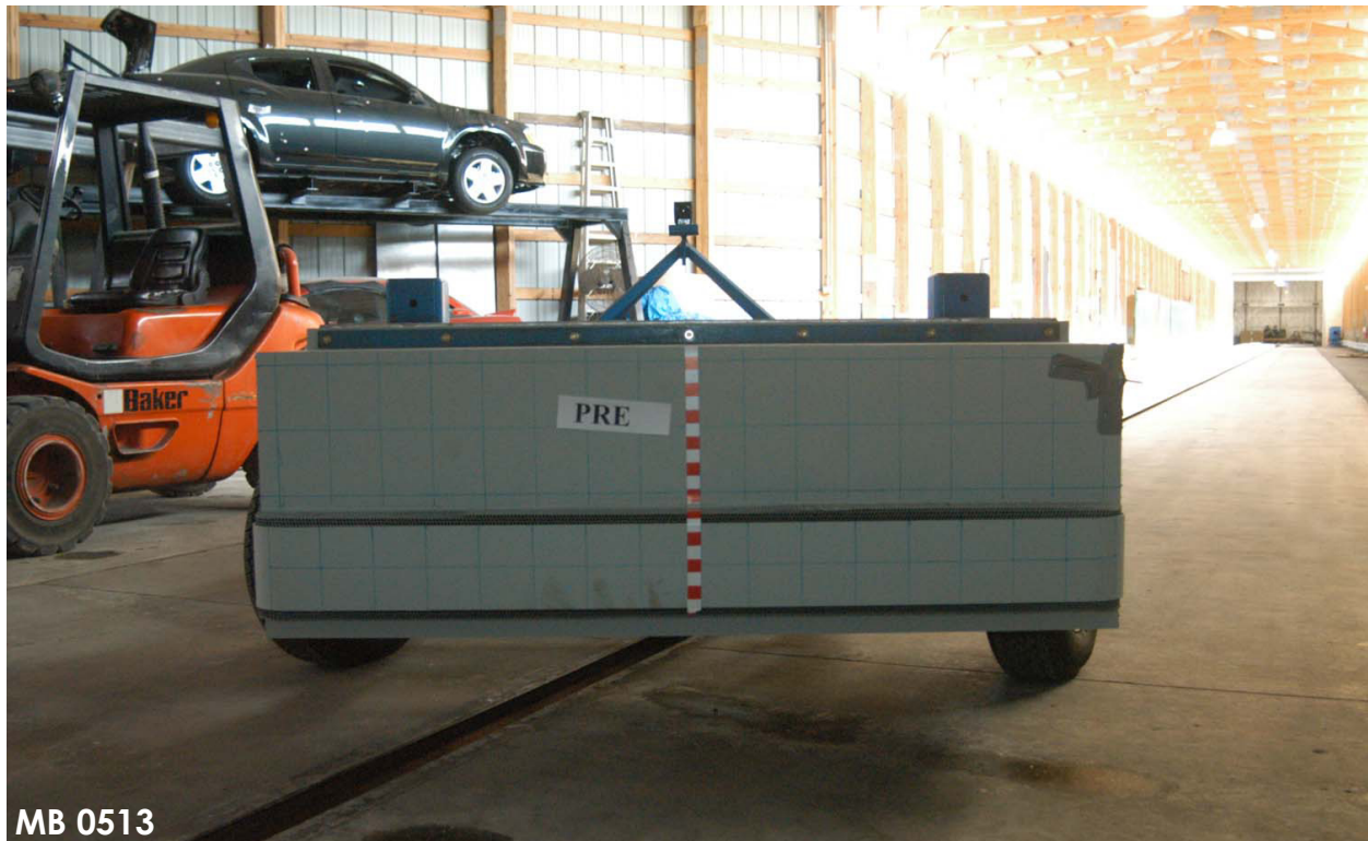
Figure A-81: Pre-Test Front View of MDB Impactor Face
