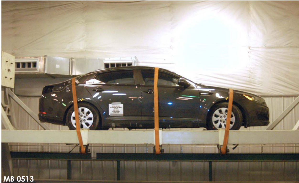
Figure A-97: FMVSS No. 301/305 Rollover 360°
