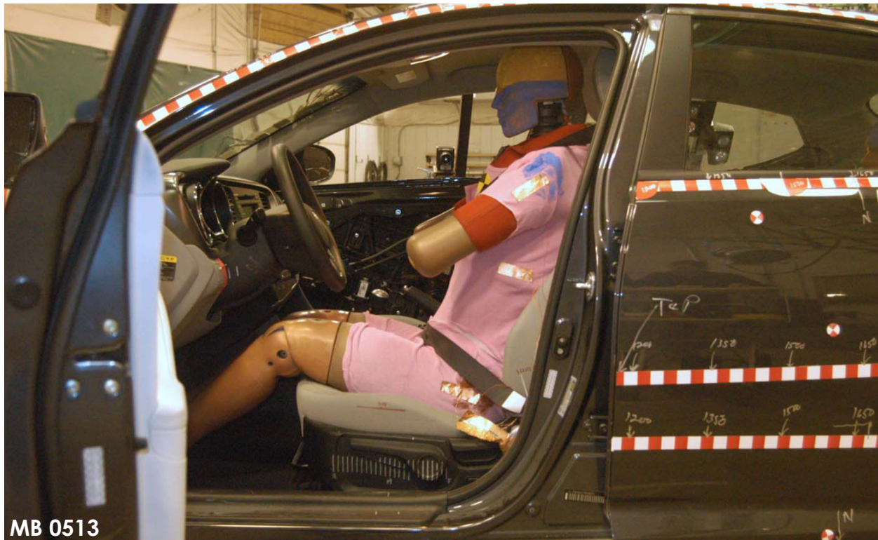
Figure A-27: Pre-Test Left Side View of Driver Dummy Showing Belt, Chalking, and Contact Switches
