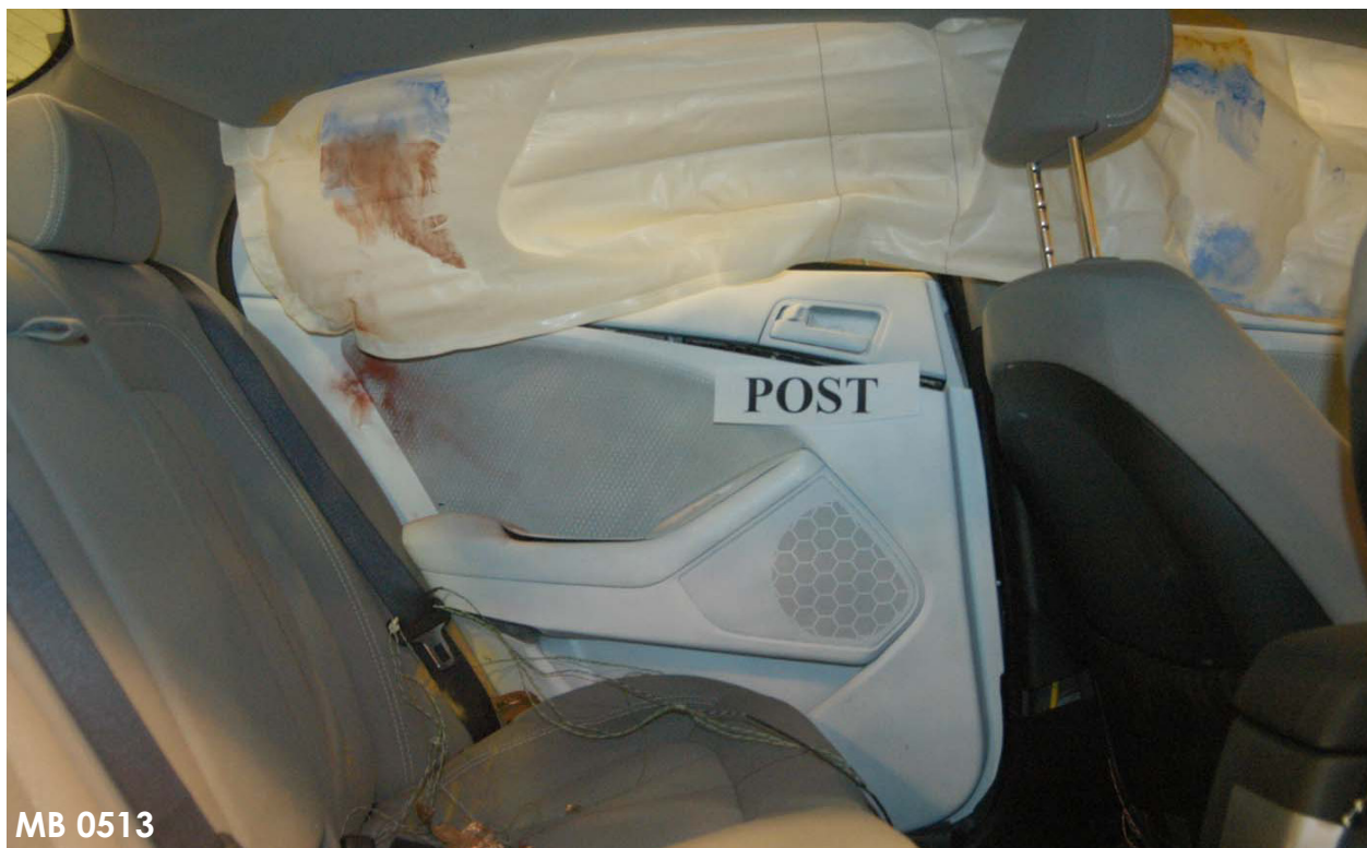
Figure A-72: Post-Test Rear Passenger Inner Door Panel View Showing Rear Passenger Dummy Contact Locations
