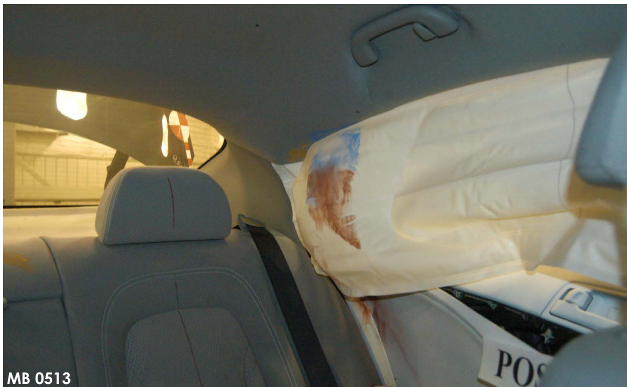
Figure A-74: Post-Test Rear Passenger Dummy Close-Up Head Contact with Side Airbag View
