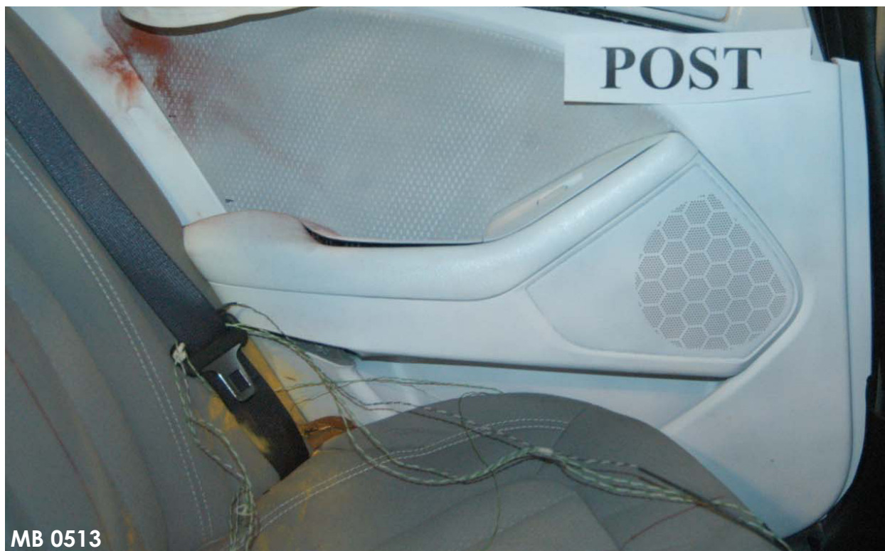
Figure A-77: Post-Test Rear Passenger Dummy Close-Up Pelvis Contact View
