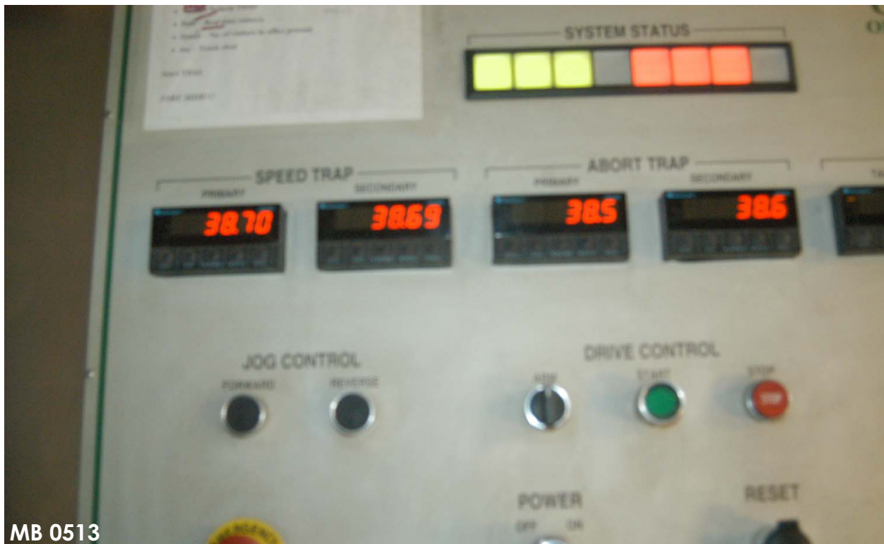
Figure A-92: Post-Test Primary and Redundant Speed Trap Read-Out
