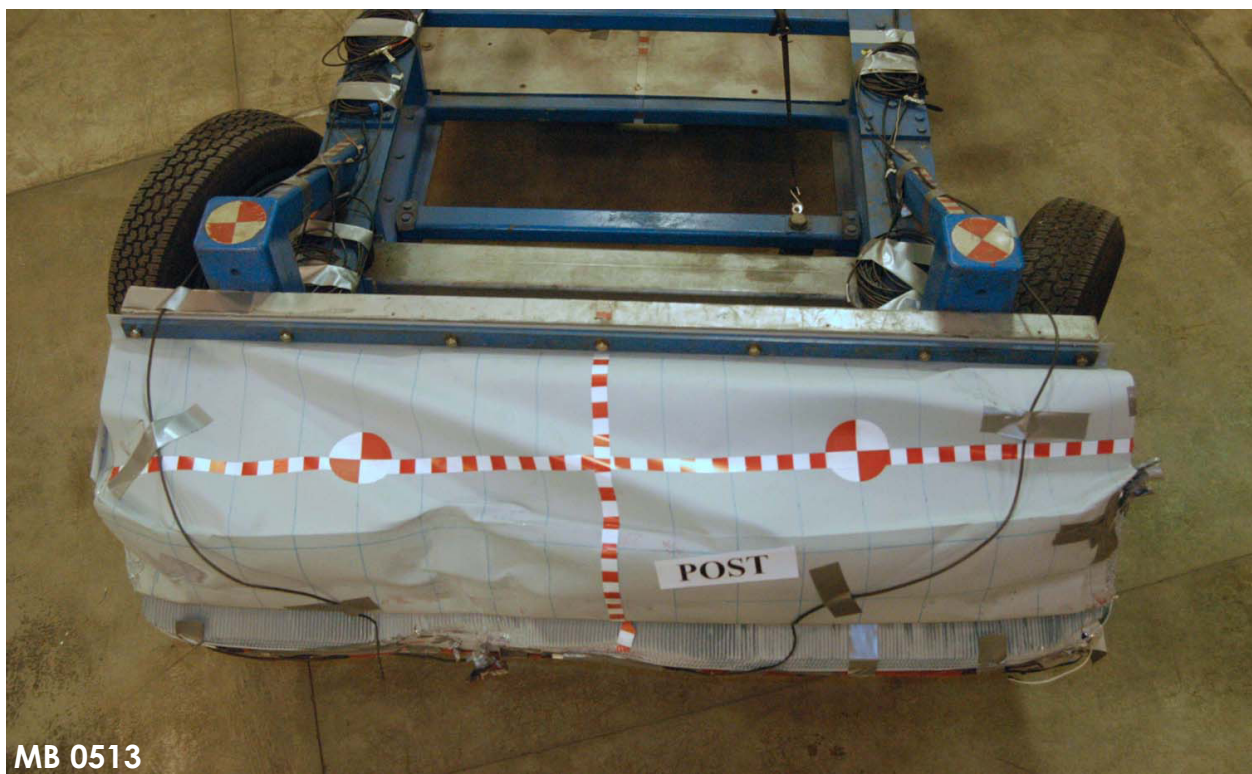
Figure A-84: Post-Test Top View of MDB Impactor Face
