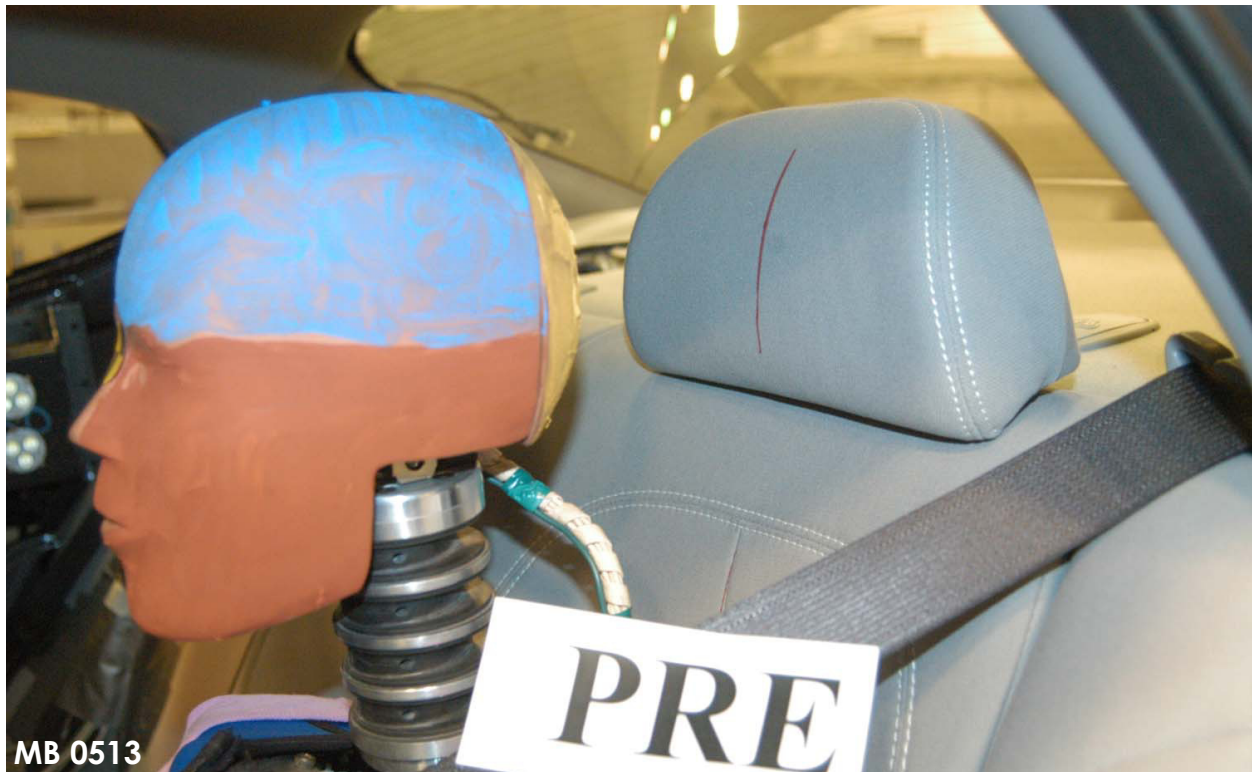
Figure A-57: Pre-Test Frontal View of Rear Passenger Dummy Head and Shoulders in Relation to Head Restraint
