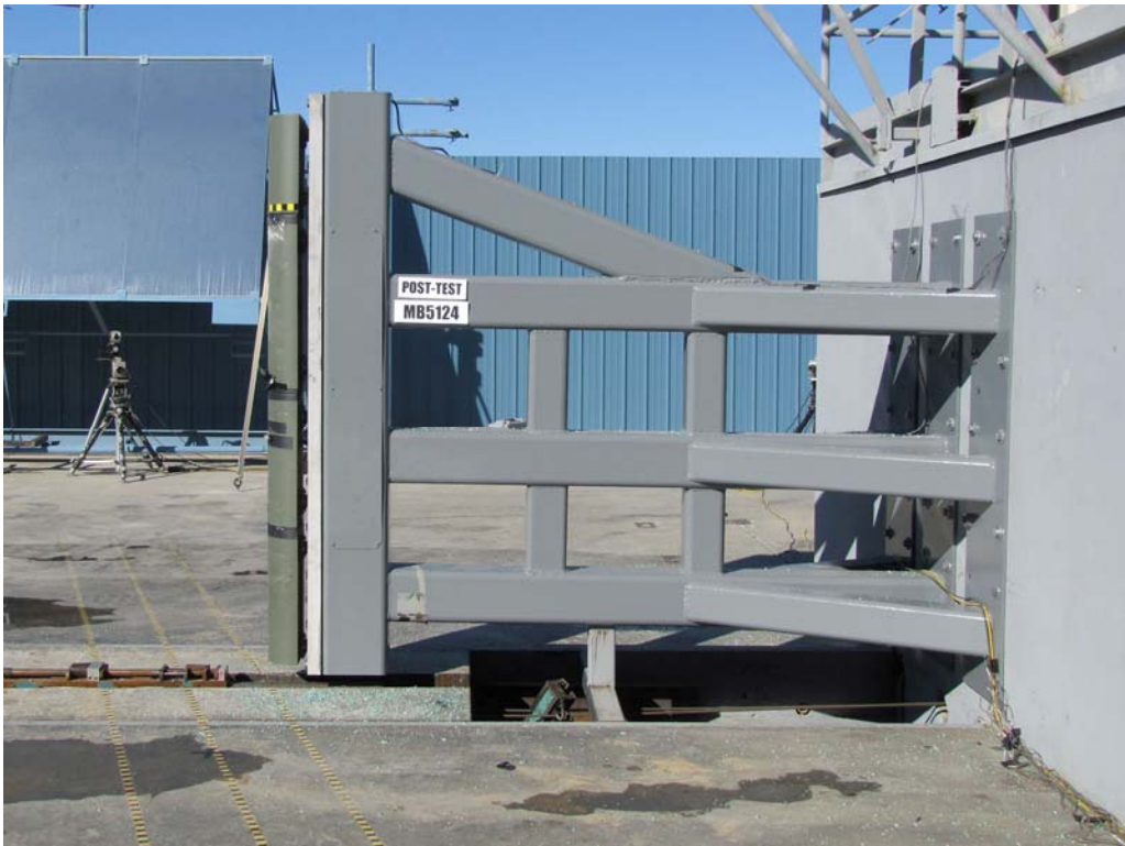
FIGURE 58. Post-Test Pole Barrier Side View
