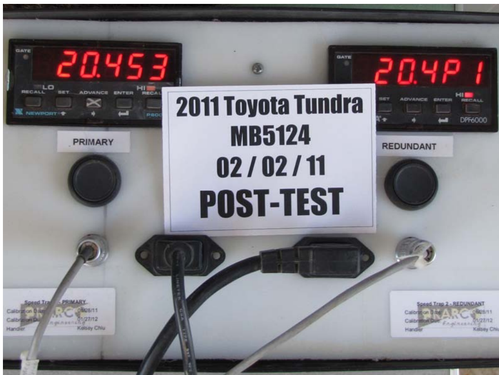
FIGURE 60. Post-Test Primary and Redundant Speed Trap Read-Out
