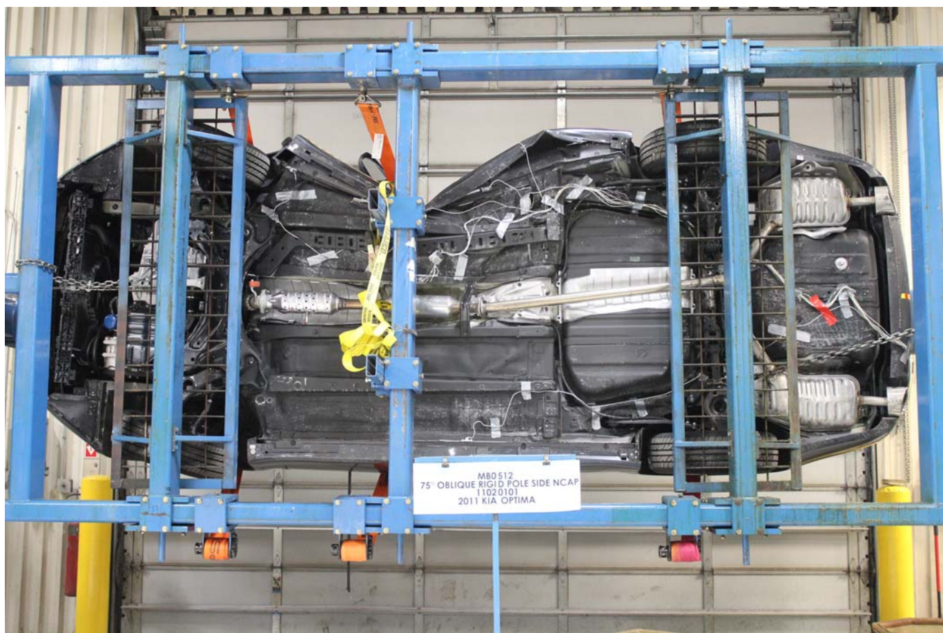
FMVSS No. 301/305 Rollover 270 Degrees
