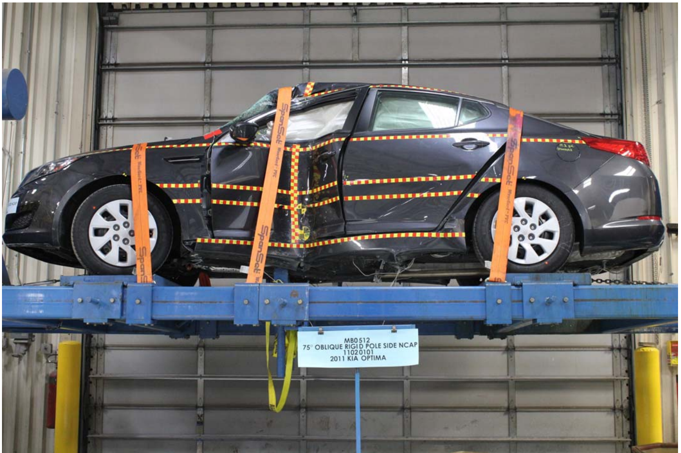
FMVSS No. 301/305 Rollover 0 Degrees
