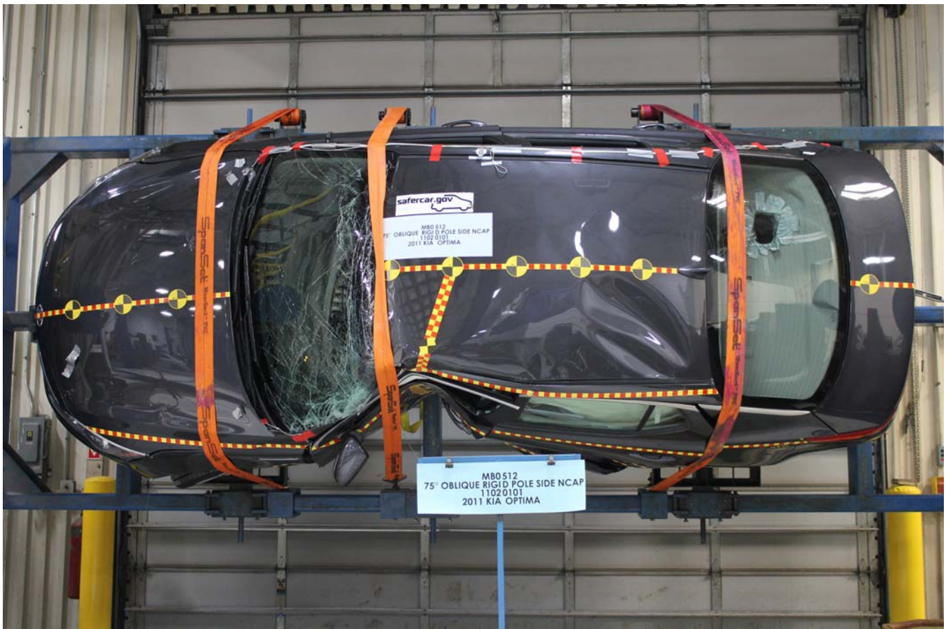
FMVSS No. 301/305 Rollover 90 Degrees
