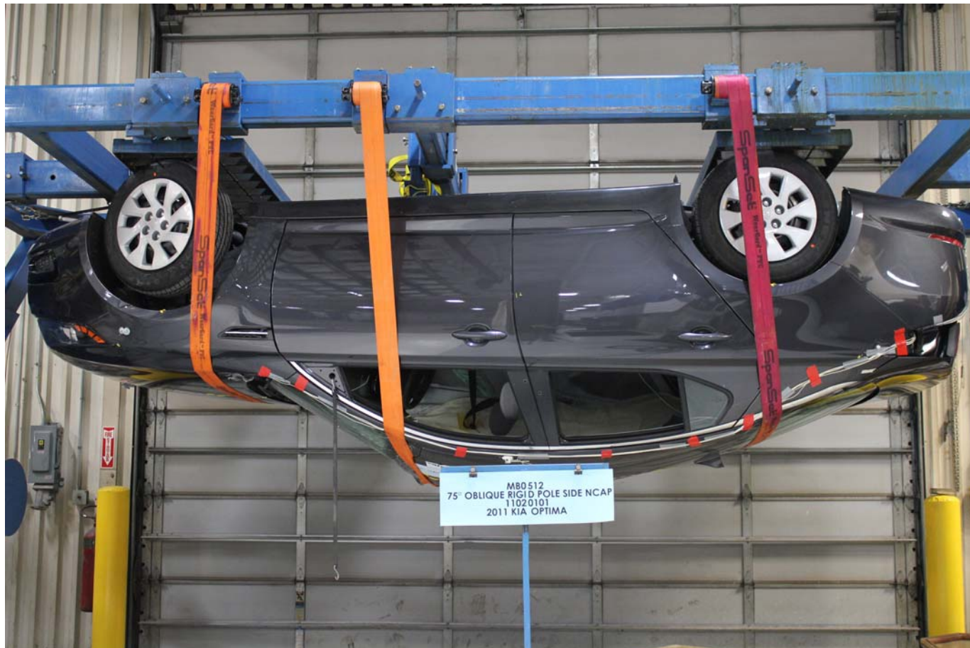
FMVSS No. 301/305 Rollover 180 Degrees
