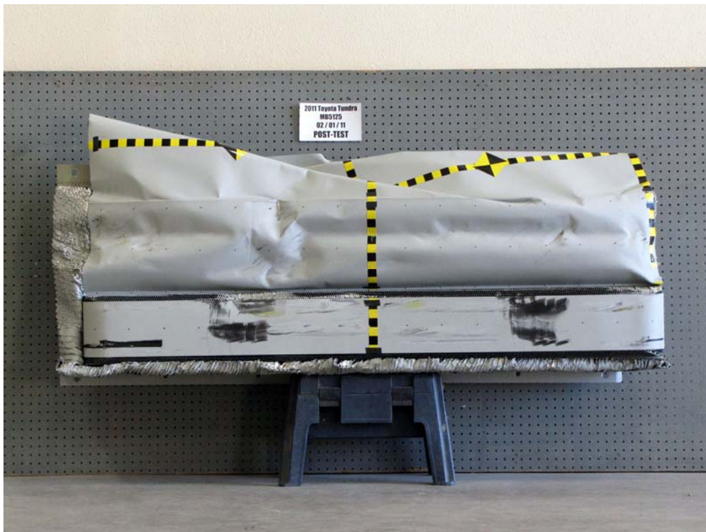
FIGURE 82. Post-Test Front View of MDB Impactor Face
