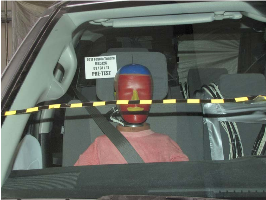
FIGURE 46. Pre-Test Passenger Dummy Front View
