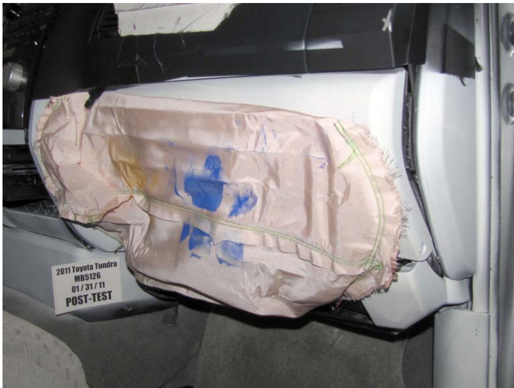
FIGURE 57. Post-Test Passenger's Side Knee Bolster
