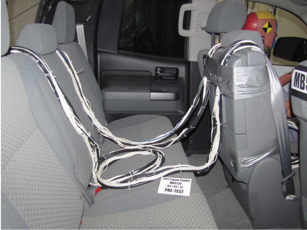
FIGURE 27. Pre-Test Dummy Cable Routing
