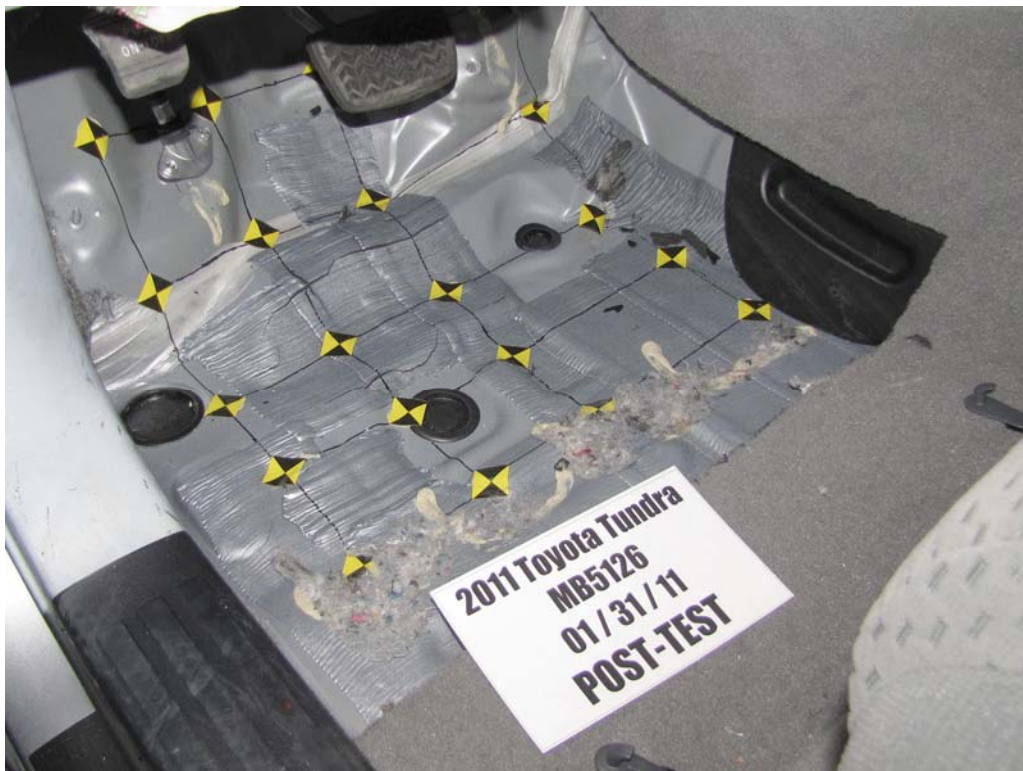
FIGURE 42. Post-Test Driver's Side Floorpan
