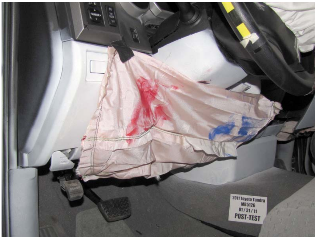
FIGURE 40. Post-Test Driver's Side Knee Bolster
