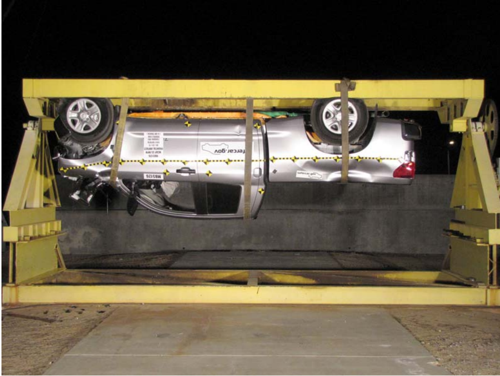
FIGURE 66. Vehicle at 180°on Static Rollover Device
