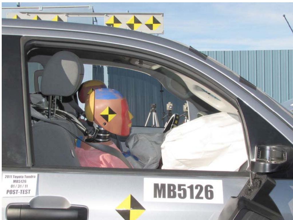
FIGURE 49. Post-Test Passenger Dummy Window View
