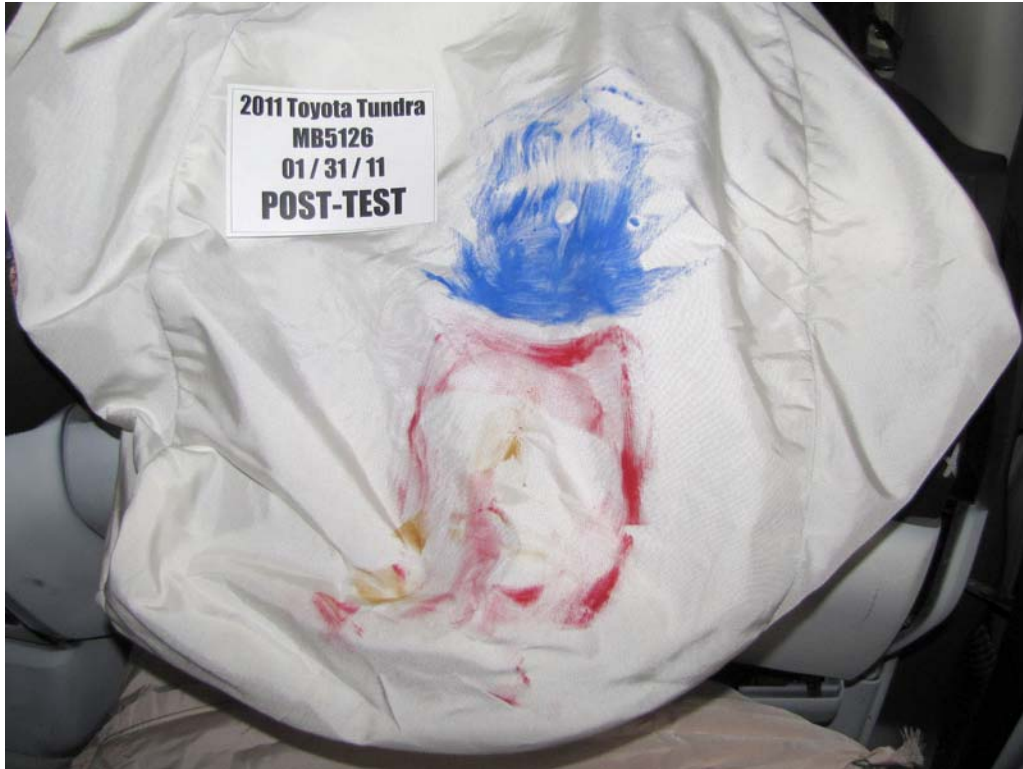
FIGURE 60. Post-Test Passenger Dummy Contact With Airbag
