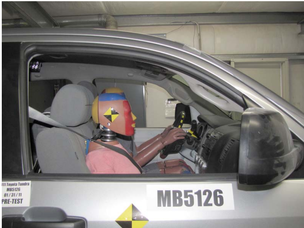
FIGURE 48. Pre-Test Passenger Dummy Window View
