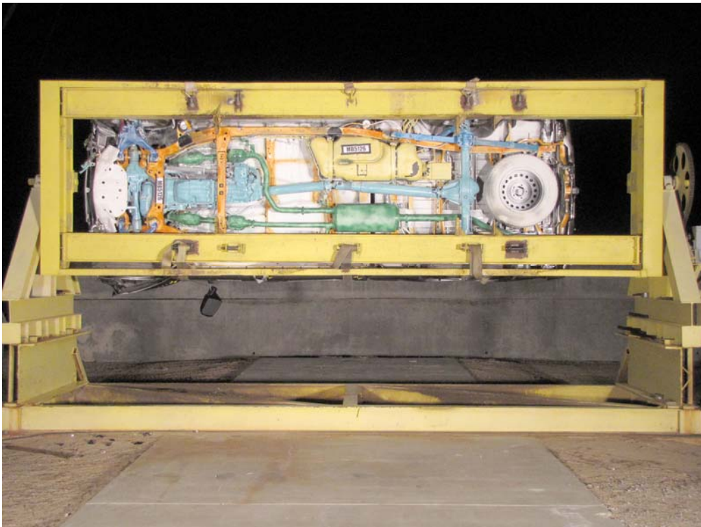
FIGURE 67. Vehicle at 270°on Static Rollover Device
