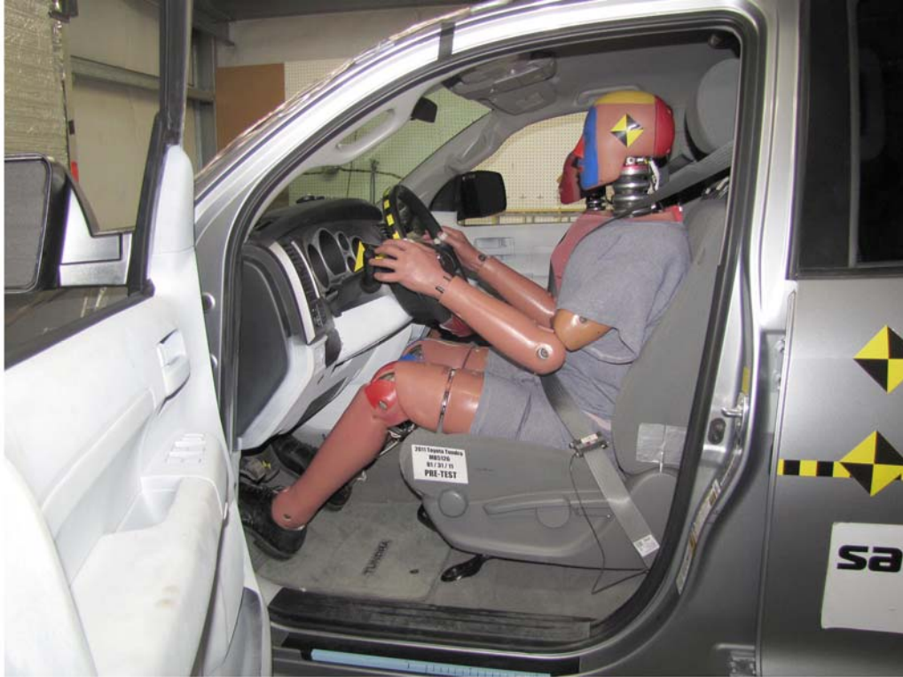
FIGURE 33. Pre-Test Driver Dummy and Vehicle Interior View
