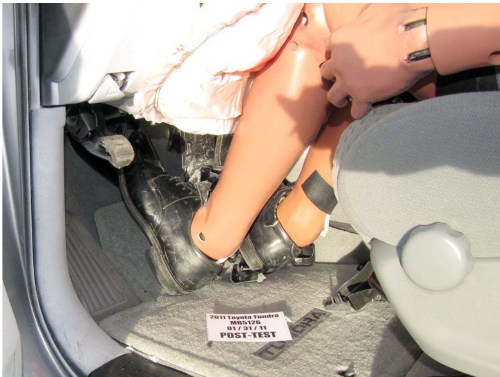
FIGURE 38. Post-Test Driver Dummy Feet
