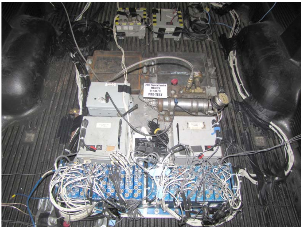
FIGURE 61. Pre-Test of Ballast Installed in Vehicle
