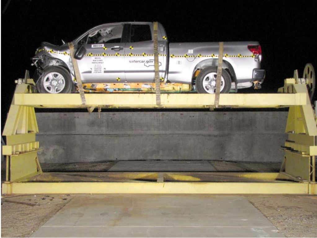
FIGURE 68. Vehicle at 360° on Static Rollover Device
