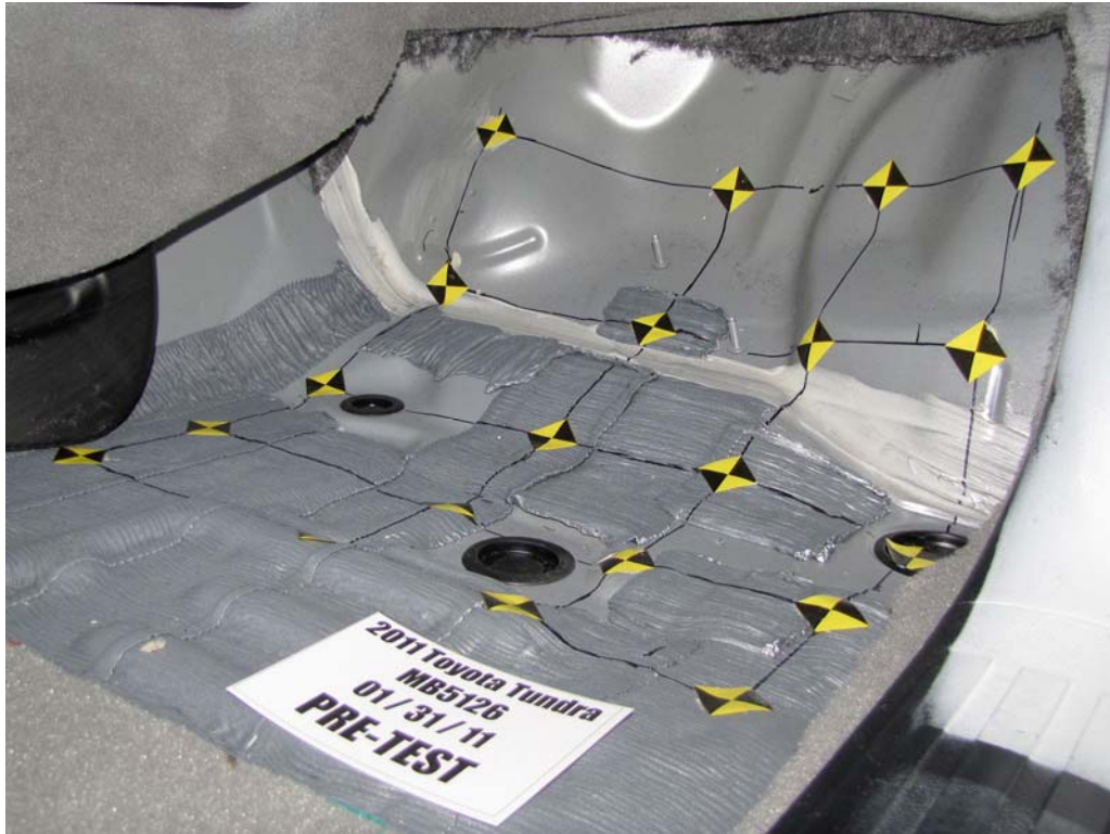
FIGURE 58. Pre-Test Passenger's Side Floorpan
