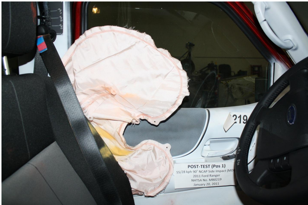
Figure A-50: Post-Test Driver Dummy Close-Up Torso Contact with Side Airbag View
