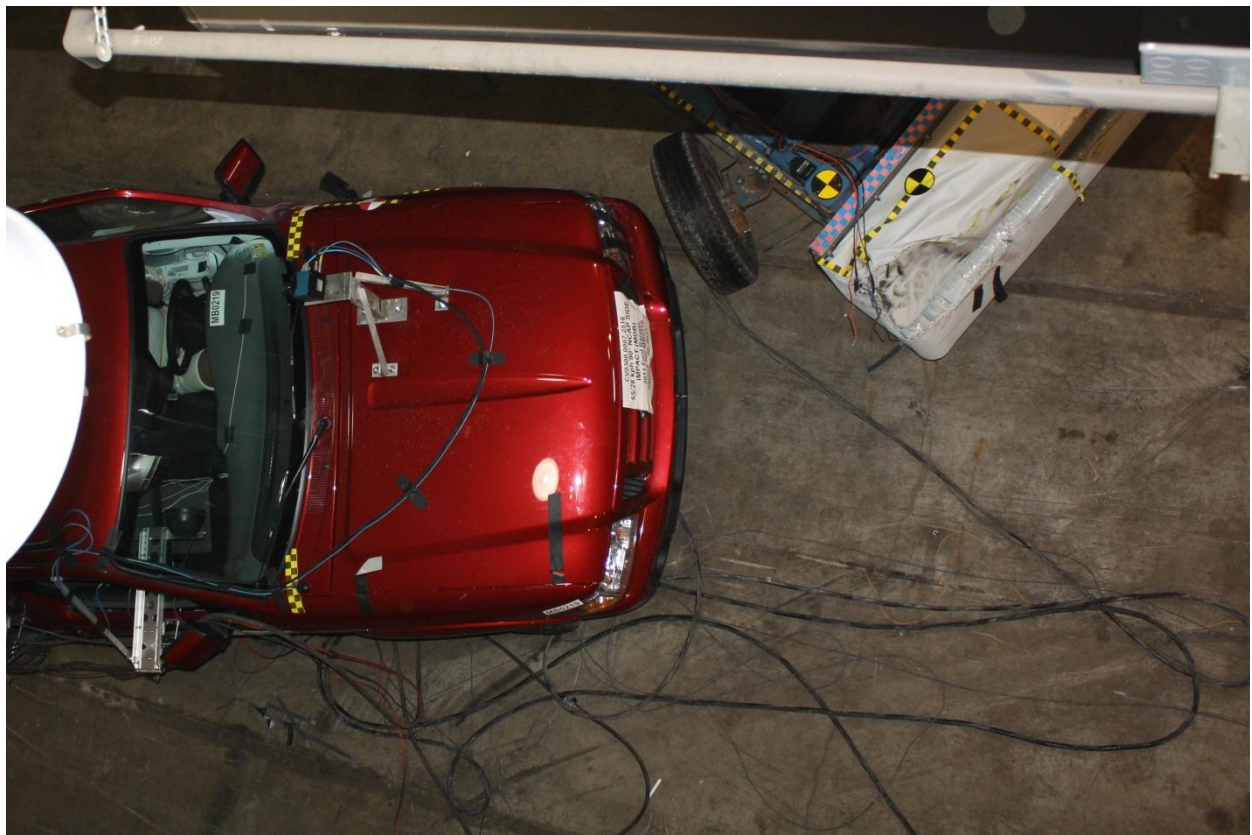
Figure A-16: Post-Test Overhead View of Test Vehicle and MDB
