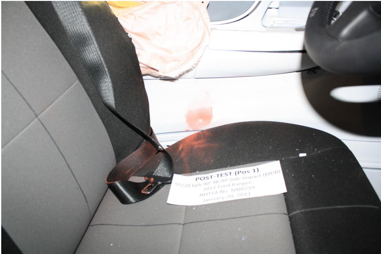
Figure A-51: Post-Test Driver Dummy Close-Up Pelvis Contact With Vehicle Interior View
