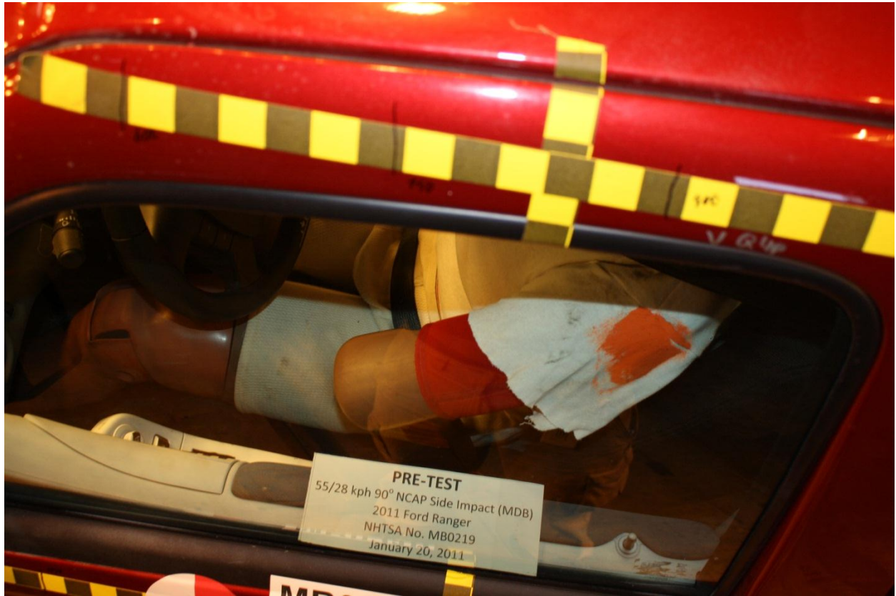
Figure A-41: Pre-test Driver Dummy and Door Clearance View
