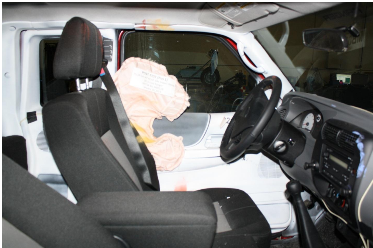
Figure A-46: Post-test Driver Inner Door Panel View Showing Driver Dummy Contact Locations
