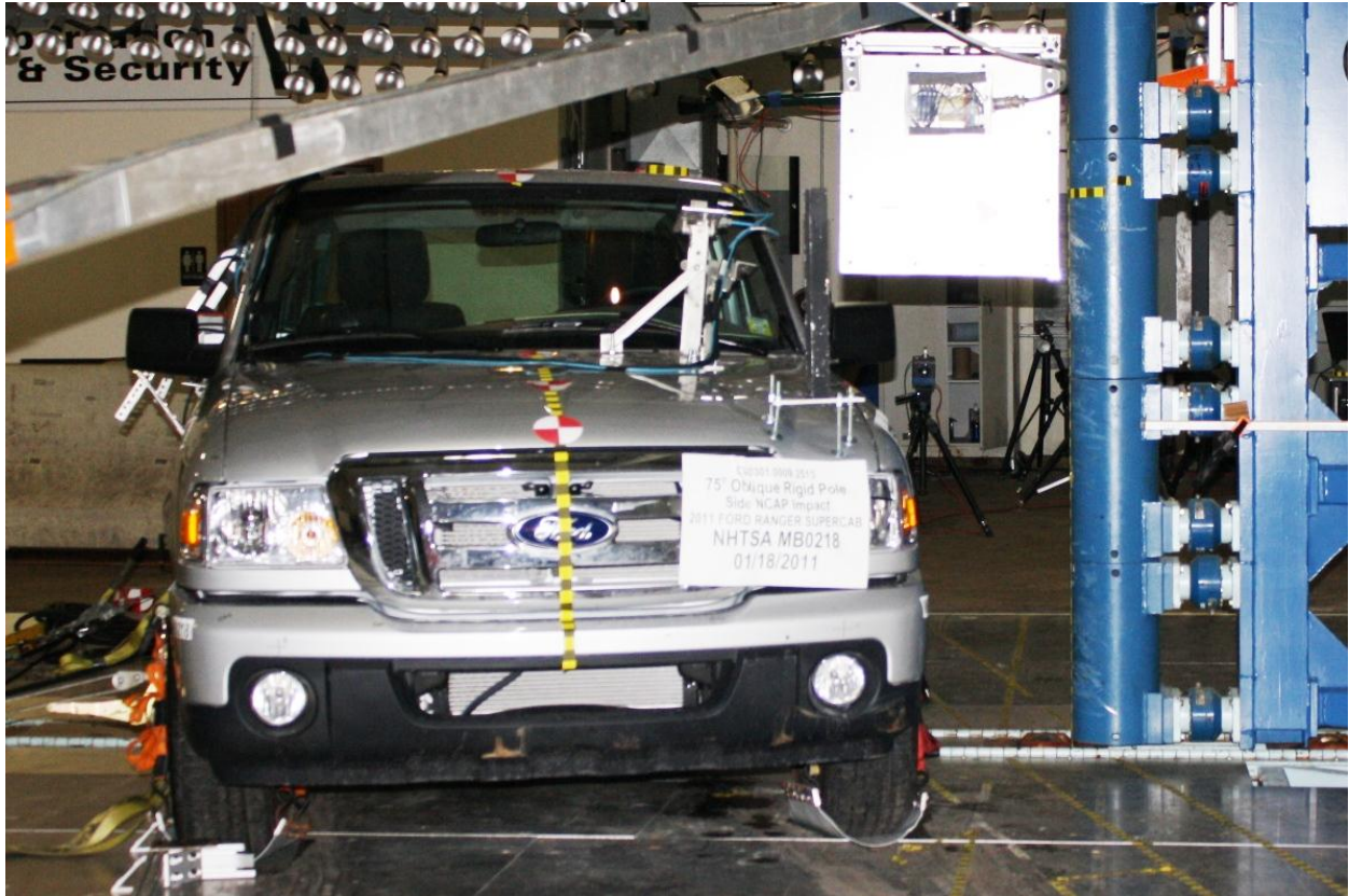
Figure A-18: Pre-Test Right Side View of Pole Positioned Against Side of Vehicle at Ideal Impact Point
