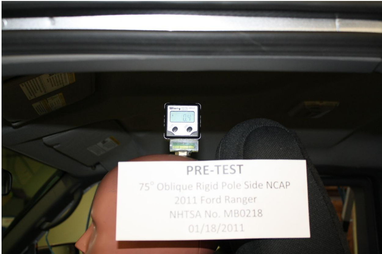
Figure A-31: Pre-Test View of Dummy's Head Showing Dummy's Head is Level
