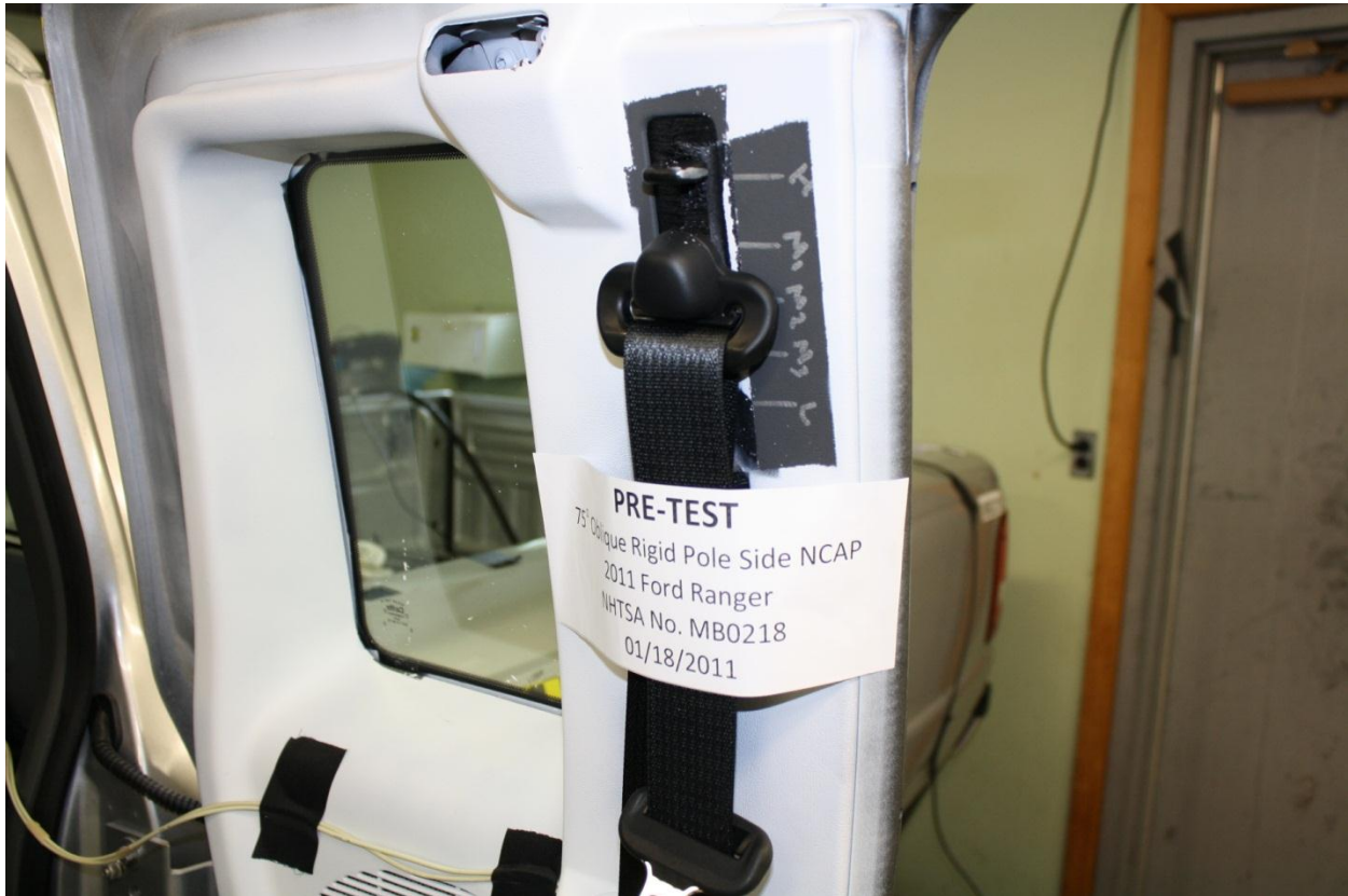
Figure A-33: Pre-Test View of Belt Anchorage for Dummy to Show Position
