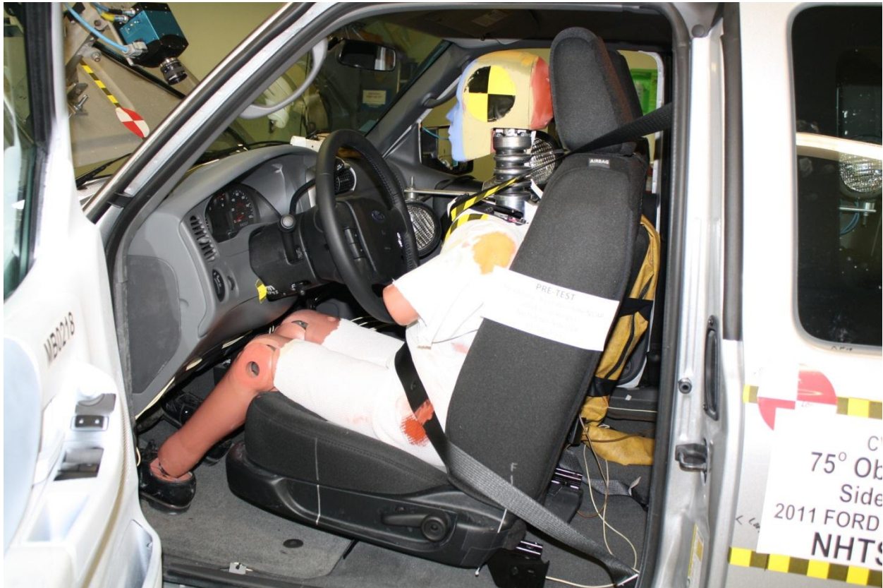
Figure A-23. Pre-Test Left Side View of Dummy Showing Belt, Chalking, and Contact Switches
