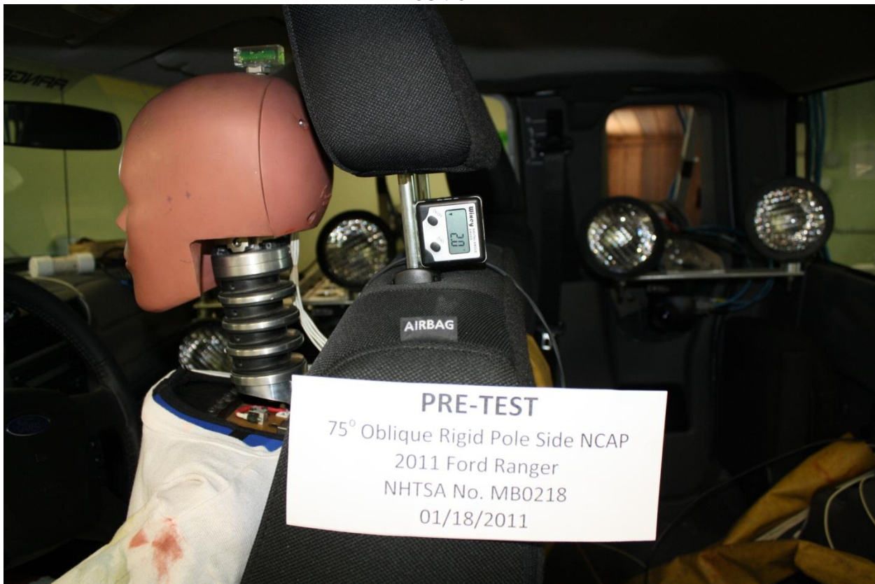
Figure A-38: Pre-Test Close-Up View of Driver Seat Back or Head Restraint Showing Seat Back Test Position
