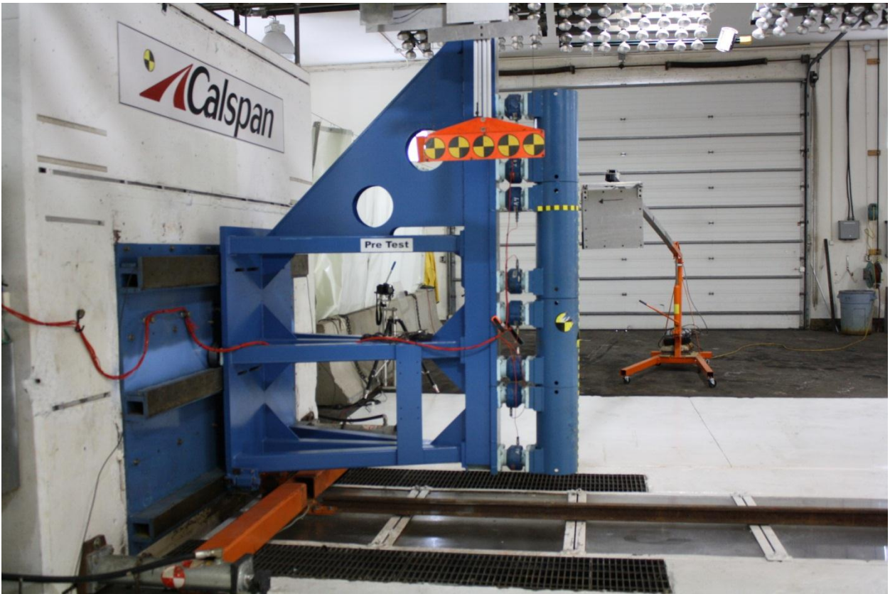
Figure A-57: Pre-Test Pole Barrier Side View
