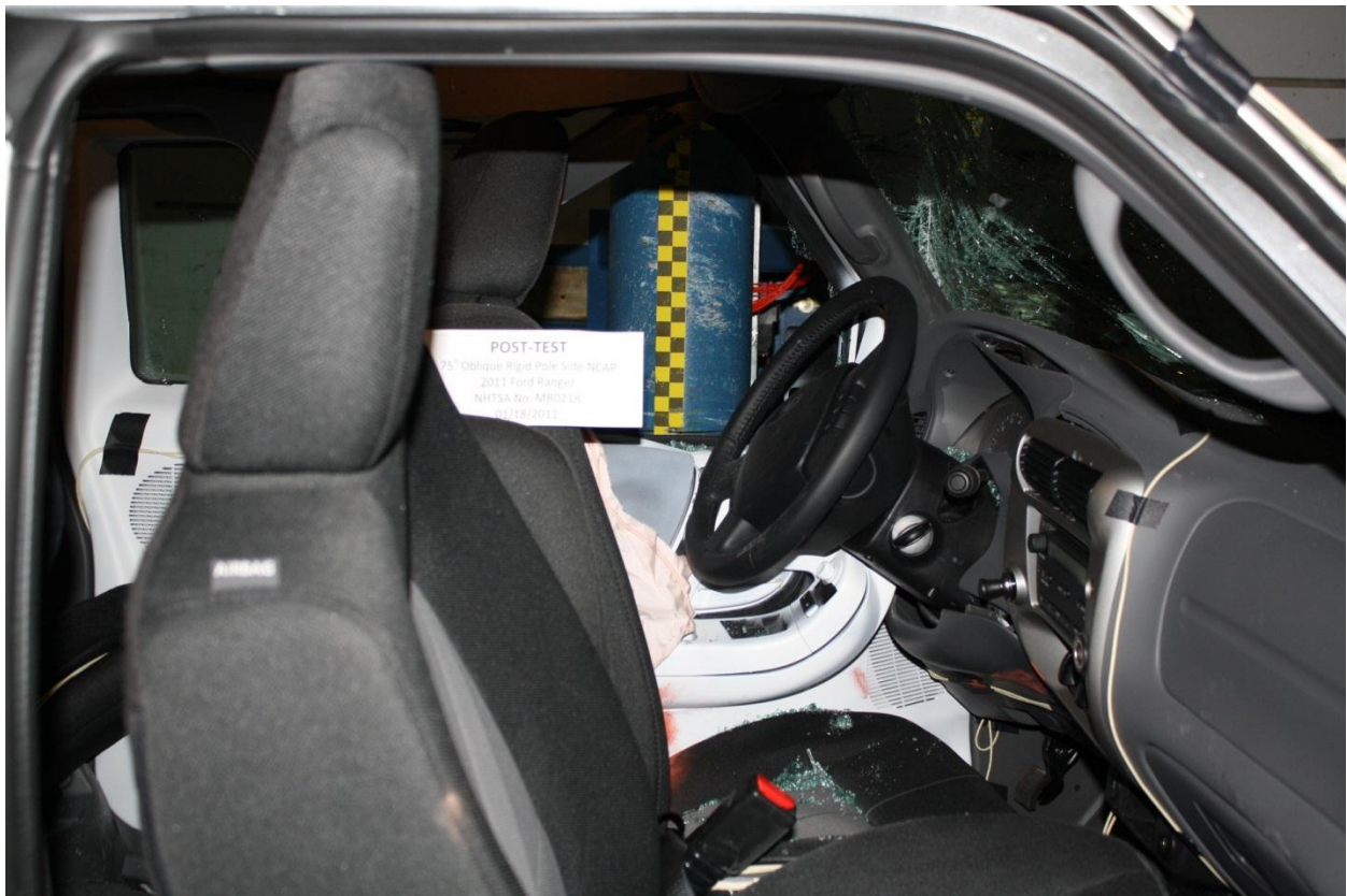
Figure A-44: Post-Test Inner Door Panel View Showing Dummy Contact Location
