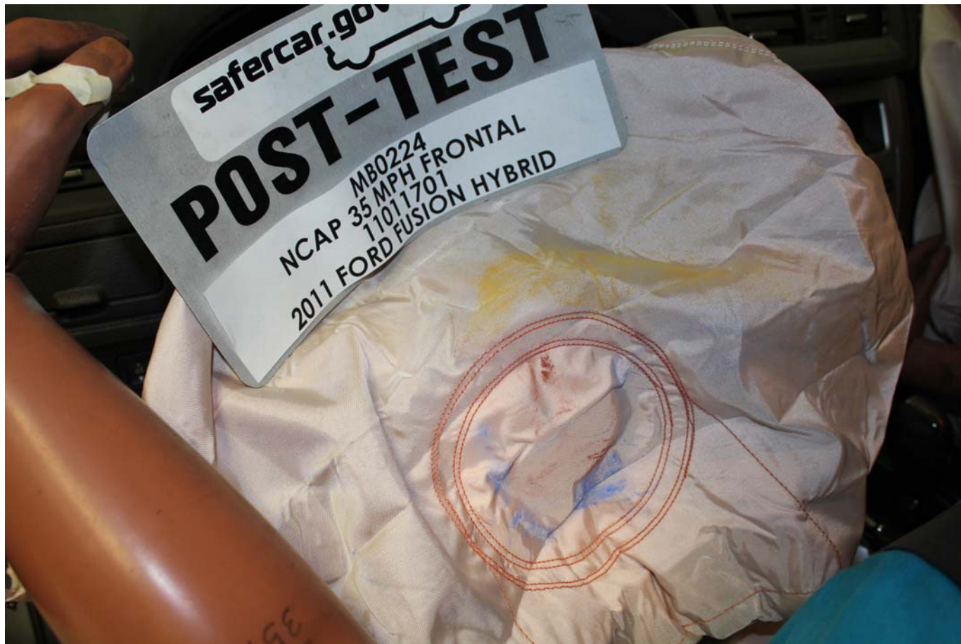
Post-Test Driver Dummy Contact with Airbag
