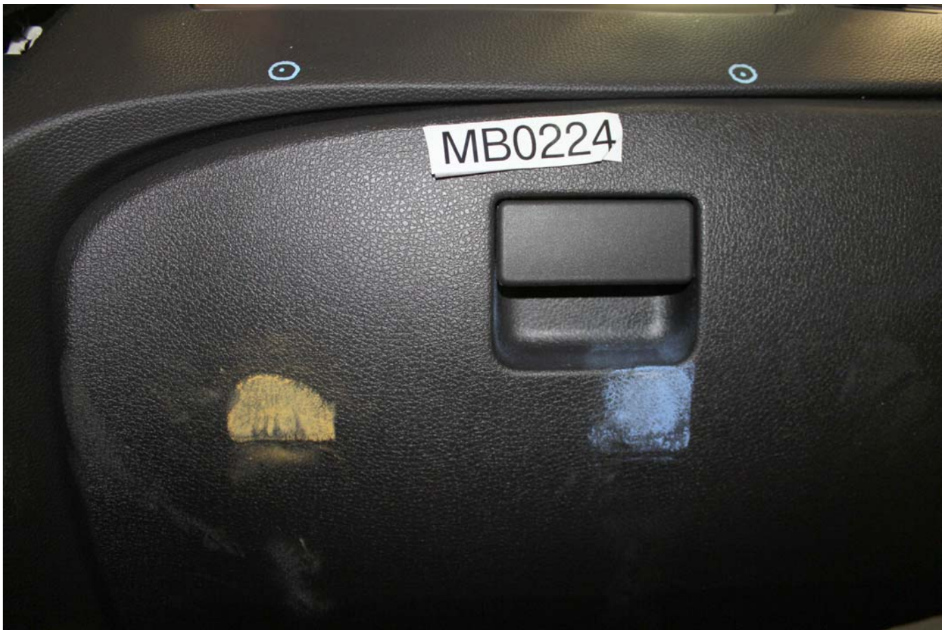
Post-Test Passenger Dummy Contact with Glovebox
