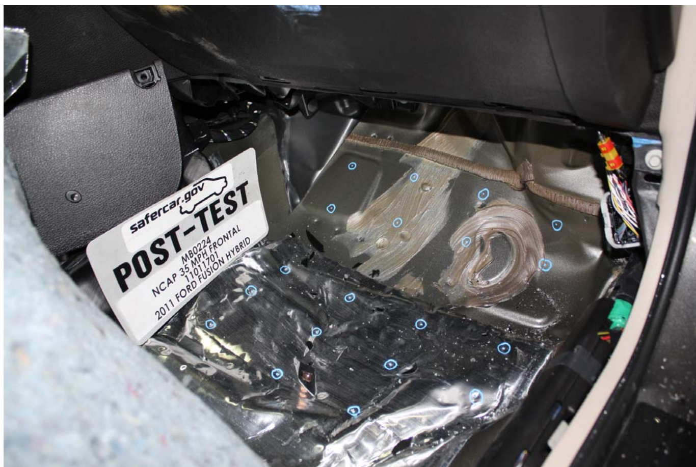
Post-Test Passenger's Side Floorpan
