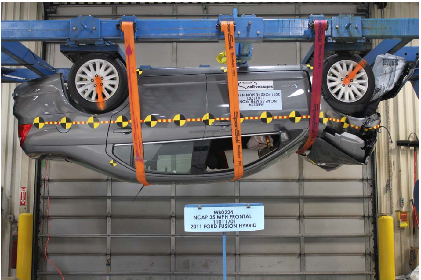
Vehicle at 180 Degrees on Static Rollover Device
