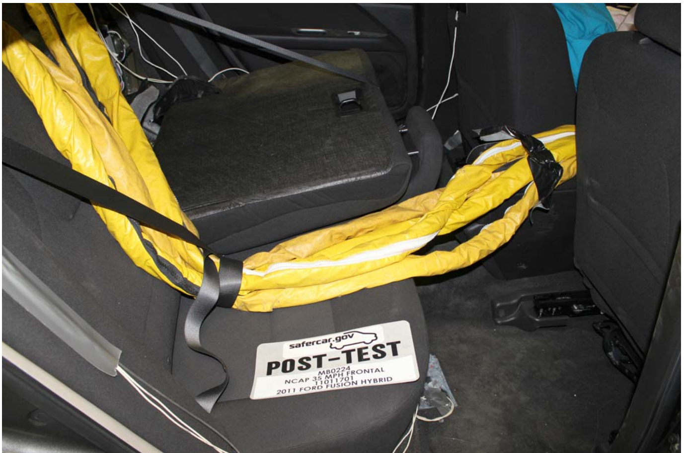
Post-Test Dummy Cable Routing
