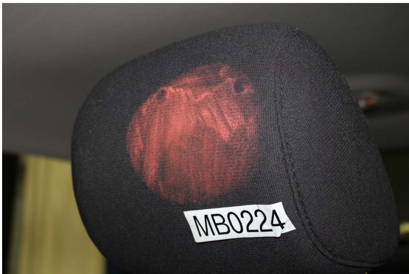
Post-Test Driver Dummy Contact with Headrest
