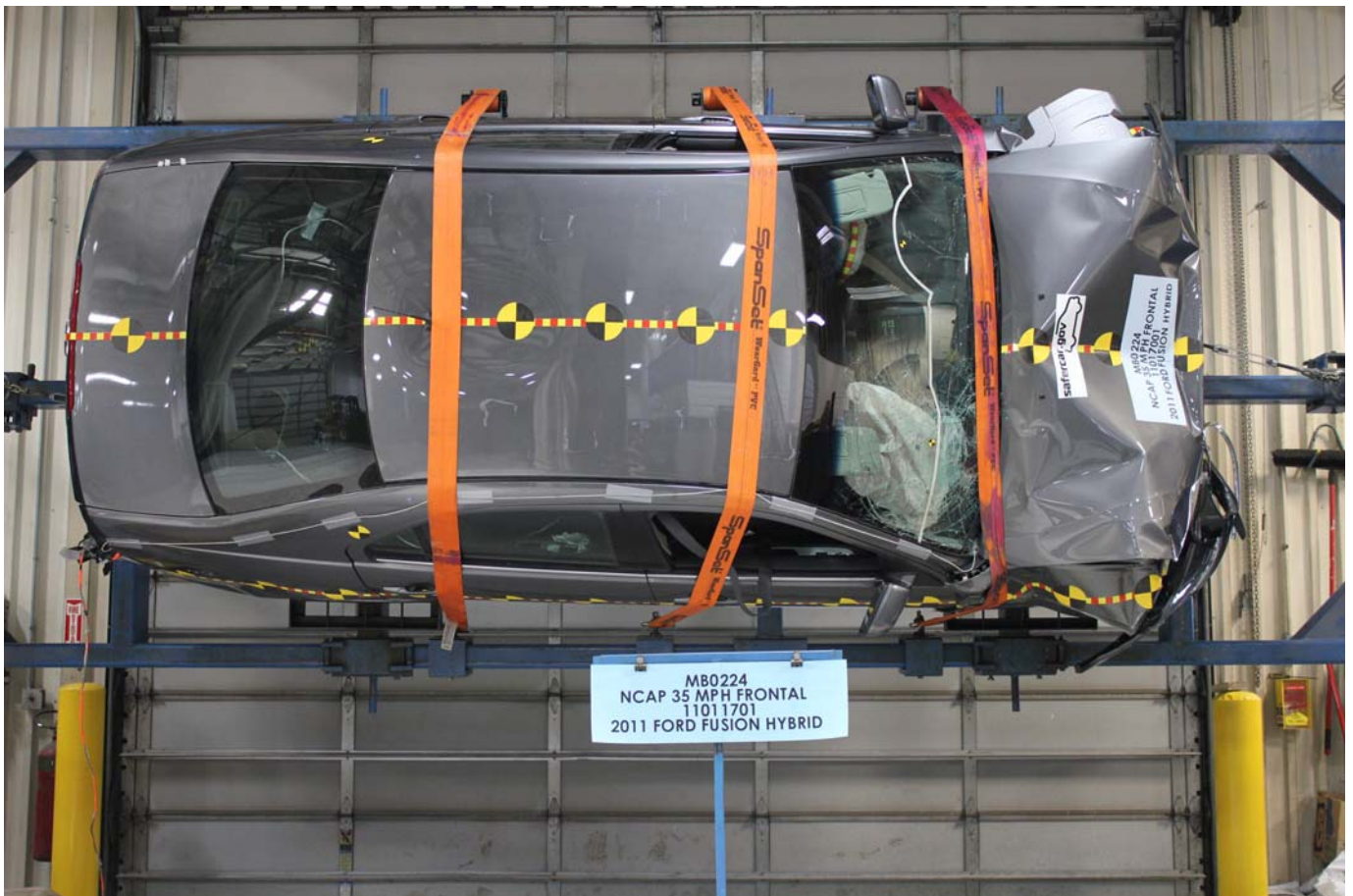
Vehicle at 270 Degrees on Static Rollover Device
