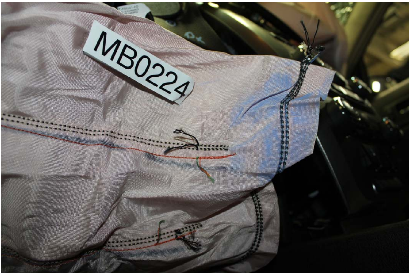
Post-Test Driver Dummy Contact with Knee Airbag
