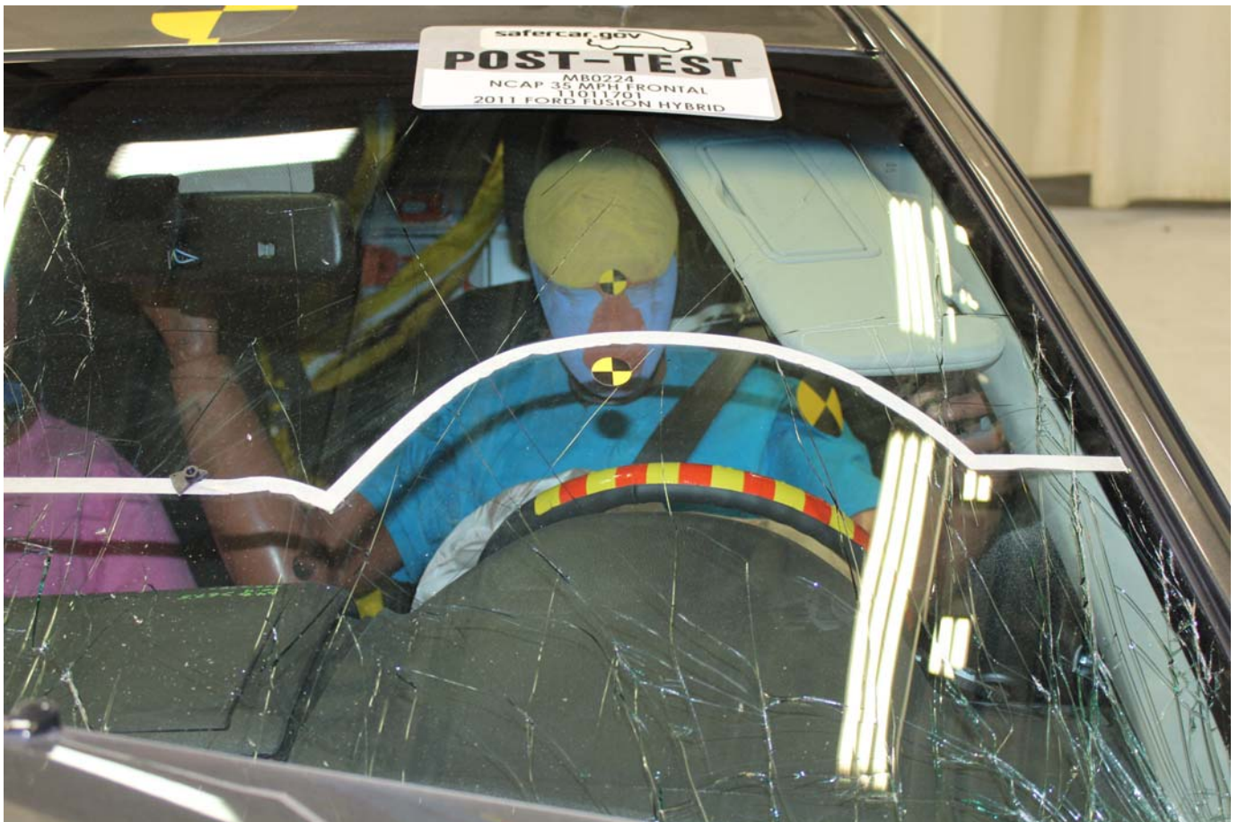
Post-Test Driver Dummy Front View
