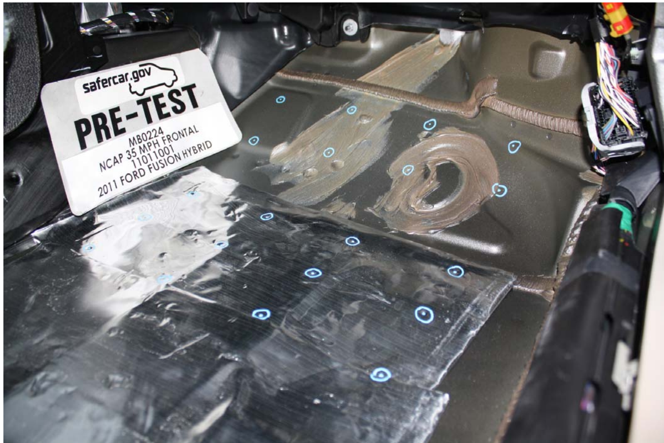
Pre-Test Passenger's Side Floorpan
