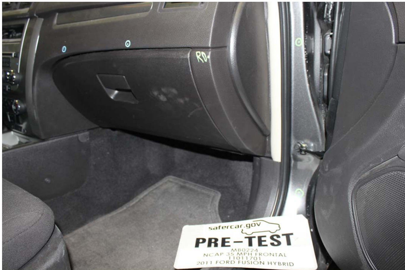
Pre-Test Passenger's Side Knee Bolster (without dummy)
