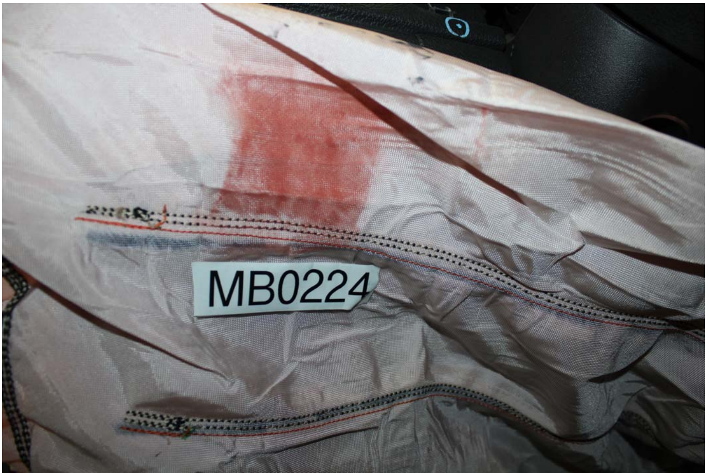
Post-Test Driver Dummy Contact with Knee Airbag
