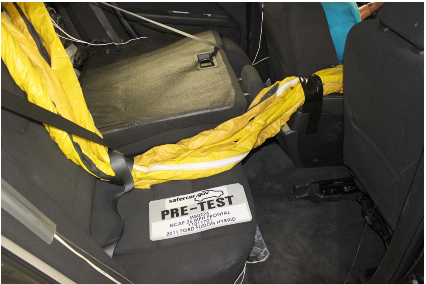
Pre-Test Dummy Cable Routing
