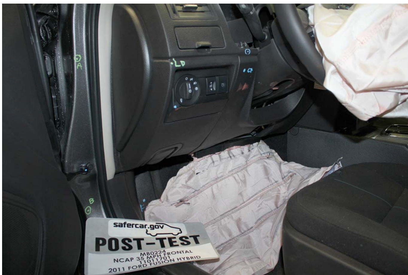
Post-Test Driver's Side Knee Bolster (without dummy)
