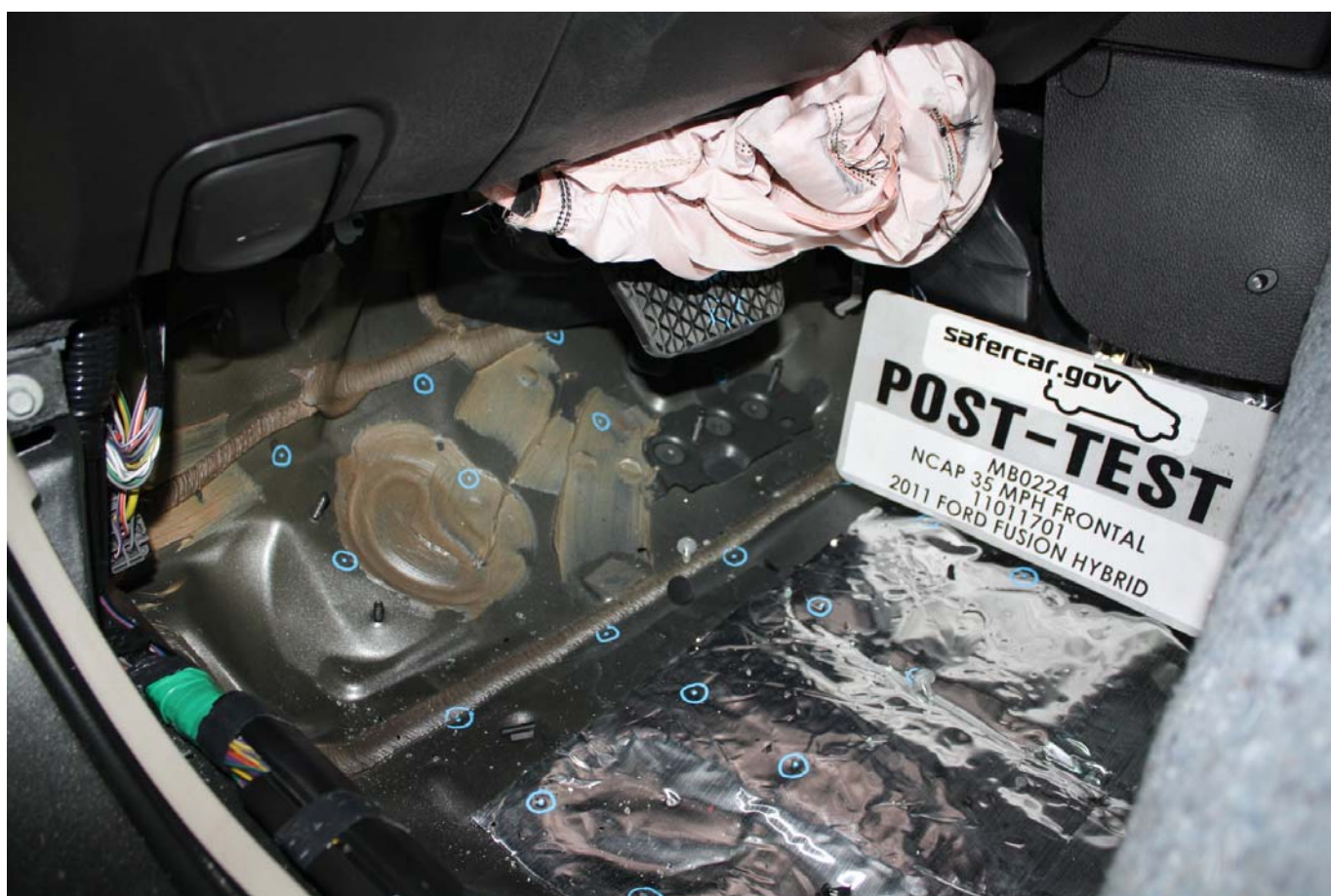
Post-Test Driver's Side Floorpan
