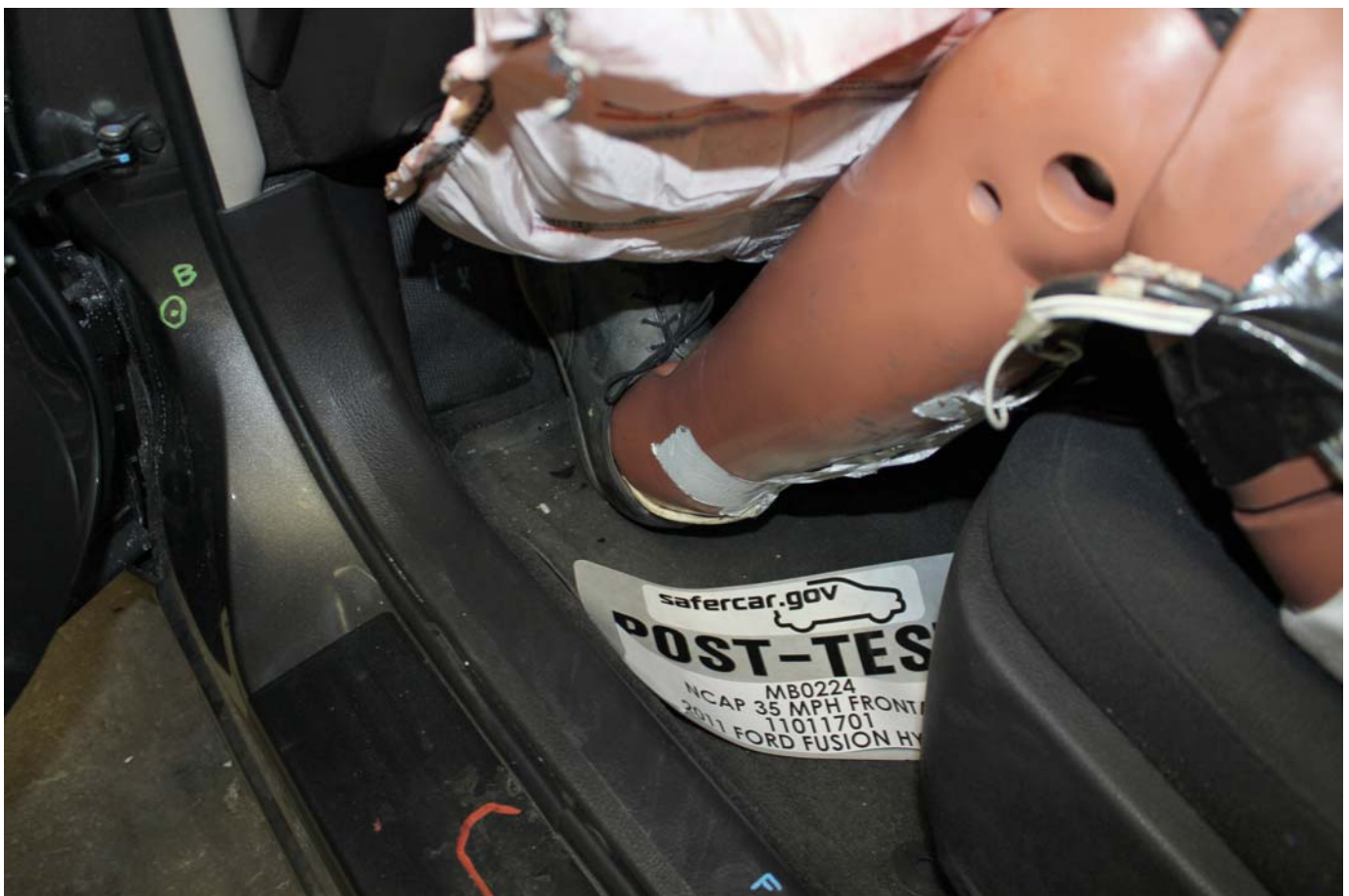
Post-Test Driver Dummy Feet
