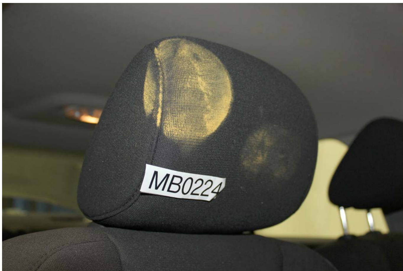
Post-Test Passenger Dummy Contact with Headrest
