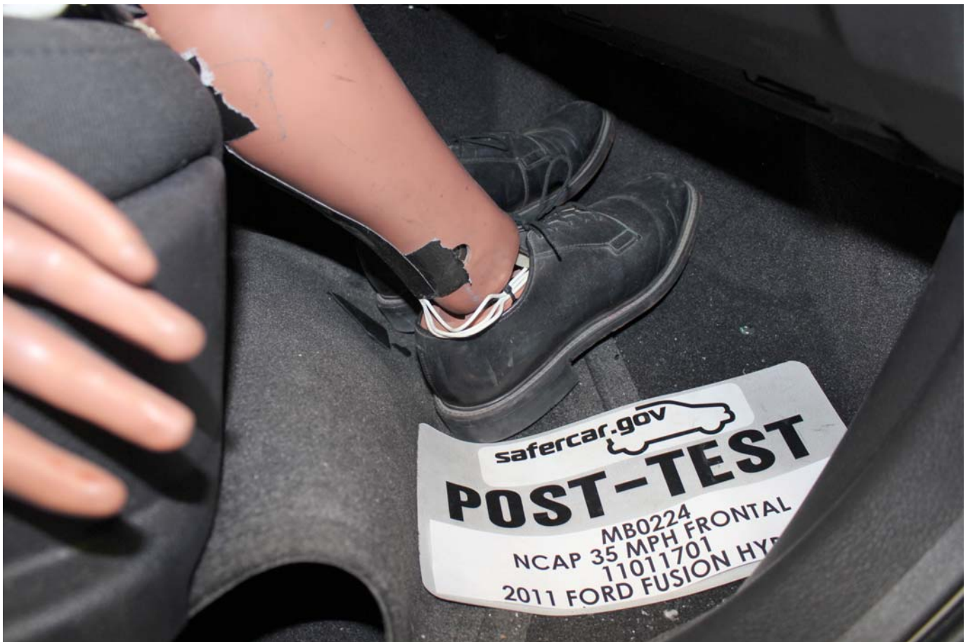
Post-Test Passenger Dummy Feet
