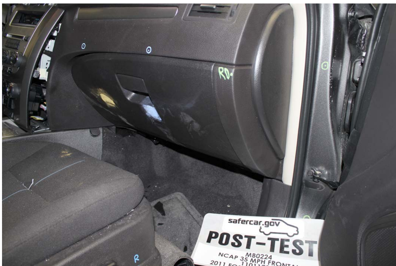
Post-Test Passenger's Side Knee Bolster (without dummy)
