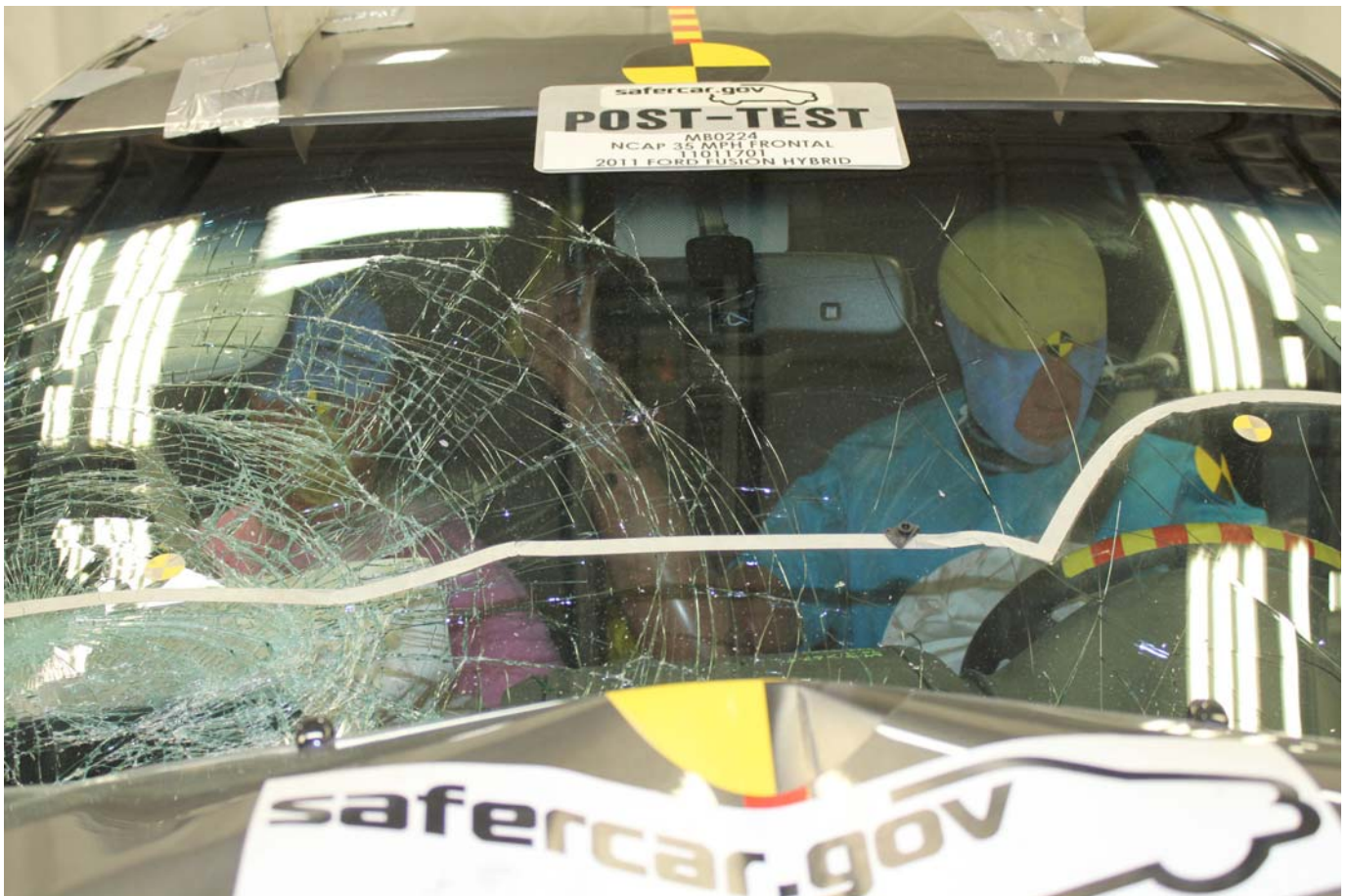
Post-Test Windshield View
