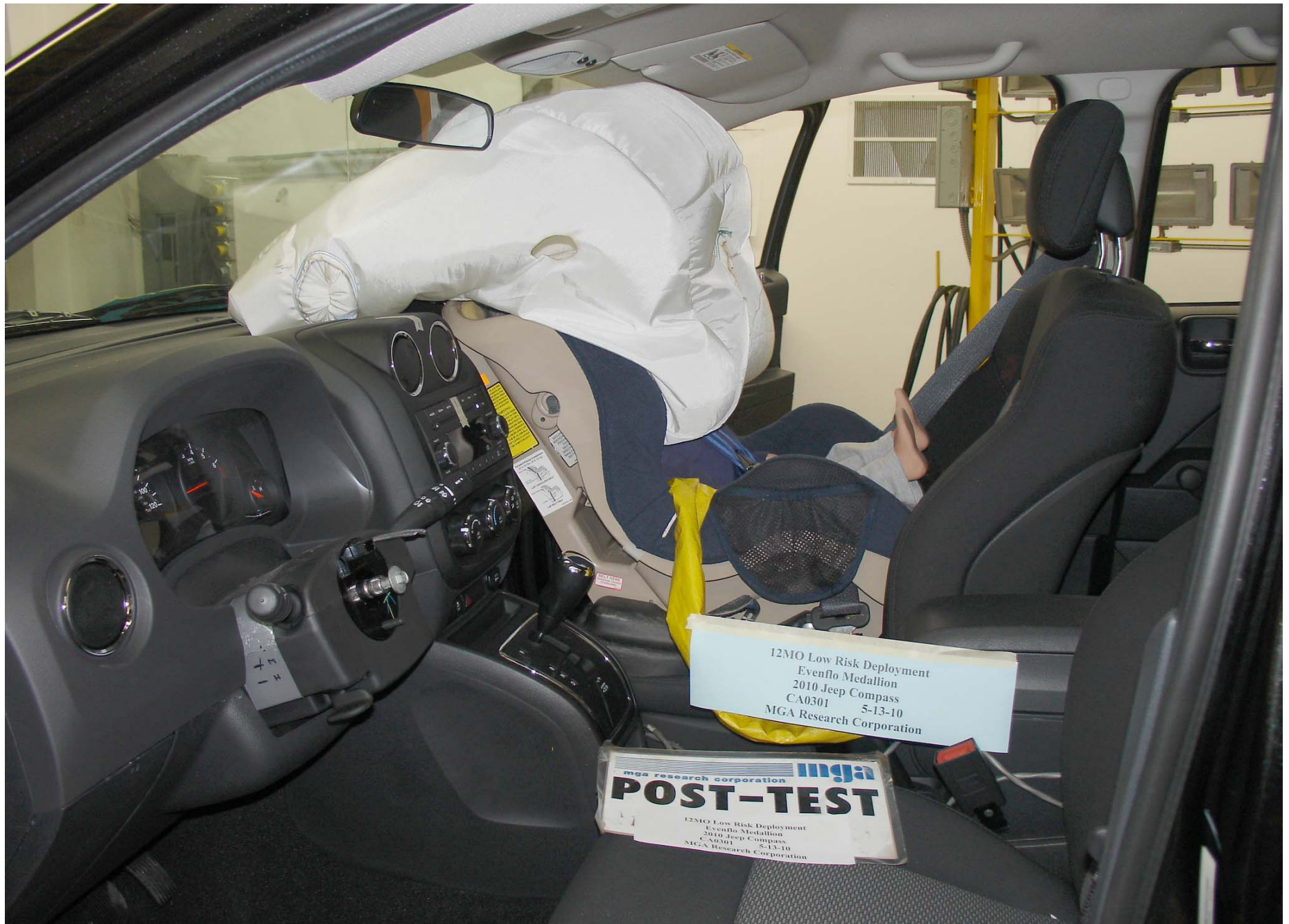
Post-Test 12 Mo Pass. Dummy Left Side View (Evenflo Medallion)
