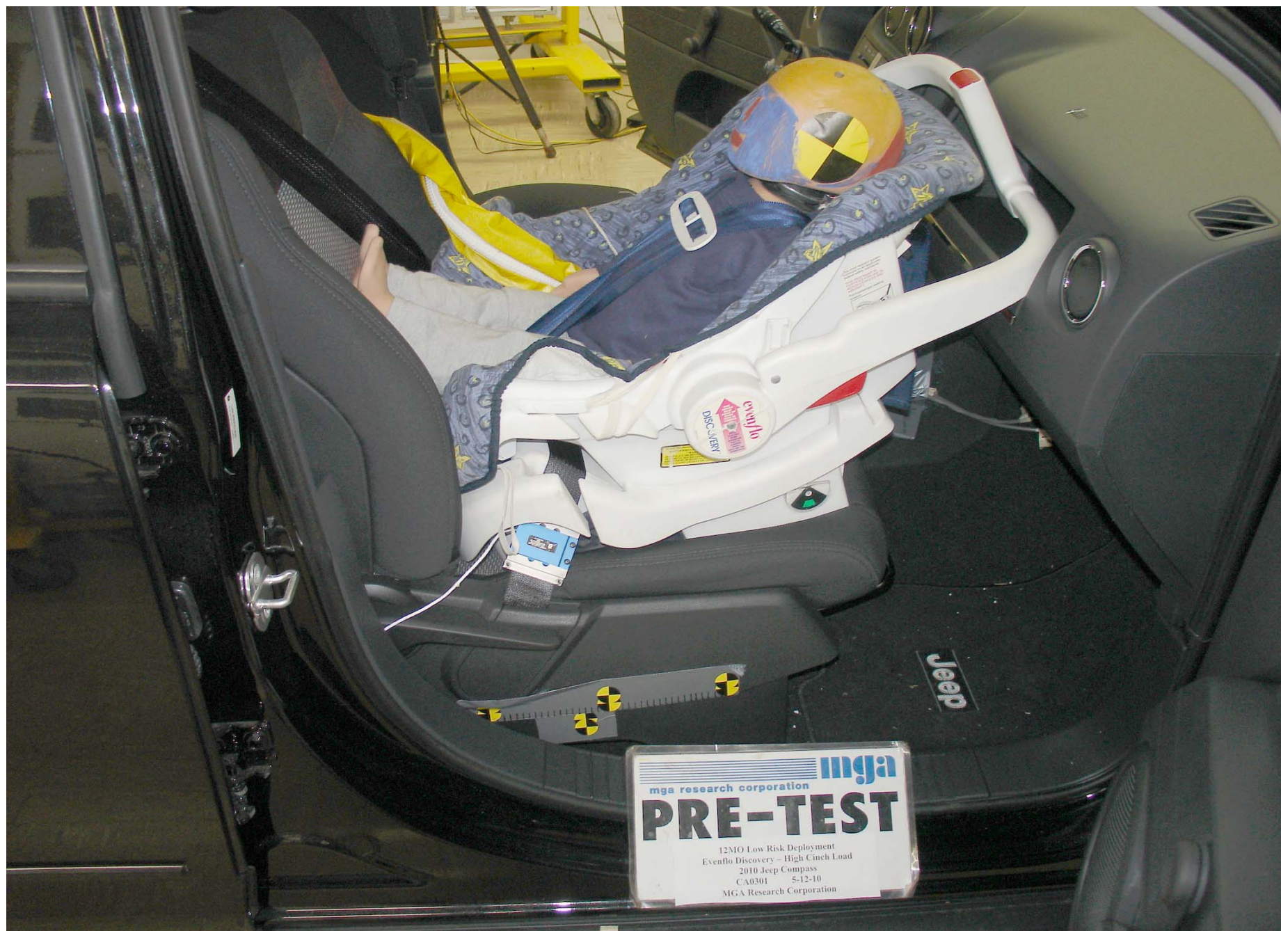
Pre-Test 12 Mo Pass. Dummy Right Side View (Evenflo Discovery) (High Cinch)
