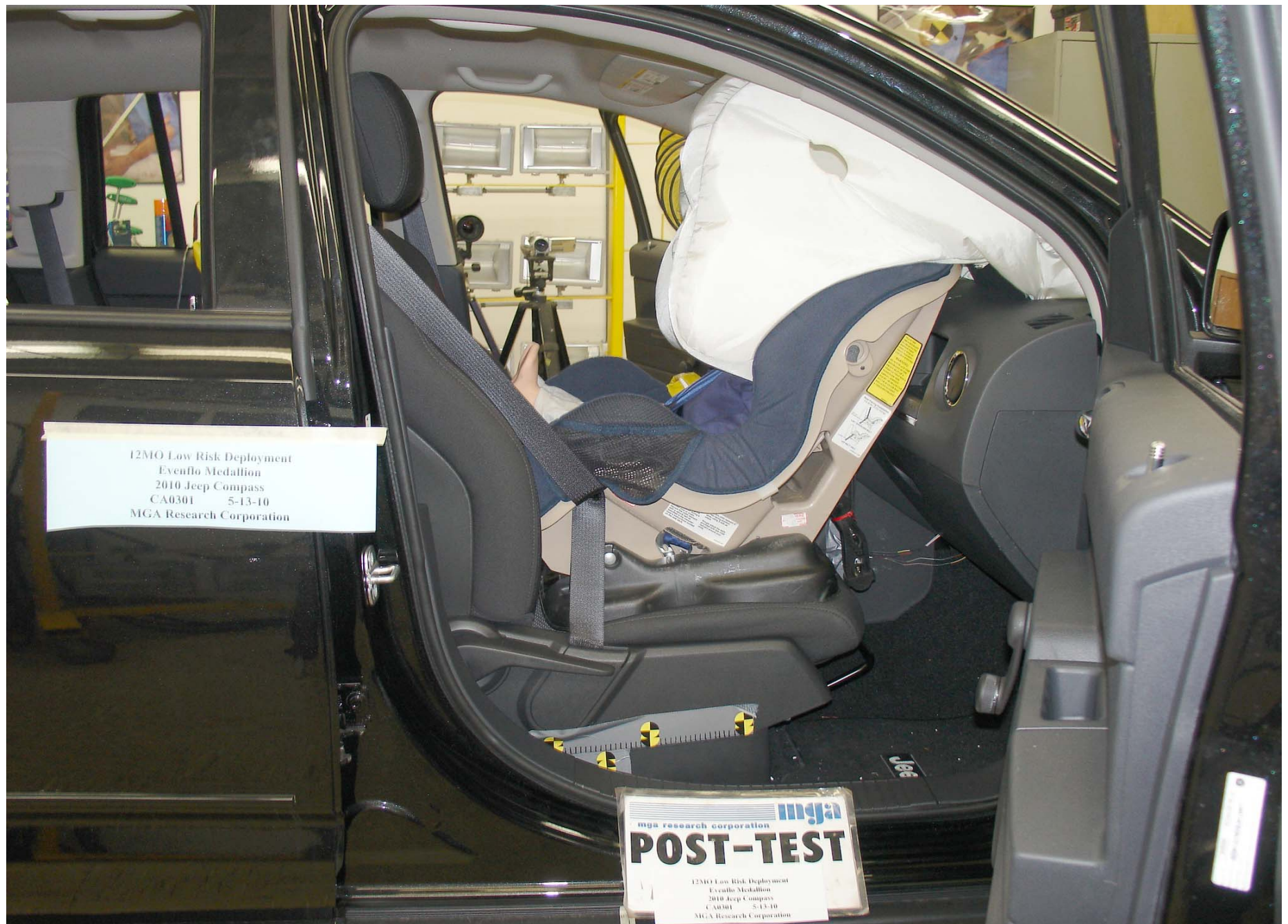
Post-Test 12 Mo Pass. Dummy Right Side View (Evenflo Medallion)
