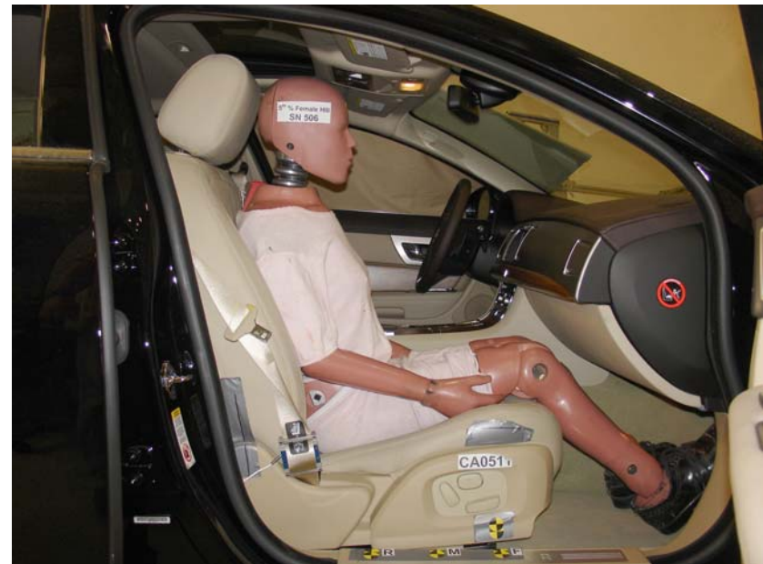
Unbelted 5th Percentile Female Dummy Reactivation, Forward Seat Track
