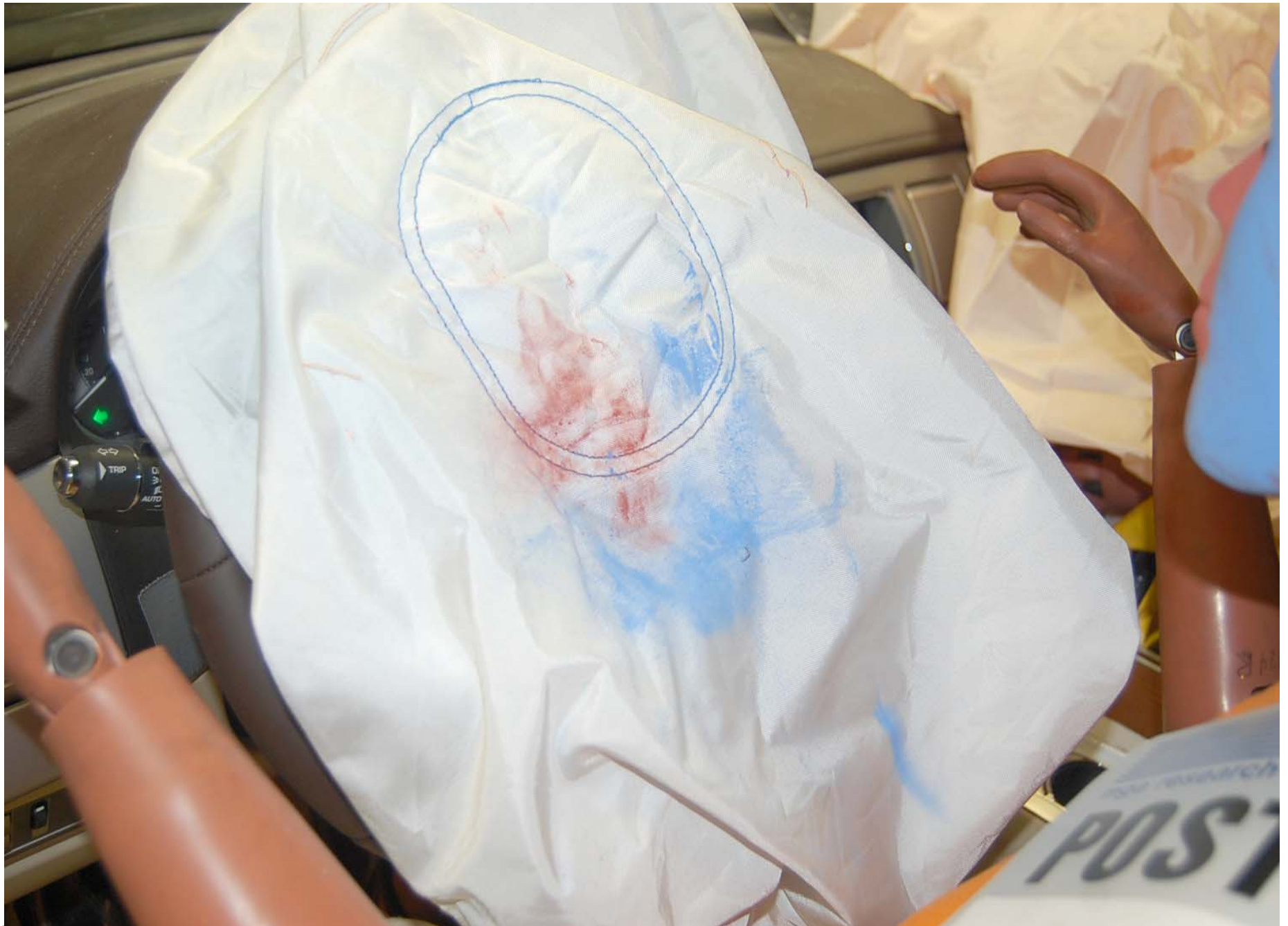
Post-Test Driver Dummy Airbag Contact
