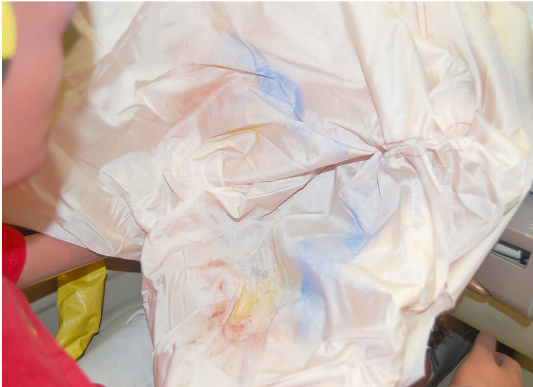
Post-Test Passenger Dummy Airbag Contact View
