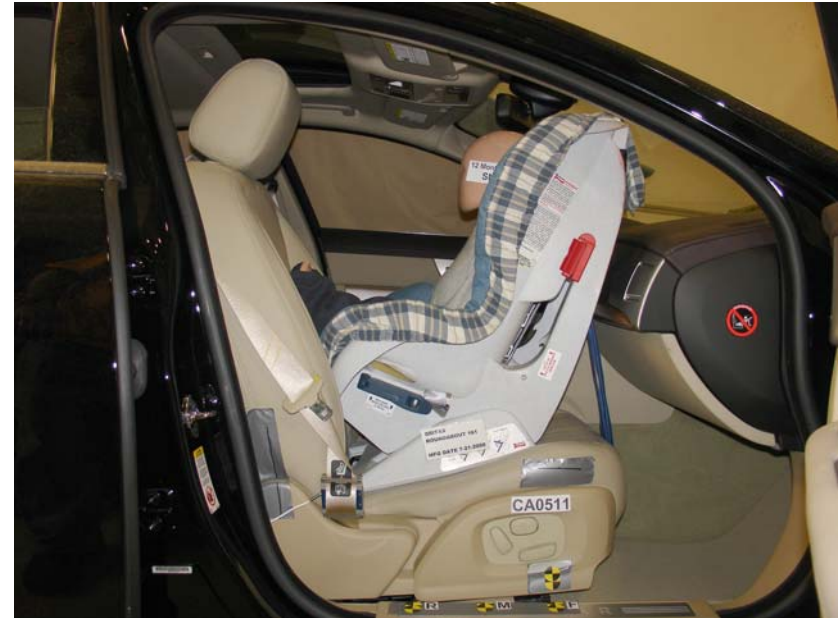
Britax Roundabout 161 Rear Facing Unbelted, Forward Seat Track
