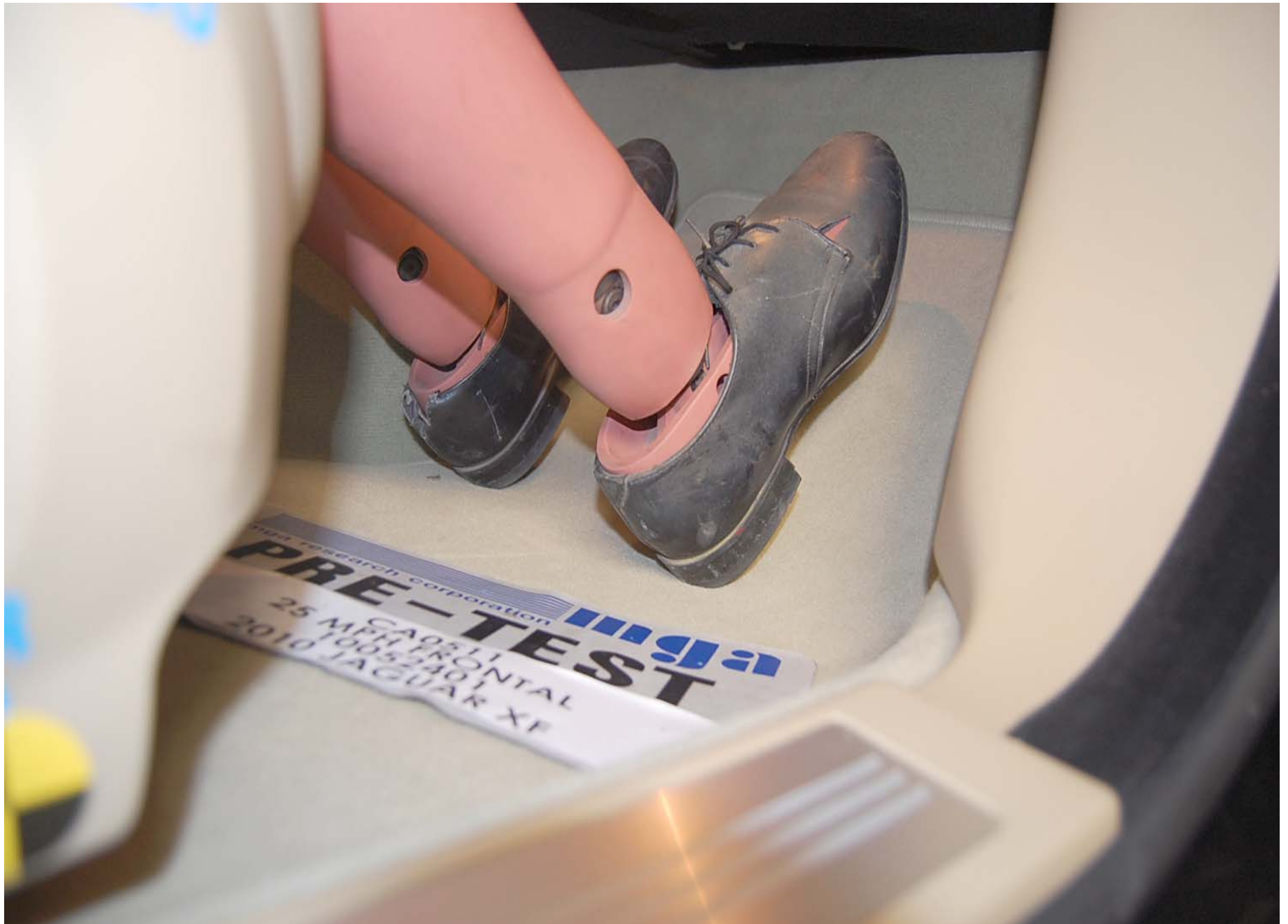
Pre-Test Passenger Dummy Feet Position
