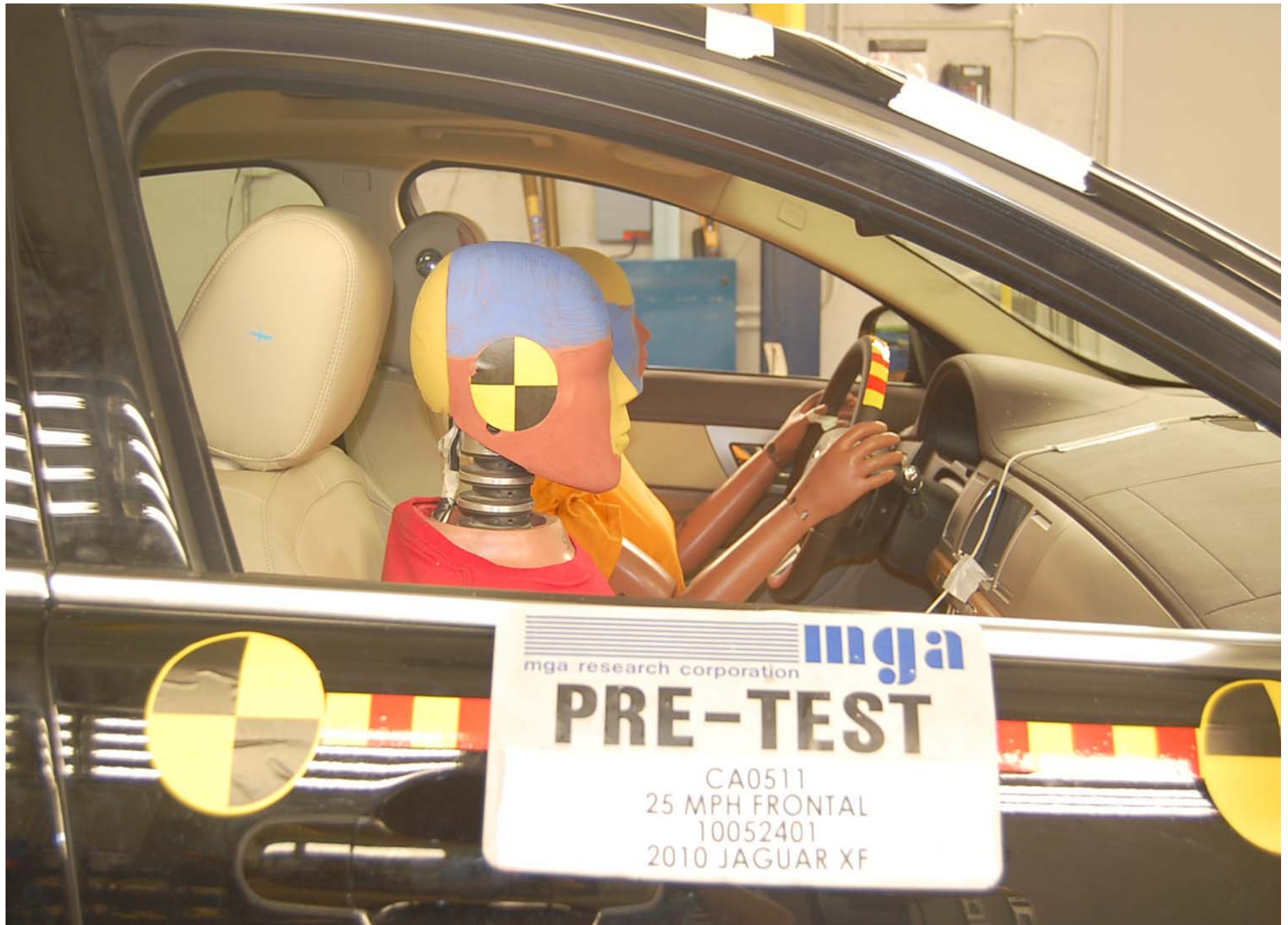
Pre-Test Passenger Dummy Position Right Side View
