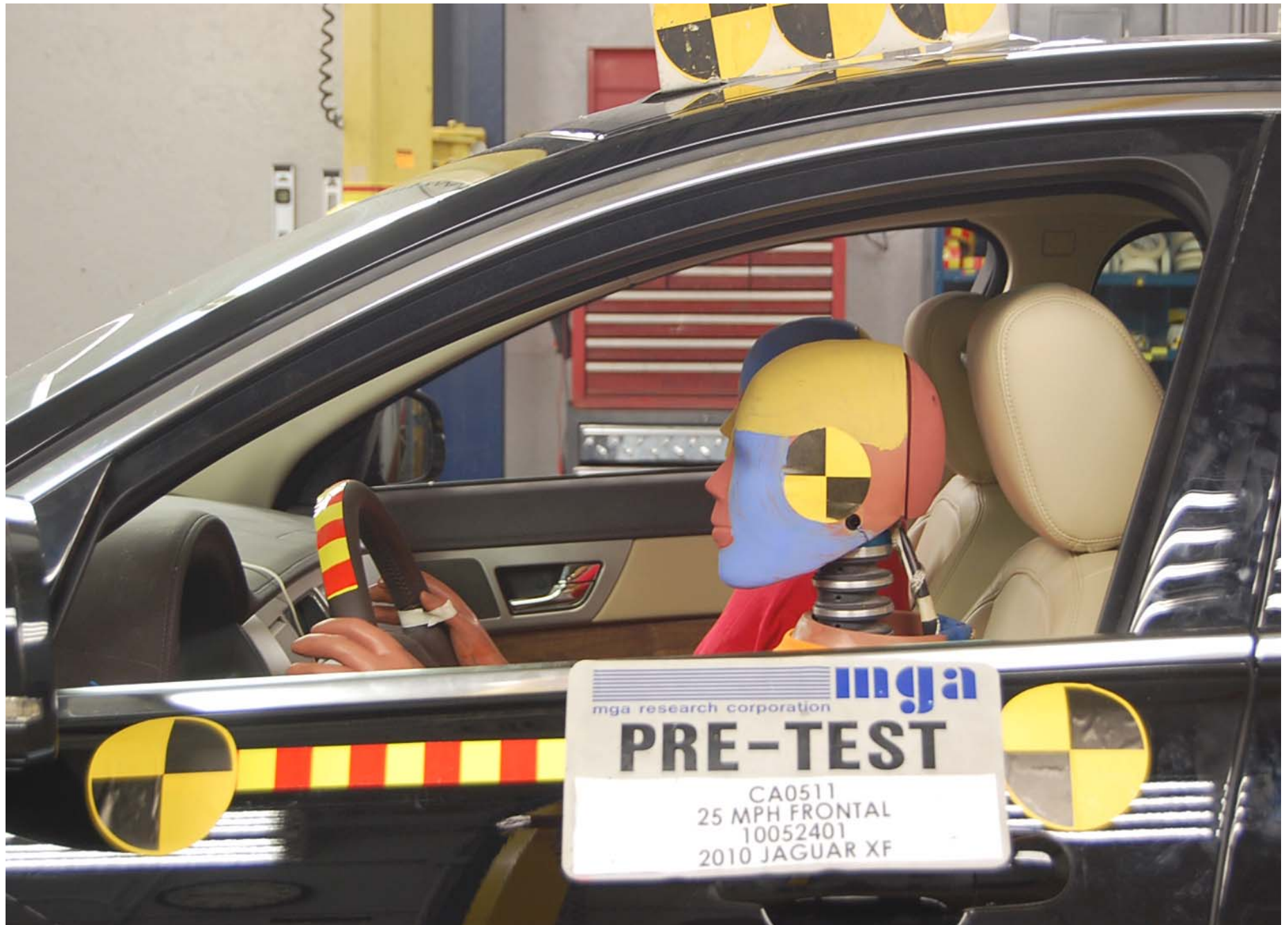
Pre-Test Driver Dummy Position Left Side View
