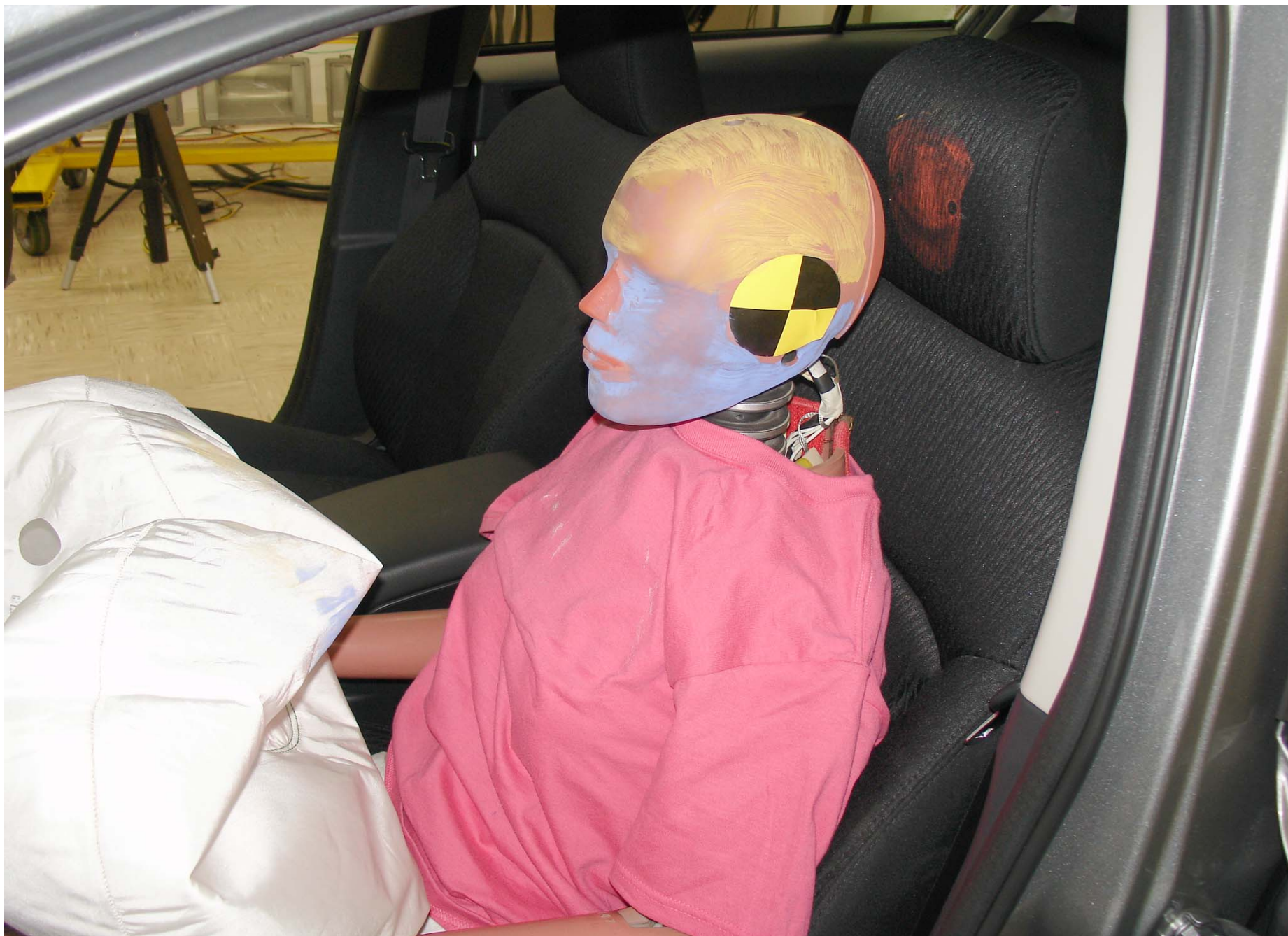
Post-Test 5th Fem. P1 Driver Dummy Head Contact (headrest)
