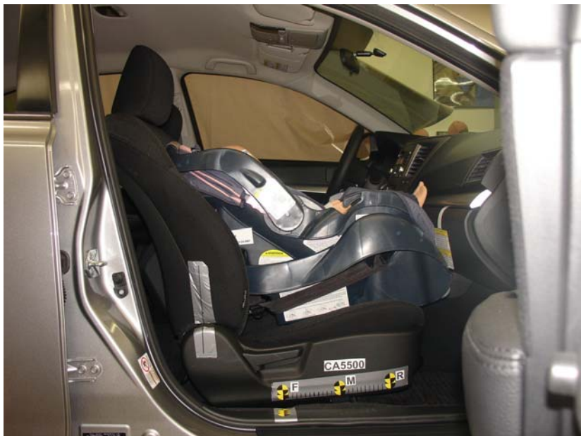
Graco Snugride WBase, Unbelted, Forward Facing, Forward Seat Track
