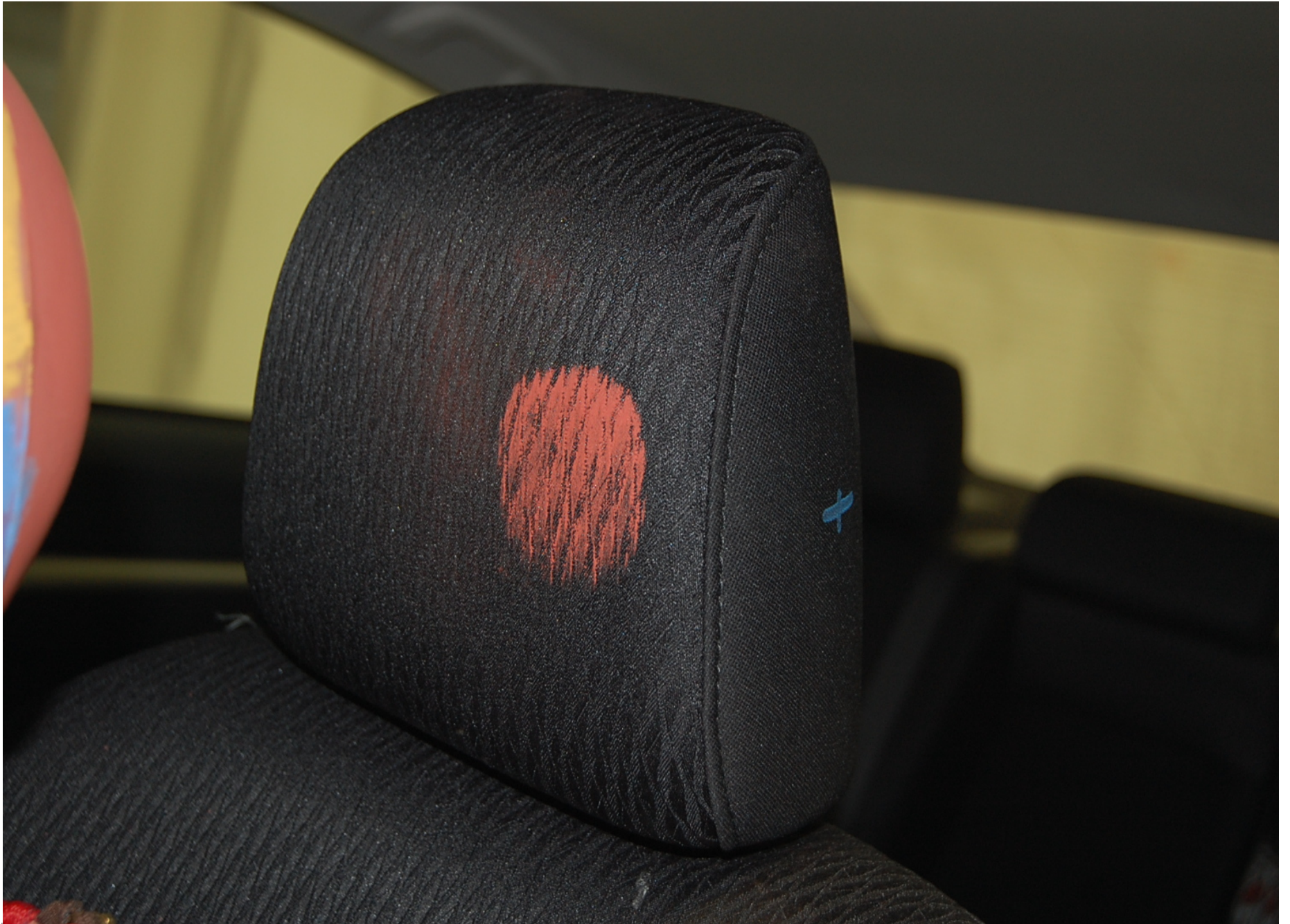
Post-Test Driver Dummy Head Contact (headrest)
