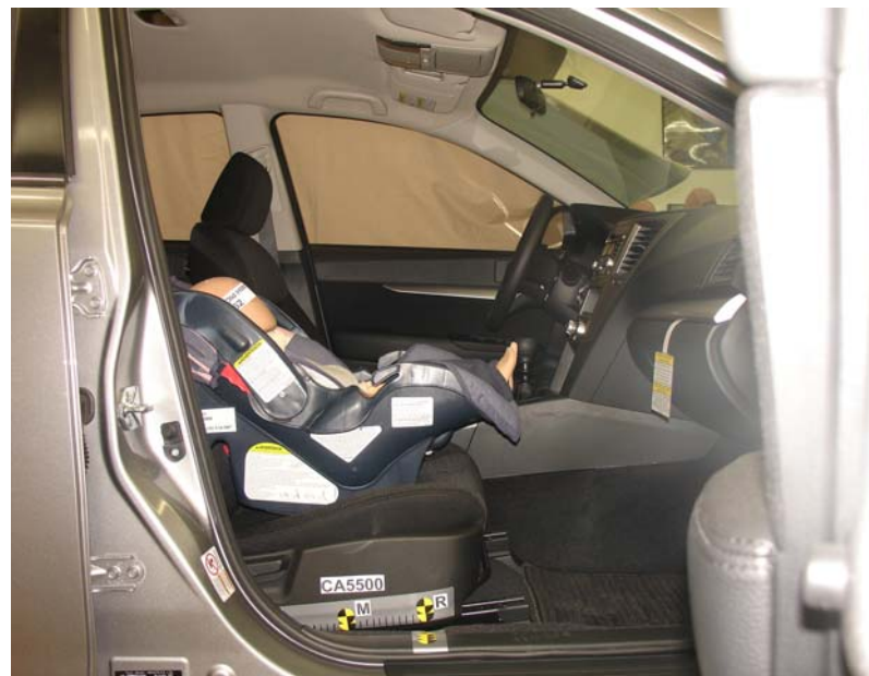
Graco Snugride WOut Base, Unbelted, Forward Facing, Rearward Seat Track
