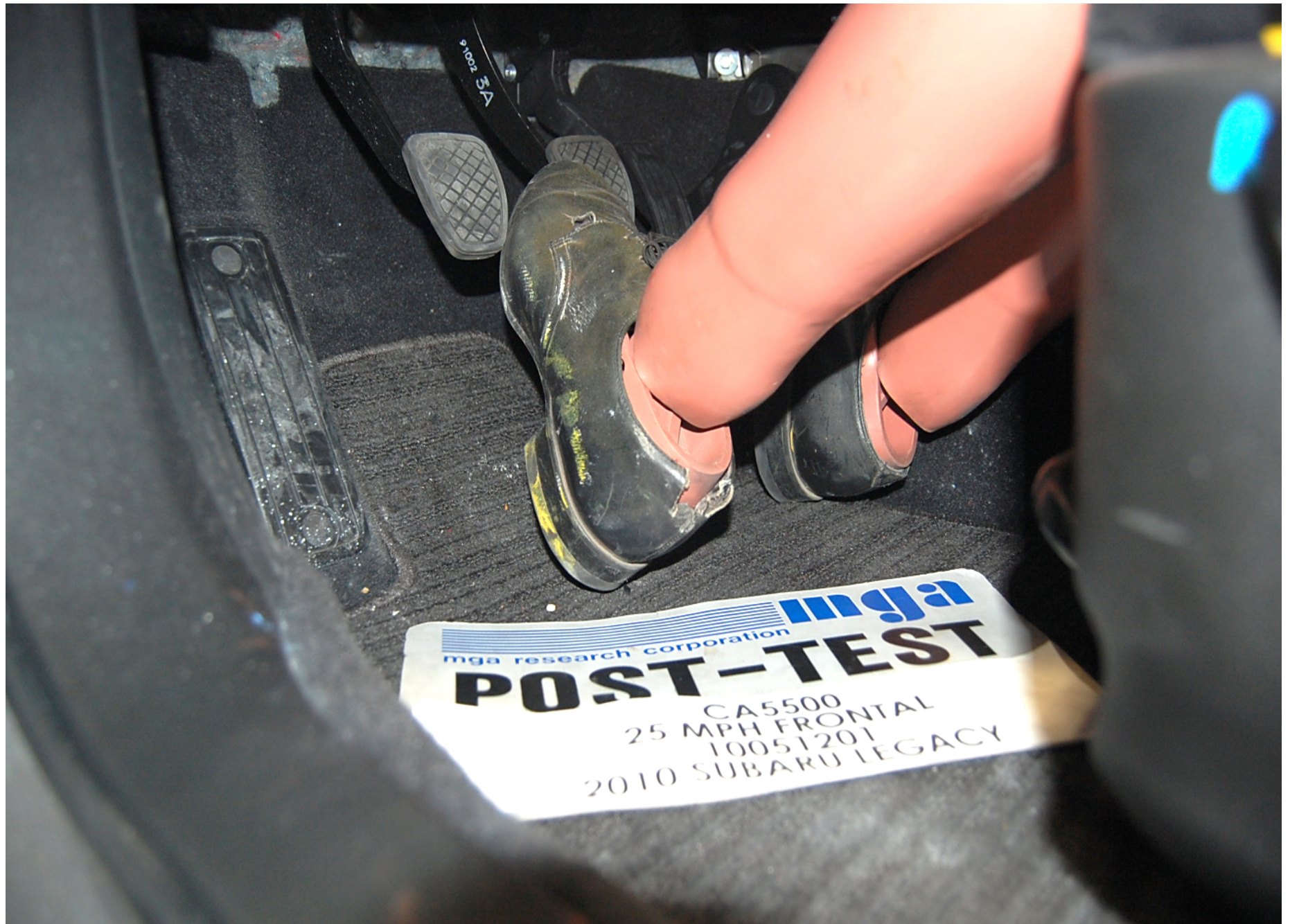
Post-Test Driver Dummy Feet Position
