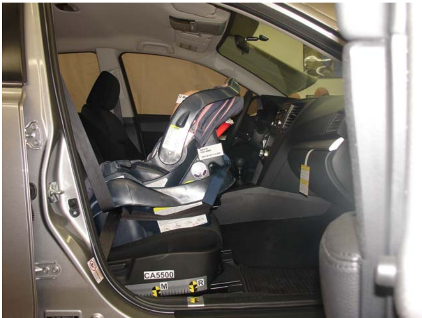
Graco Snugride WBase, Belted, Rear Facing, Rearward Seat Track
