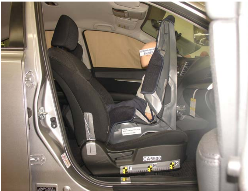
Cosco High Back Booster Rear Facing Unbelted, Forward Seat Track
