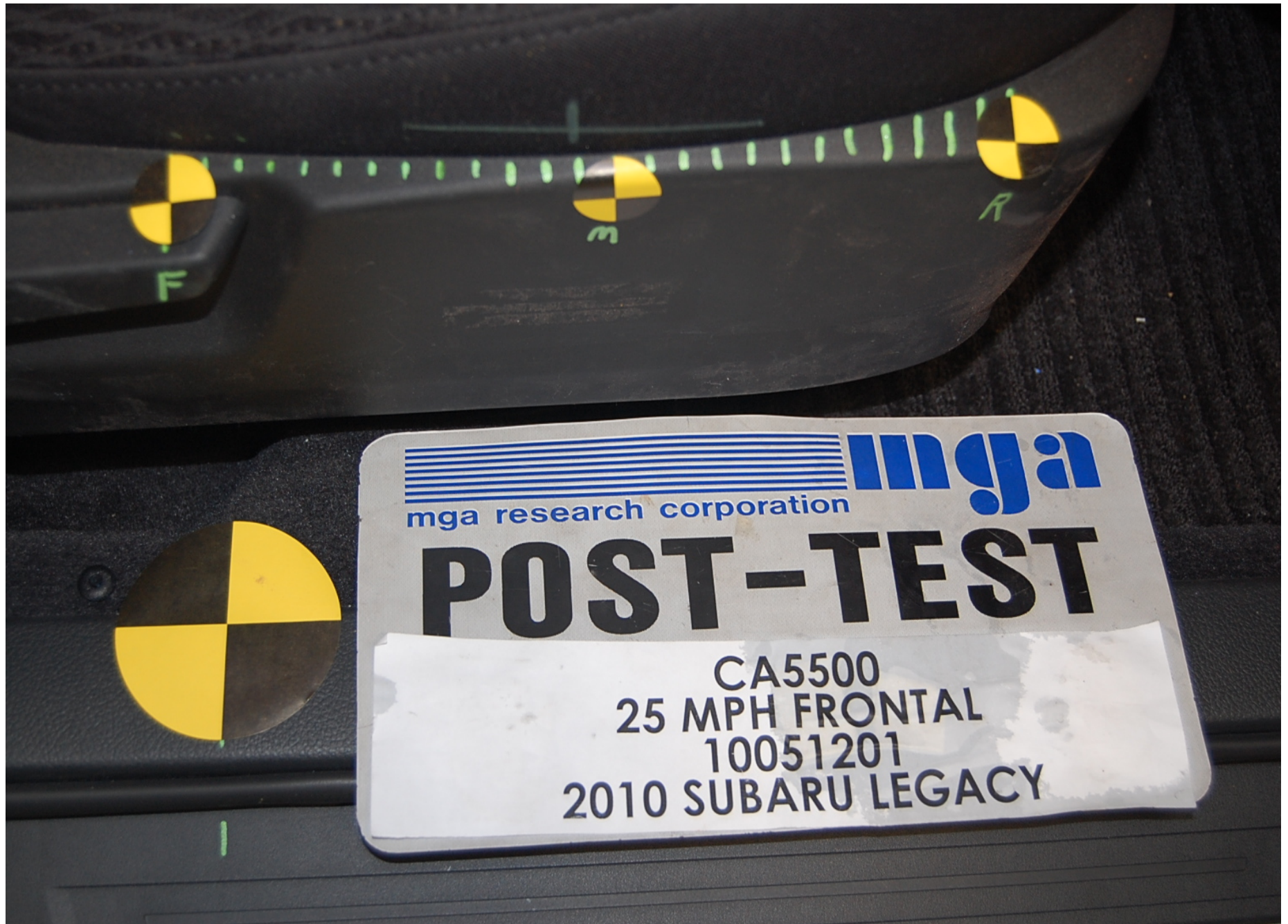
Post-Test Passenger Dummy Seat Position
