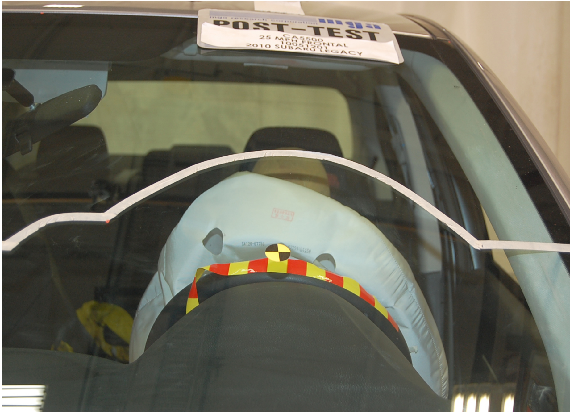
Post-Test Driver Dummy Front View (head position)
