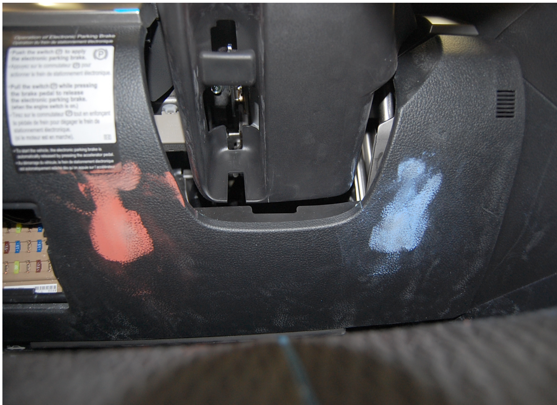
Post-Test Driver Dummy Knee Contact
