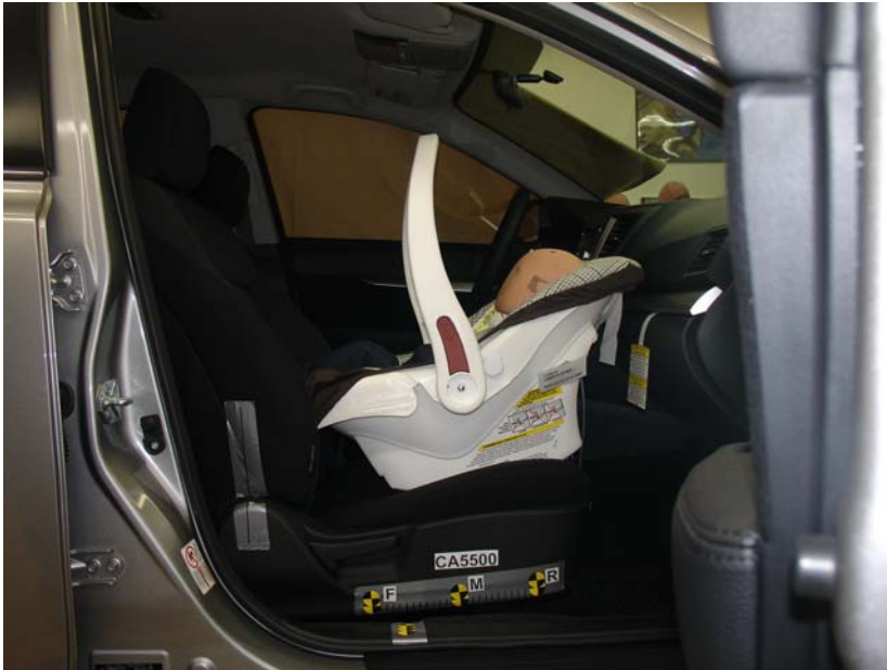
Cosco Arriva WOut Base, Unbelted, Rear Facing, Forward Seat Track
