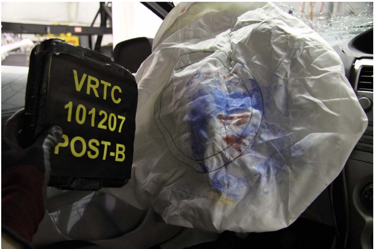
Figure A-186 Post-Test Bullet Vehicle Driver Dummy Head Contact - View 1
