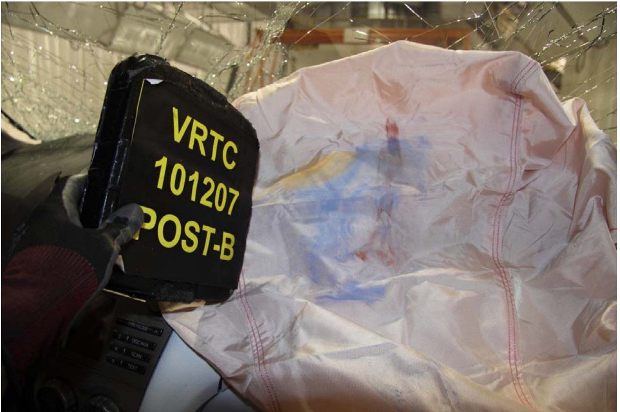
Figure A-195 Post-Test Bullet Vehicle Right Front Passenger Dummy Head Contact-View 1
