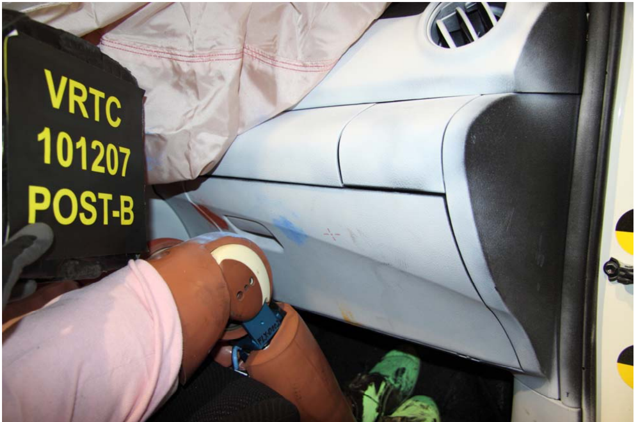
Figure A-197 Post-Test Bullet Vehicle Right Front Passenger Dummy Knee Contact-View 1
