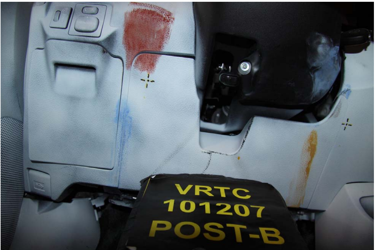
Figure A-188 Post-Test Bullet Vehicle Driver Dummy Knee Contact - View 2
