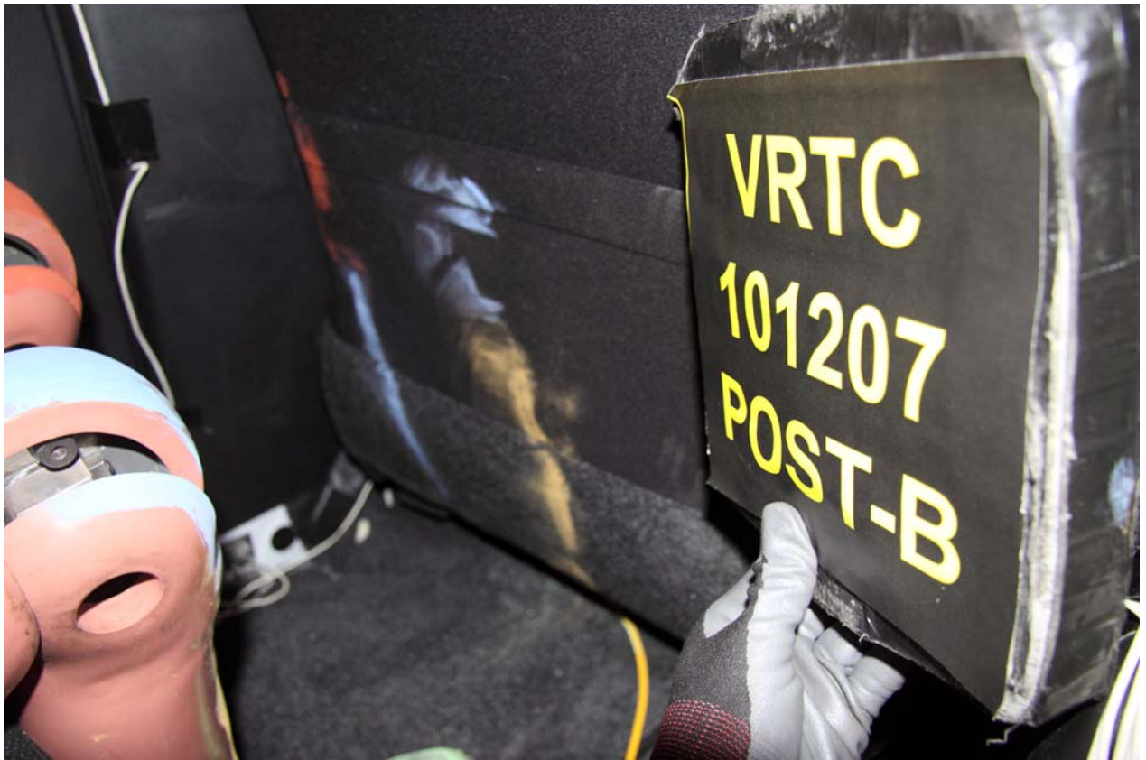
Figure A-207 Post-Test Bullet Vehicle Left Rear Passenger Dummy Knee Contact - View 1
