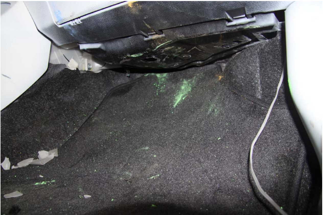
Figure A-202 Post-Test Bullet Vehicle Right Front Passenger Dummy Floorpan Contacts-View 1
