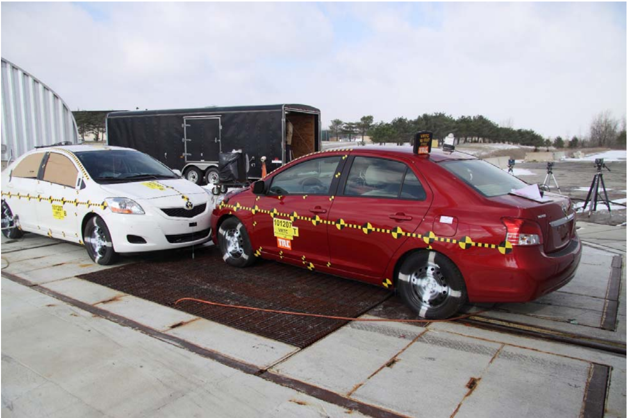
Figure A-13 Pre-Test Impact Alignment – View 1
