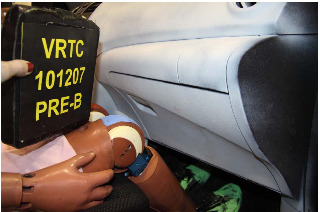
Figure A-159 Pre-Test Bullet Vehicle Right Front Passenger Dummy Knee Bolster with ATD View 1
