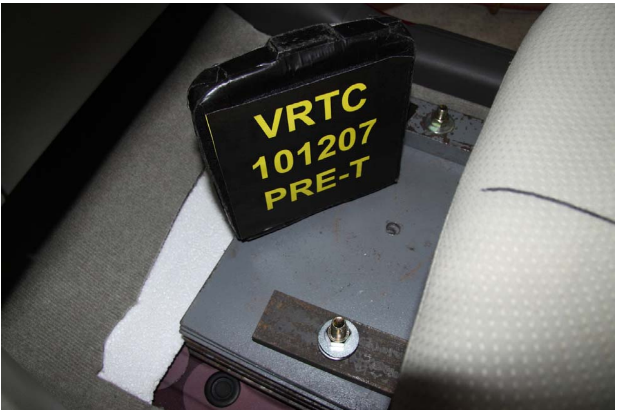
Figure A-217 Pre-Test Target Vehicle Ballast Position View
