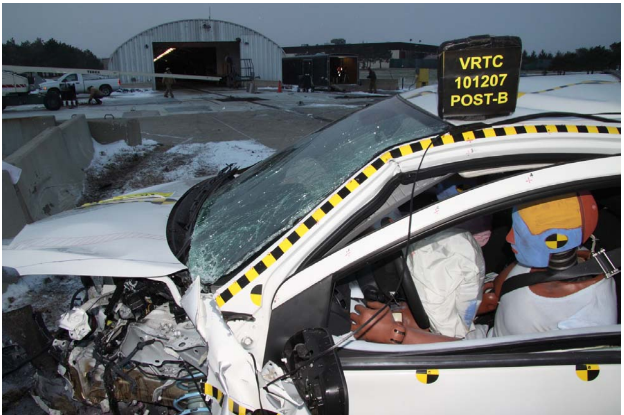
Figure A-130 Post-Test Bullet Vehicle Driver Dummy - View 1
