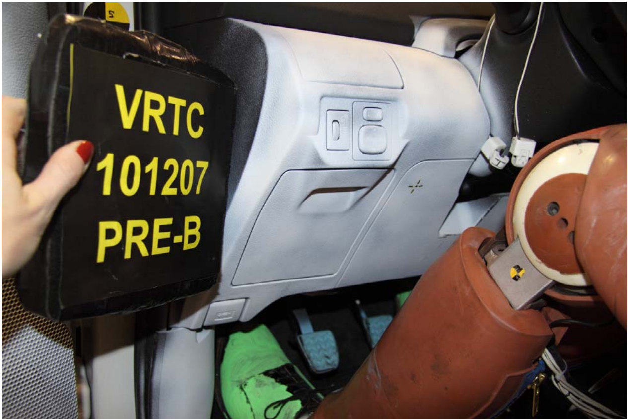
Figure A-137 Pre-Test Bullet Vehicle Driver Dummy Knee Bolster with ATD - View 1
