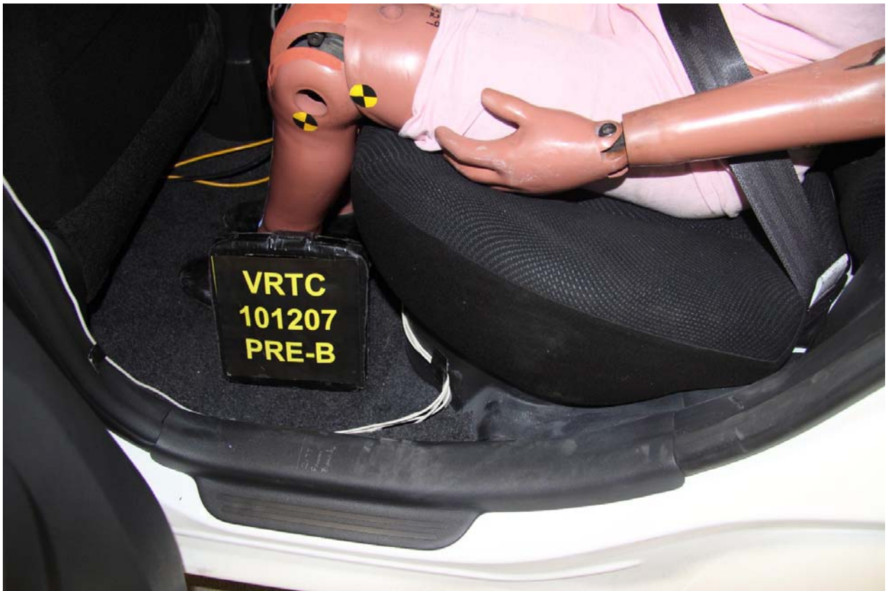
Figure A-176 Pre-Test Bullet Vehicle Left Rear Passenger Knee To Seat Back Position View
