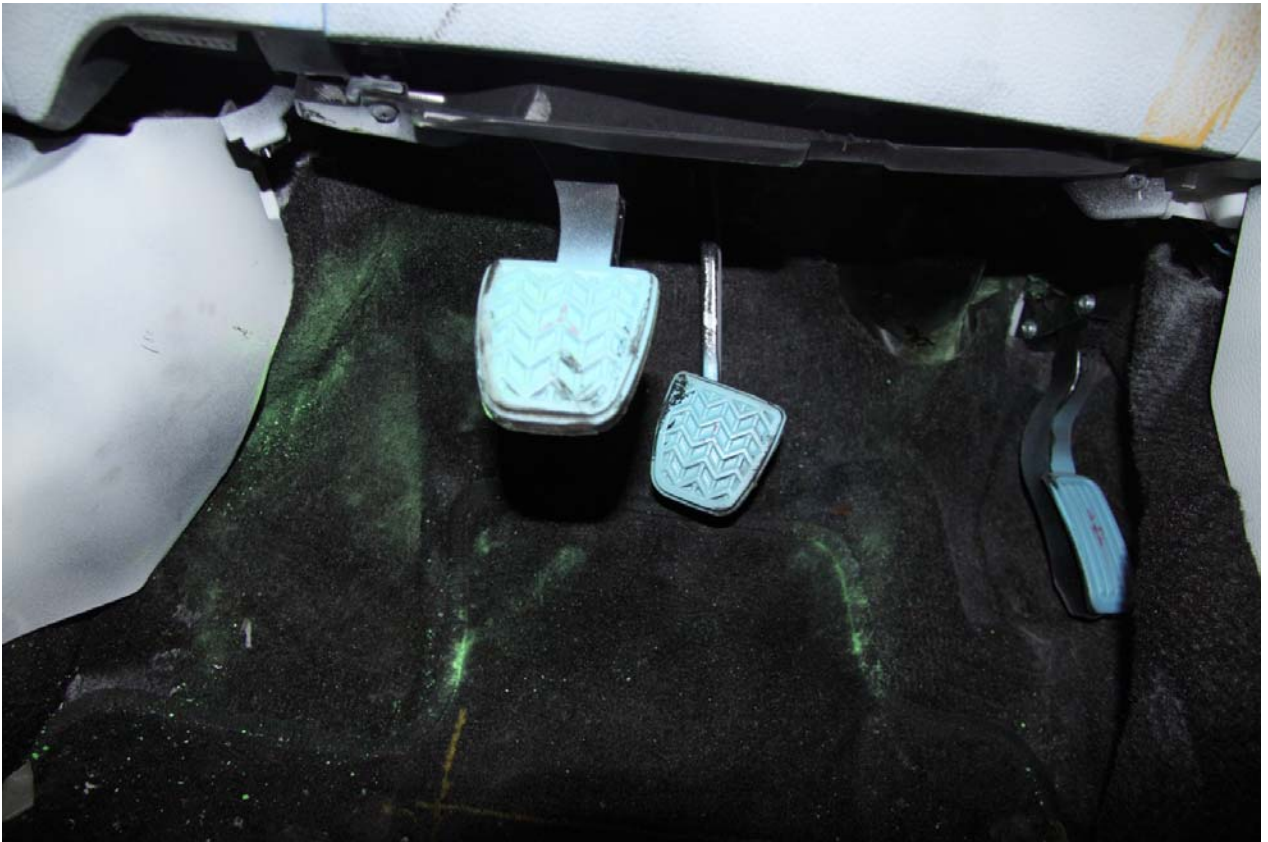
Figure A-191 Post-Test Bullet Vehicle Driver Dummy Floorpan Feet Contacts – View 2
