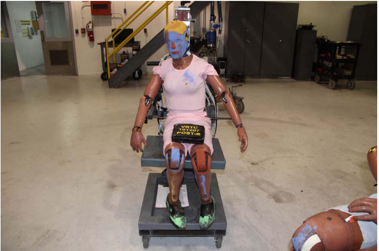
Figure A-205 Post-Test Bullet Vehicle Left Rear Passenger Dummy Overall Contact View
