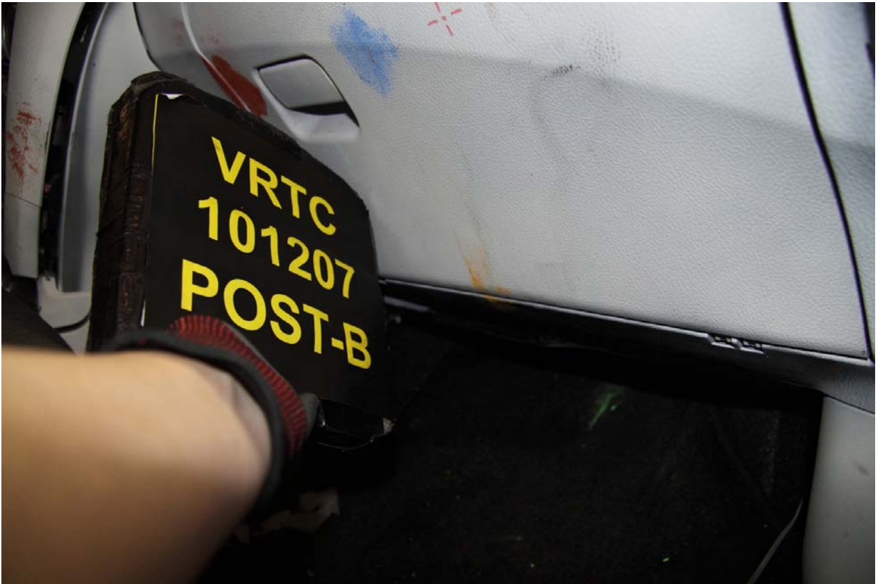
Figure A-199 Post-Test Bullet Vehicle Right Front Passenger Dummy Knee Contact-View 3
