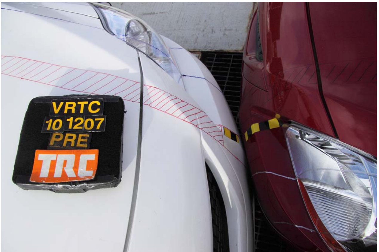
Figure A-8 Pre-Test Overhead Impact Alignment View
