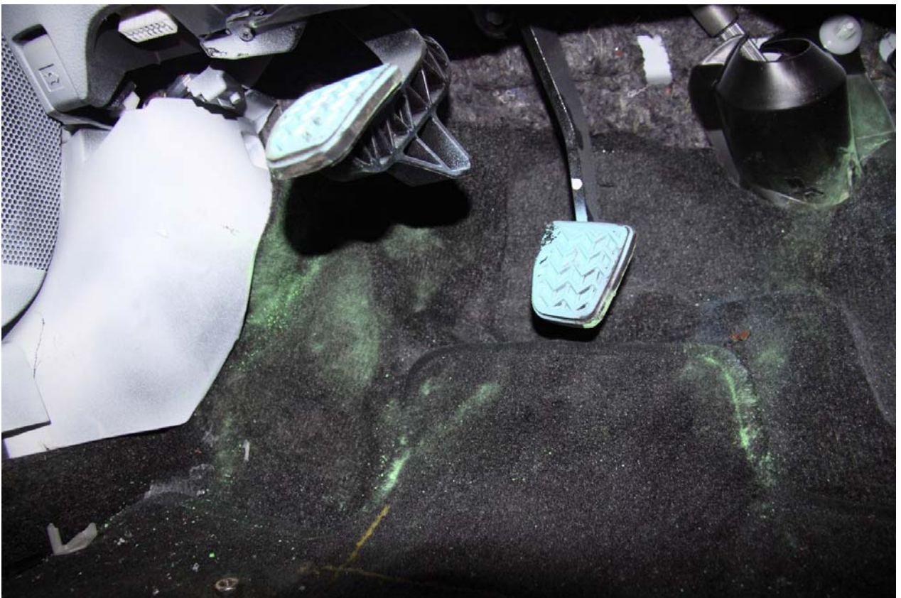
Figure A-190 Post-Test Bullet Vehicle Driver Dummy Floorpan Feet Contacts – View 1
