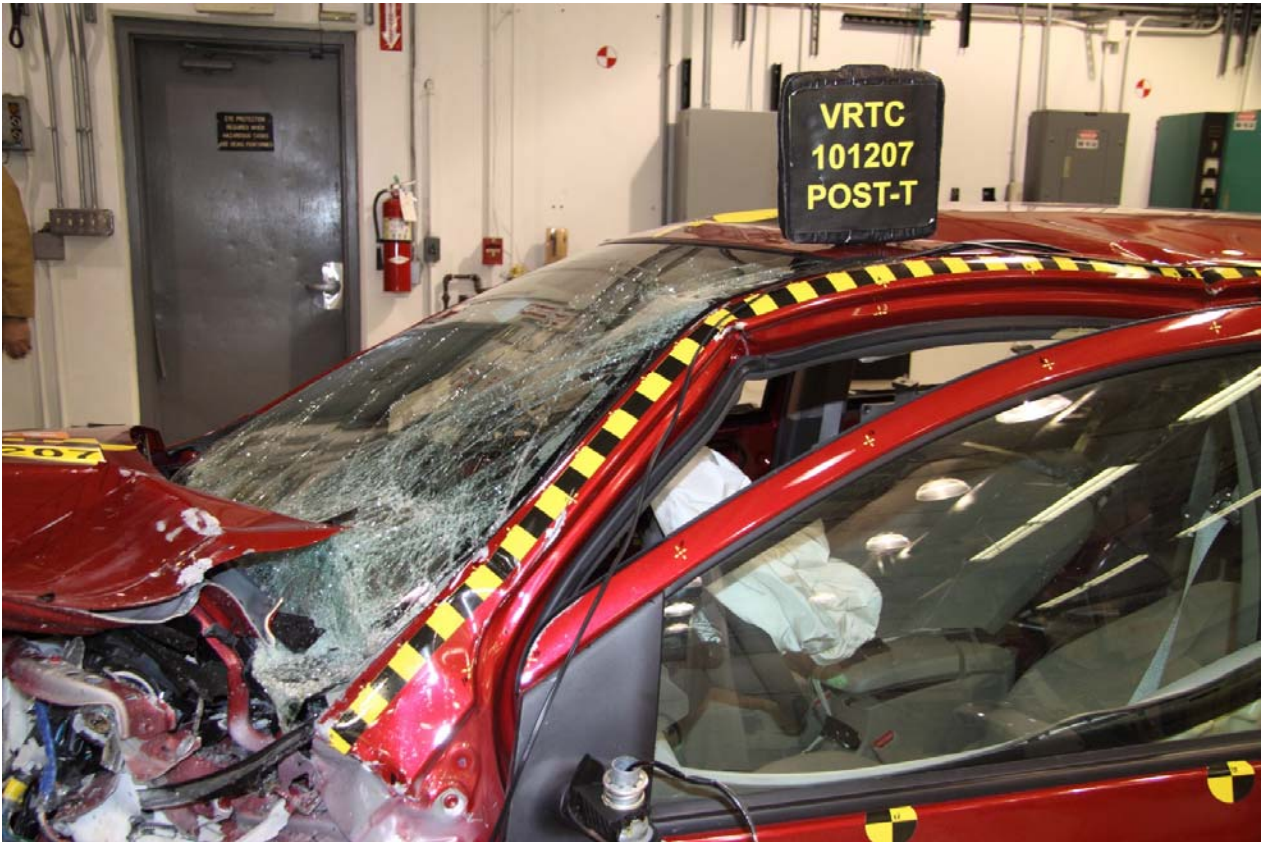
Figure A-220 Post-Test Target Vehicle Damage – View 1
