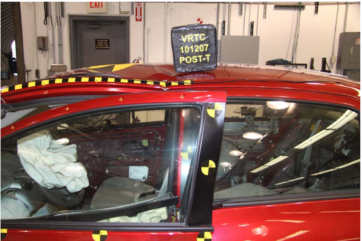
Figure A-221 Post-Test Target Vehicle Damage – View 2
