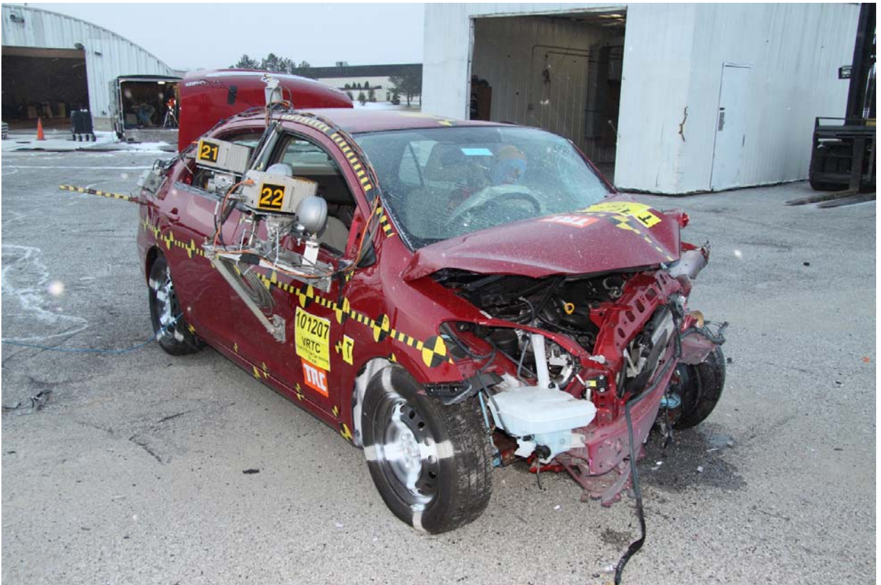
Figure A-32 Post-Test Target Vehicle Right Front View
