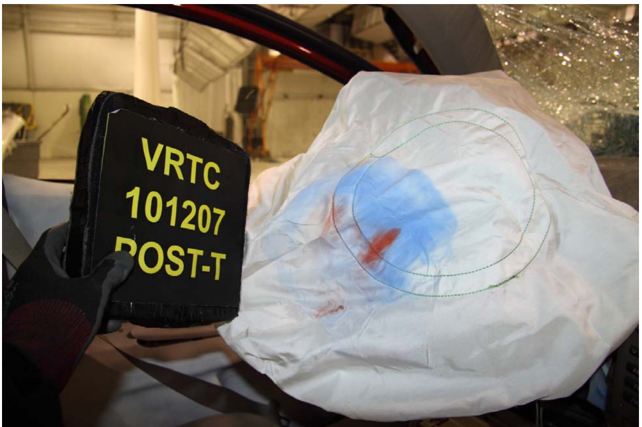
Figure A-178 Post-Test Target Vehicle Driver Dummy Head Contact View
