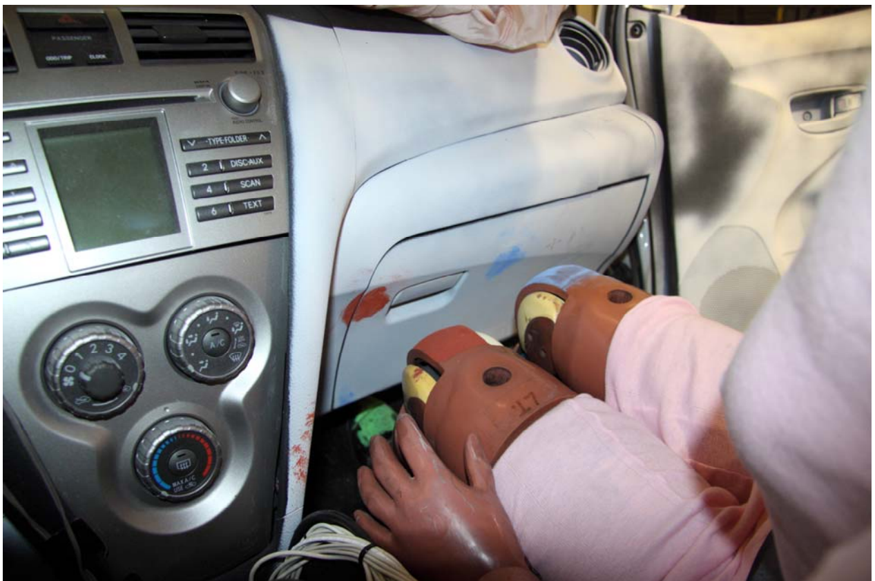
Figure A-198 Post-Test Bullet Vehicle Right Front Passenger Dummy Knee Contact-View 2
