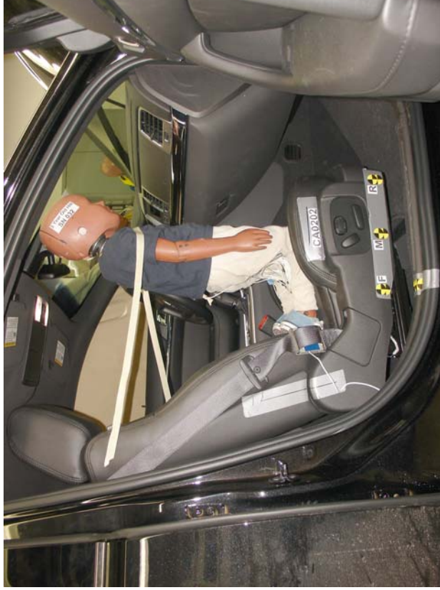
3-Year-Old Unbelted, Forward Seat Track, Position 6
