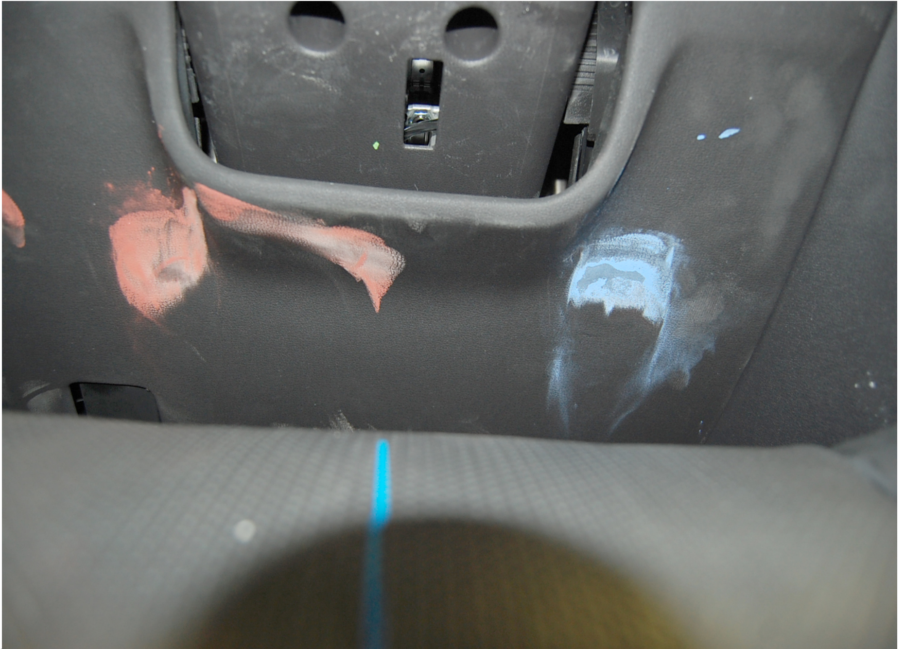
Post-Test Driver Dummy Knee Contact
