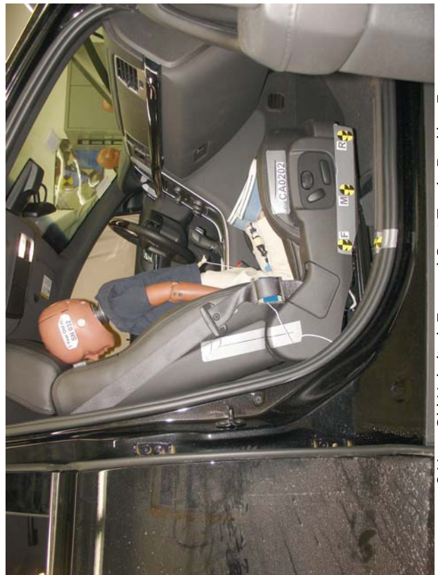
3-Year-Old Unbelted, Forward Seat Track, Position 7
