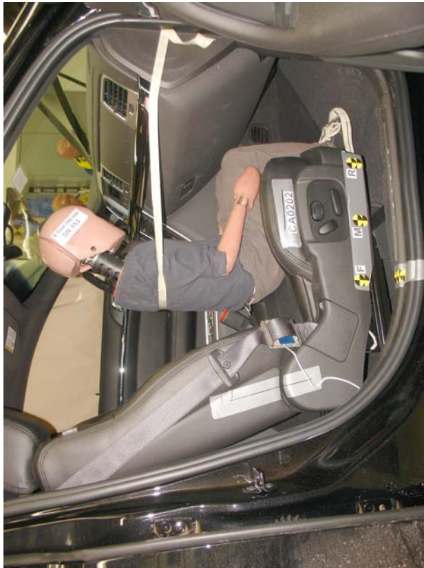
6-Year-Old Unbelted, Forward Seat Track, Position 3
