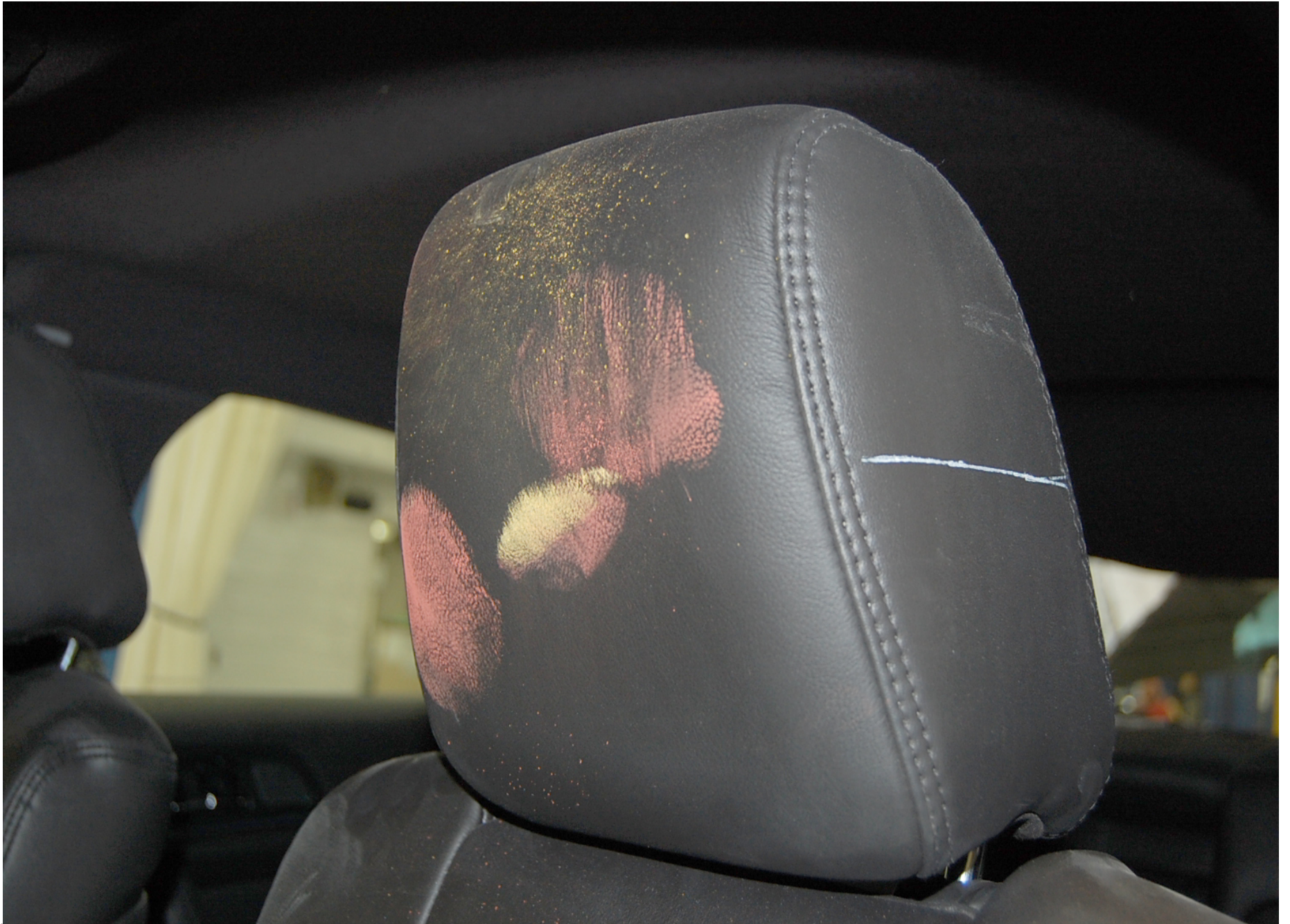
Post-Test Driver Dummy Head Contact (headrest)
