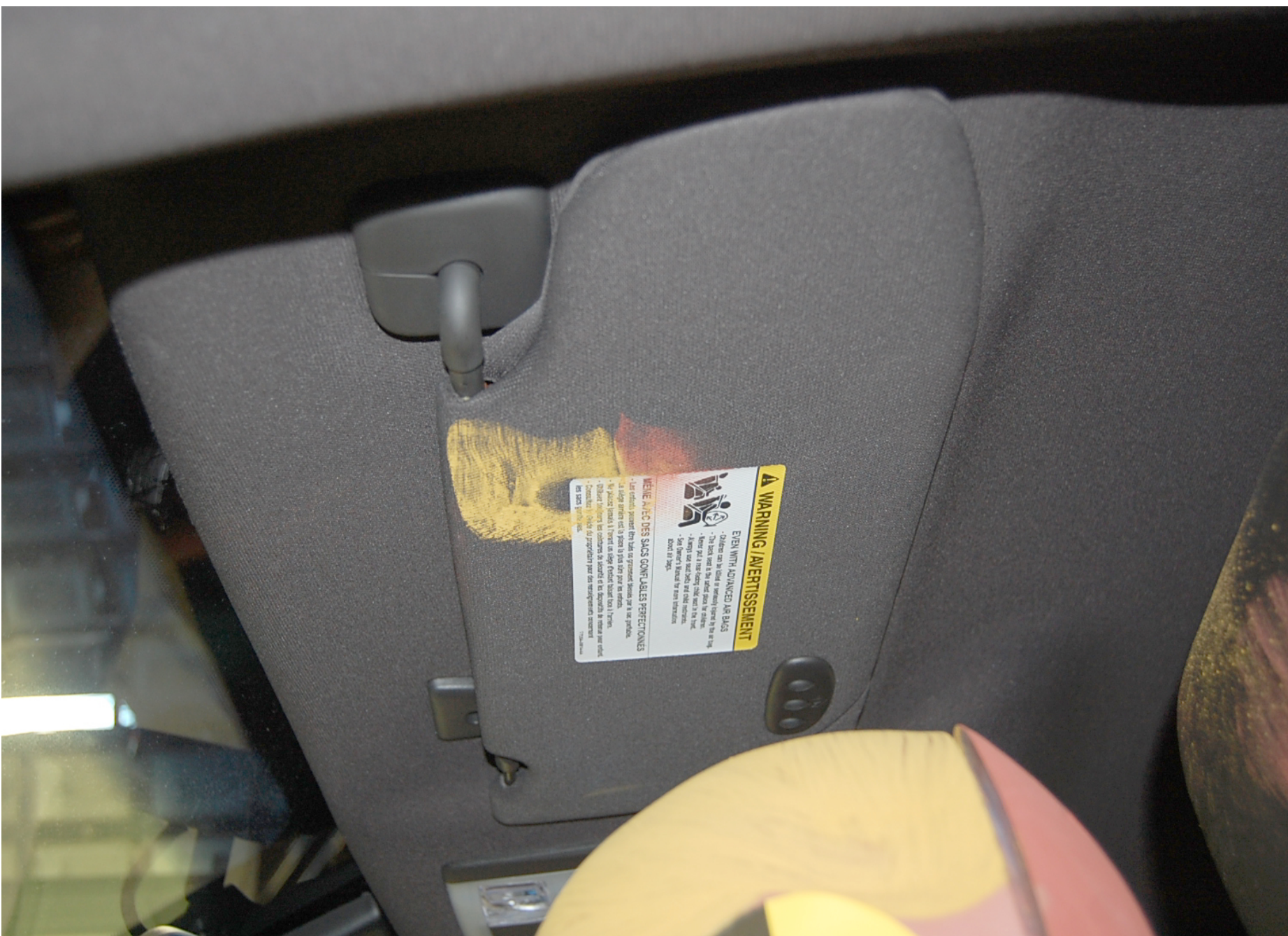
Post-Test Driver Dummy Head Contact (visor)
