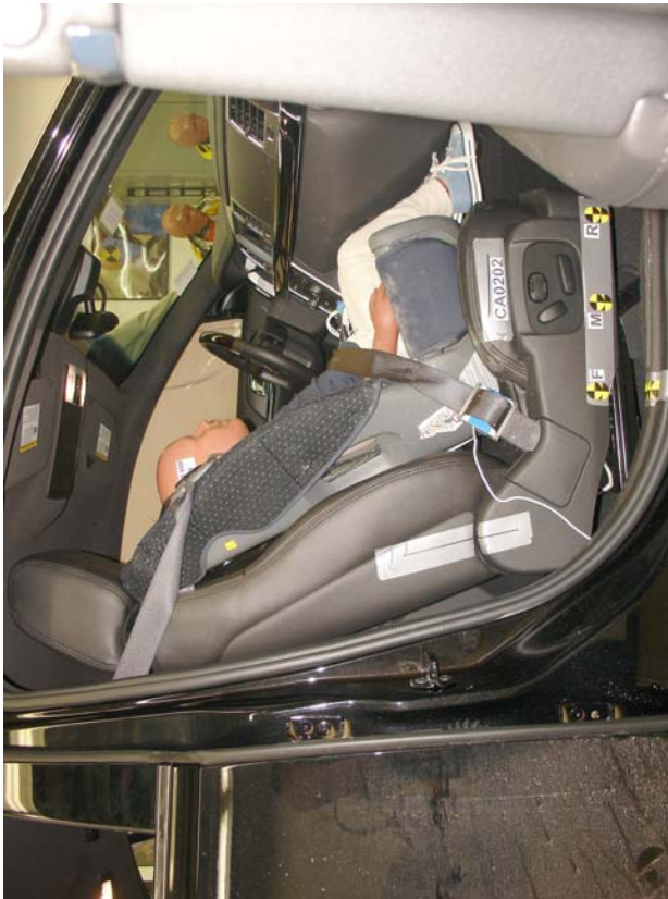
3-Year-Old Century Next Step Belted, Forward Seat Track
