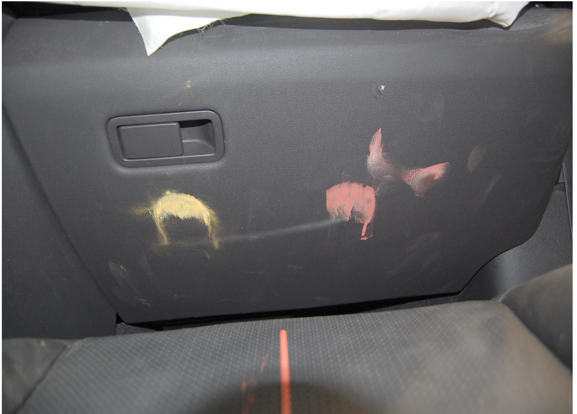
Post-Test Passenger Dummy Knee Contact
