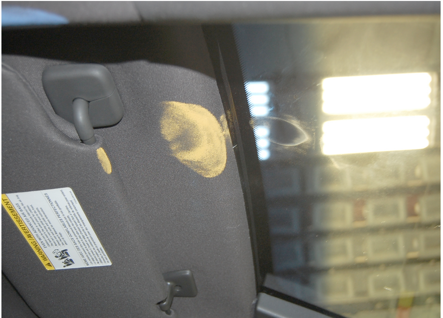
Post-Test Passenger Dummy Head Contact (windshield/header)
