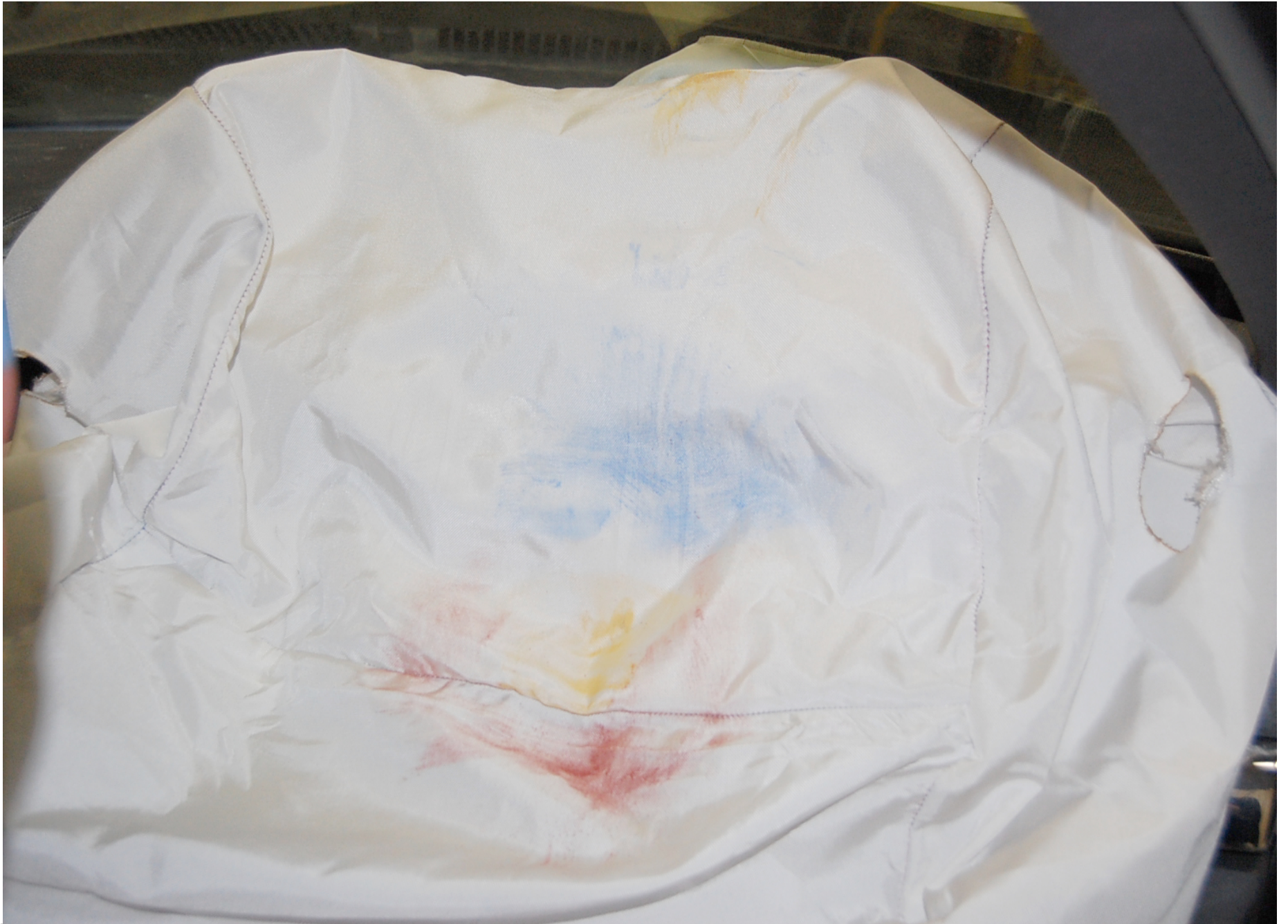
Post-Test Passenger Dummy Airbag Contact
