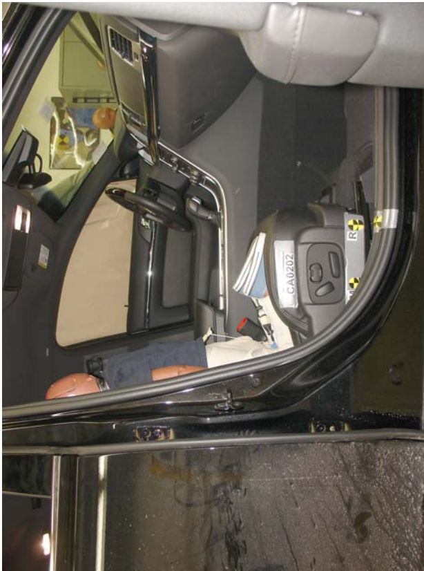
3-Year-Old Unbelted, Rearward Seat Track, Position 7
