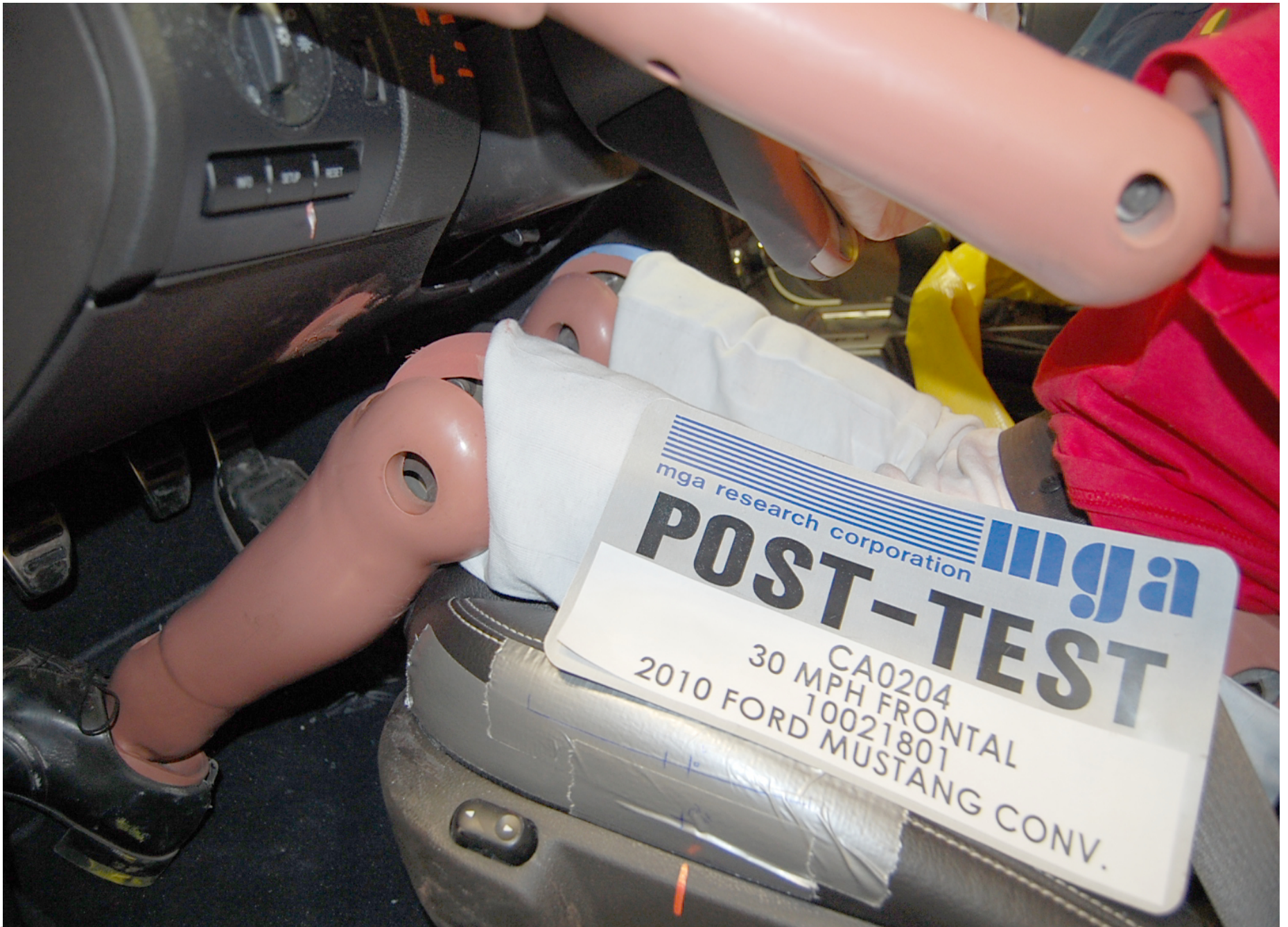
Post-Test Driver Side Knee Bolster View
