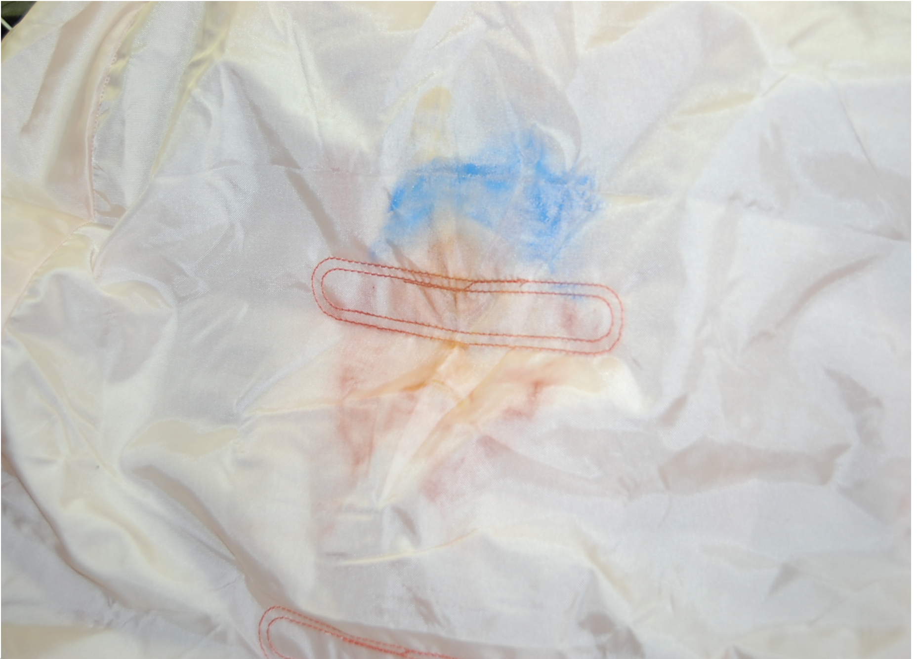
Post-Test Passenger Dummy Airbag Contact
