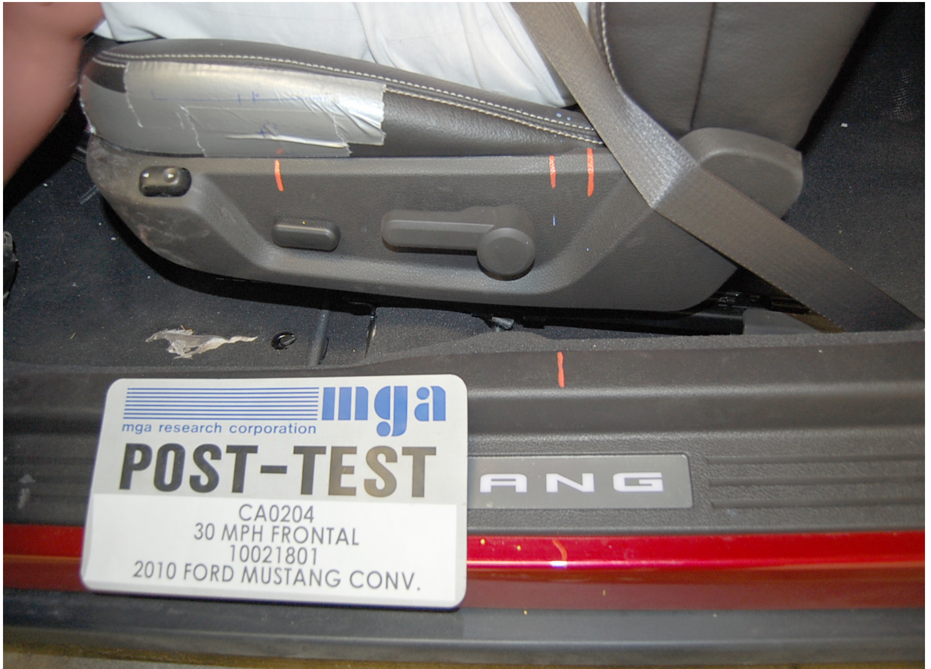
Post-Test Driver Dummy Seat Position
