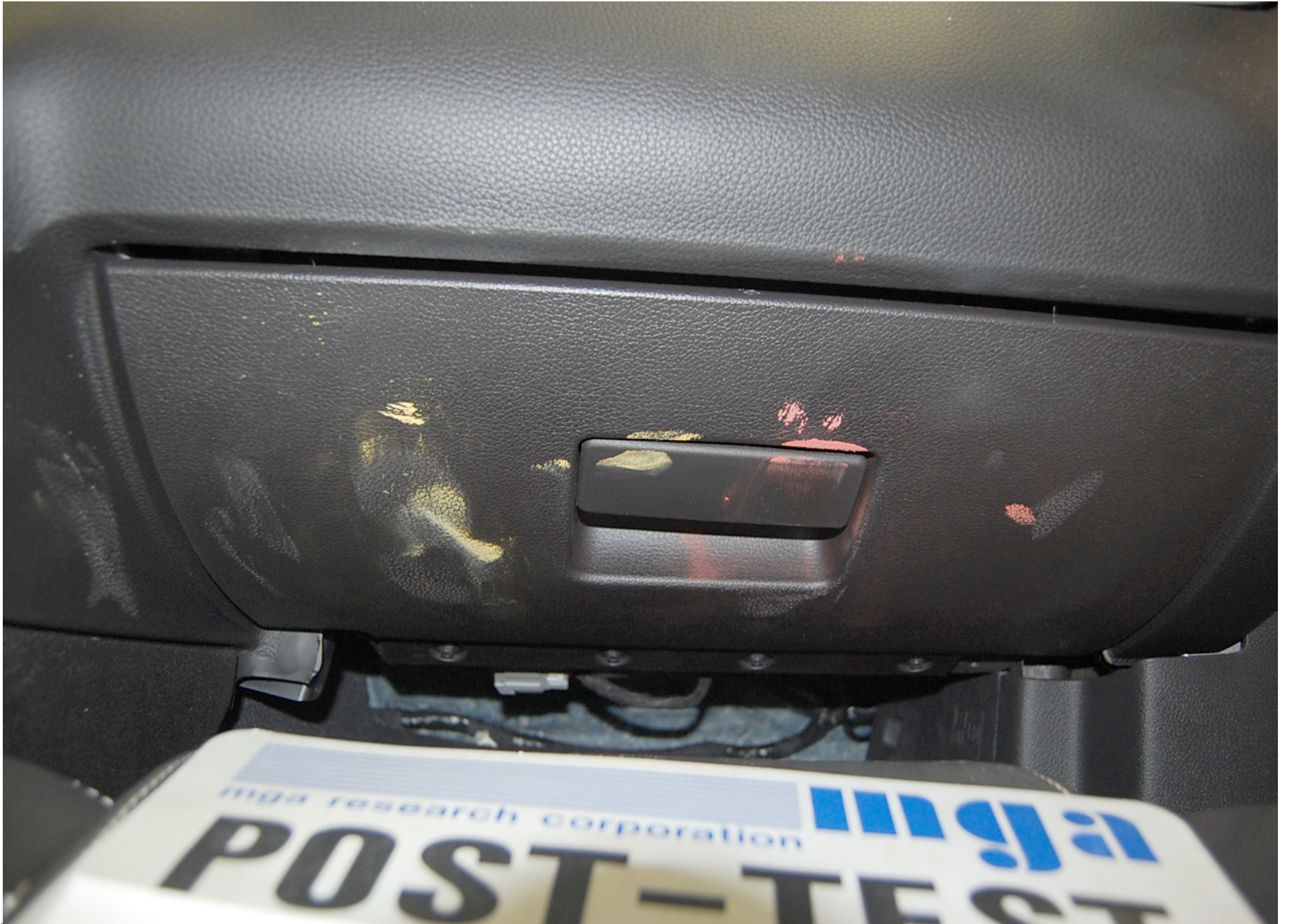
Post-Test Passenger Dummy Knee Contact
