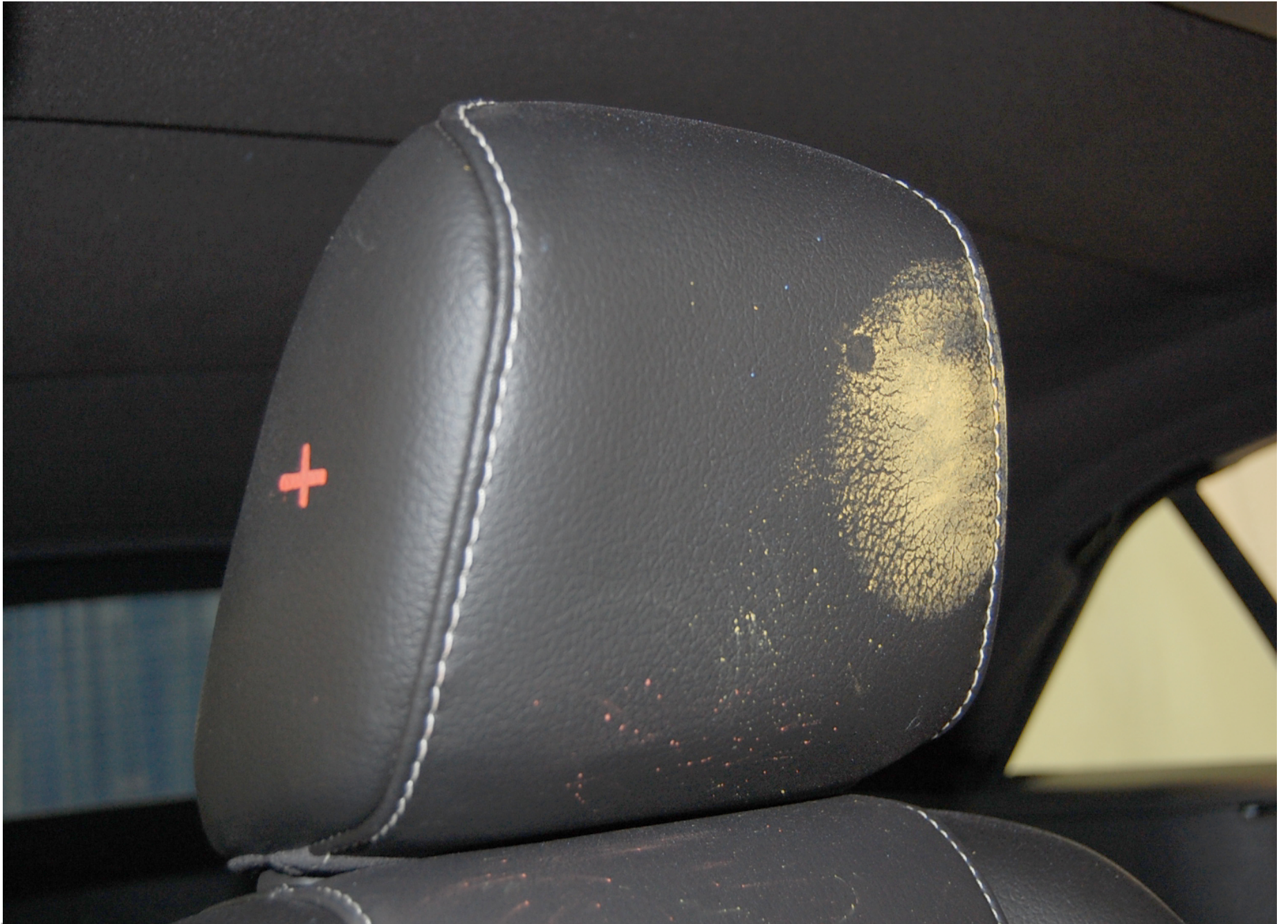
Post-Test Passenger Dummy Head Contact (headrest)
