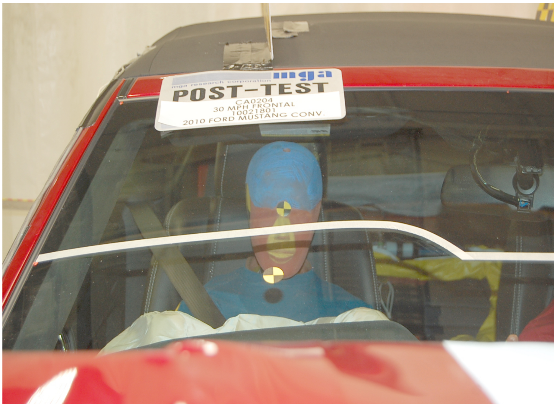
Post-Test Passenger Dummy Front View (head position)
