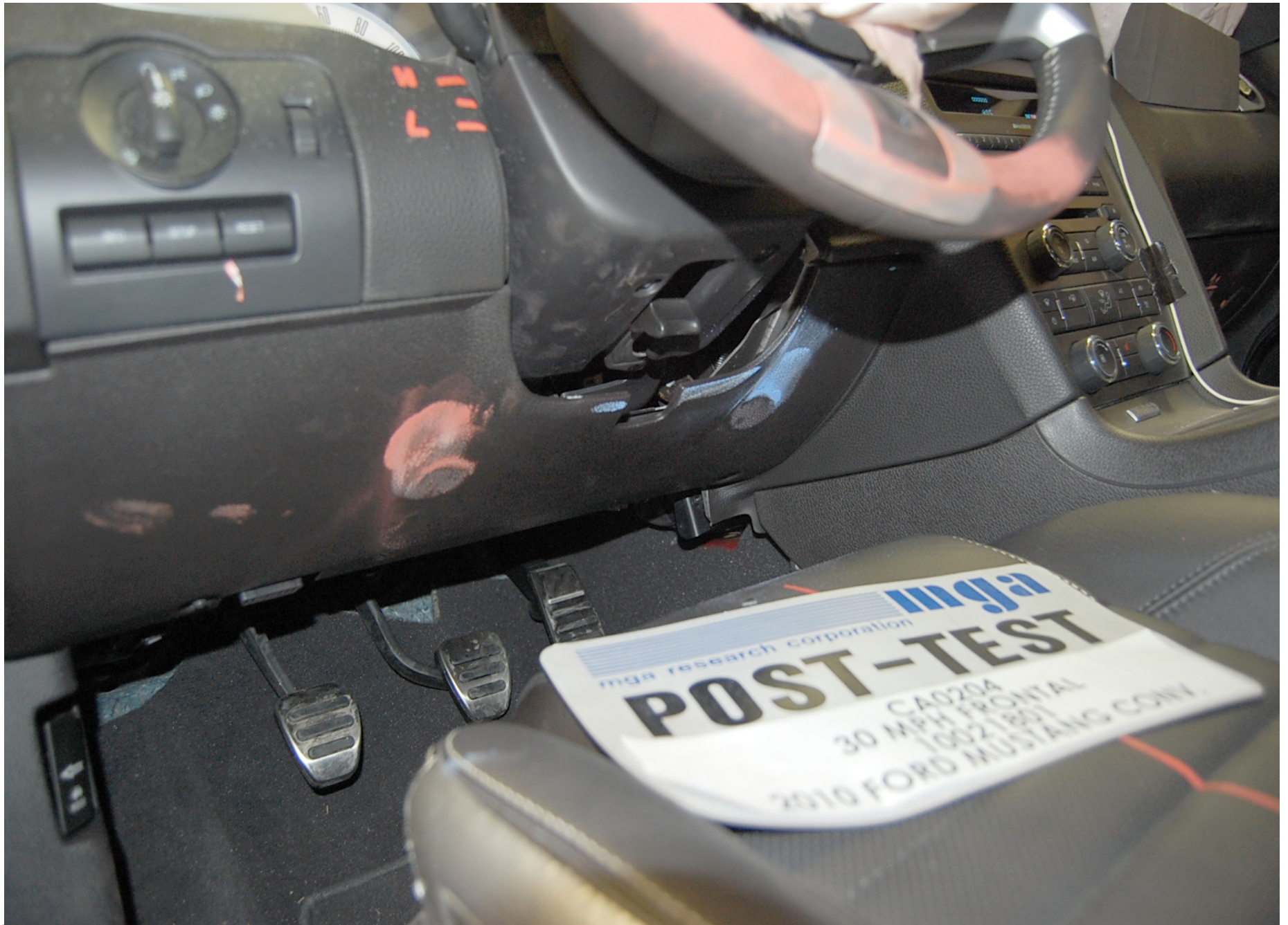
Post-Test Driver Dummy Knee Contact
