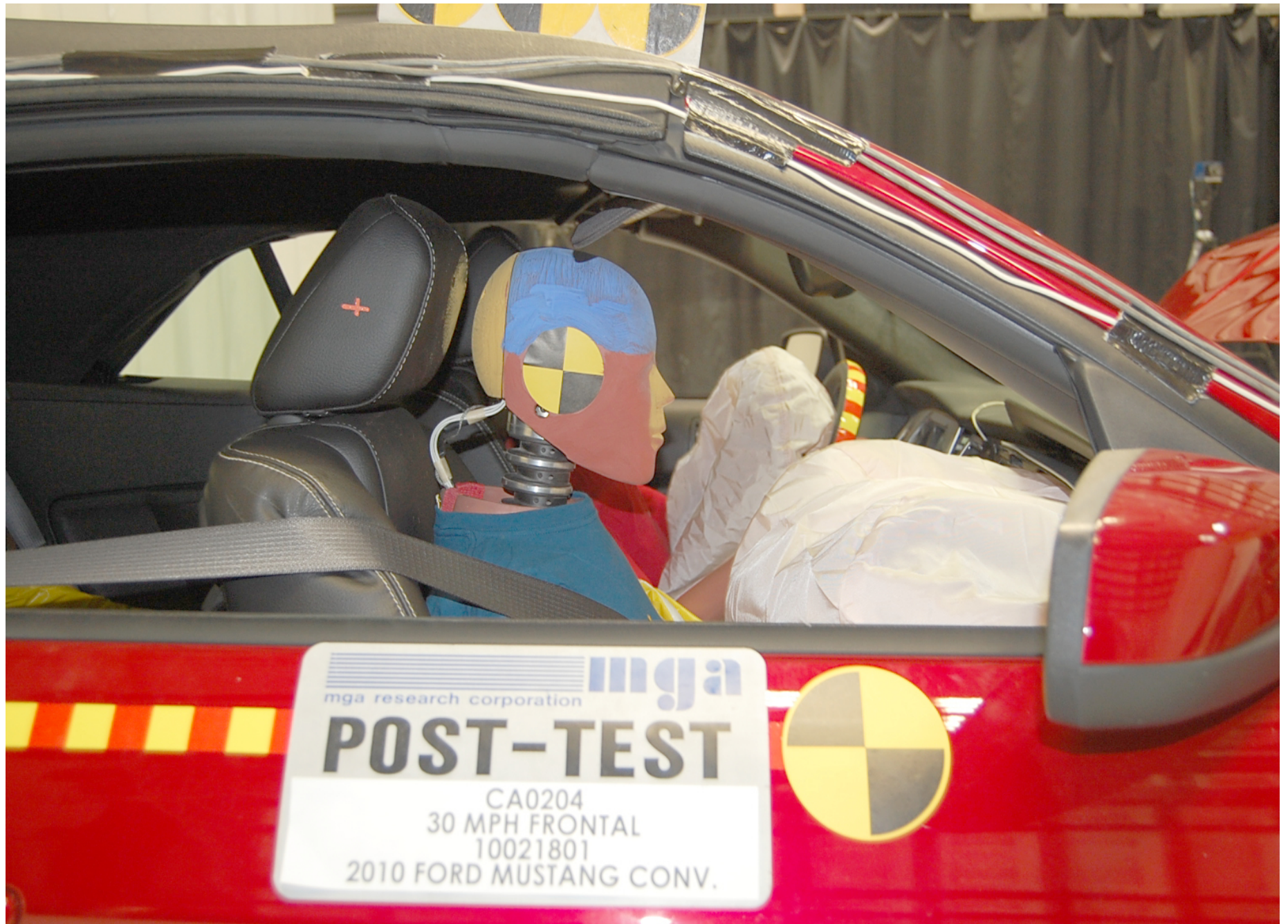
Post-Test Passenger Dummy Position Right Side View
