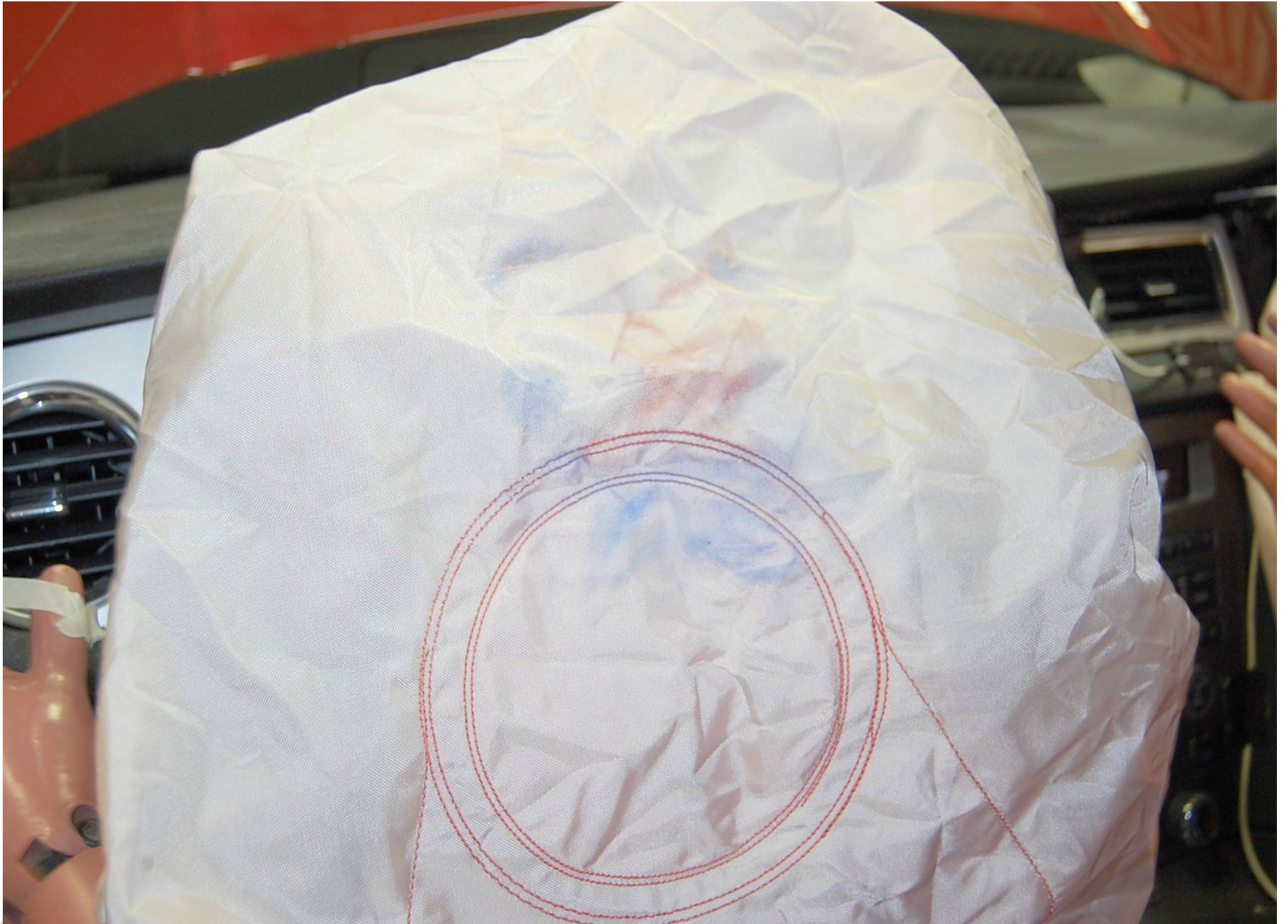
Post-Test Driver Dummy Airbag Contact
