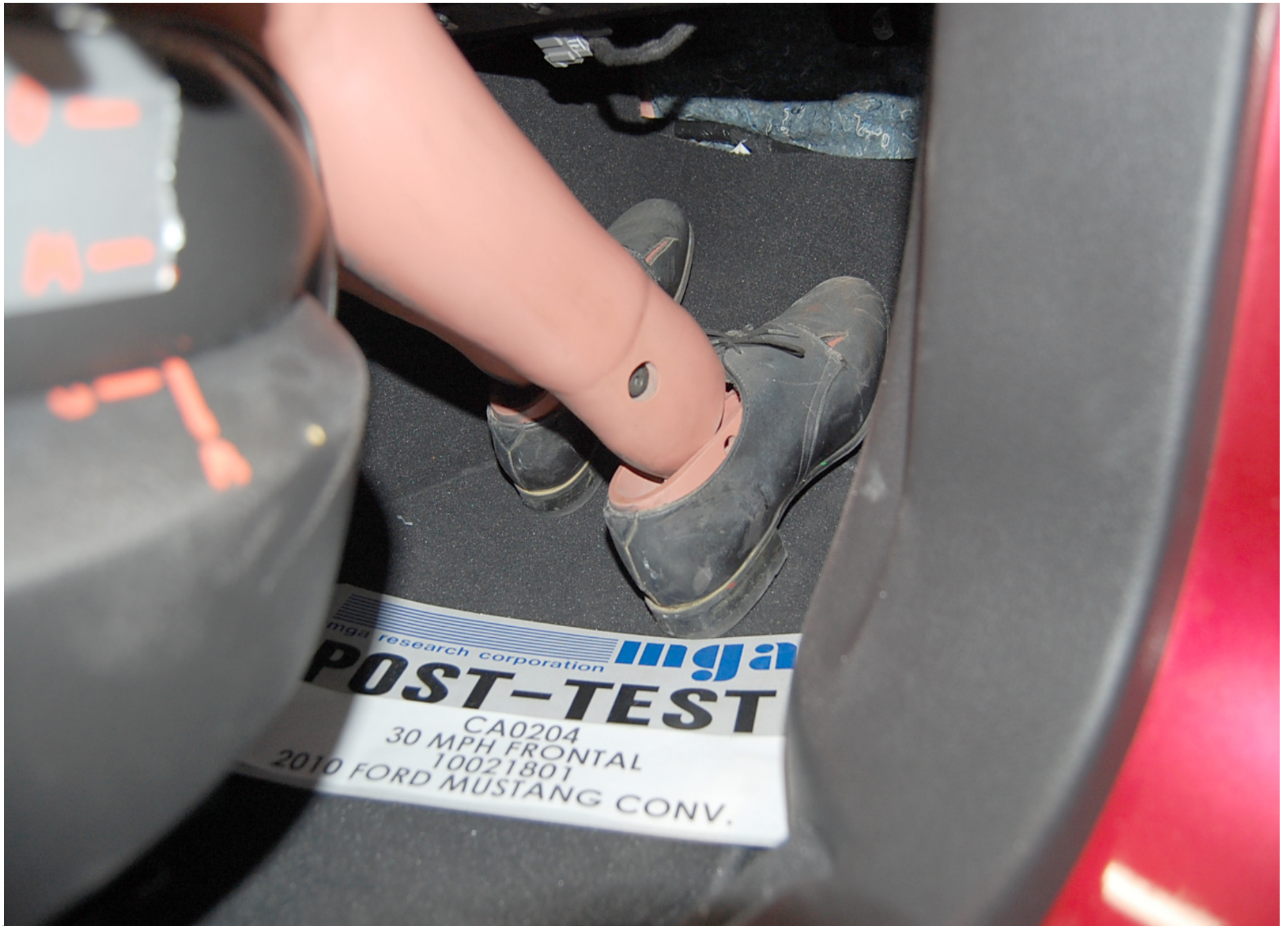
Post-Test Passenger Dummy Feet Position
