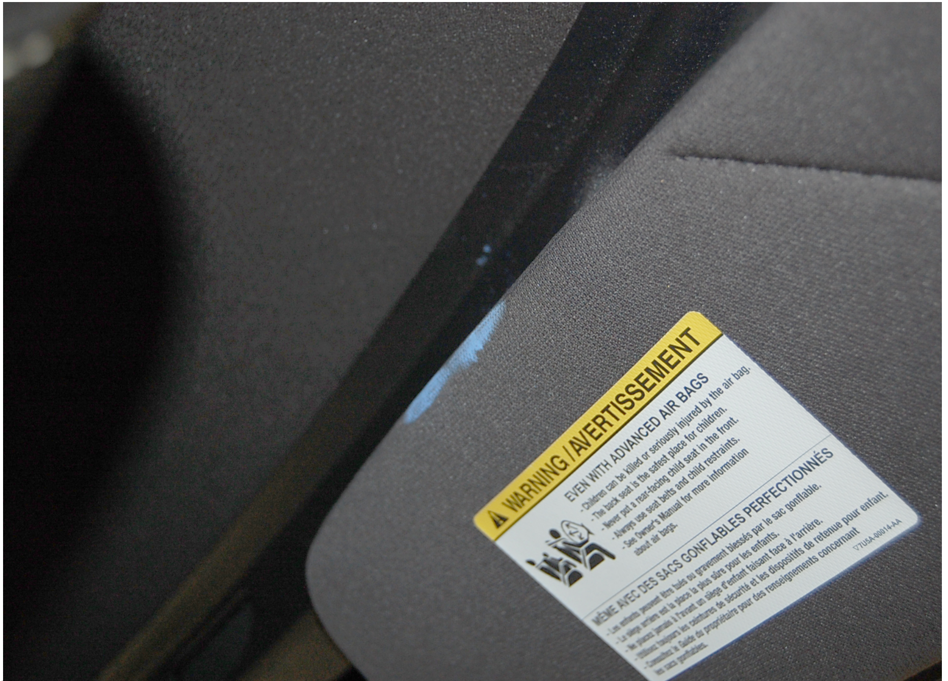
Post-Test Passenger Dummy Head Contact (visor)
