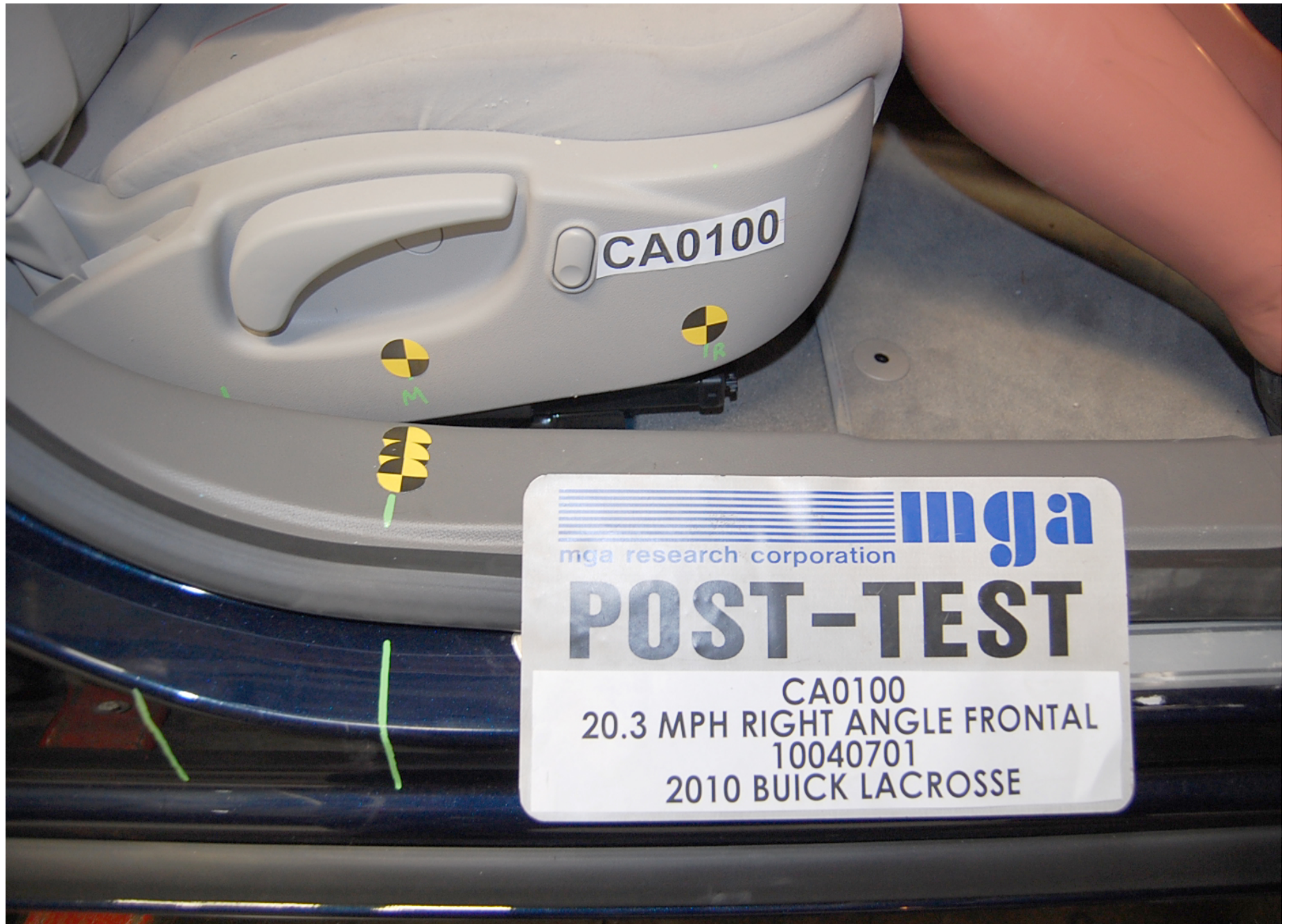
Post-Test Passenger Dummy Seat Position
