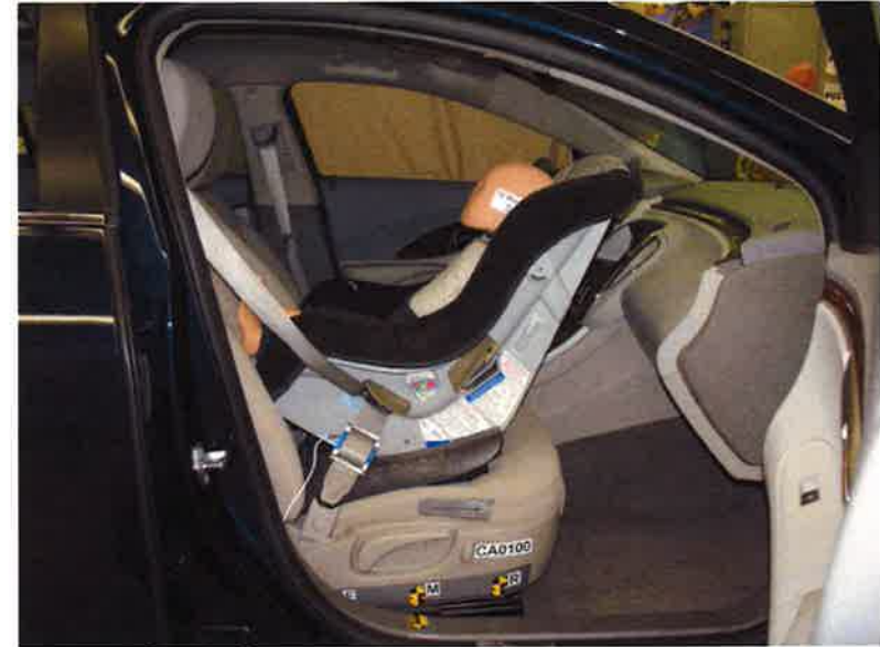
Century Encore Rear Facing Belted, Middle Seat Track
