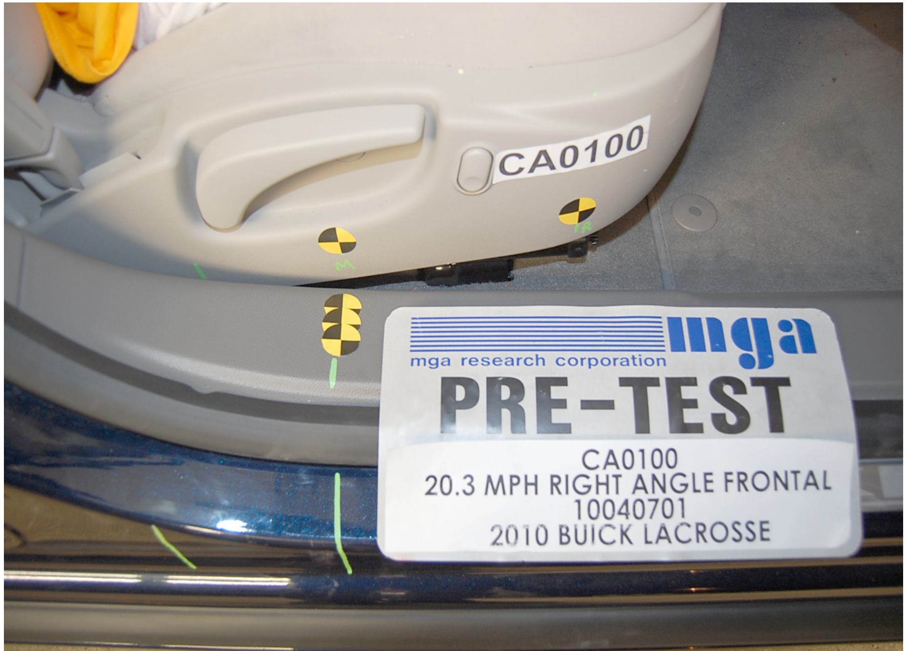
Pre-Test Passenger Dummy Seat Position
