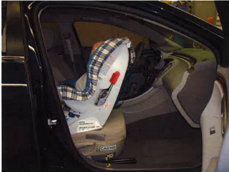
Britax Roundabout 161 Rear Facing Belted, Rearward Seat Track
