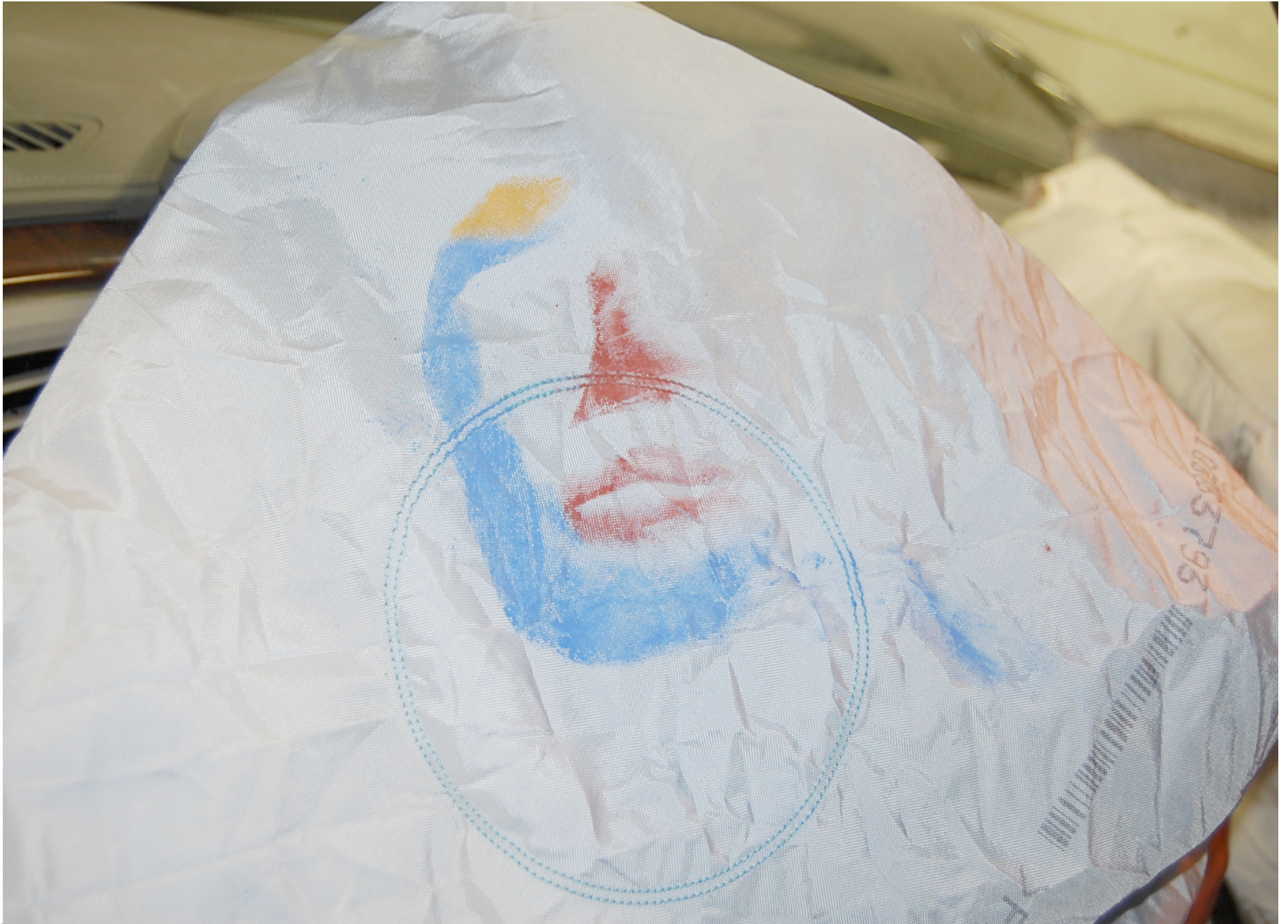
Post-Test Driver Dummy Airbag Contact
